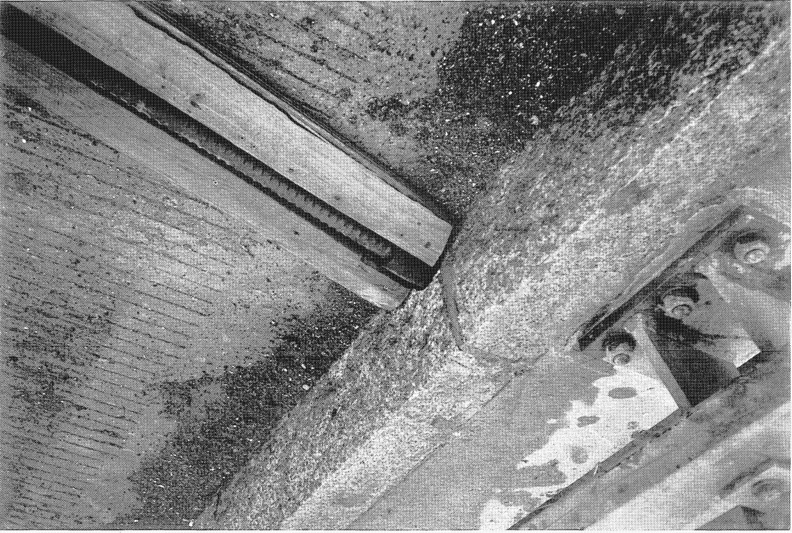
FIGURE 2-19 Overview of the Tension Loading System at the Deck Level
