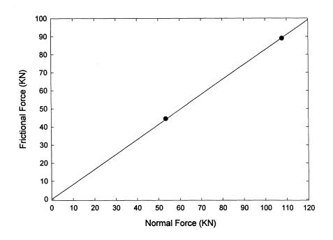
FIGURE 4-12: Normal force versus ultimate lateral capacity for Tests CB and CBL.
