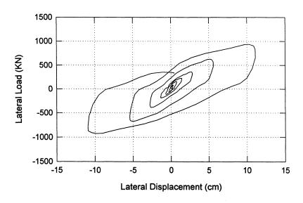
FIGURE 6-4: Measured load-displacement response for Test PCBSPI (pile-cap system with instrumented pile).
