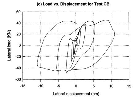
FIGURE 4-5: Load-displacement response for Test CB in prototype scale.
