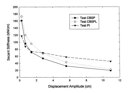
FIGURE 5-4: Stiffness versus displacement amplitude in prototype scale.
