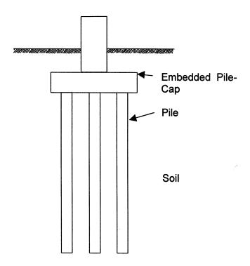
FIGURE 2-1: Pile foundation with embedded cap.
