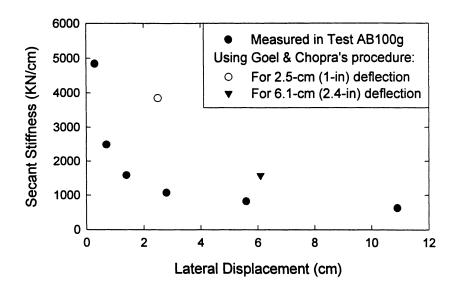
FIGURE 9-9: Measured and computed secant stiffnesses for Test AB100g.
