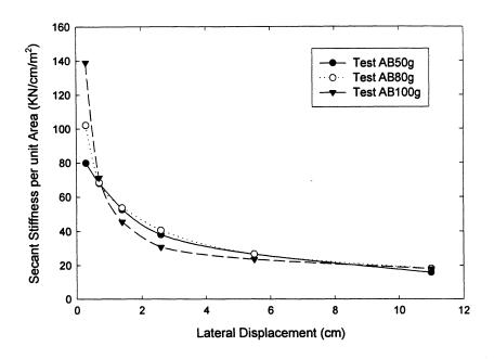
FIGURE 9-11: Measured secant stiffness per unit area for centrifuge tests on abutments.
