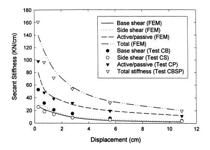
FIGURE 7-14: Measured and computed secant stiffness contributions versus displacement amplitude. (FE results are for Test CBSP with parameters in table 7-1).
