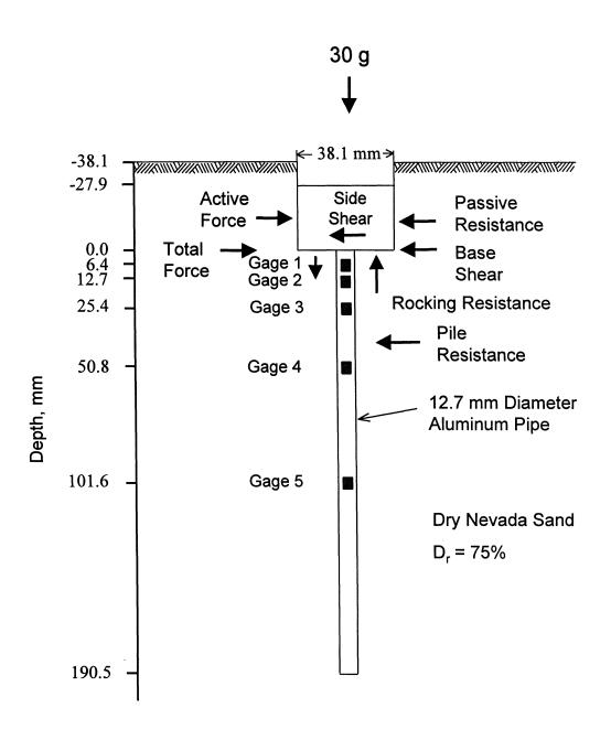
FIGURE 6-1: Model of pile-cap system used in Test PCBSPI.
