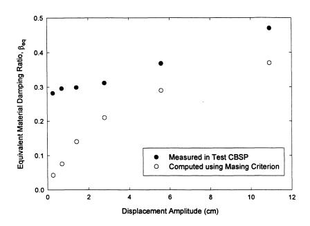
FIGURE 7-9: Measured and computed equivalent damping ratios for Test CBSP.
