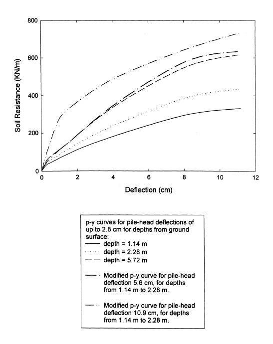
FIGURE 6-10: p-y Curves Used for Large Displacement Amplitudes.
