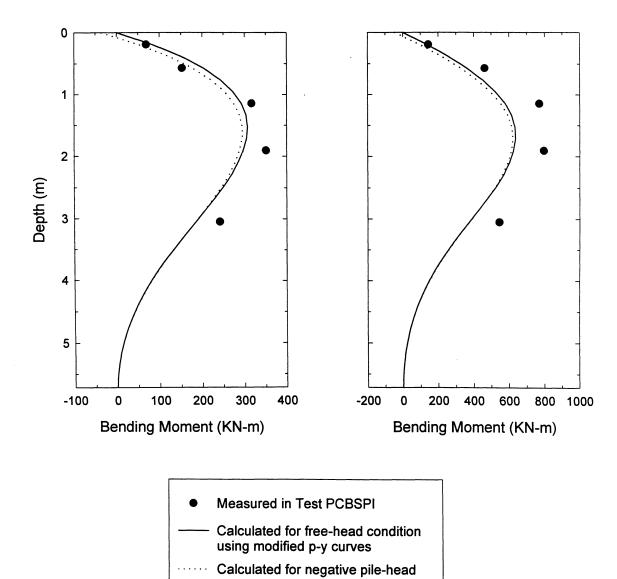
FIGURE 6-11: Measured and Calculated Bending Moments for Test PCBSPI at Large Displacements.
