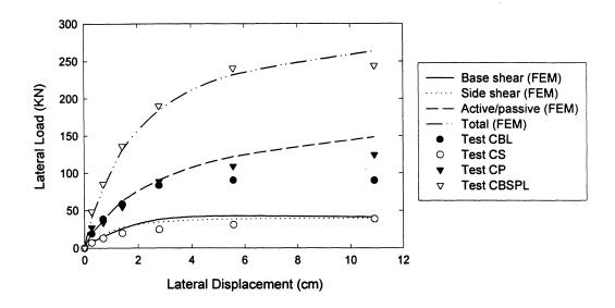
FIGURE 7-15: Measured and computed contributions to the load-displacement response of the cap. (FE results are for Test CBSPL with parameters in table 7-1).
