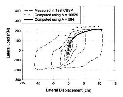
FIGURE 8-1: Measured and computed load-displacement response for Tests CBSP.
