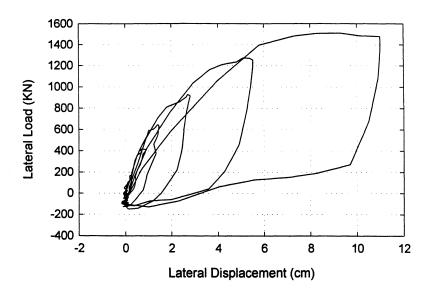
FIGURE 9-4: Measured load-displacement response for Test AB50g in prototype scale.
