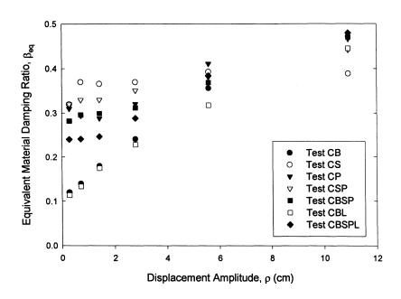
FIGURE 4-16: Measured equivalent damping ratio versus displacement amplitude.
