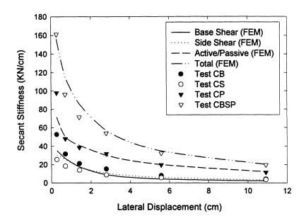
FIGURE 8-5: Measured and computed contributions to secant stiffness in Test CBSP (FEM analyses are with  $G=584~\sigma_o^{0.5}$ ).
