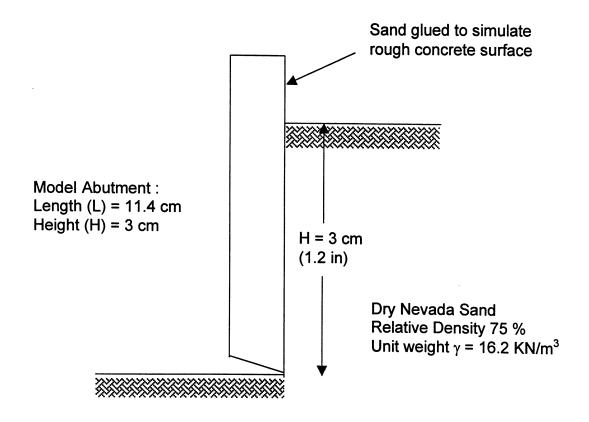
FIGURE 9-1: Schematic view of model abutment.
