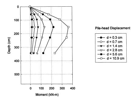
FIGURE 5-6: Measured prototype bending moments along the length of the pile in Test PI.
