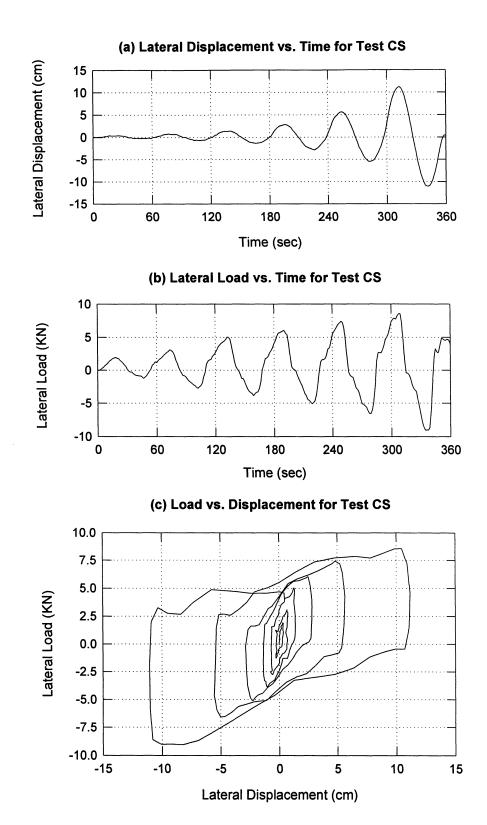
FIGURE 4-7: Load-displacement response for Test CS in prototype scale.
