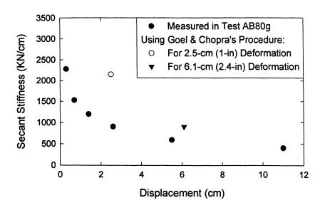
FIGURE 9-8: Measured and computed secant stiffnesses for Test AB80g.
