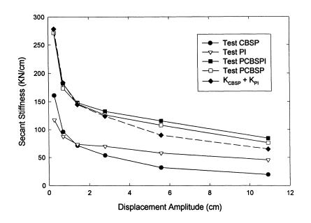
FIGURE 6-5: Measured secant stiffness versus displacement amplitude.
