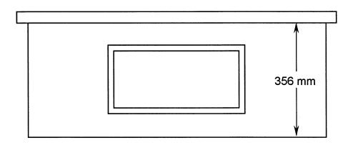
FIGURE 3-4: Model container used for centrifuge tests.
