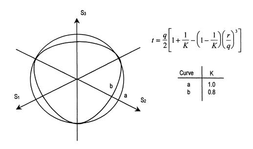
FIGURE 7-4: Modified Drucker-Prager/Cap model: typical yield/flow surfaces in the deviatoric plane (after Hibbit, Karlsson & Sorensen Inc., 1994).
