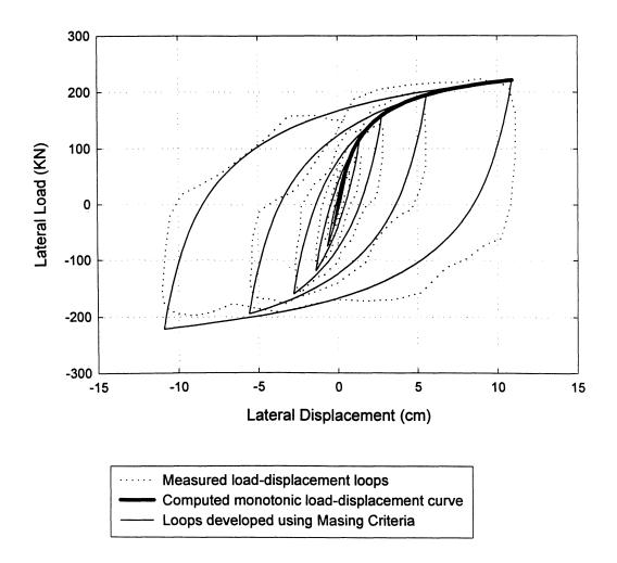
FIGURE 7-8: Load-displacement loops generated for Test CBSP from finite element results using Masing criterion.
