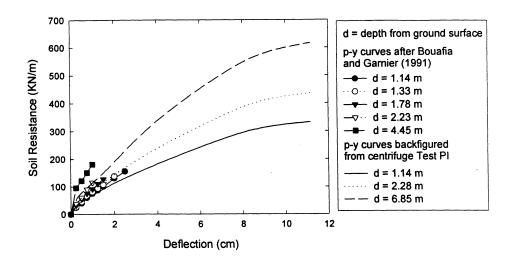
FIGURE 5-9: Comparison of p-y curves backfigured from centrifuge Test PI with the p-y curves modified after Bouafia and Garnier (1991).
