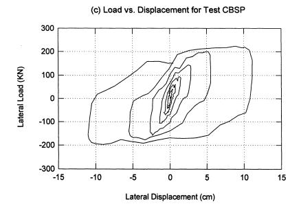
FIGURE 4-10: Load-displacement response for Test CBSP in prototype scale.
