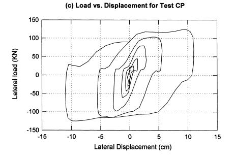
FIGURE 4-8: Load-displacement response for Test CP in prototype scale.
