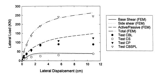
FIGURE 8-6: Measured and computed contribution to load-displacement response in Test CBSPL (FEM analyses are with  $G=584~\sigma_o^{0.5}$ ).
