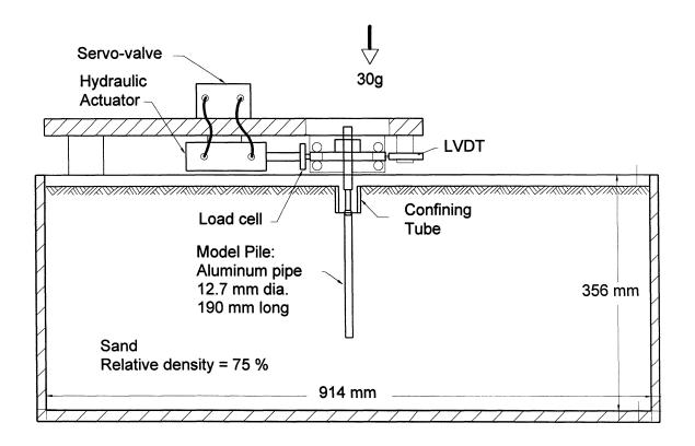
FIGURE 5-2: Set-up for centrifuge Test PI.
