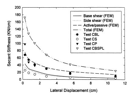
FIGURE 8-7: Measured and computed contributions to secant stiffness of Test CBSPL. (FEM analyses are with G = 584  $\sigma_o^{0.5}$ )
