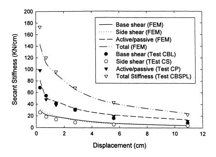
FIGURE 7-16: Measured and computed secant stiffness contributions versus displacement amplitude. (FE results are for Test CBSPL with parameters in table 7-1).
