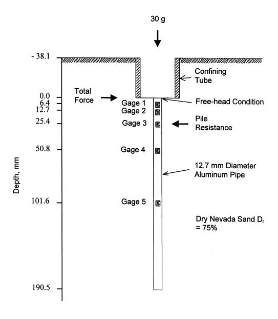
FIGURE 5-1: Model pile used in Test PI.
