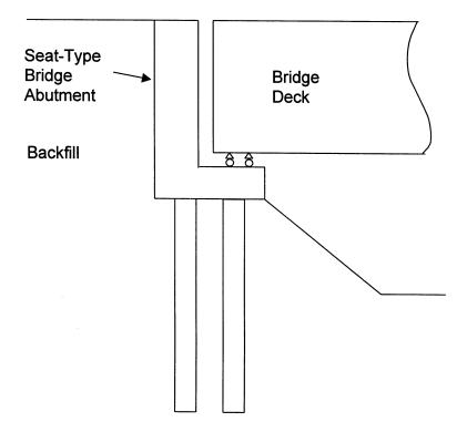
FIGURE 2-2: Bridge abutment in dense dry sand subjected to lateral load.
