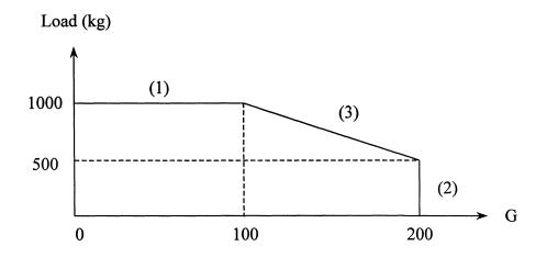
FIGURE 2-5: Performance envelope for RPI centrifuge (after Elgamal et al., 1996).
