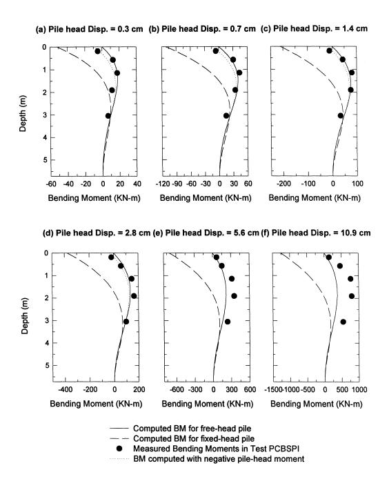
FIGURE 6-9: Measured bending moments for Test PCBSPI superimposed on moment distributions calculated using p-y curves obtained from Test PI for free-head and fixed-head conditions.
