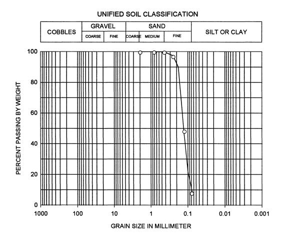
FIGURE 3-3: Grain size distribution for Nevada sand (after Arulmoli et al., 1992).
