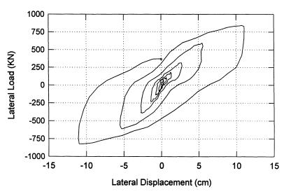
FIGURE 6-3: Measured load-displacement response for Test PCBSP in prototype scale (pile-cap system).
