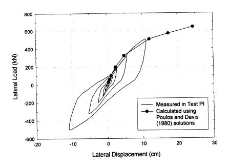
FIGURE 5-12: Measured and calculated load-deflection curves for Test PI.
