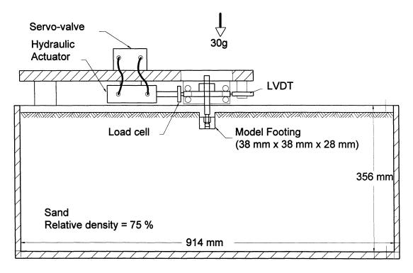
FIGURE 4-3: General set-up for centrifuge tests on embedded footing (pile cap).
