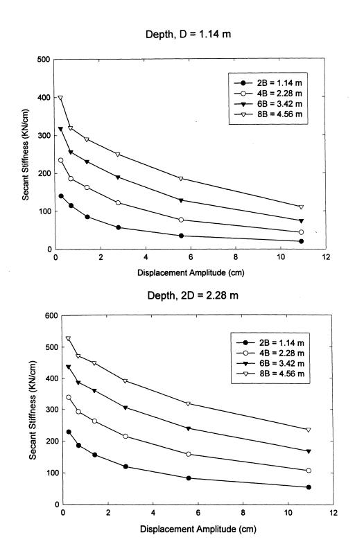
FIGURE 7-19: Results of parametric FE analyses conducted to study the influence of footing geometry on lateral secant stiffness. (FE analyses performed with G = 1.73 MPa).
