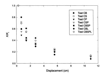
FIGURE 4-14: Measured normalized secant stiffness versus displacement amplitude.
