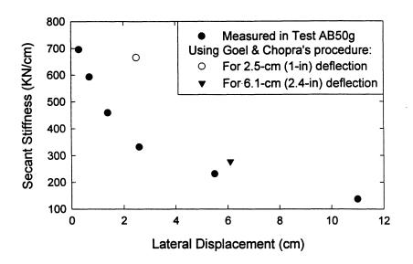
FIGURE 9-7: Measured and computed secant stiffnesses for Test AB50g.
