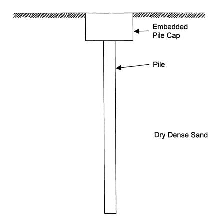
FIGURE 3-1: Pile foundation with embedded cap
