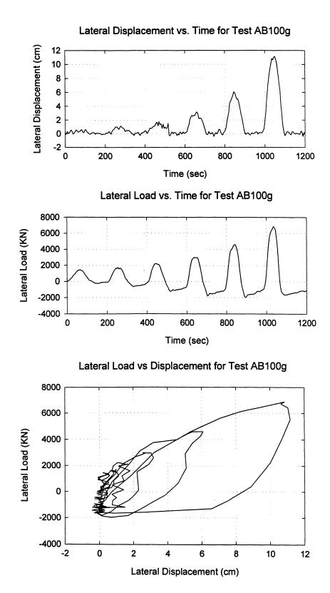
FIGURE 9-6: Measured load-displacement response for Test AB100g in prototype scale.
