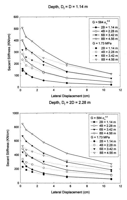
FIGURE 8-8: Results of parametric FE analyses conducted to study the influence of footing geometry on lateral secant stiffness.
