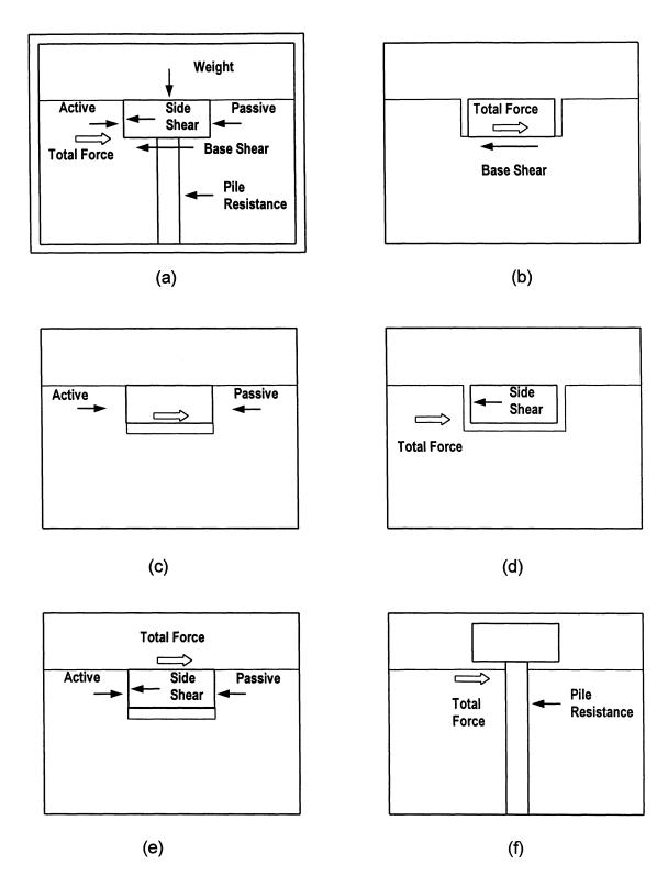
FIGURE 3-2: Isolation of forces contributing to lateral response of pile-cap system.
