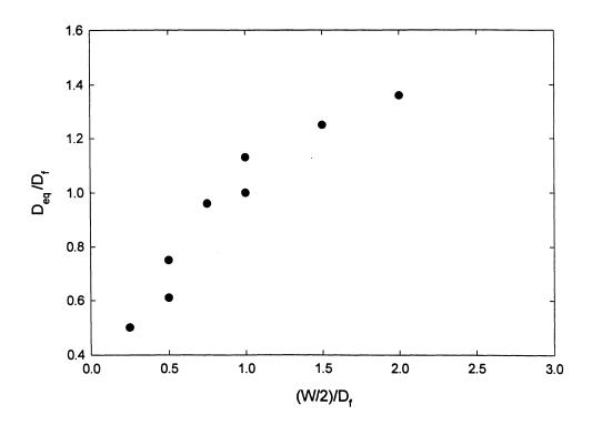
FIGURE 8-9: Normalized equivalent depth versus normalized side of the footing (m/D $_{\rm f}$  = 0.26).
