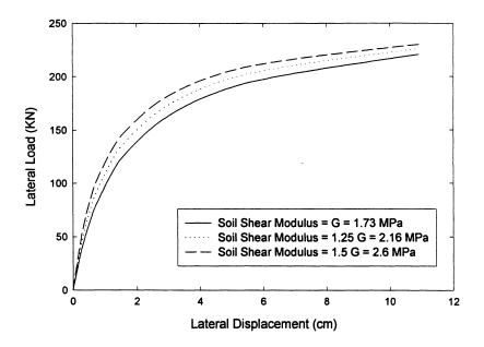
FIGURE 7-17: Computed load-displacement responses for Test CBSP with different soil shear moduli.
