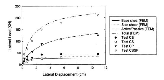
FIGURE 7-13: Measured and computed contributions to the load-displacement response of the cap. (FE results are for Test CBSP with parameters in table 7-1).
