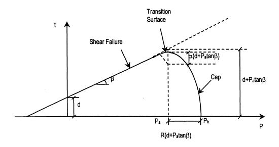
FIGURE 7-3: Modified Drucker-Prager/Cap model: yield surface in the *p-t* plane (after Hibbit, Karlsson & Sorensen Inc., 1994).
