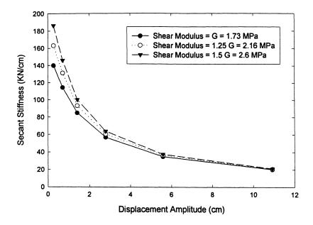
FIGURE 7-18: Computed horizontal secant stiffness versus displacement amplitude for Test CBSP with different soil shear moduli.
