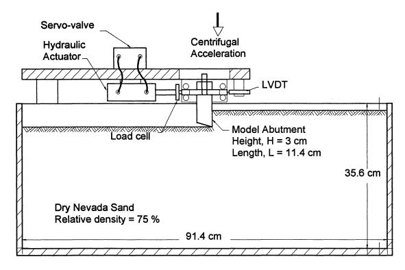
FIGURE 9-2: General setup for centrifuge tests on abutments.
