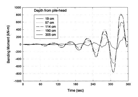
FIGURE 6-7: Measured bending moments versus time in Test PCBSPI in prototype scale.
