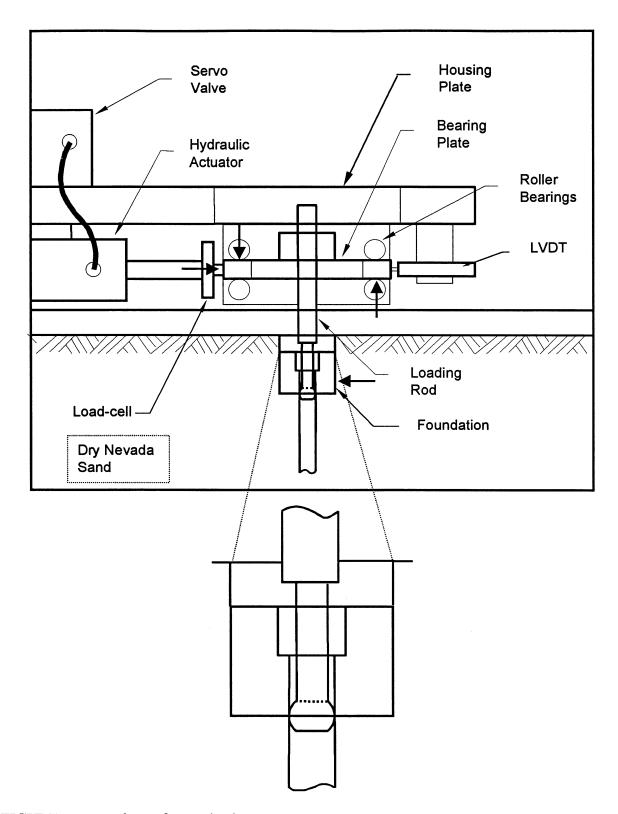
FIGURE 3-5: Load transfer mechanism.
