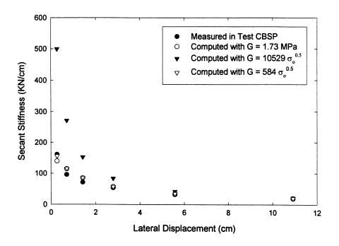
FIGURE 8-3: Measured and computed secant stiffness for Test CBSP.
