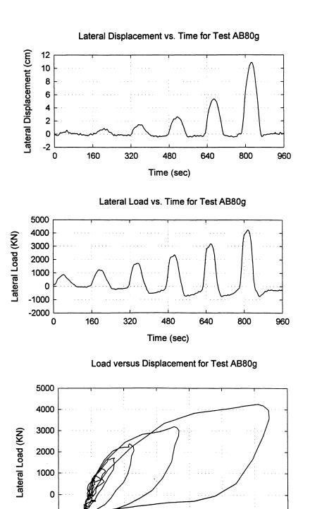
FIGURE 9-5: Measured load displacement response for Test AB80g in prototype scale.
