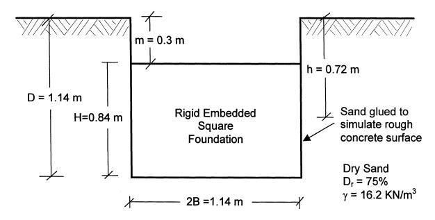
FIGURE 4-2: Dimensions of the footing/cap model used in the centrifuge tests in prototype scale.
