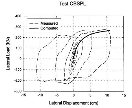
FIGURE 7-7: Measured and computed load-displacement response for Tests CBSP and CBSPL.
