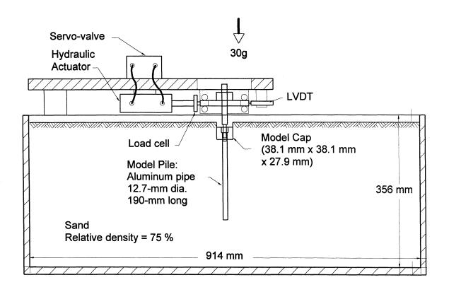
FIGURE 6-2: Set-up for centrifuge tests on pile-cap system.
