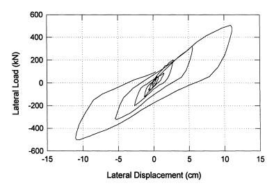
FIGURE 5-3: Load-displacement response for Test PI in prototype scale.
