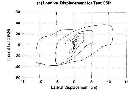
FIGURE 4-9: Load-displacement response for Test CSP in prototype scale.
