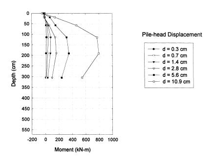
FIGURE 6-8: Measured Bending Moments along the Length of the Pile in Test PCBSPI.
