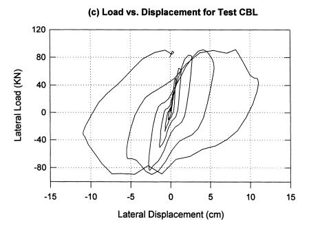
FIGURE 4-6: Load-displacement response for Test CBL in prototype scale.
