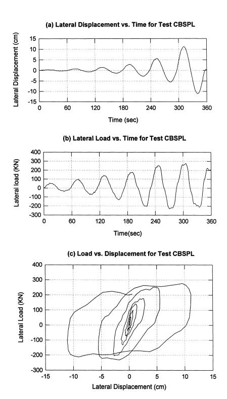
FIGURE 4-11: Load-displacement response for Test CBSPL in prototype scale.
