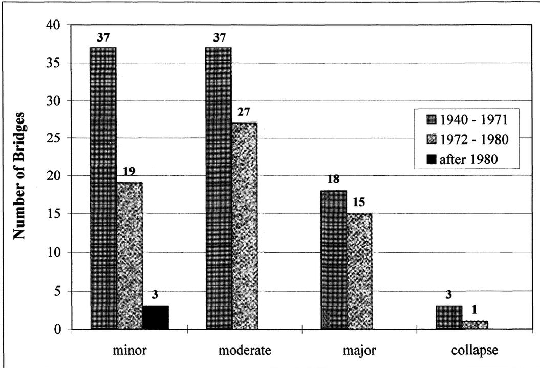
**FIGURE 4-13** Distribution of Damaged Bridges by Design Year and Damage State (*correlation data set*)
