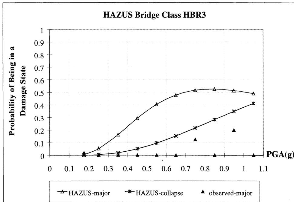
**FIGURE 4-27.b** Comparison of Damage Probabilities from Data to HAZUS Fragility Functions, Major damage and Collapse
