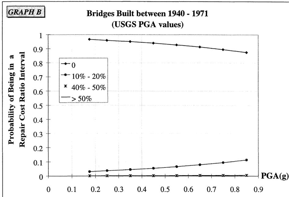
**FIGURE 4-48** Empirical Fragility Curves for Bridges Built between 1940 and 1971
