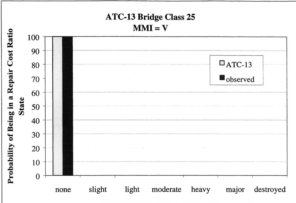
**FIGURE 4-50.a** Comparison of Observed and Predicted Probabilities of being in a given Repair Cost Ratio State, ATC-13 Bridge Class 25 MMI V
