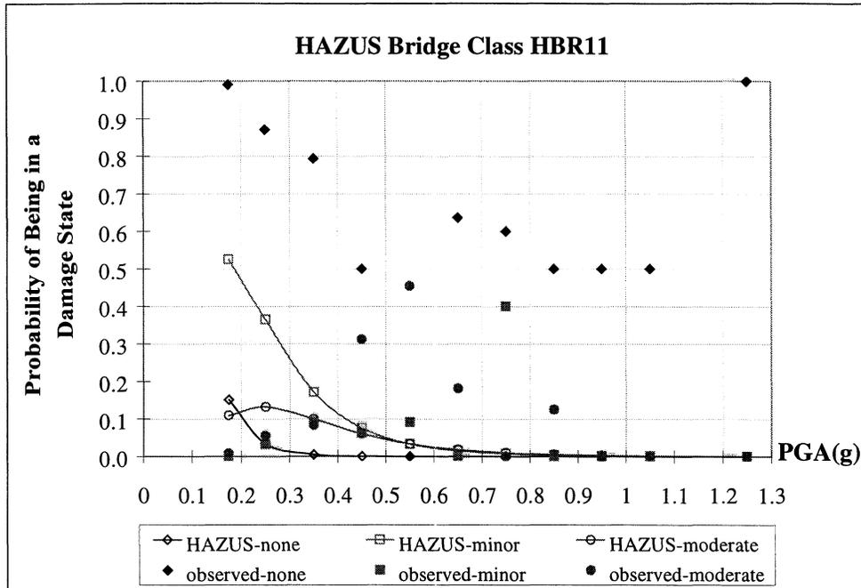
**FIGURE 4-30.a** Comparison of Damage Probabilities from Data to HAZUS Fragility Functions, No Damage, Minor Damage and Moderate Damage
