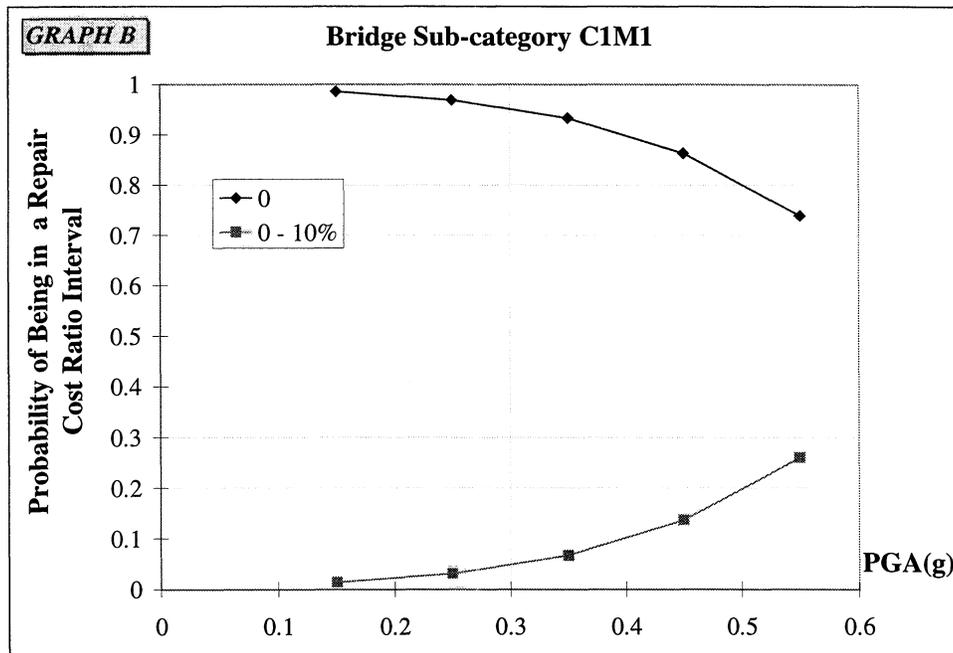
**FIGURE 3-25** Empirical Fragility Curves for Multiple Span Bridges with Monolithic Type Abutments and Multiple Column Bents (Sub-category C1M1), Repair Cost Ratio
