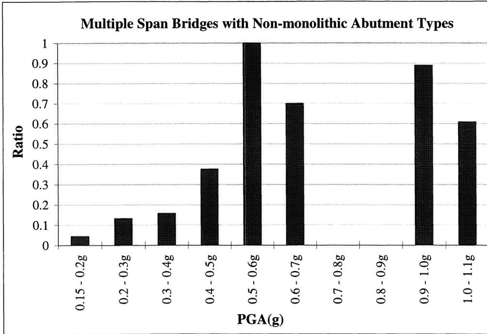
**FIGURE 4-16.b** Comparison of Damaged Bridges with Non-monolithic Abutment Types to Total Number of Bridges with Non-monolithic Abutment Types
