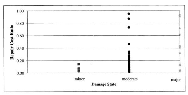
FIGURE 4-43 Distribution of Repair Cost Ratio by Damage State
