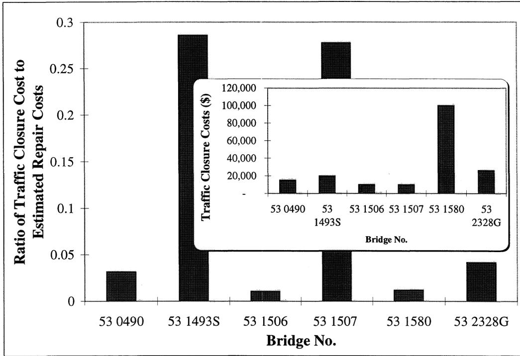
**FIGURE 4-42** Ratio of Traffic Closure Cost to Estimated Repair Cost - Major Damage
