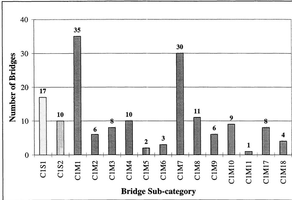
**FIGURE 4-11** Distribution of Damaged Bridges by Bridge Sub-category (*correlation data set*)<sup>1</sup>
