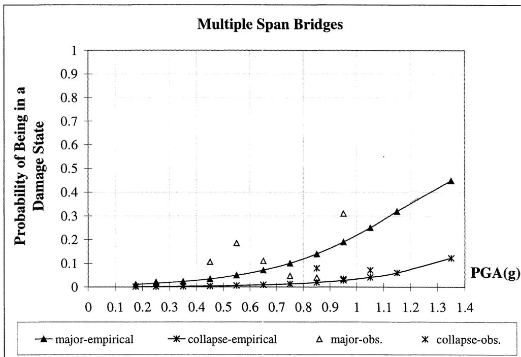
**FIGURE 4-21.b** Empirical Fragility Curves and Observed Data for Multiple Span Bridges - Major Damage and Collapse
