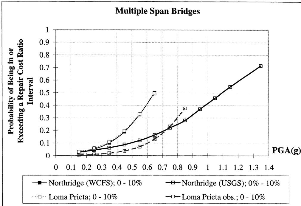
**FIGURE 5-16** Empirical Fragility Curves for Multiple Span Bridges obtained from the Loma Prieta and Northridge Earthquakes (*correlation data set*) - Repair Cost Ratio
