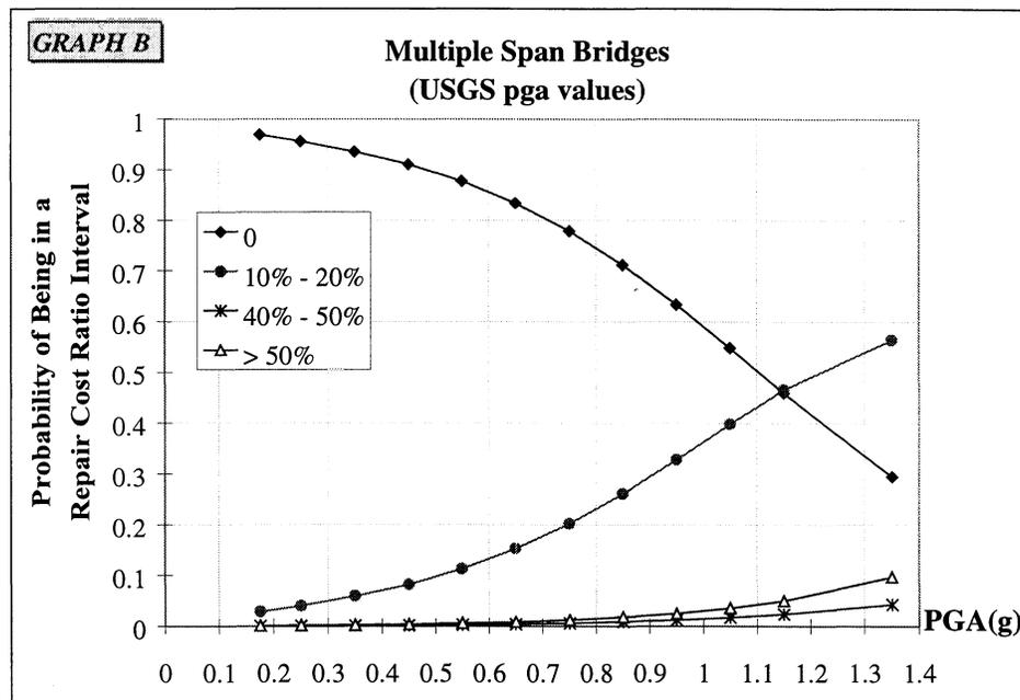
**FIGURE 4-44** Empirical Fragility Curves for Multiple Span Bridges, Repair Cost Ratio
