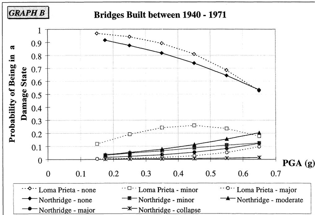
**FIGURE 5-8** Empirical Fragility Curves for Bridges Built between 1940 and 1971 in the Loma Prieta and Northridge Earthquakes
