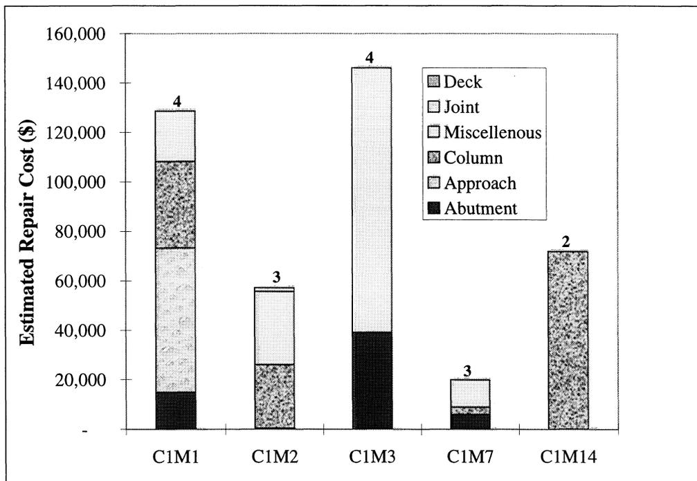
**FIGURE 3-23** Distribution of Estimated Repair Cost by Bridge Components for Different Bridge Sub-categories
