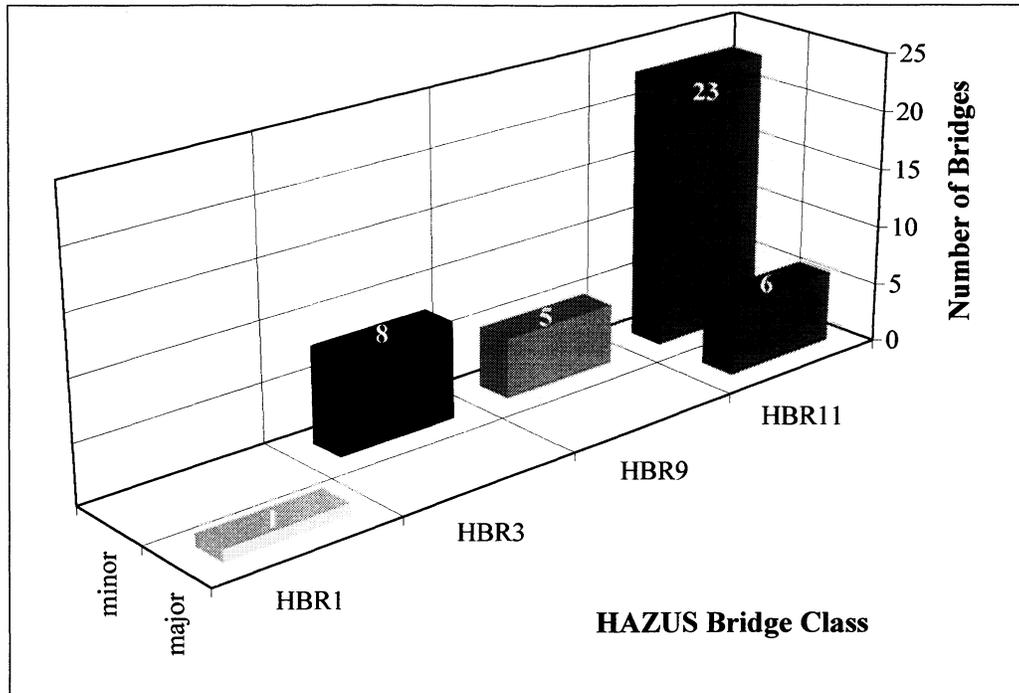
**FIGURE 3-14** Distribution of Damaged Concrete Bridges by HAZUS Bridge Classification and Damage State for  $PGA \geq 0.10g$
