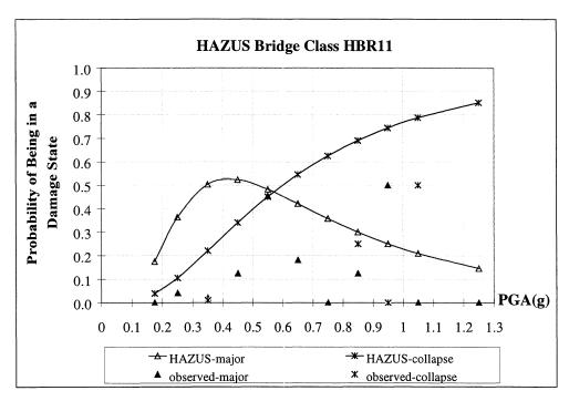
FIGURE 4-30.b Comparison of Damage Probabilities from Data to HAZUS Fragility Functions, Major Damage and Collapse
