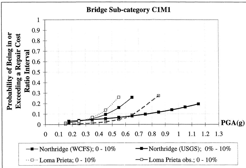
**FIGURE 5-17** Empirical Fragility Curves for Bridges in Sub-category C1M1 obtained from the Loma Prieta and Northridge Earthquakes (*correlation data set*) - Repair Cost Ratio
