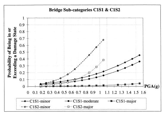
FIGURE 4-57 Empirical Fragility Curves for Single Span Bridges with Monolithic (C1S1) and Non-monolithic (C1S2) Abutments
