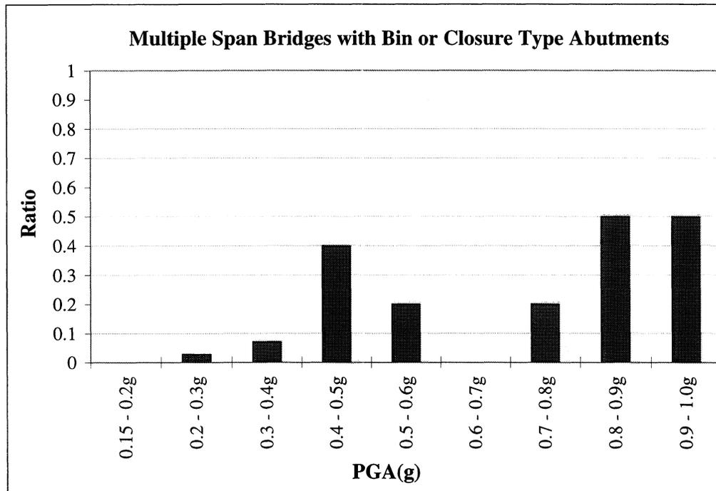
**FIGURE 4-16.c** Comparison of Damaged Bridges with Partial Abutment Types to Total Number of Bridges with Partial Abutment Types
