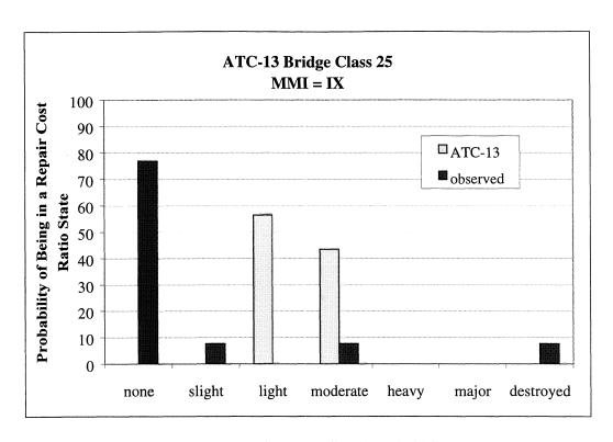
FIGURE 4-50.e Comparison of Observed and Predicted Probabilities of being in a given Repair
