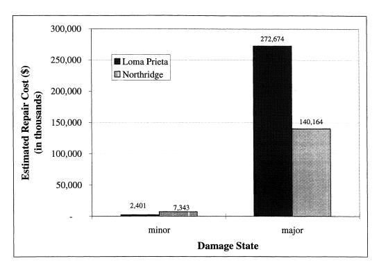
FIGURE 5-14 Estimated Repair Costs in the Loma Prieta and Northridge Earthquakes
