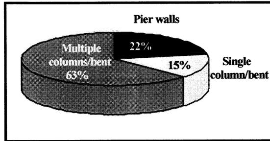
**FIGURE 4-4.b** Distribution of Multiple Span Bridges by Column Bent Type<sup>2</sup> (*correlation data set*)
