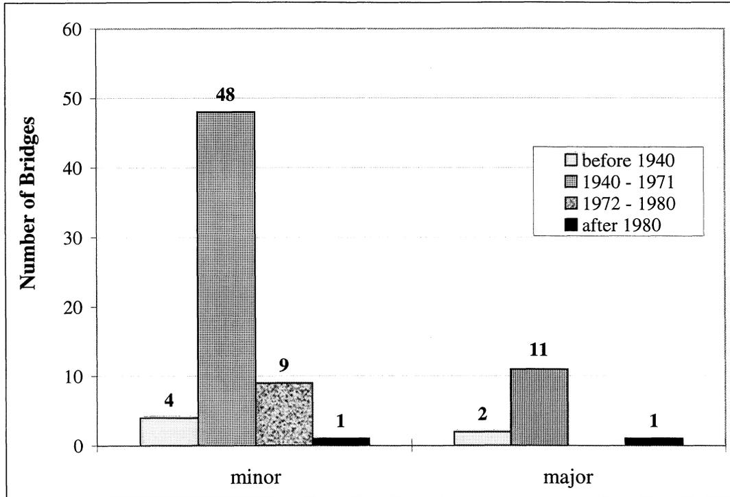
**FIGURE 3-10** Distribution of All Damaged Bridges by Design Year
