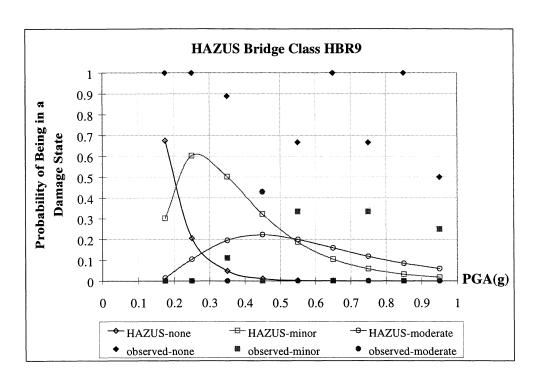
FIGURE 4-29.a Comparison of Damage Probabilities from Data to HAZUS Fragility Functions,
