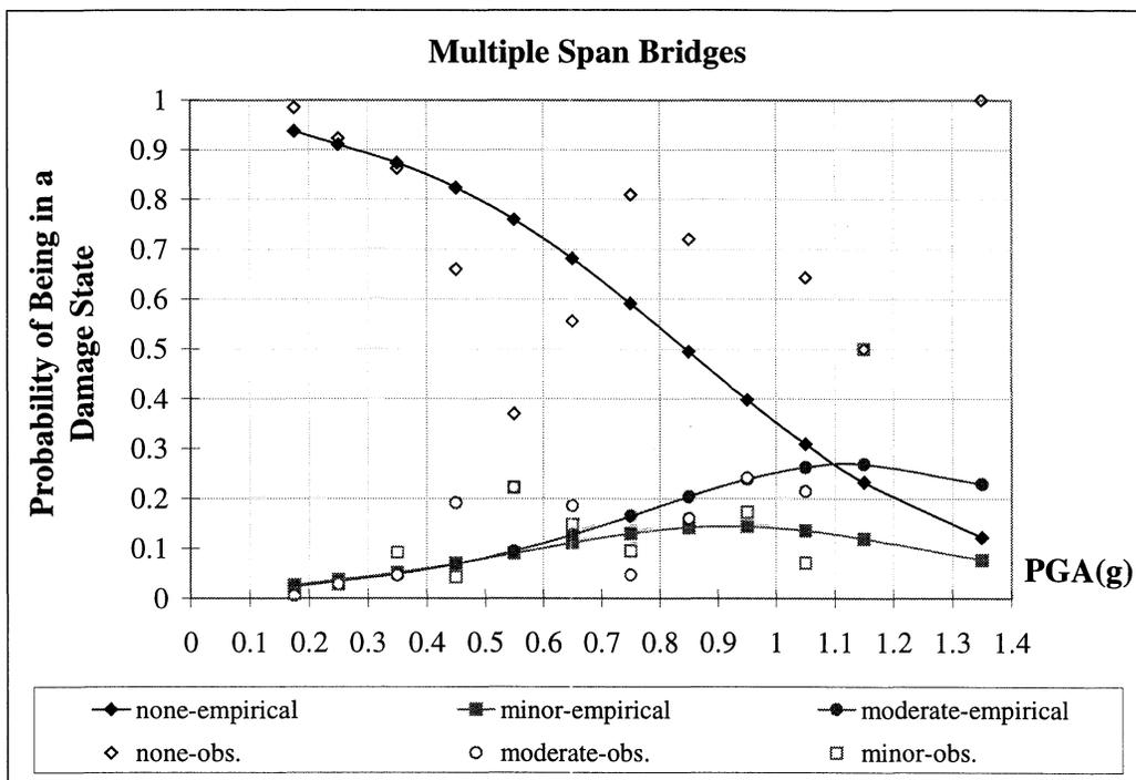
**FIGURE 4-21.a** Empirical Fragility Curves and Observed Data for Multiple Span Bridges – No Damage, Minor Damage and Moderate Damage
