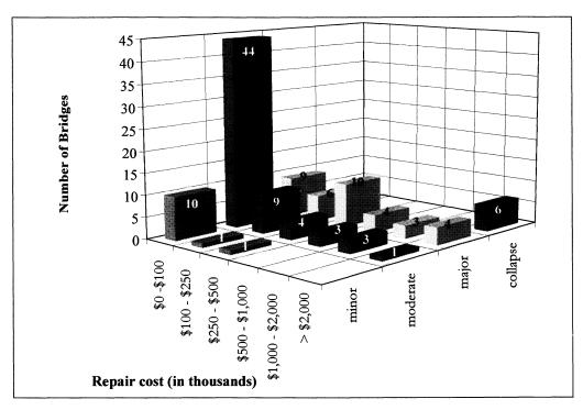
FIGURE 4-37 Distribution of All Damaged Bridges by Repair Cost and Damage State
