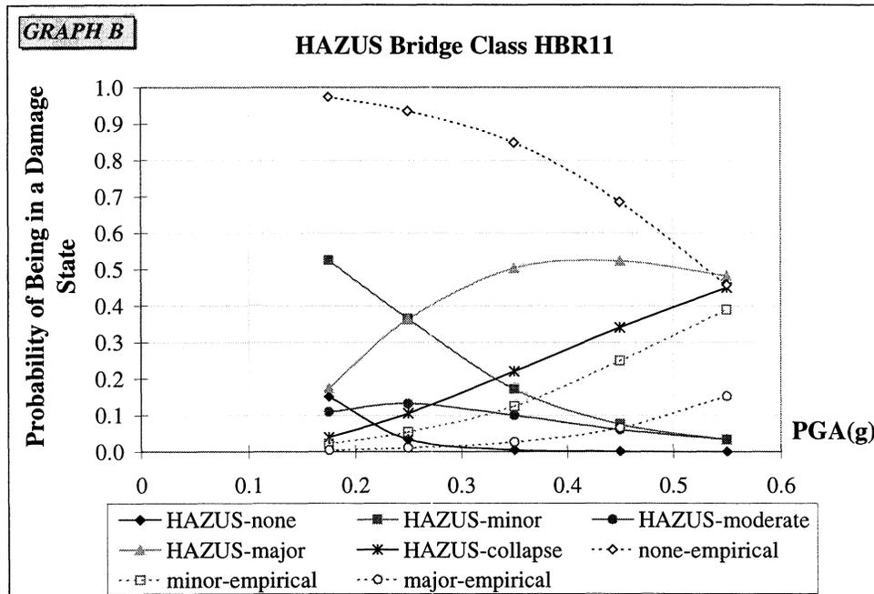
**FIGURE 3-20** Comparison between the Empirical and the HAZUS Fragility Curves for HAZUS Bridge Class HBR11
