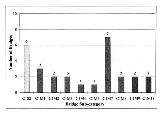
FIGURE 3-13 Distribution of Damaged Bridges by Bridge Sub-Categories (correlation data set)
