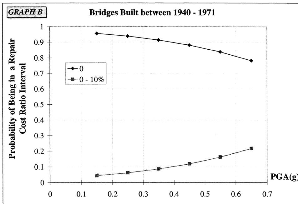
**FIGURE 3-26** Empirical Fragility Curves for Bridges Built between 1940 and 1971, Repair Cost Ratio
