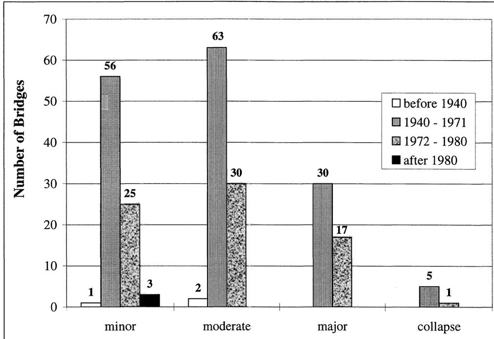
**FIGURE 4-9** Distribution of All Damaged Bridges by Design Year and Damage State
