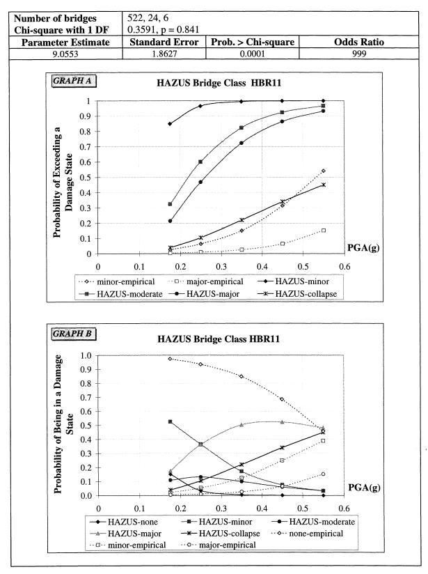
FIGURE 3-20 Comparison between the Empirical and the HAZUS Fragility Curves for HAZUS
