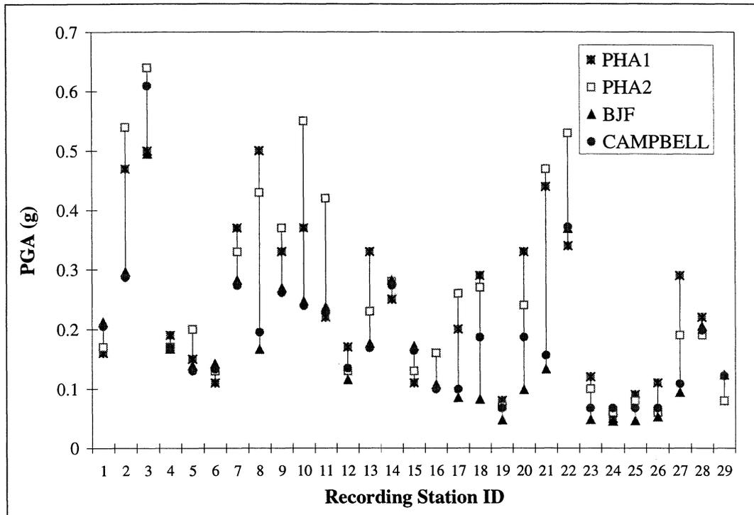
**FIGURE 3-27** Recorded and Estimated PGA Levels at Sample Recording Stations - Loma Prieta Earthquake
