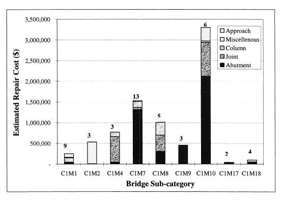
FIGURE 4-40 Distribution of Estimated Repair Cost by Bridge Components for Different
