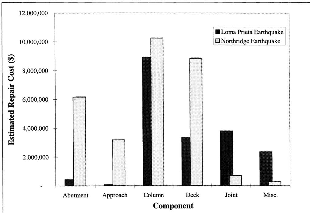
**FIGURE 5-15** Estimated Component Repair Costs in the Loma Prieta and Northridge Earthquakes
