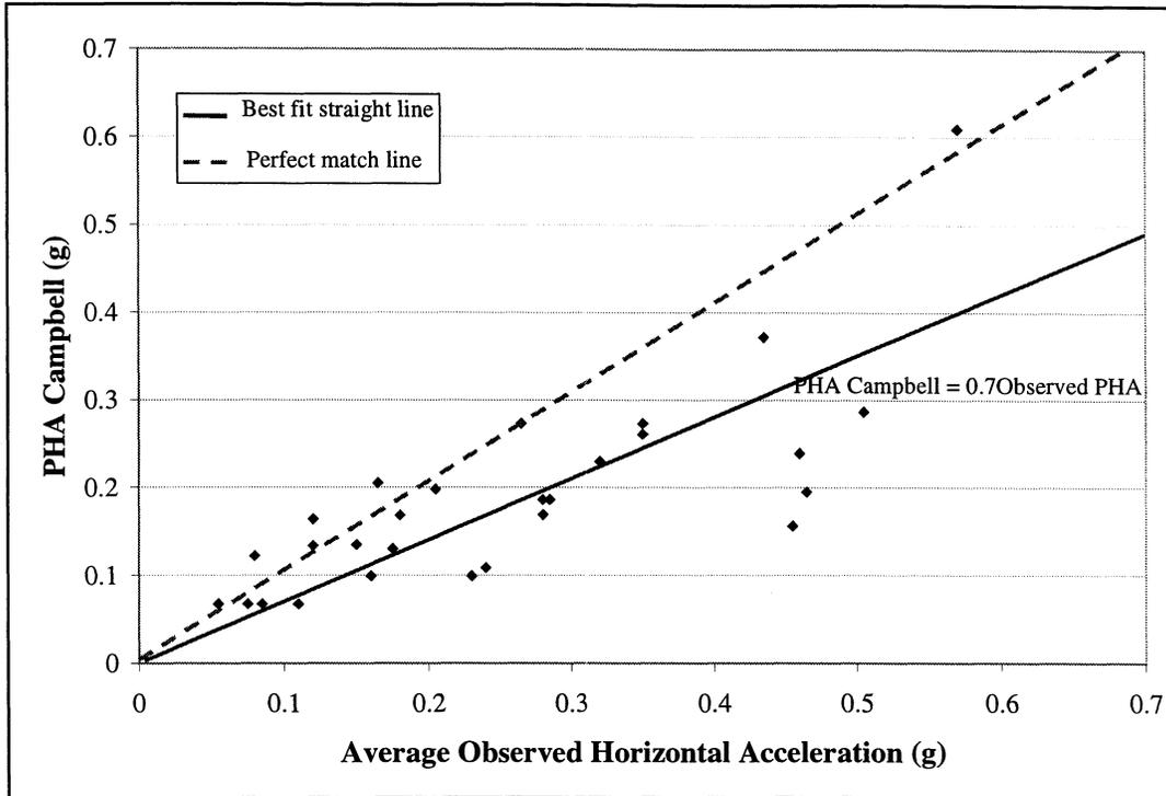
**FIGURE 3-3** Comparison of Recorded and Estimated PGA Levels, Loma Prieta Earthquake
