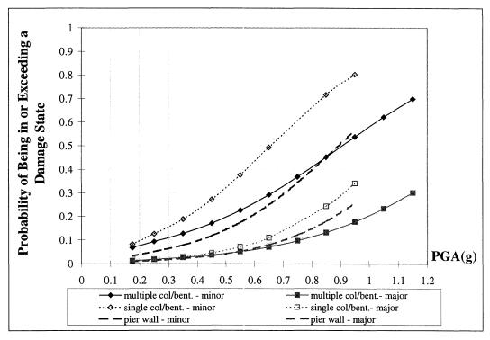
FIGURE 4-56 Performance Comparison of Different Types of Column Bents – Minor Damage and Major Damage
