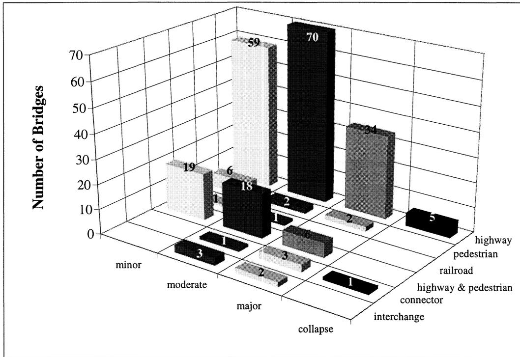
**FIGURE 4-8** Distribution of All Damaged Bridges by Service Type and Damage State
