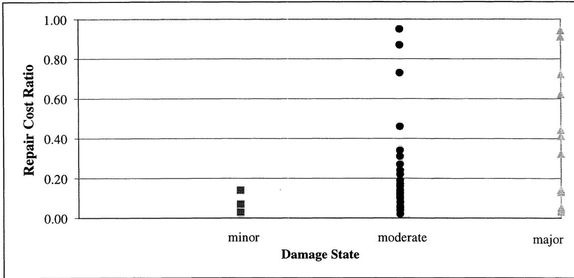
**FIGURE 4-43** Distribution of Repair Cost Ratio by Damage State
