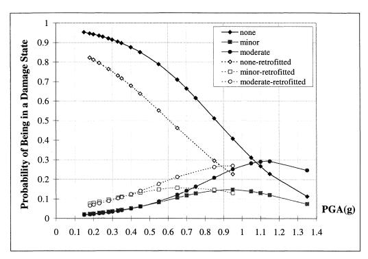
**FIGURE 4-26.a** Comparison of Empirical Fragility Curves for Retrofitted and Unretrofitted Bridges - No Damage, Minor Damage and Moderate Damage
