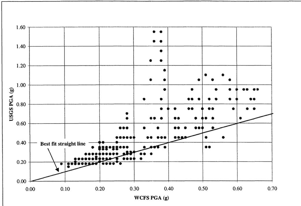
**FIGURE 4-51** PGA Values Reported by USGS [1994] and WCFS [1995] – Northridge Earthquake
