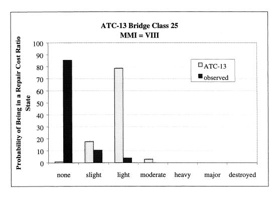
FIGURE 4-50.d Comparison of Observed and Predicted Probabilities of being in a given Repair
