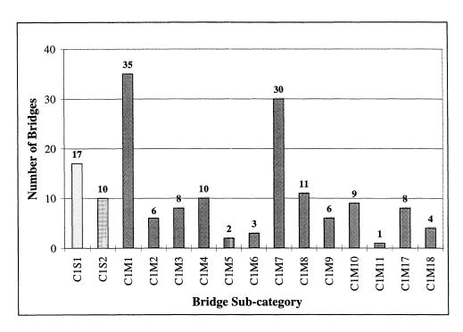
FIGURE 4-11 Distribution of Damaged Bridges by Bridge Sub-category (correlation data set)<sup>1</sup>
