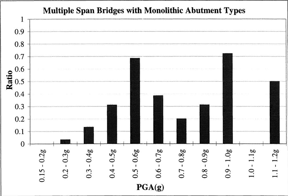
**FIGURE 4-16.a** Comparison of Damaged Bridges with Monolithic Abutment Types to Total Number of Bridges with Monolithic Abutment Types
