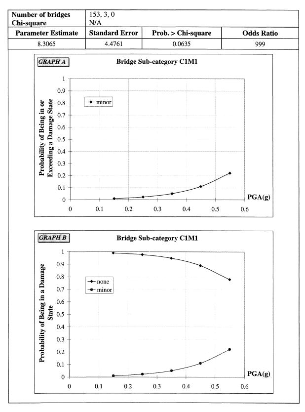
**FIGURE 3-18** Empirical Fragility Curves for Multiple Span Bridges with Monolithic Type Abutments, Continuous Spans and Multiple Column Bents (Sub-category C1M1)
