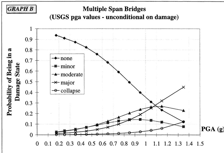
**FIGURE 4-19** Empirical Fragility Curves for Multiple Span Bridges, Unconditional on Damage
