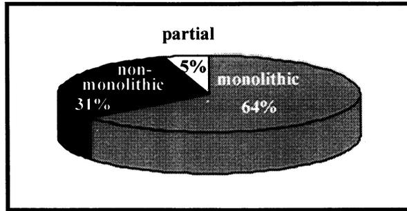
**FIGURE 4-3** Distribution of Single Span Bridges by Abutment Type (*correlation data set*)<sup>1</sup>
