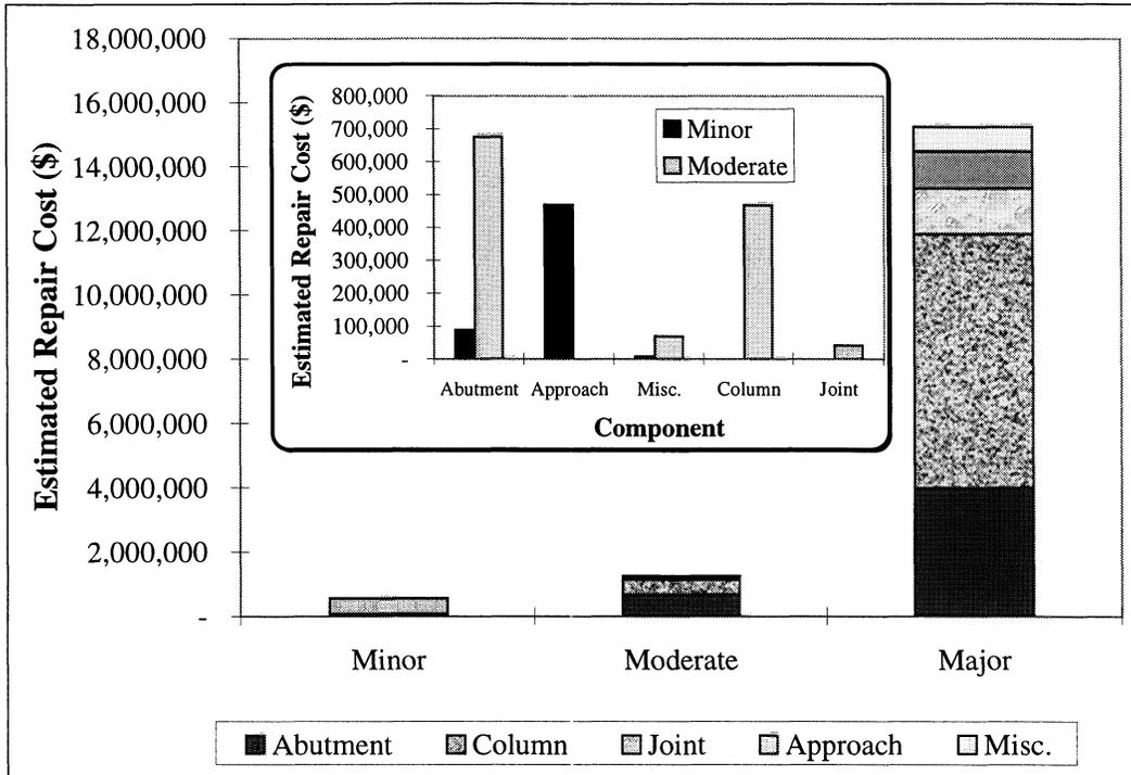
**FIGURE 4-39** Distribution of Estimated Repair Cost by Bridge Components for Different Damage States
