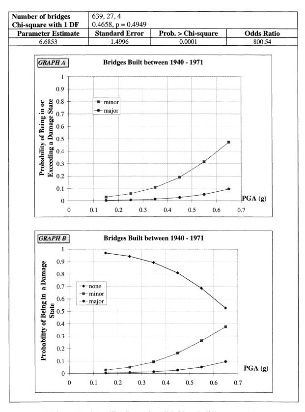
FIGURE 3-19 Empirical Fragility Curves for All Bridges Built between 1940 and 1971
