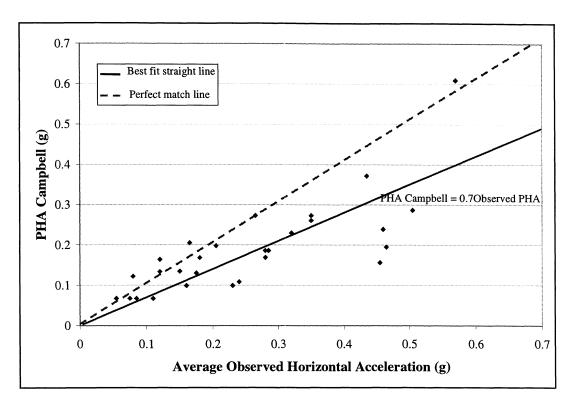
FIGURE 3-3 Comparison of Recorded and Estimated PGA Levels, Loma Prieta Earthquake
