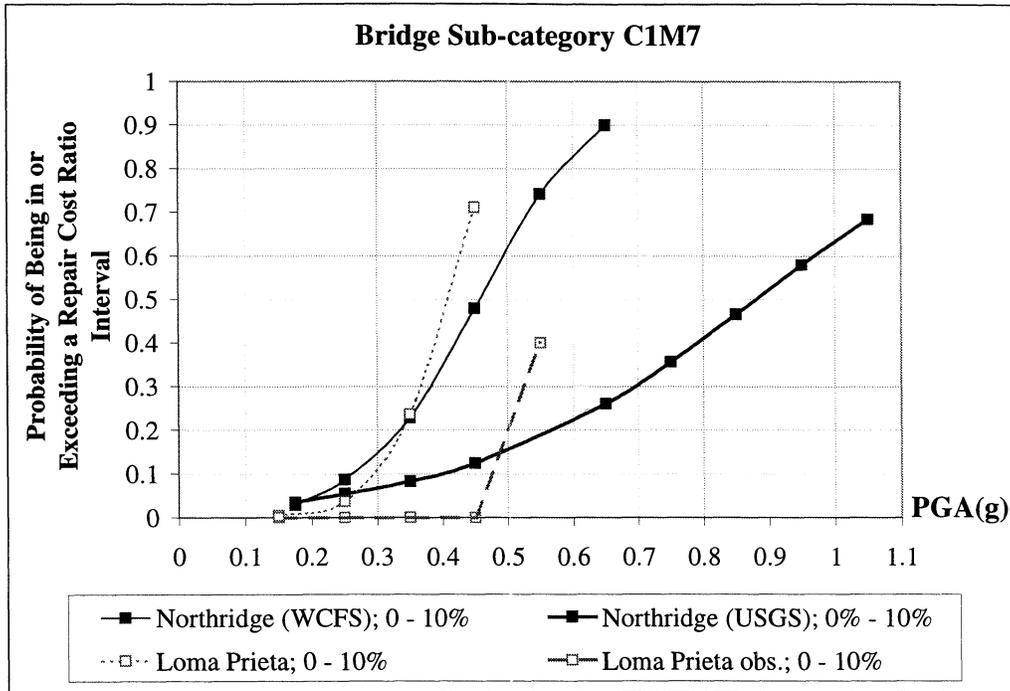
**FIGURE 5-18** Empirical Fragility Curves for Bridges in Sub-category C1M7 obtained from the Loma Prieta and Northridge Earthquakes (*correlation data set*) - Repair Cost Ratio
