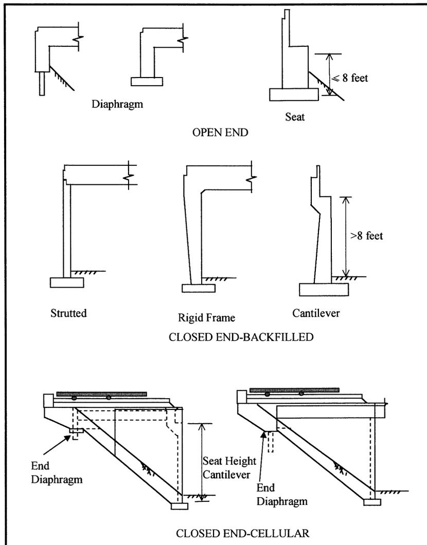
**FIGURE 2-2** Different Abutment Types Referred in Table 2-2
