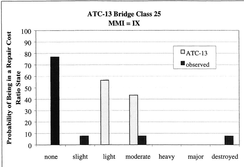
**FIGURE 4-50.e** Comparison of Observed and Predicted Probabilities of being in a given Repair Cost Ratio State, ATC-13 Bridge Class 25 MMI IX
