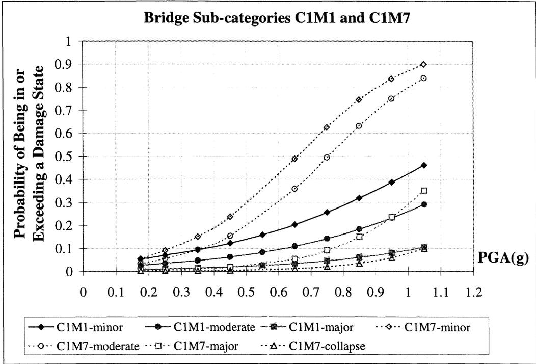
**FIGURE 4-60** Empirical Fragility Curves for Sub-categories C1M1 and C1M7
