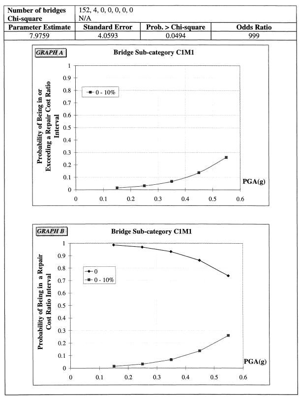
**FIGURE 3-25** Empirical Fragility Curves for Multiple Span Bridges with Monolithic Type Abutments and Multiple Column Bents (Sub-category C1M1), Repair Cost Ratio
