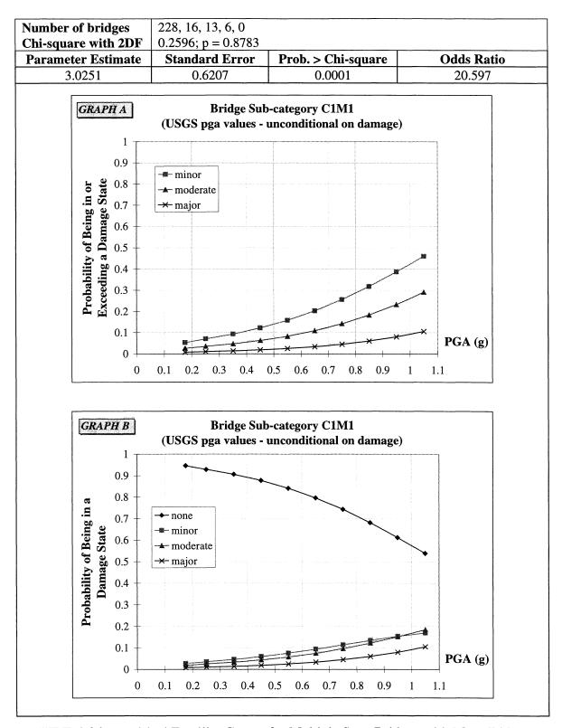
**FIGURE 4-24** Empirical Fragility Curves for Multiple Span Bridges with Monolithic Type Abutments, Continuous Spans and Multiple Column Bents (Sub-category C1M1)
