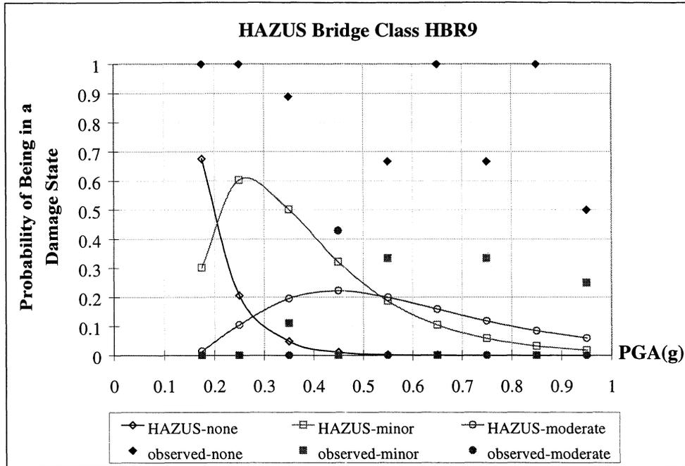
**FIGURE 4-29.a** Comparison of Damage Probabilities from Data to HAZUS Fragility Functions, No Damage, Minor Damage and Moderate Damage
