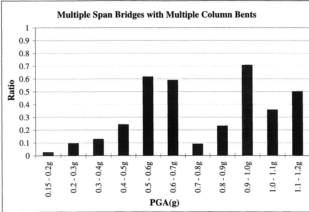
**FIGURE 4-17.a** Comparison of Damaged Bridges with Multiple Column Bents to Total Number of Bridges with Multiple Column Bents
