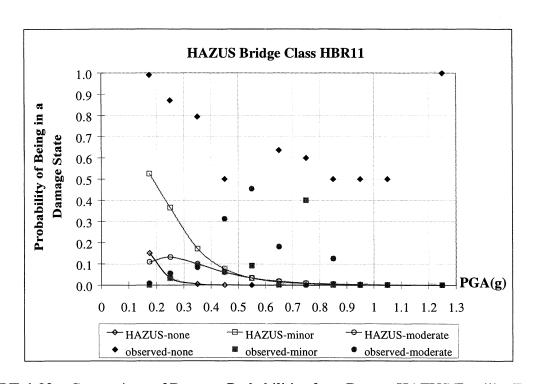
**FIGURE 4-30.a** Comparison of Damage Probabilities from Data to HAZUS Fragility Functions, No Damage, Minor Damage and Moderate Damage
