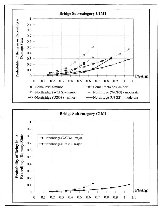
**FIGURE 5-12** Empirical Fragility Curves for Bridges in Sub-category C1M1 obtained from the Loma Prieta and Northridge Earthquakes (*correlation data set*) - Damage States
