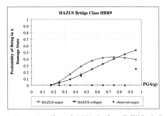
FIGURE 4-29.b Comparison of Damage Probabilities from Data to HAZUS Fragility Functions,
