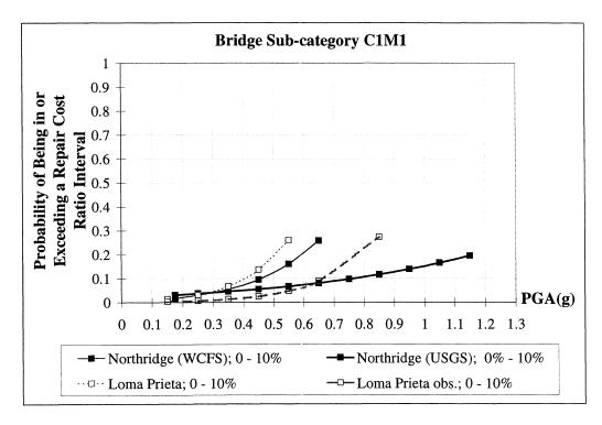
**FIGURE 5-17** Empirical Fragility Curves for Bridges in Sub-category C1M1 obtained from the Loma Prieta and Northridge Earthquakes (*correlation data set*) - Repair Cost Ratio
