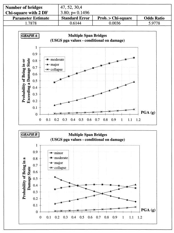
FIGURE 4-20 Empirical Fragility Curves for Multiple Span Bridges, Conditional on Damage
