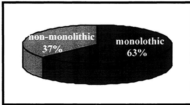
**FIGURE 4-14** Distribution of Damaged Single Span Bridges by Abutment Type (*correlation data set*)
