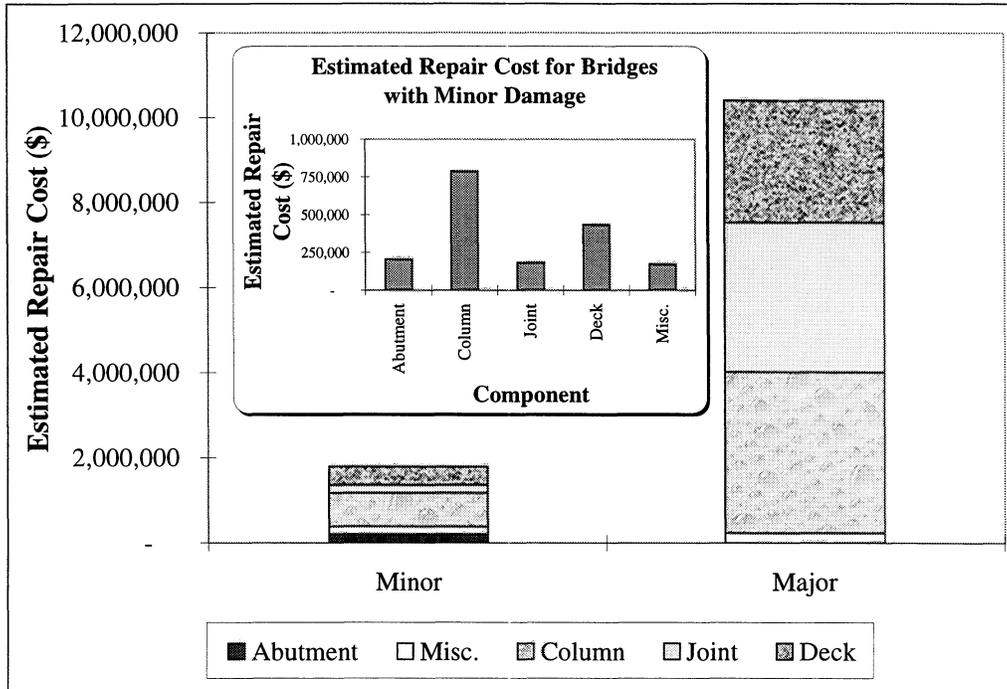
**FIGURE 3-22** Distribution of Estimated Repair Cost by Bridge Components for Different Damage States
