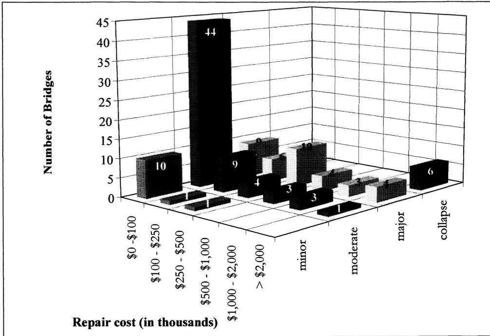
**FIGURE 4-37** Distribution of All Damaged Bridges by Repair Cost and Damage State
