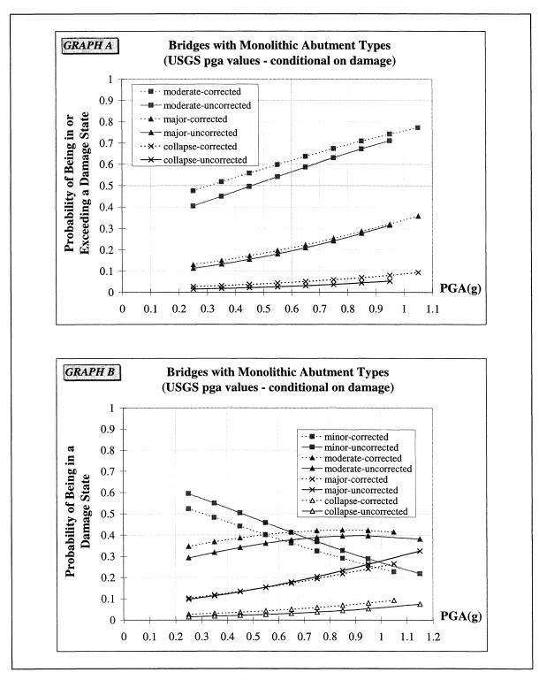
**FIGURE 4-35** Comparison of Conditional Empirical Fragility Curves for Multiple Span Bridges with Monolithic Abutments based on Corrected and Uncorrected Data
