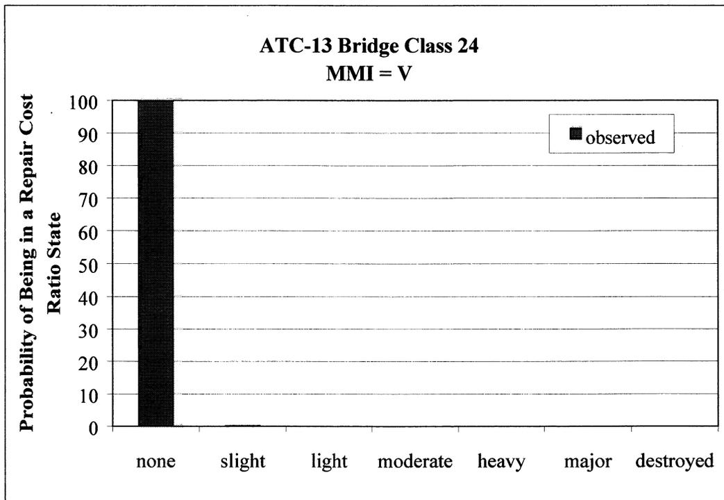
**FIGURE 4-49.a** Comparison of Observed and Predicted Probabilities of being in a given Repair Cost Ratio State, ATC-13 Bridge Class 24 MMI V
