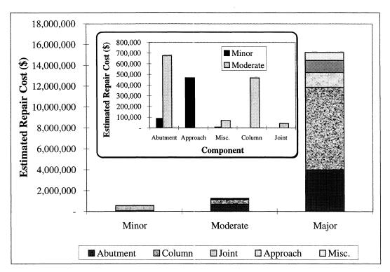
FIGURE 4-39 Distribution of Estimated Repair Cost by Bridge Components for Different
