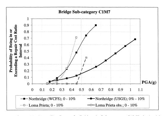
**FIGURE 5-18** Empirical Fragility Curves for Bridges in Sub-category C1M7 obtained from the Loma Prieta and Northridge Earthquakes (*correlation data set*) - Repair Cost Ratio
