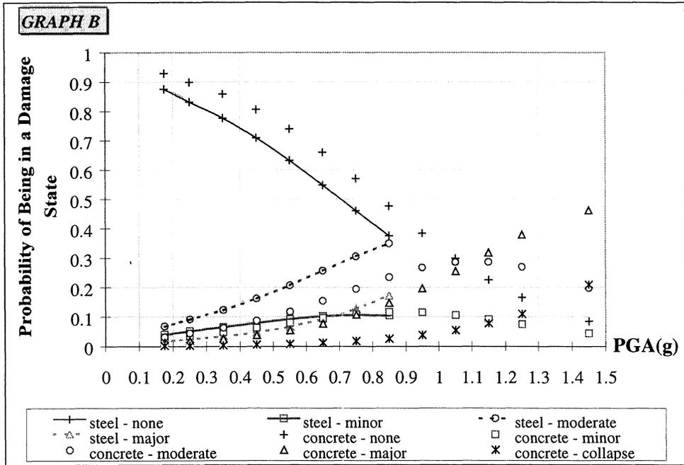
**FIGURE 4-54** Empirical Fragility Curves for Steel and Concrete Bridges
