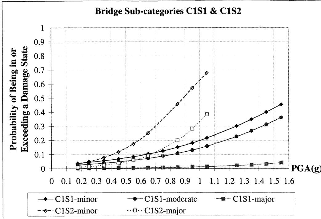
**FIGURE 4-57** Empirical Fragility Curves for Single Span Bridges with Monolithic (C1S1) and Non-monolithic (C1S2) Abutments
