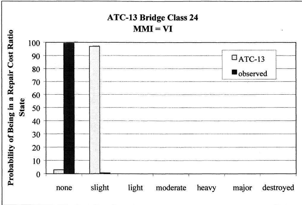
**FIGURE 4-49.b** Comparison of Observed and Predicted Probabilities of being in a given Repair Cost Ratio State, ATC-13 Bridge Class 24 MMI VI
