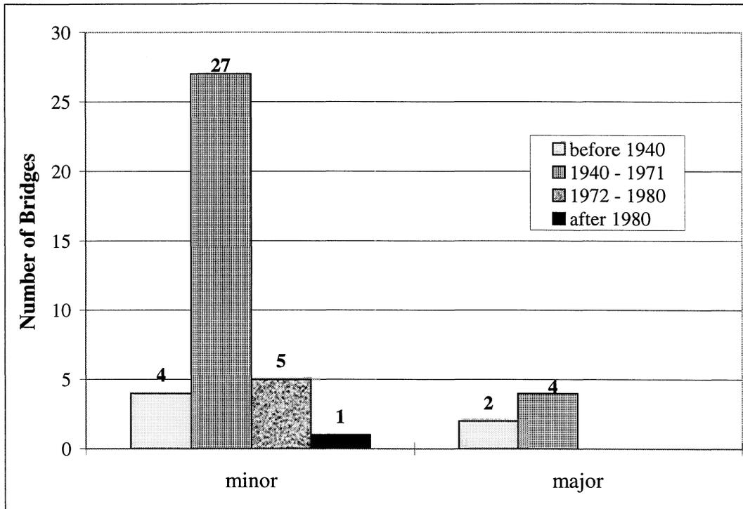
**FIGURE 3-12** Distribution of Damaged Concrete Highway Bridges by Design Year for  $PGA \geq 0.10g$
