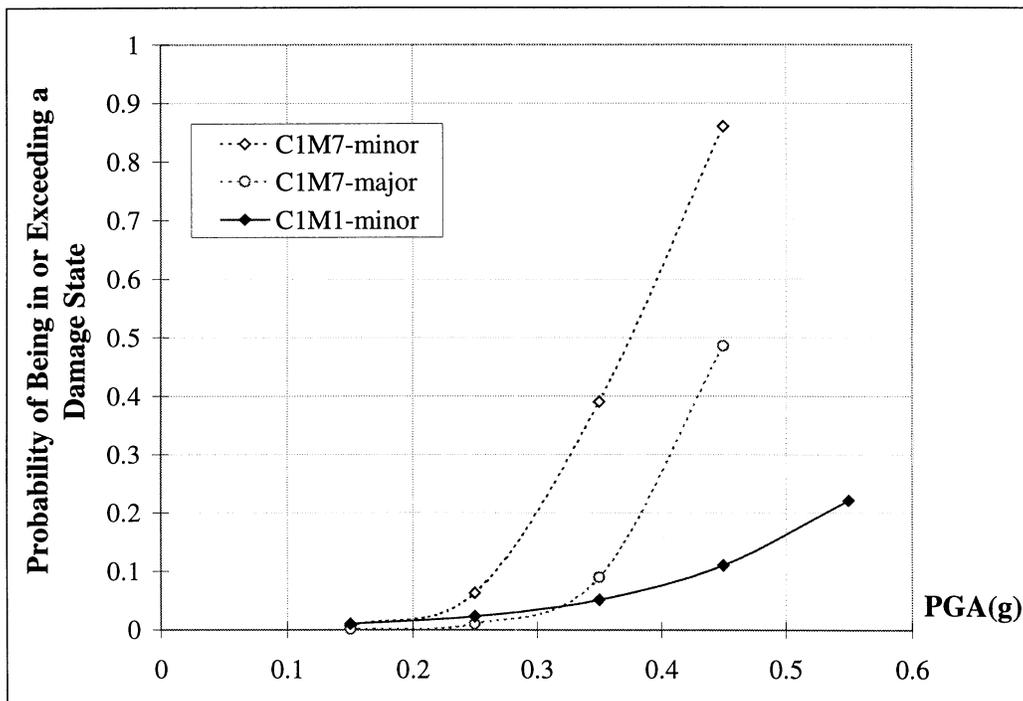
**FIGURE 3-31** Empirical Fragility Curves for Sub-categories C1M1 and C1M7
