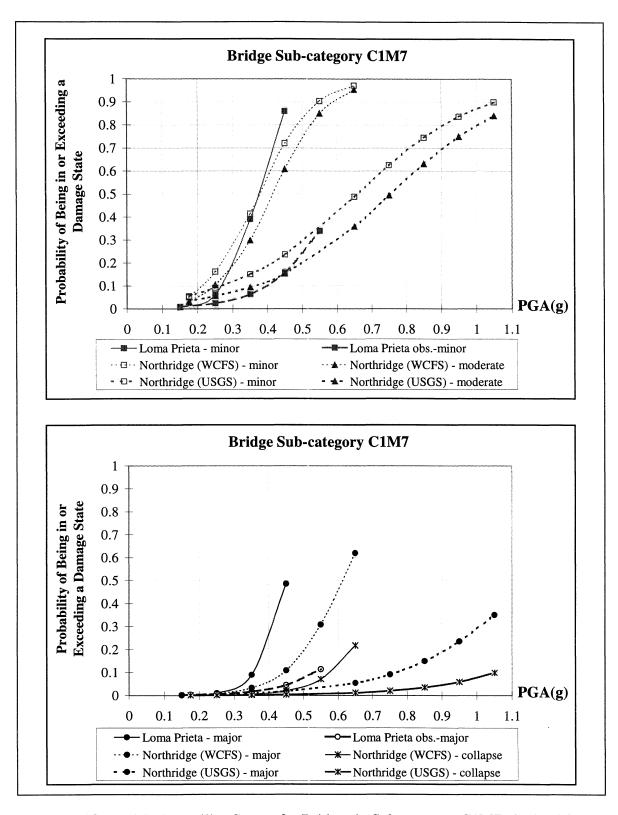
**FIGURE 5-13** Empirical Fragility Curves for Bridges in Sub-category C1M7 obtained from the Loma Prieta and Northridge Earthquakes (*correlation data set*) - Damage States
