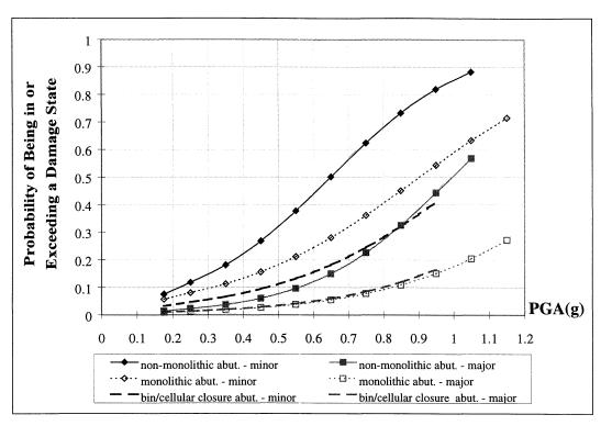
FIGURE 4-55 Performance Comparison of Different Types of Abutments - Minor Damage and Major Damage
