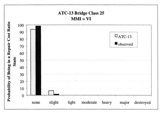
FIGURE 4-50.b Comparison of Observed and Predicted Probabilities of being in a given Repair
