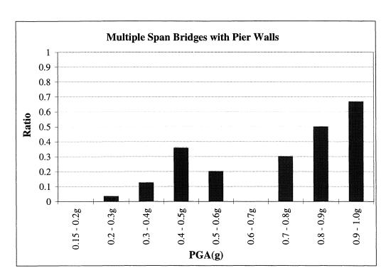
FIGURE 4-17.c Comparison of Damaged Bridges with Pier Walls to Total Number of Bridges with Pier Walls
