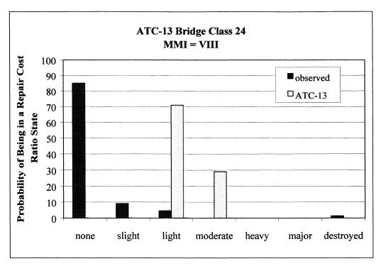
**FIGURE 4-49.d** Comparison of Observed and Predicted Probabilities of being in a given Repair Cost Ratio State, ATC-13 Bridge Class 24 MMI VIII
