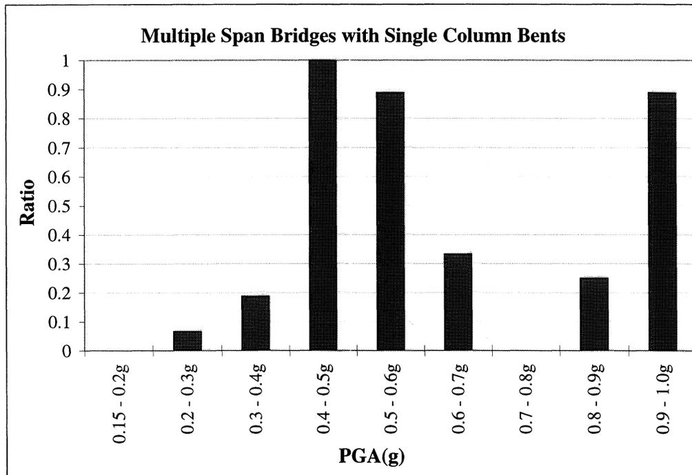
**FIGURE 4-17.b** Comparison of Damaged Bridges with Single Column Bents to Total Number of Bridges with Single Column Bents
