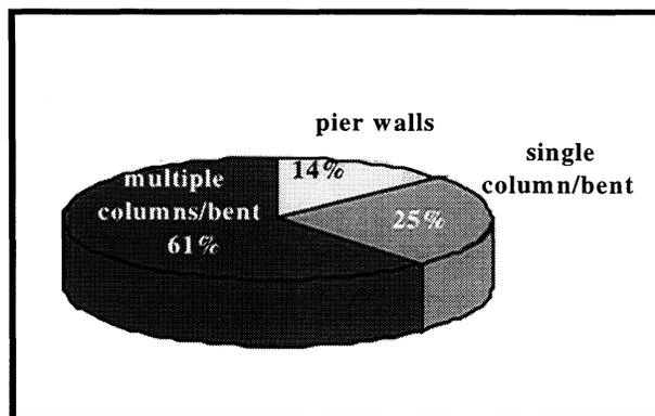
**FIGURE 4-15.b** Distribution of Damaged Multiple Span Bridges by Column Bent Type
