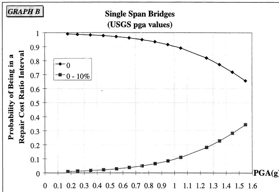
**FIGURE 4-45** Empirical Fragility Curves for Single Span Bridges, Repair Cost Ratio
