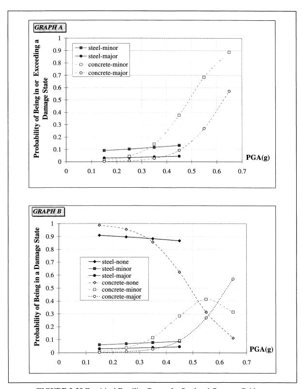
FIGURE 3-28 Empirical Fragility Curves for Steel and Concrete Bridges
