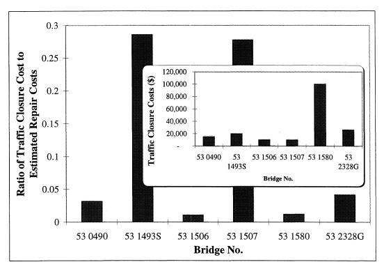
FIGURE 4-42 Ratio of Traffic Closure Cost to Estimated Repair Cost - Major Damage
