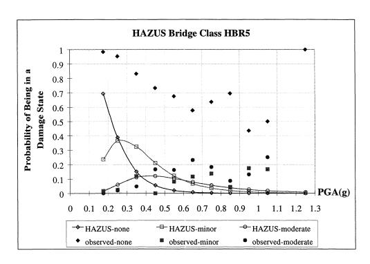
FIGURE 4-28.a Comparison of Damage Probabilities from Data to HAZUS Fragility Functions,
