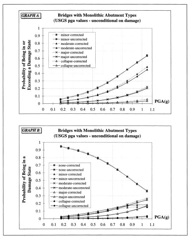
**FIGURE 4-33** Comparison of Empirical Fragility Curves for Multiple Span Bridges with Monolithic Abutments based on Corrected and Uncorrected Data
