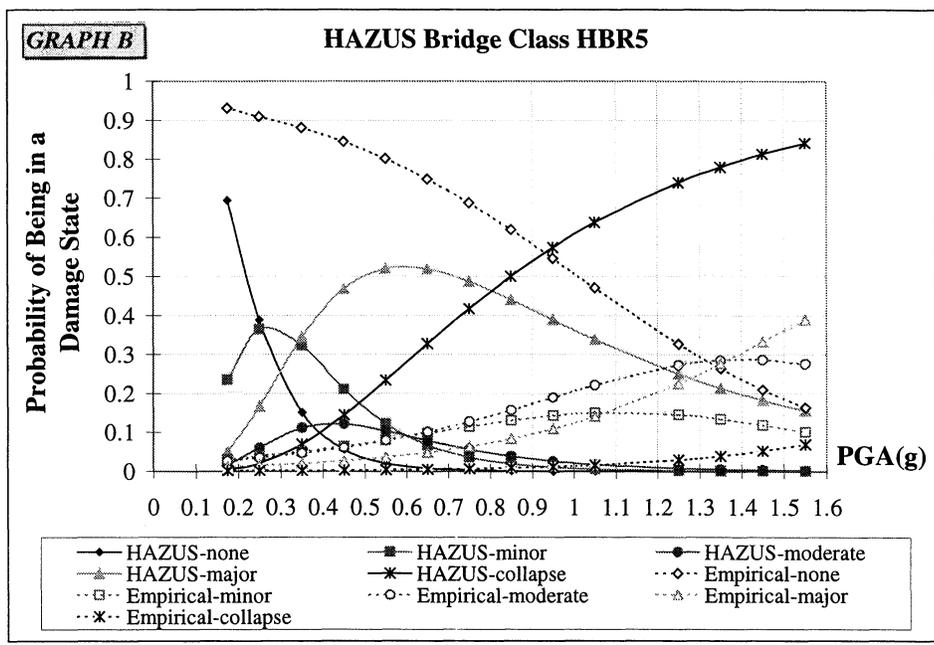
**FIGURE 4-31** Comparison of Empirical and the HAZUS Fragility Curves for HAZUS Bridge Class HBR5, USGS PGA values
