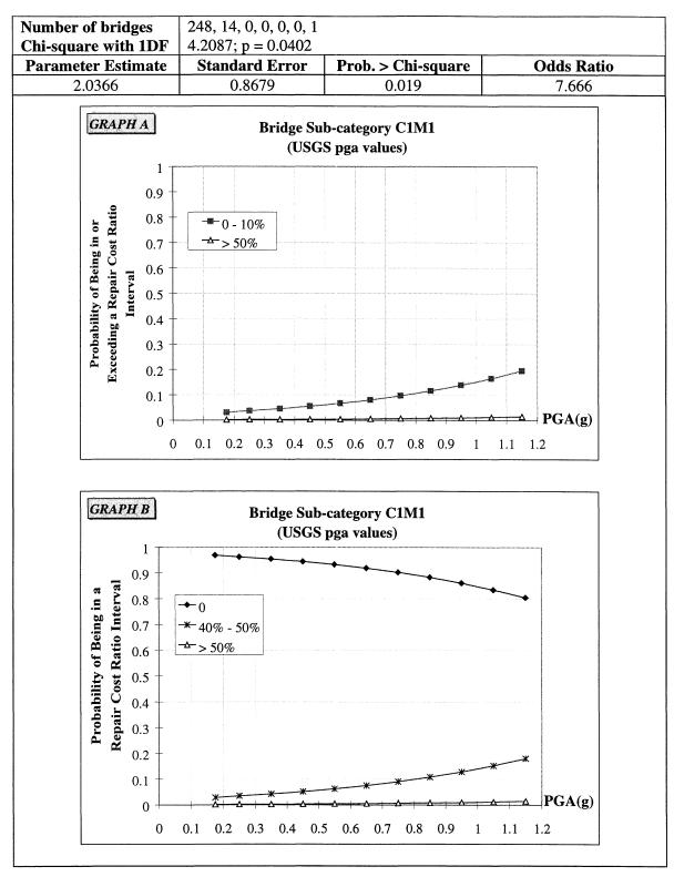
FIGURE 4-47 Empirical Fragility Curves for Multiple Span Bridges with Monolithic Type
