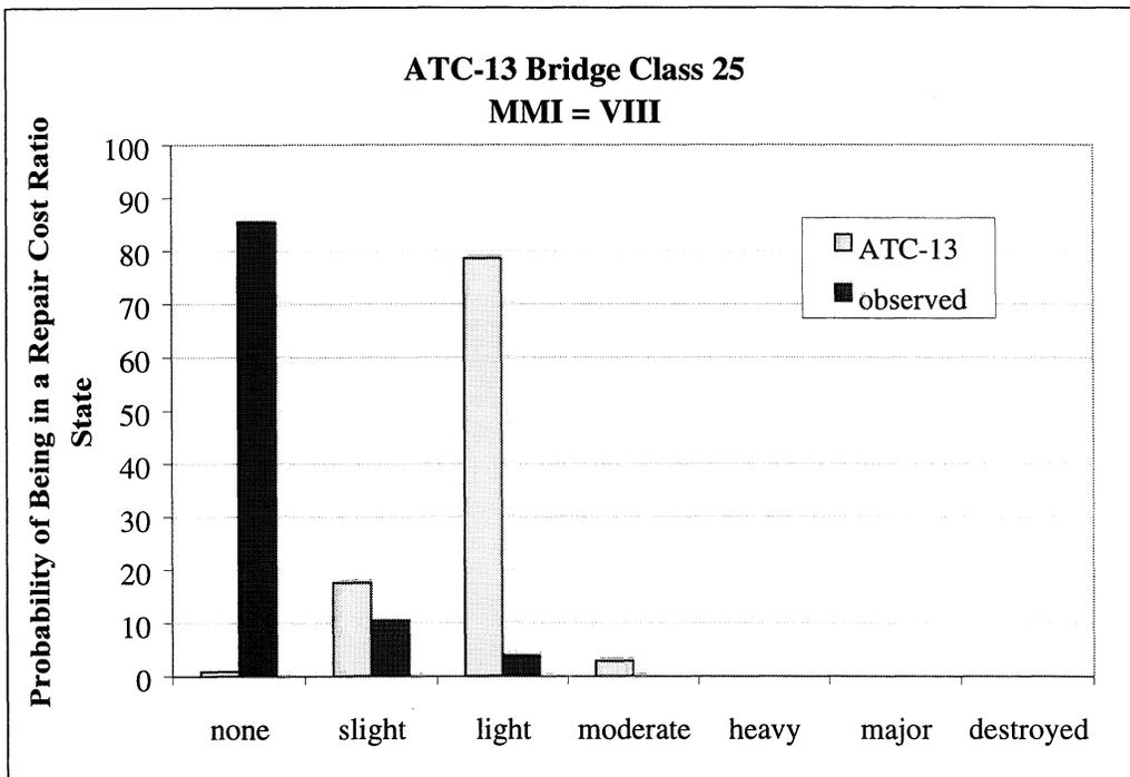
**FIGURE 4-50.d** Comparison of Observed and Predicted Probabilities of being in a given Repair Cost Ratio State, ATC-13 Bridge Class 25 MMI VIII
