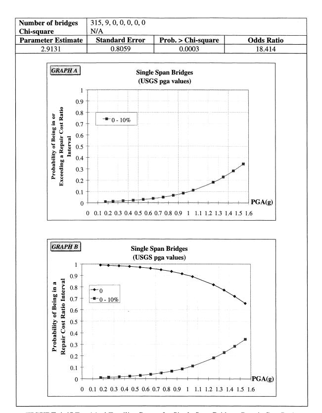
FIGURE 4-45 Empirical Fragility Curves for Single Span Bridges, Repair Cost Ratio
