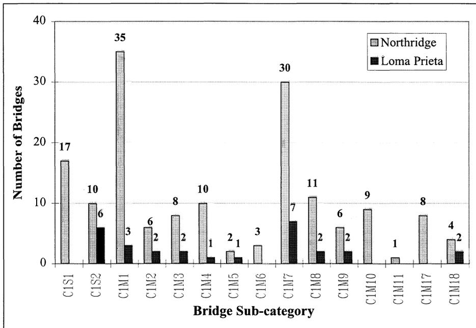
**FIGURE 5-10** Number of Damaged Bridges in the Loma Prieta and Northridge Earthquakes by Bridge Sub-categories (*correlation data set*)
