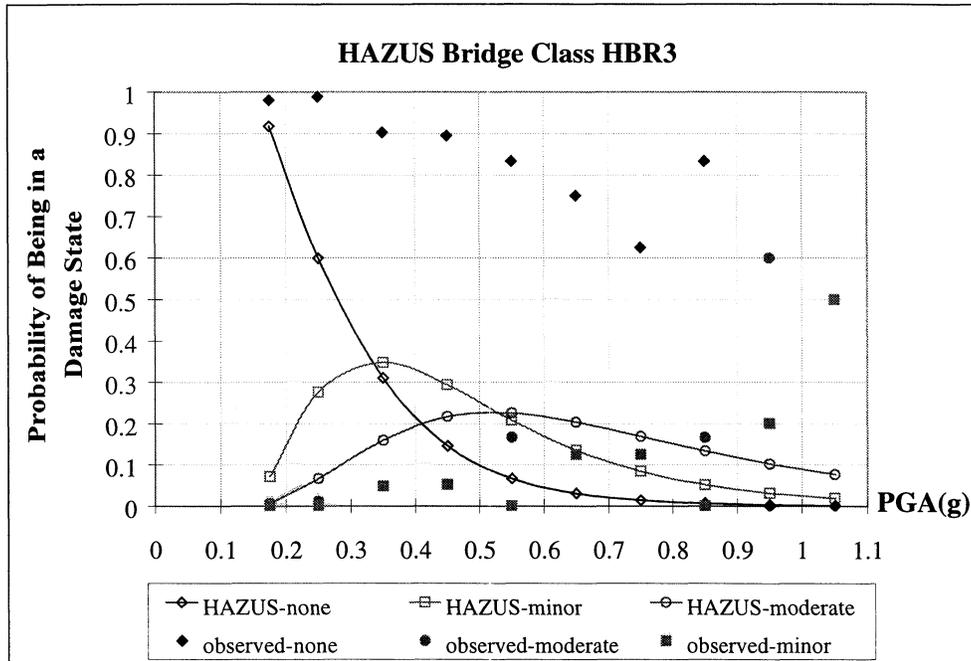
**FIGURE 4-27.a** Comparison of Damage Probabilities from Data to HAZUS Fragility Functions, No Damage, Minor Damage and Moderate Damage.
