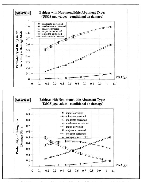
**FIGURE 4-36** Comparison of Conditional Empirical Fragility Curves for Multiple Span Bridges with Non-monolithic Abutments based on Corrected and Uncorrected Data
