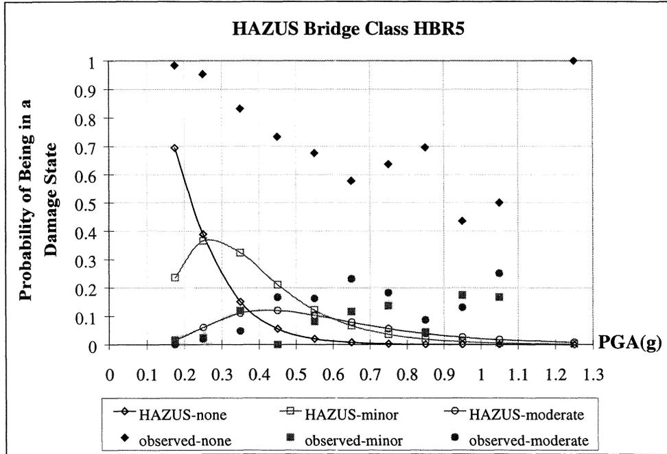
**FIGURE 4-28.a** Comparison of Damage Probabilities from Data to HAZUS Fragility Functions, No Damage, Minor Damage and Moderate Damage
