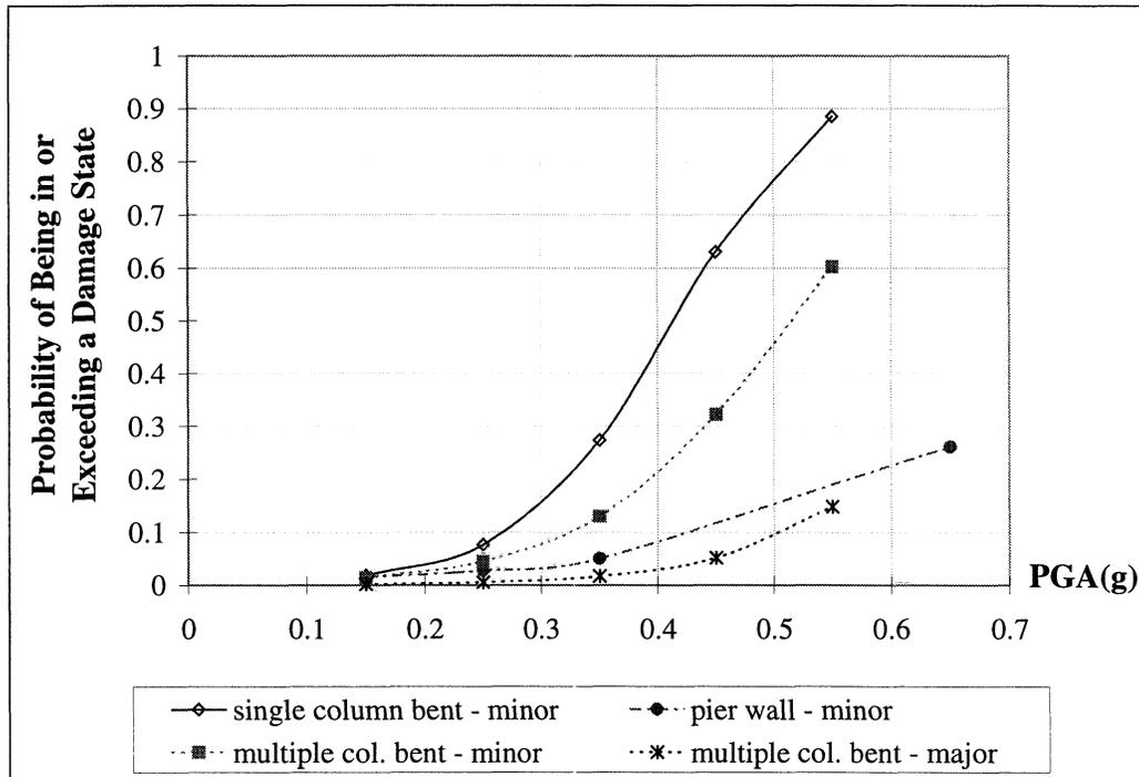
**FIGURE 3-30** Performance Comparison of Different Types of Column Bents
