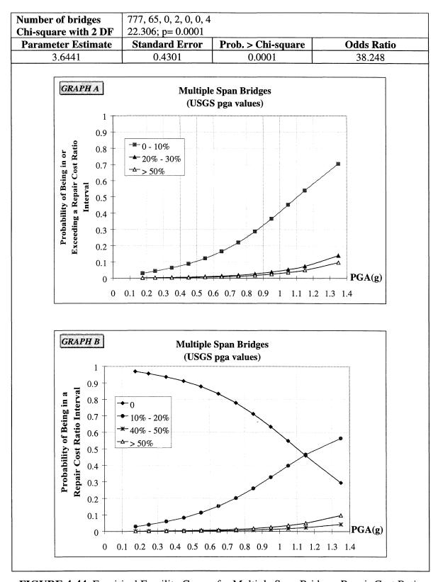
FIGURE 4-44 Empirical Fragility Curves for Multiple Span Bridges, Repair Cost Ratio
