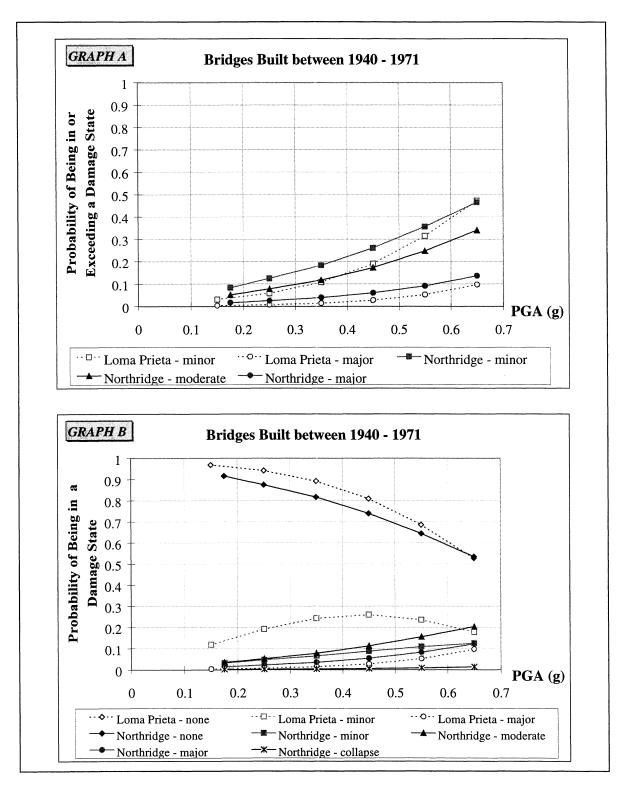
FIGURE 5-8 Empirical Fragility Curves for Bridges Built between 1940 and 1971 in the Loma
