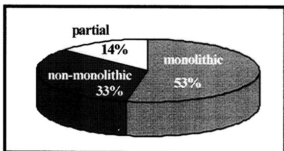
**FIGURE 3-8.a** Distribution of Multiple Span Bridges by Abutment Type
