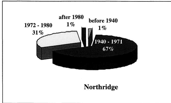
Figure 5-7 shows the distribution of damaged bridges in the Loma Prieta and Northridge earthquakes by design year interval. The distribution of damaged bridges by design year interval shows similar characteristics to that of the bridge inventories except that a much higher percent of bridges built between 1972 and 1980 sustained damage in the Northridge earthquake.
