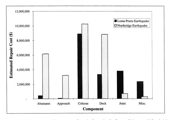
FIGURE 5-15 Estimated Component Repair Costs in the Loma Prieta and Northridge
