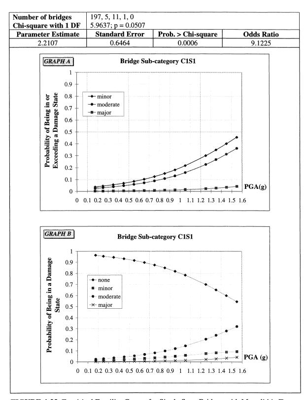
**FIGURE 4-23** Empirical Fragility Curves for Single Span Bridges with Monolithic Type
