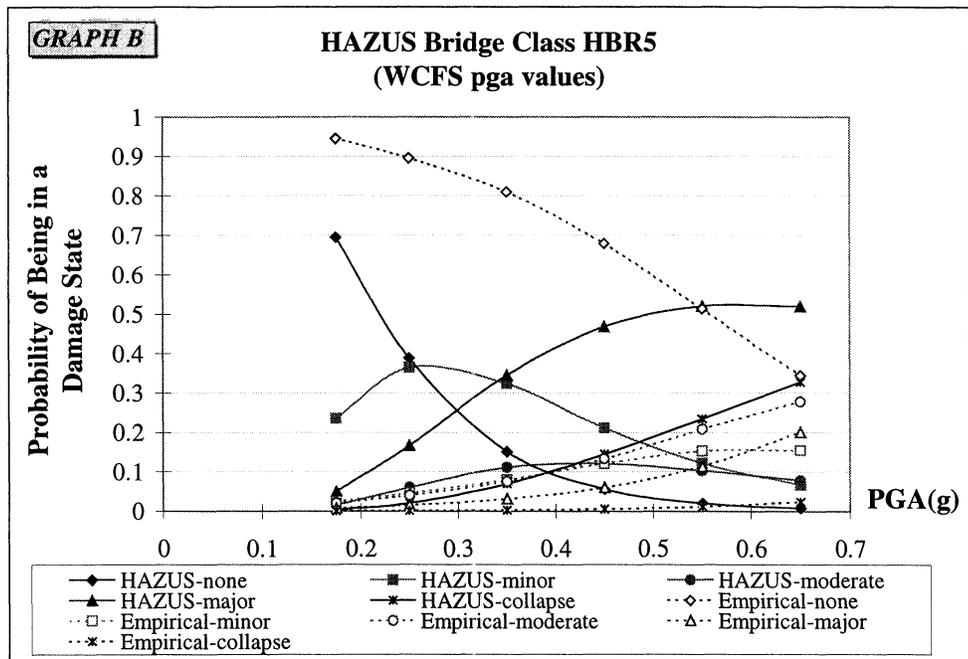
**FIGURE 4-32** Comparison of Empirical and the HAZUS Fragility Curves for HAZUS Bridge Class HBR5, WCFS PGA values
