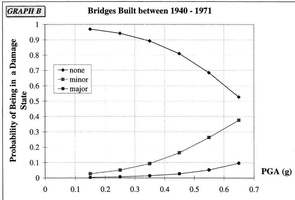
**FIGURE 3-19** Empirical Fragility Curves for All Bridges Built between 1940 and 1971
