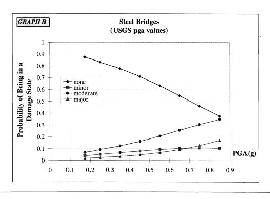
FIGURE 4-18 Empirical Fragility Curves for Steel Bridges
