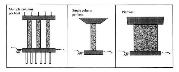
FIGURE 2-1 Different Column Bent Types Referred in Table 2-1
