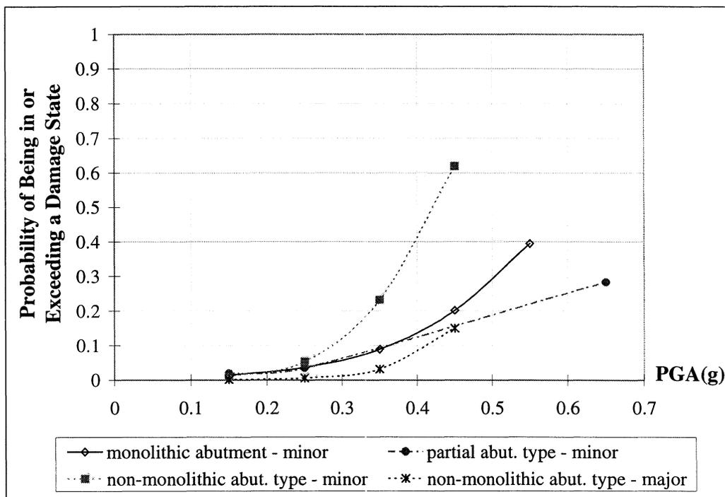
**FIGURE 3-29** Performance Comparison of Different Types of Abutments
