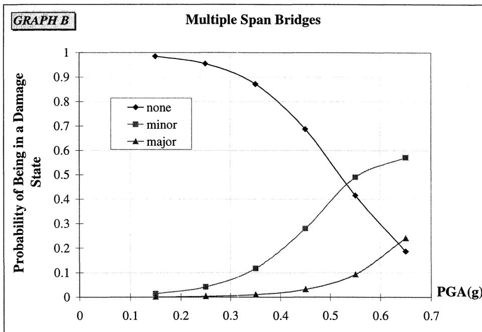
**FIGURE 3-15** Empirical Fragility Curves for Multiple Span Bridges
