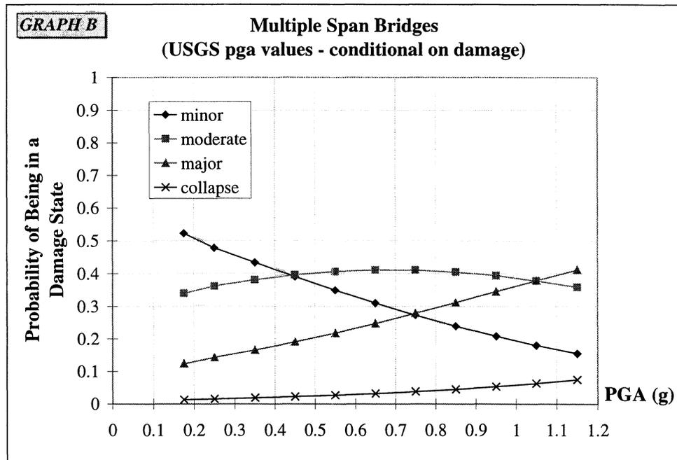
**FIGURE 4-20** Empirical Fragility Curves for Multiple Span Bridges, Conditional on Damage
