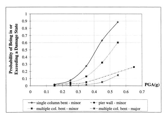
FIGURE 3-30 Performance Comparison of Different Types of Column Bents
