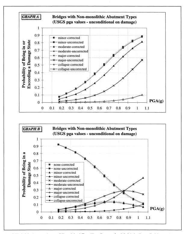
FIGURE 4-34 Comparison of Empirical Fragility Curves for Multiple Span Bridges with Nonmonolithic Abutments based on Corrected and Uncorrected Data
