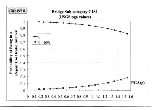
FIGURE 4-46 Empirical Fragility Curves for Single Span Bridges with Monolithic Type
