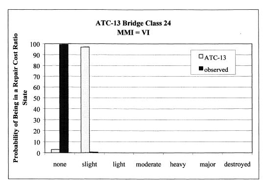
**FIGURE 4-49.b** Comparison of Observed and Predicted Probabilities of being in a given Repair Cost Ratio State, ATC-13 Bridge Class 24 MMI VI
