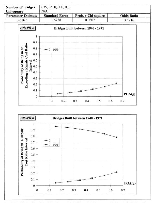
**FIGURE 3-26** Empirical Fragility Curves for Bridges Built between 1940 and 1971, Repair Cost Ratio
