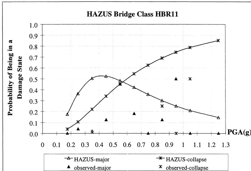
**FIGURE 4-30.b** Comparison of Damage Probabilities from Data to HAZUS Fragility Functions, Major Damage and Collapse
