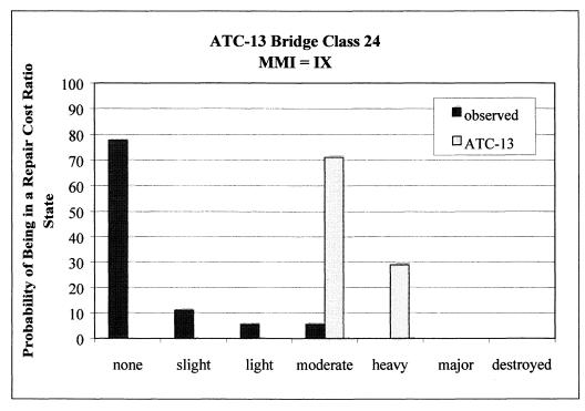
**FIGURE 4-49.e** Comparison of Observed and Predicted Probabilities of being in a given Repair Cost Ratio State, ATC-13 Bridge Class 24 MMI IX
