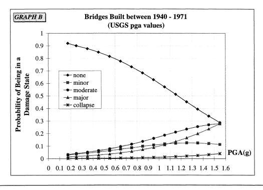
FIGURE 4-25 Empirical Fragility Curves for Bridges Built between 1940 and 1971
