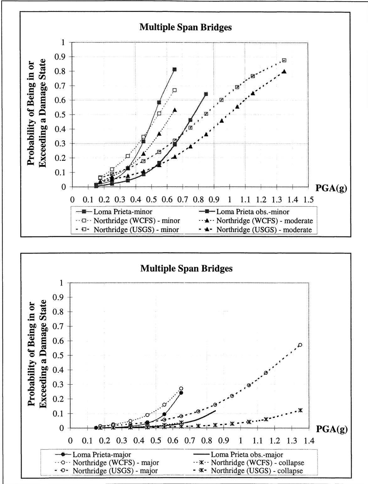
**FIGURE 5-11** Empirical Fragility Curves for Multiple Span Bridges obtained from the Loma Prieta and Northridge Earthquakes (*correlation data set*) - Damage States
