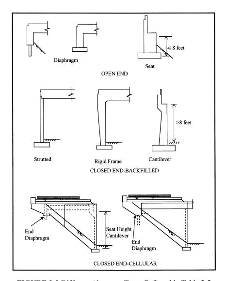
**FIGURE 2-2** Different Abutment Types Referred in Table 2-2
