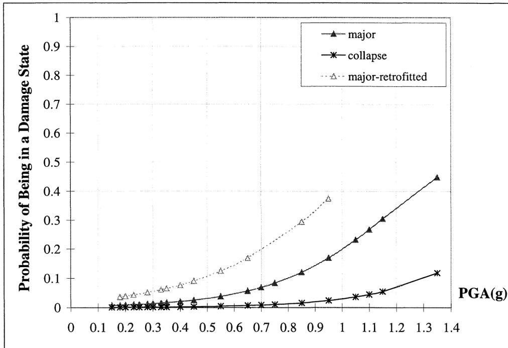
**FIGURE 4-26.b** Comparison of Empirical Fragility Curves for Retrofitted and Unretrofitted Bridges - Major Damage and Collapse
