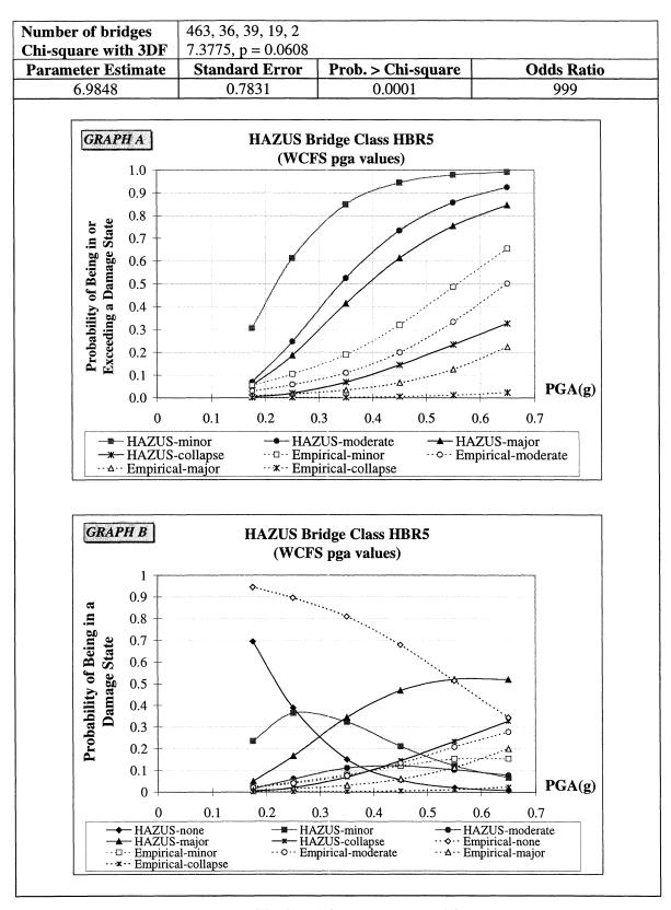
FIGURE 4-32 Comparison of Empirical and the HAZUS Fragility Curves for HAZUS Bridge
