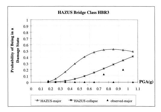
FIGURE 4-27.b Comparison of Damage Probabilities from Data to HAZUS Fragility Functions,
