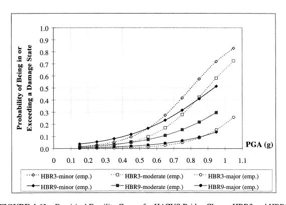
FIGURE 4-61.a Empirical Fragility Curves for HAZUS Bridge Classes HBR3 and HBR9
