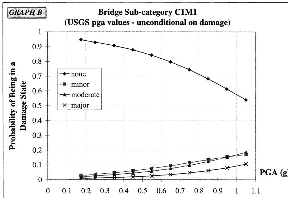
**FIGURE 4-24** Empirical Fragility Curves for Multiple Span Bridges with Monolithic Type Abutments, Continuous Spans and Multiple Column Bents (Sub-category C1M1)
