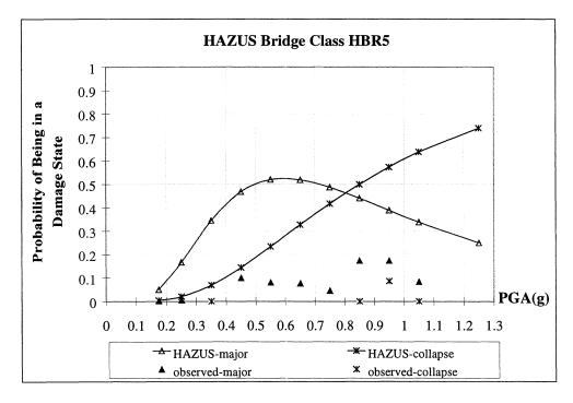
FIGURE 4-28.b Comparison of Damage Probabilities from Data to HAZUS Fragility Functions,
