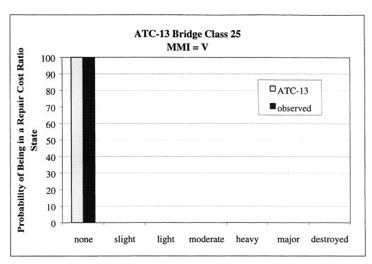
**FIGURE 4-50.a** Comparison of Observed and Predicted Probabilities of being in a given Repair Cost Ratio State, ATC-13 Bridge Class 25 MMI V
