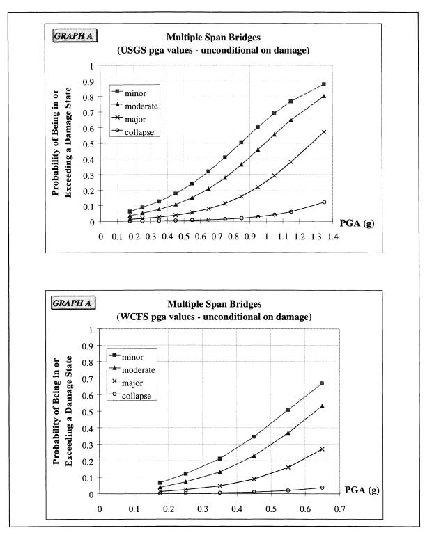
FIGURE 4-53 Empirical Fragility Curves for Multiple Span Bridges based on USGS [1994] and WCFS [1995] PGA Values
