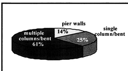
**FIGURE 3-8.b** Distribution of Multiple Span Bridges by Column Bent Type
