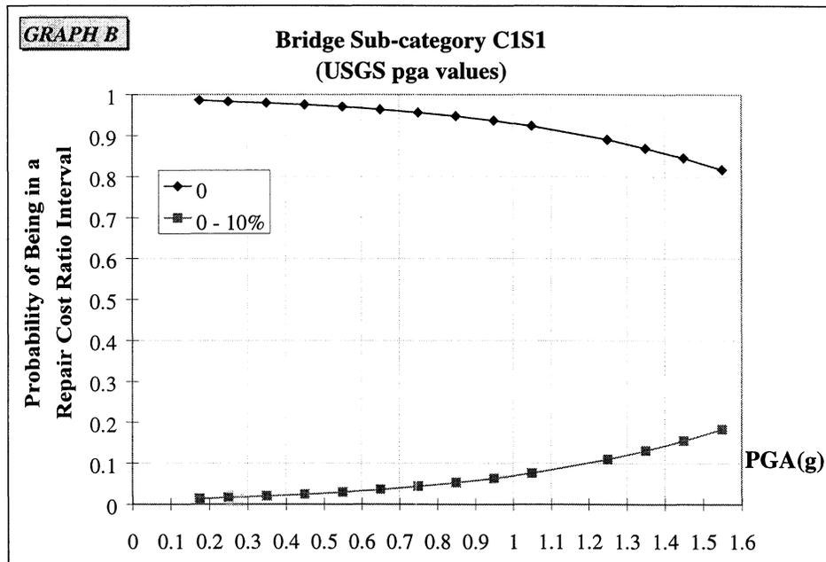
**FIGURE 4-46** Empirical Fragility Curves for Single Span Bridges with Monolithic Type Abutments (Sub-Category C1S1), Repair Cost Ratio
