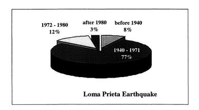
**FIGURE 5-5** Distribution of Bridges Damaged in the Loma Prieta Earthquake by Design Year
