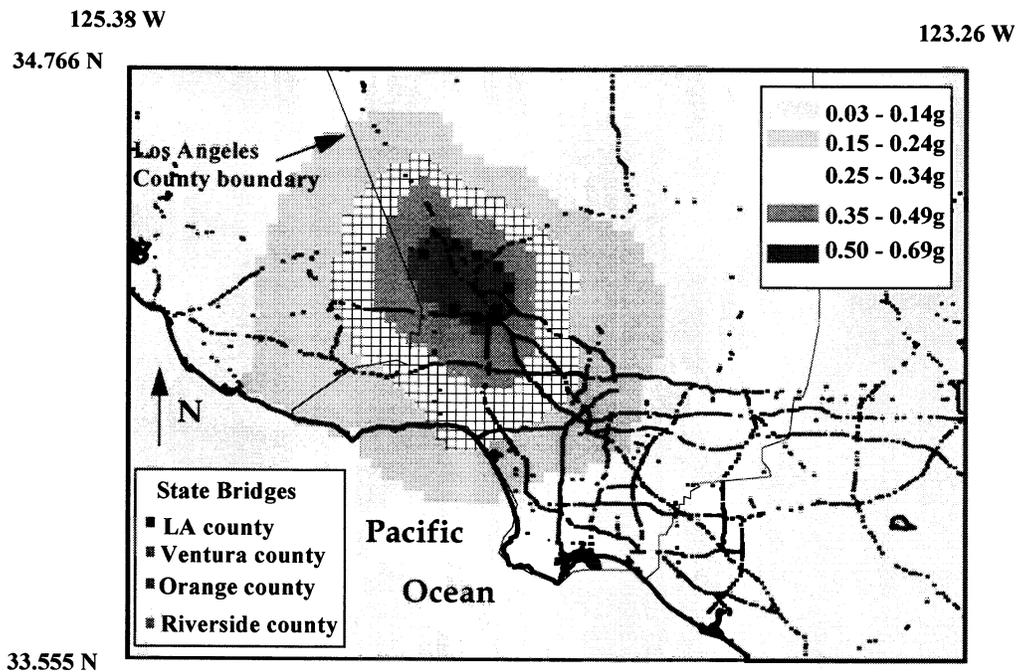
**FIGURE 4-7** Locations of the State Highway Bridges in the Greater Los Angeles Area and the PGA Levels Observed from the Northridge Earthquake [WCFS, 1995]
