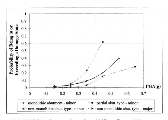
FIGURE 3-29 Performance Comparison of Different Types of Abutments
