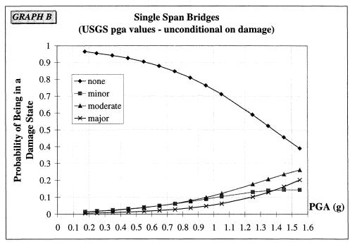
FIGURE 4-22 Empirical Fragility Curves for Single Span Bridges
