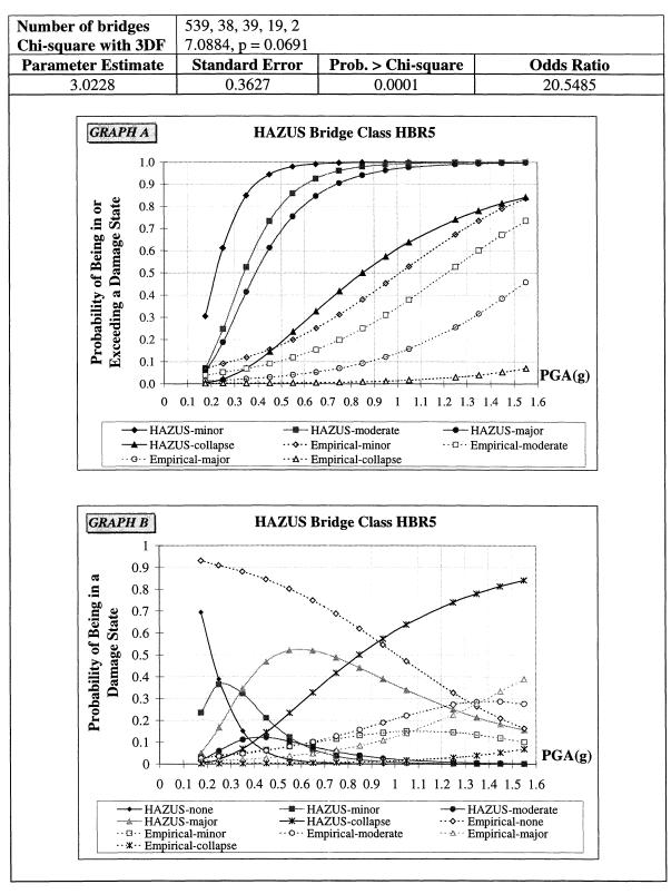
FIGURE 4-31 Comparison of Empirical and the HAZUS Fragility Curves for HAZUS Bridge
