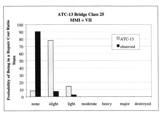
FIGURE 4-50.c Comparison of Observed and Predicted Probabilities of being in a given Repair
