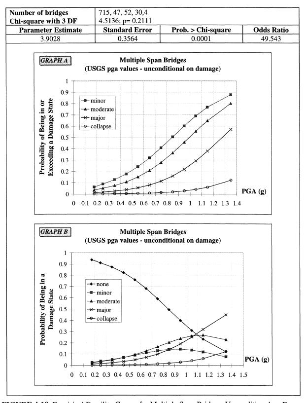
FIGURE 4-19 Empirical Fragility Curves for Multiple Span Bridges, Unconditional on Damage
