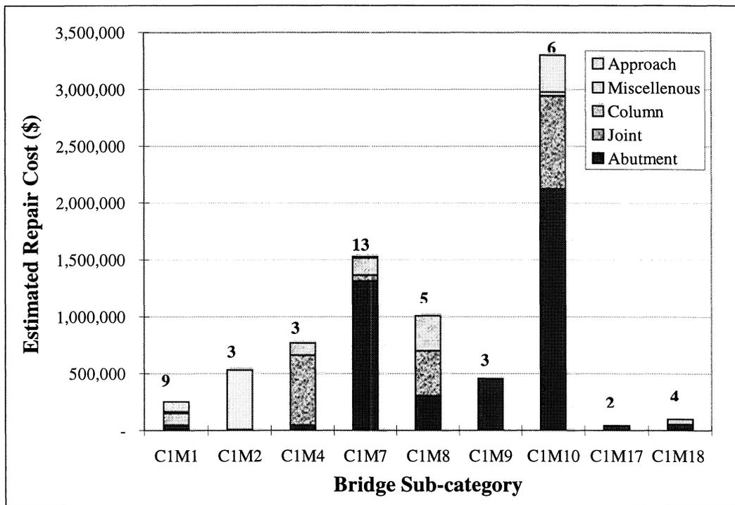
**FIGURE 4-40** Distribution of Estimated Repair Cost by Bridge Components for Different Bridge Sub-categories
