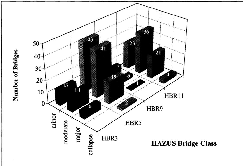
**FIGURE 4-10** Distribution of All Damaged Bridges by HAZUS Bridge Classification and Damage State
