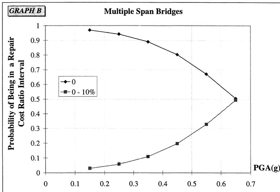
**FIGURE 3-24** Empirical Fragility Curves for Multiple Span Bridges, Repair Cost Ratio
