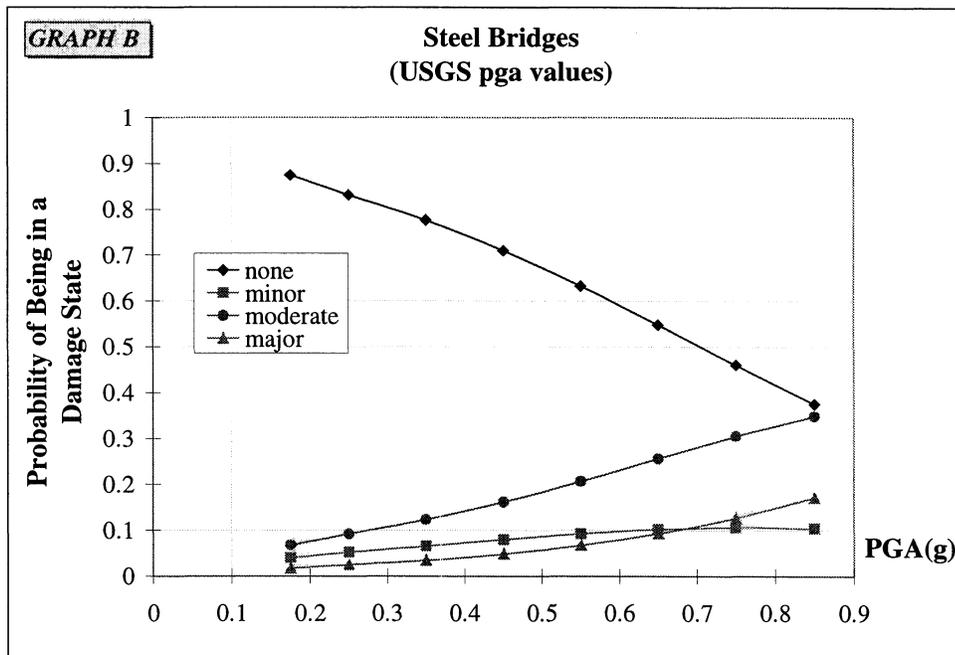
**FIGURE 4-18** Empirical Fragility Curves for Steel Bridges
