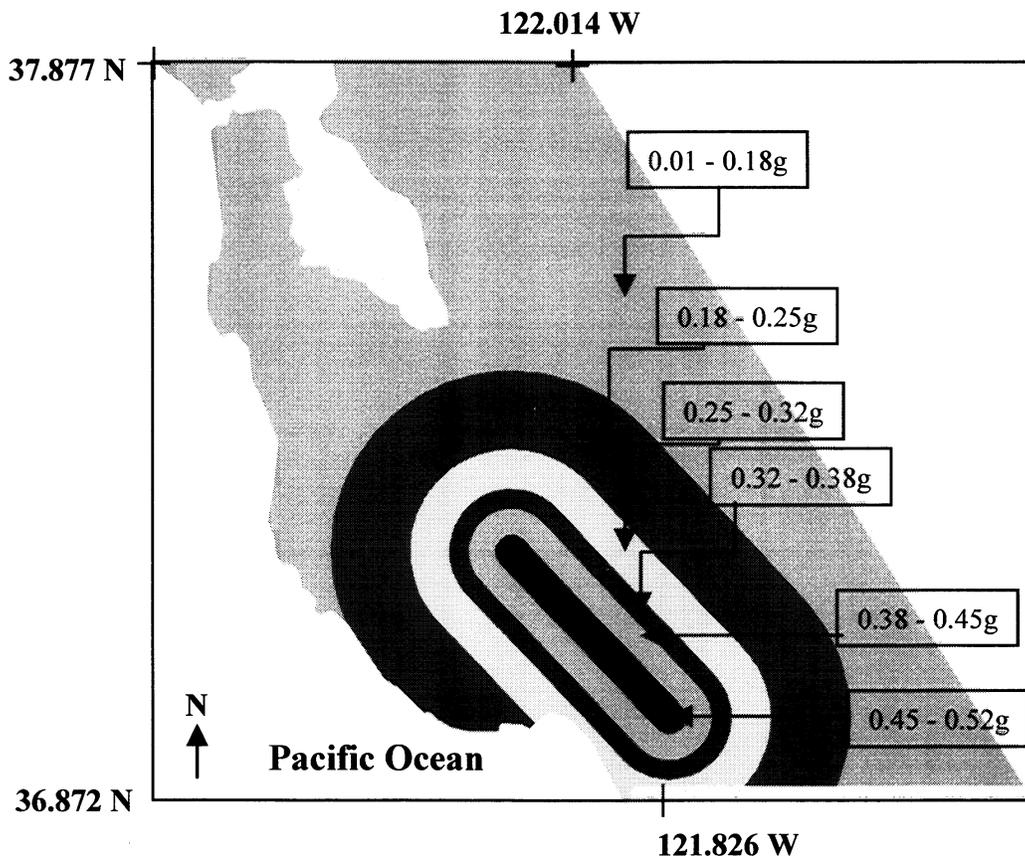
**FIGURE 3-1** Buffer Zones for Ground Shaking at Bedrock Level from the Loma Prieta Scenario Event
