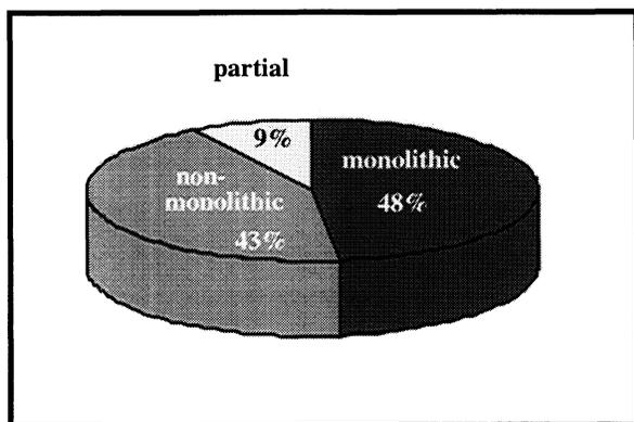
**FIGURE 4-15.a** Distribution of Damaged Multiple Span Bridges by Abutment Type
