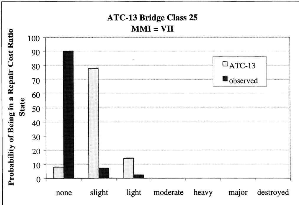
**FIGURE 4-50.c** Comparison of Observed and Predicted Probabilities of being in a given Repair Cost Ratio State, ATC-13 Bridge Class 25 MMI VII
