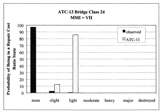
**FIGURE 4-49.c** Comparison of Observed and Predicted Probabilities of being in a given Repair Cost Ratio State, ATC-13 Bridge Class 24 MMI VII
