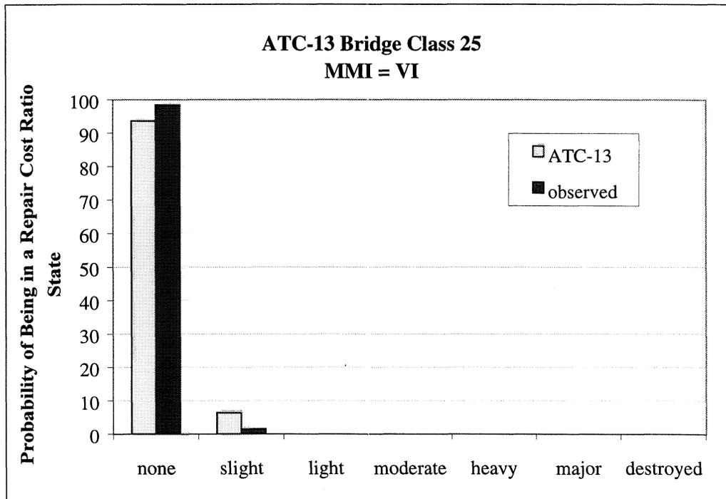
**FIGURE 4-50.b** Comparison of Observed and Predicted Probabilities of being in a given Repair Cost Ratio State, ATC-13 Bridge Class 25 MMI VI
