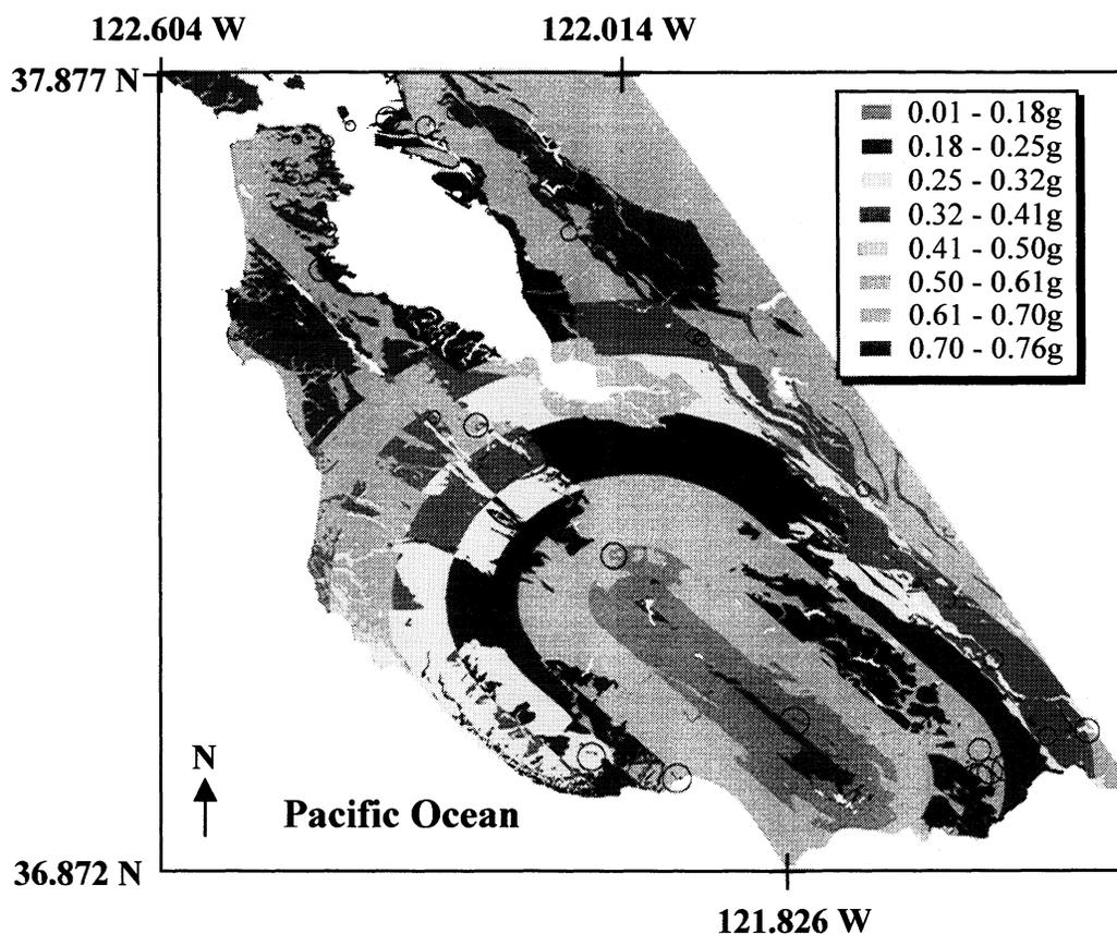
**FIGURE 3-2** Sample Recording Stations and Estimated Ground Shaking Levels for the Loma Prieta Earthquake
