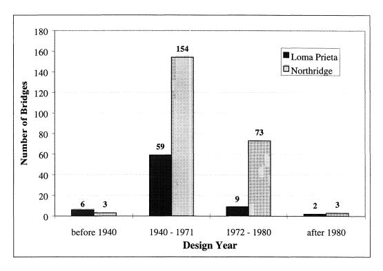
FIGURE 5-7 Number of Bridges Damaged in the Loma Prieta and Northridge Earthquakes by
