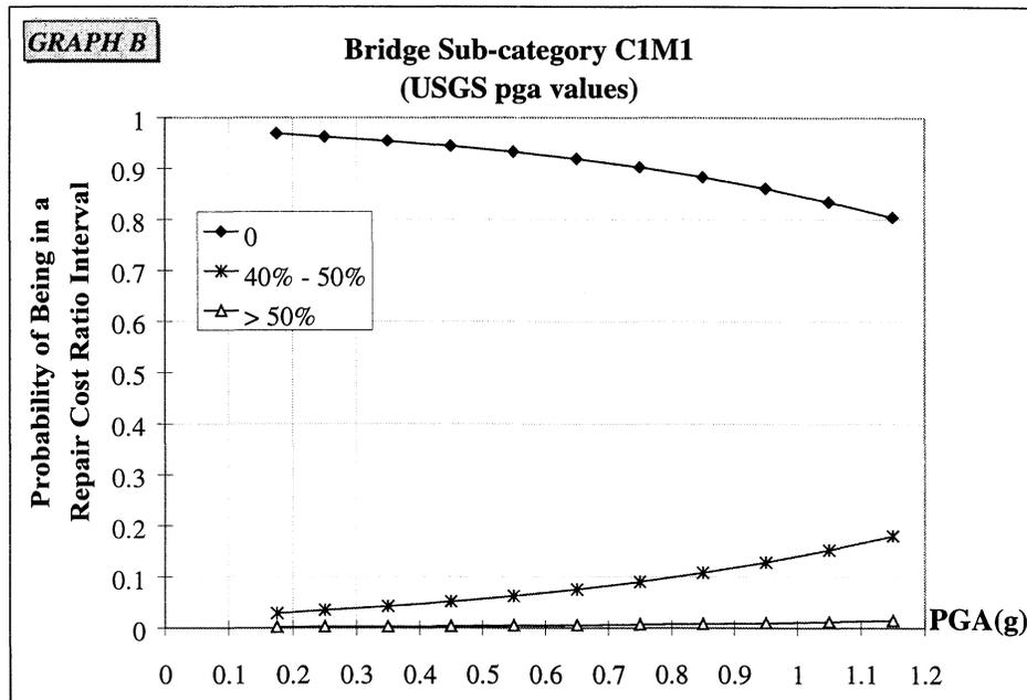
**FIGURE 4-47** Empirical Fragility Curves for Multiple Span Bridges with Monolithic Type Abutments, Continuous Spans and Multiple Column Bents (Sub-category C1M1), Repair Cost Ratio
