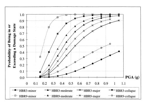
FIGURE 4-61.b HAZUS Fragility Curves for Bridge Classes HBR3 and HBR9
