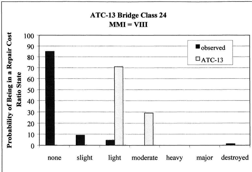
**FIGURE 4-49.d** Comparison of Observed and Predicted Probabilities of being in a given Repair Cost Ratio State, ATC-13 Bridge Class 24 MMI VIII
