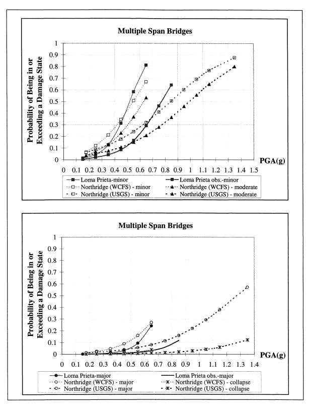
FIGURE 5-11 Empirical Fragility Curves for Multiple Span Bridges obtained from the Loma
