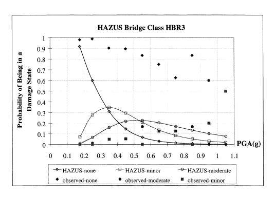
**FIGURE 4-27.a** Comparison of Damage Probabilities from Data to HAZUS Fragility Functions, No Damage, Minor Damage and Moderate Damage.
