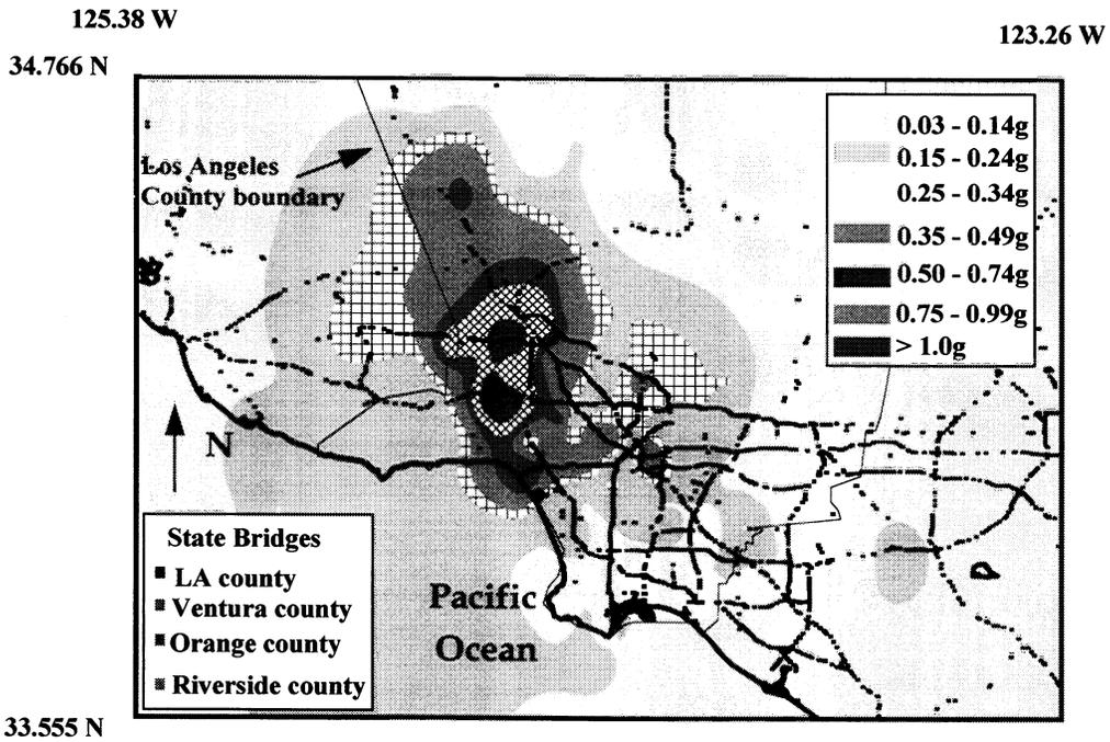
**FIGURE 4-6** Locations of the State Highway Bridges in the Greater Los Angeles Area and the PGA Levels Observed from the Northridge Earthquake [USGS, 1994]
