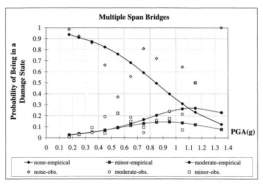
**FIGURE 4-21.a** Empirical Fragility Curves and Observed Data for Multiple Span Bridges – No Damage, Minor Damage and Moderate Damage
