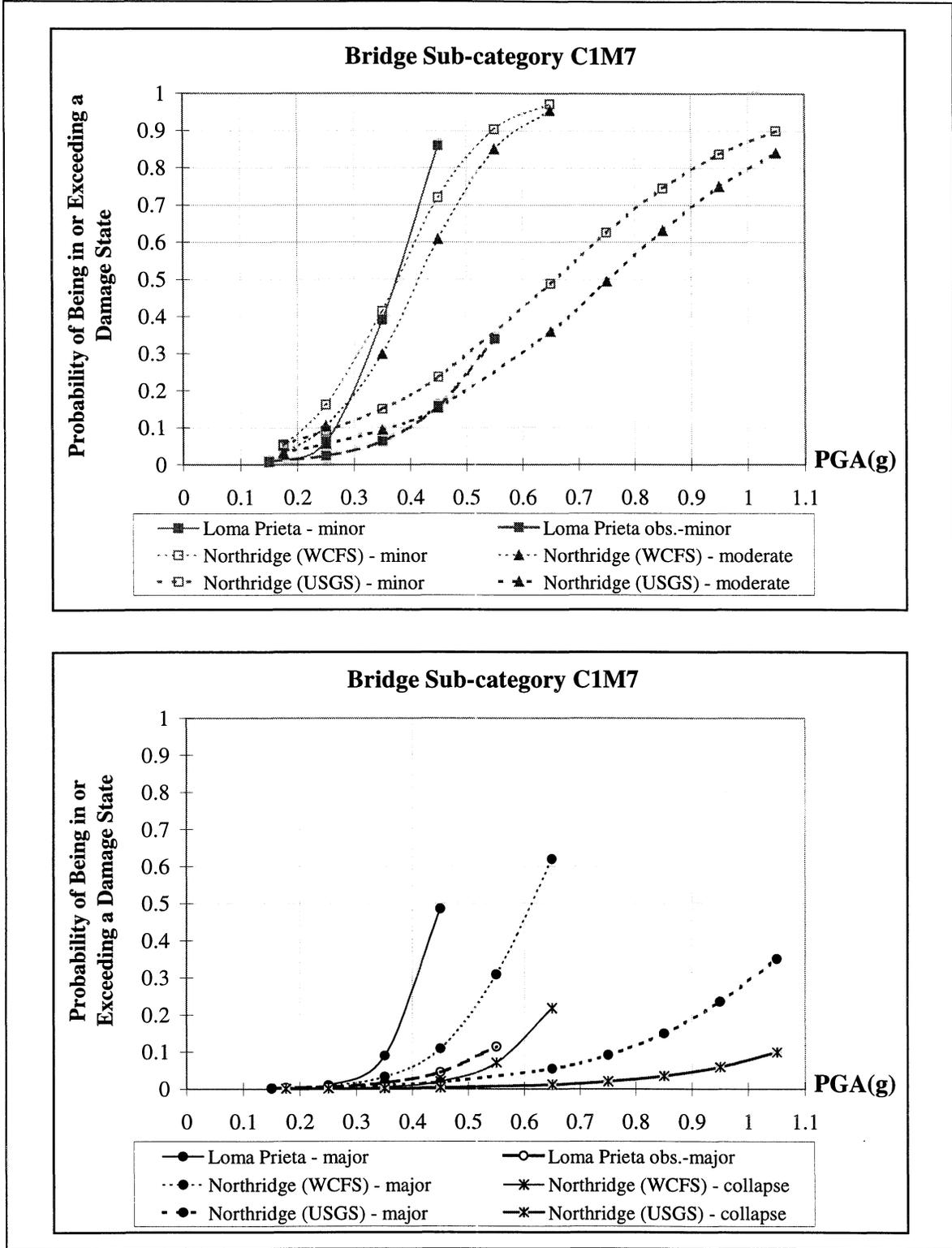
**FIGURE 5-13** Empirical Fragility Curves for Bridges in Sub-category C1M7 obtained from the Loma Prieta and Northridge Earthquakes (*correlation data set*) - Damage States
