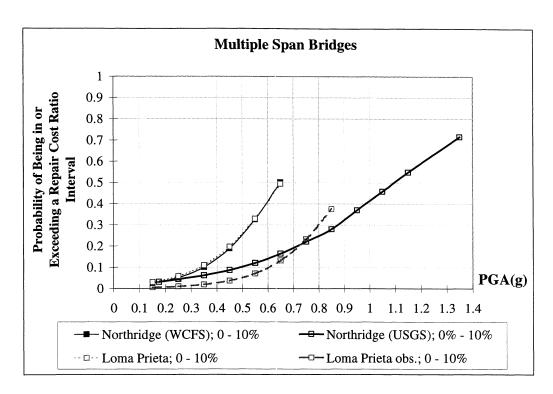
FIGURE 5-16 Empirical Fragility Curves for Multiple Span Bridges obtained from the Loma
