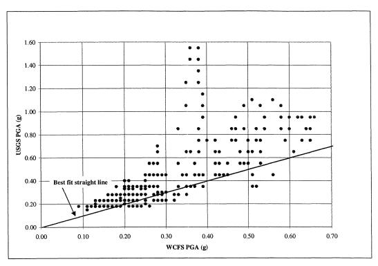
FIGURE 4-51 PGA Values Reported by USGS [1994] and WCFS [1995] – Northridge Earthquake
