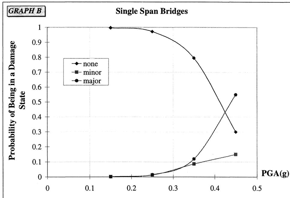
**FIGURE 3-17** Empirical Fragility Curves for Single Span Bridges
