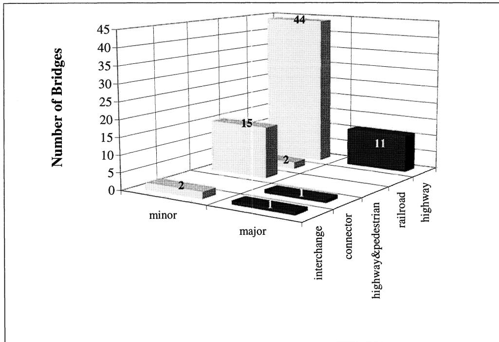
**FIGURE 3-11** Distribution of All Damaged Bridges by Service Type and Damage State
