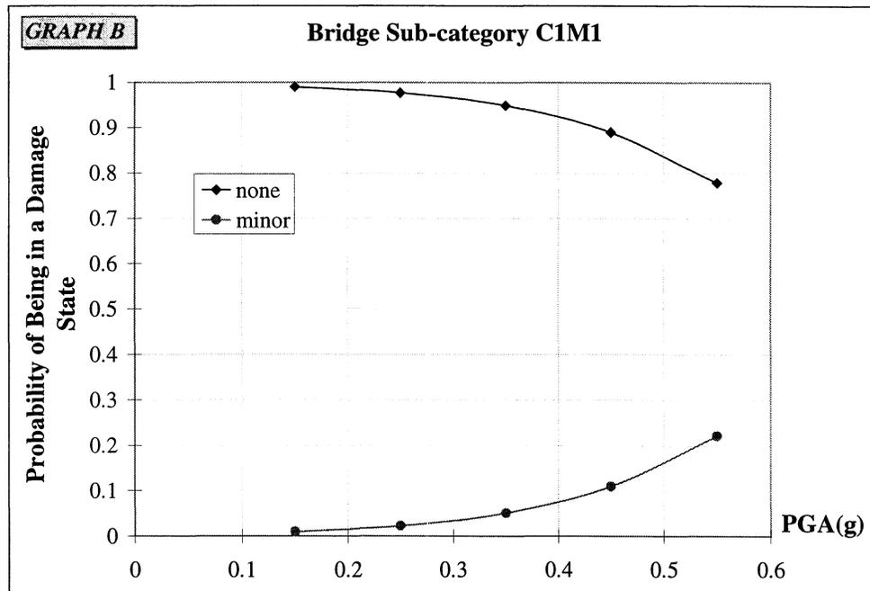
**FIGURE 3-18** Empirical Fragility Curves for Multiple Span Bridges with Monolithic Type Abutments, Continuous Spans and Multiple Column Bents (Sub-category C1M1)
