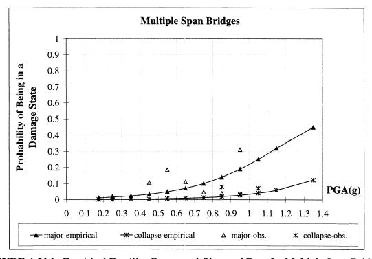
FIGURE 4-21.b Empirical Fragility Curves and Observed Data for Multiple Span Bridges - Major Damage and Collapse
