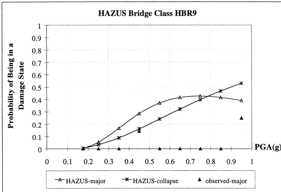
**FIGURE 4-29.b** Comparison of Damage Probabilities from Data to HAZUS Fragility Functions, Major Damage and Collapse
