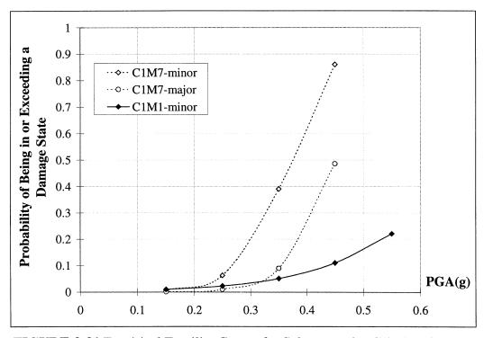
FIGURE 3-31 Empirical Fragility Curves for Sub-categories C1M1 and C1M7
