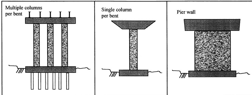
**FIGURE 2-1** Different Column Bent Types Referred in Table 2-1
