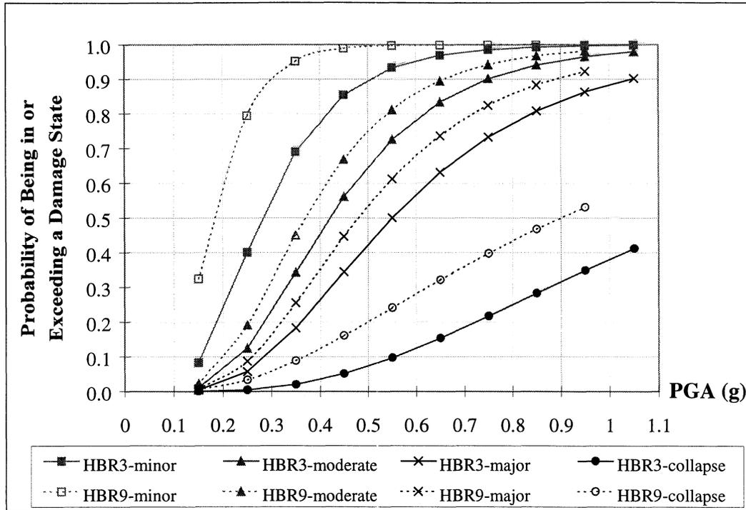
**FIGURE 4-61.b** HAZUS Fragility Curves for Bridge Classes HBR3 and HBR9
