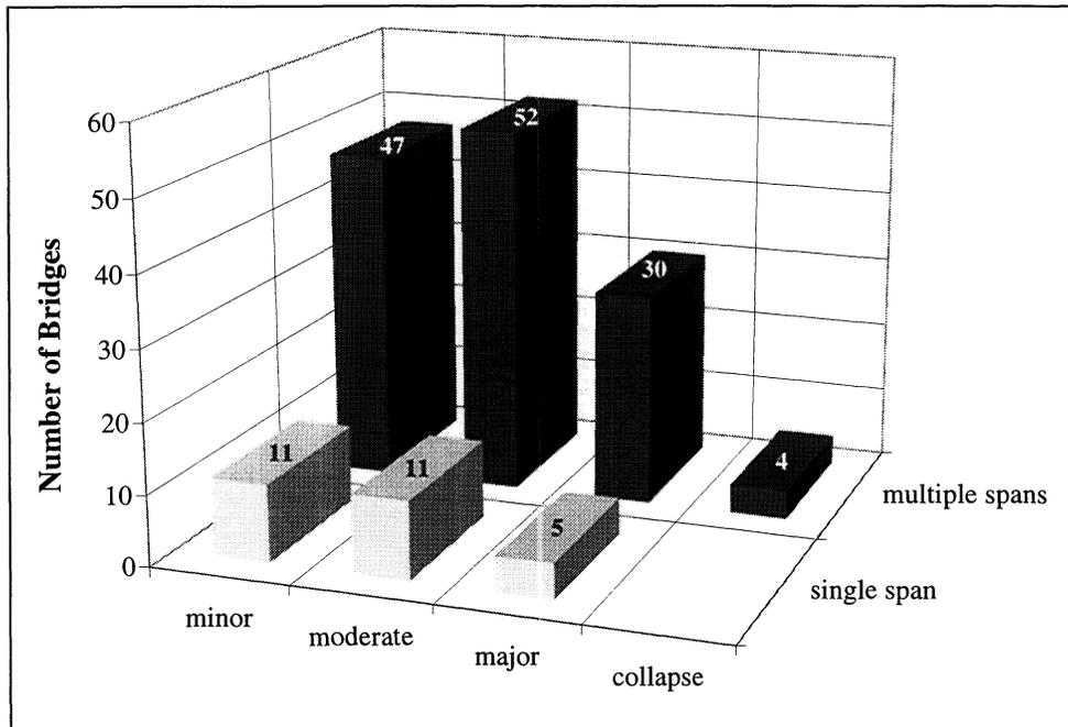
**FIGURE 4-12** Distribution of Damaged Bridges by Number of Spans and Damage State (*correlation data set*)
