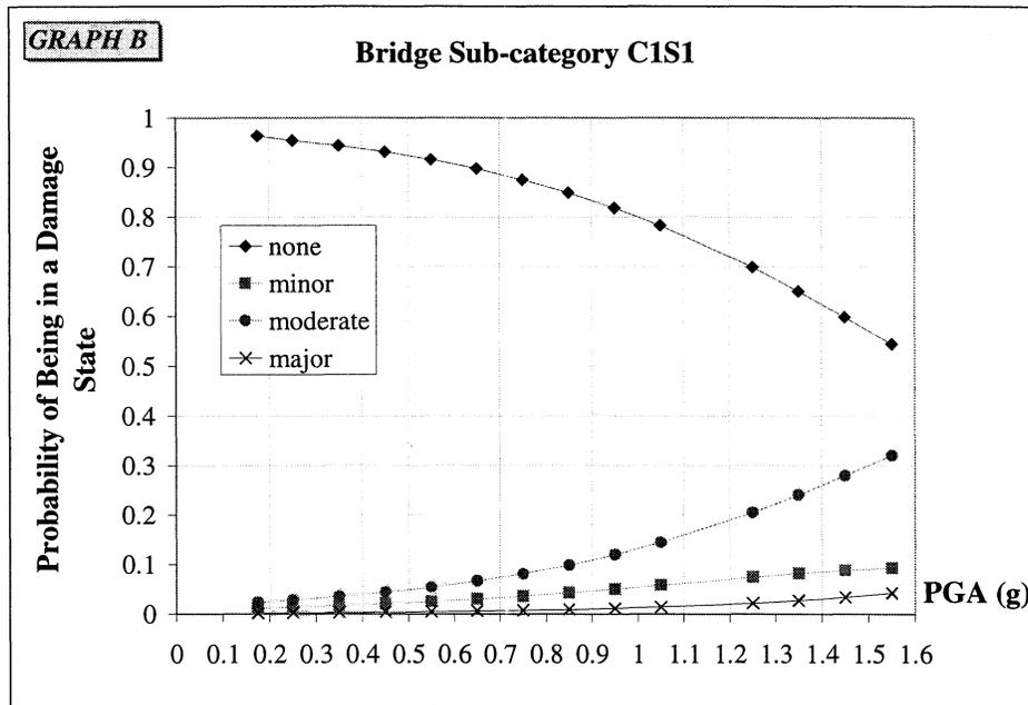
**FIGURE 4-23** Empirical Fragility Curves for Single Span Bridges with Monolithic Type Abutments (Sub-category C1S1)
