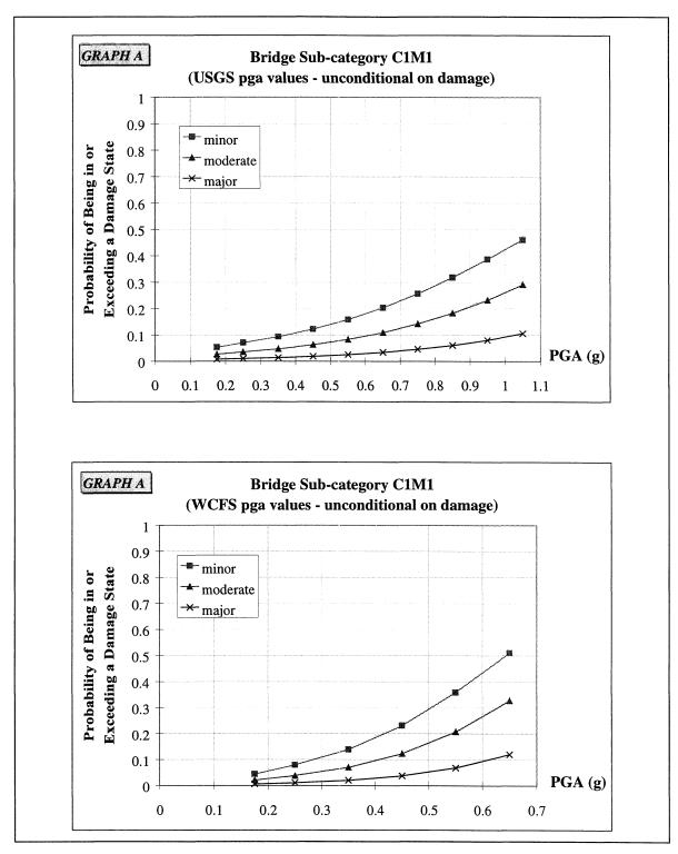
FIGURE 4-52 Empirical Fragility Curves for Multiple Span Bridges with Monolithic Type Abutments, Continuous Spans and Multiple Column Bents (Sub-category C1M1) based on USGS [1994] and WCFS [1995] PGA Values
