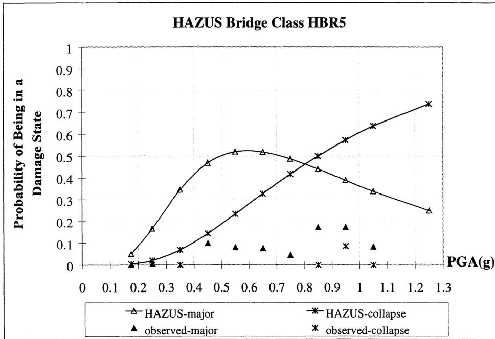
**FIGURE 4-28.b** Comparison of Damage Probabilities from Data to HAZUS Fragility Functions, Major Damage and Collapse
