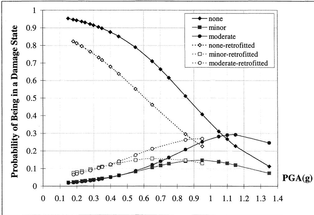
**FIGURE 4-26.a** Comparison of Empirical Fragility Curves for Retrofitted and Unretrofitted Bridges - No Damage, Minor Damage and Moderate Damage
