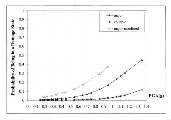
**FIGURE 4-26.b** Comparison of Empirical Fragility Curves for Retrofitted and Unretrofitted
