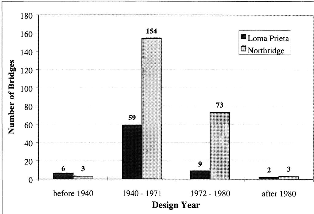
**FIGURE 5-7** Number of Bridges Damaged in the Loma Prieta and Northridge Earthquakes by Design Year
