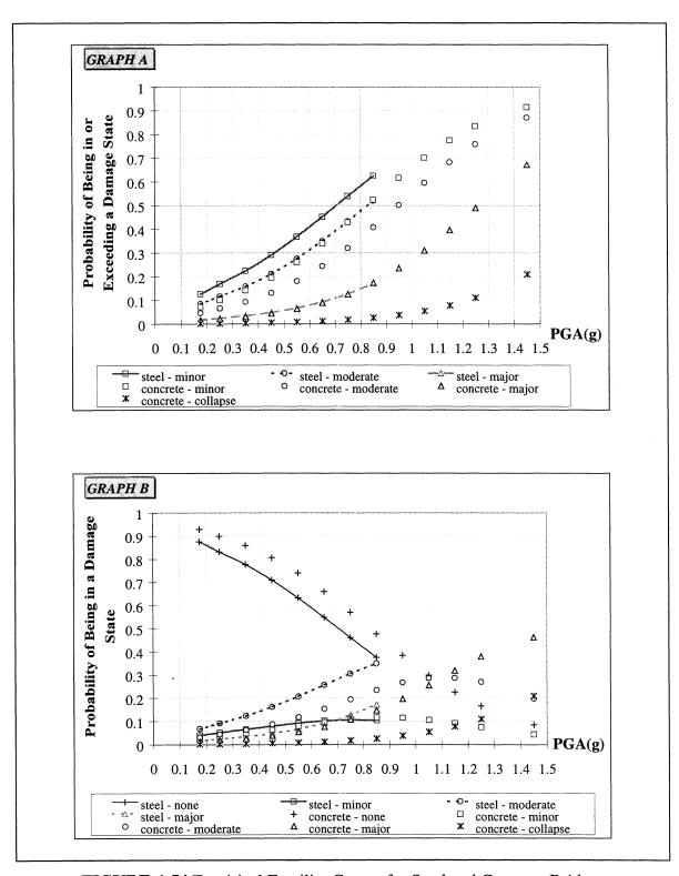
FIGURE 4-54 Empirical Fragility Curves for Steel and Concrete Bridges
