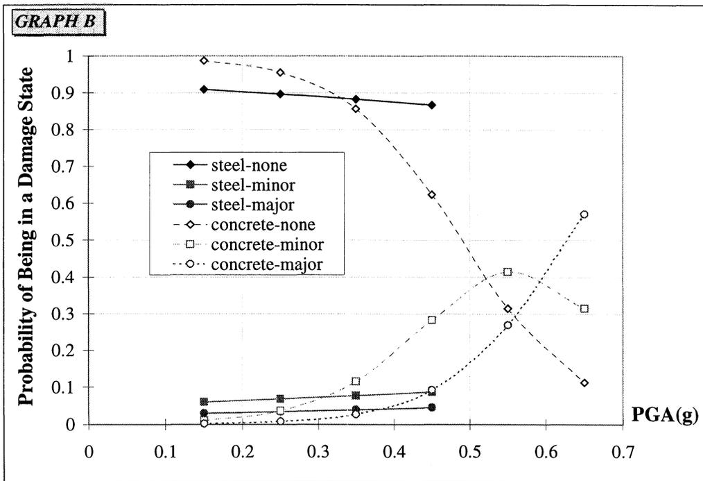
**FIGURE 3-28** Empirical Fragility Curves for Steel and Concrete Bridges
