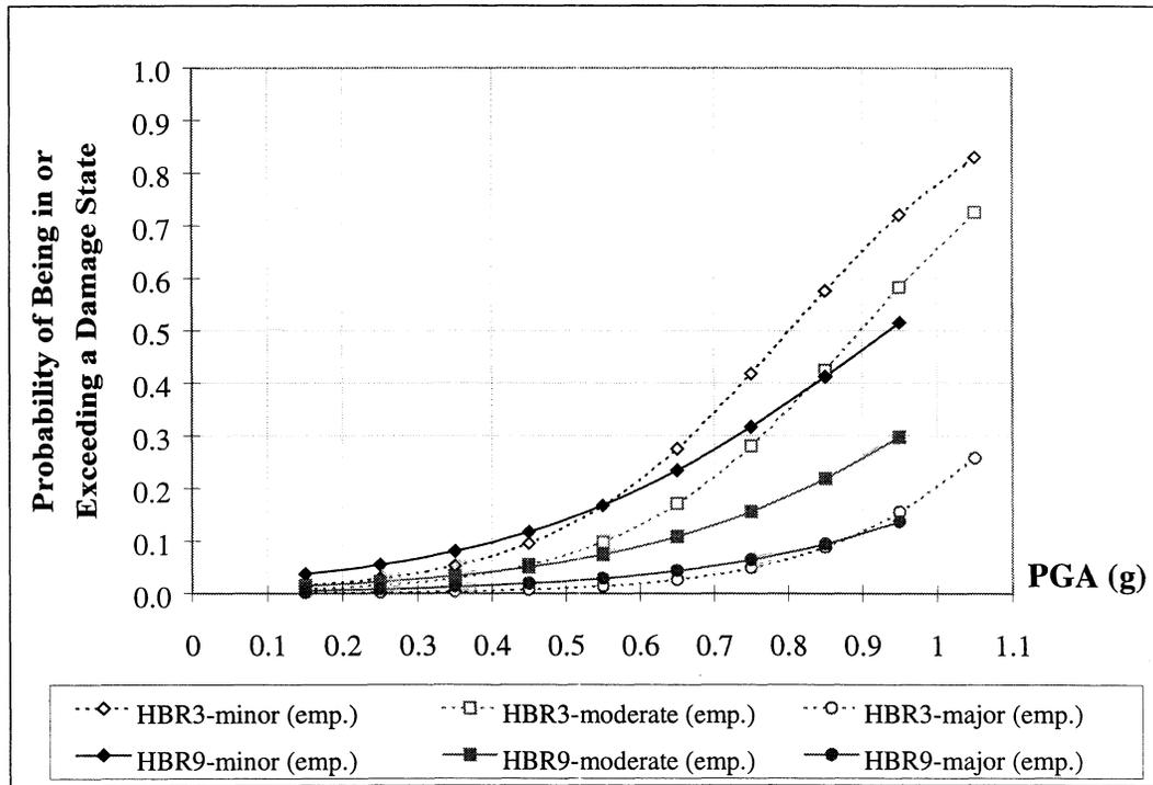
**FIGURE 4-61.a** Empirical Fragility Curves for HAZUS Bridge Classes HBR3 and HBR9
