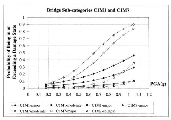
FIGURE 4-60 Empirical Fragility Curves for Sub-categories C1M1 and C1M7
