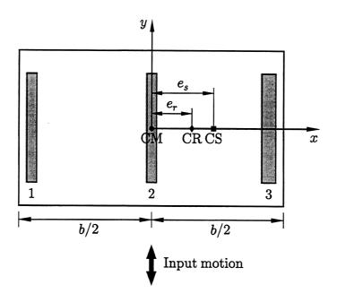
FIGURE 2-2 Plan view of a typical one-storey system
