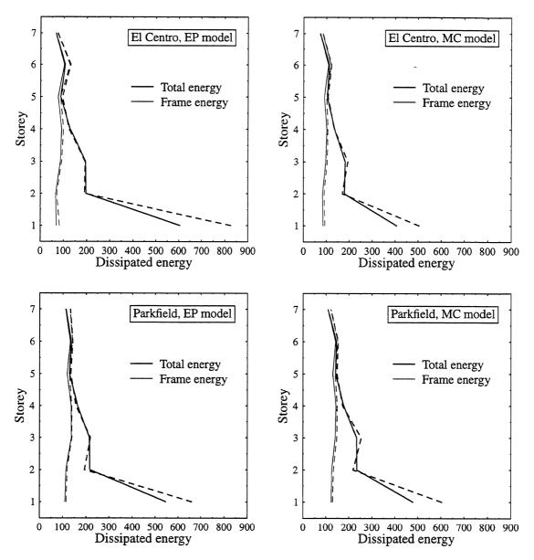
FIGURE 4-12 Dissipated energy (—— sample mean; —— symmetric system).
