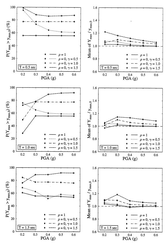
FIGURE 3-37 Comparison of  $Y_{\text{max}}$  and  $y_{\text{max},0}$ . MC model. Input: Parkfield.
