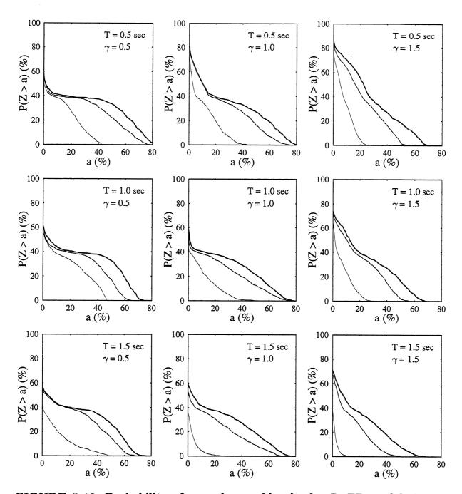
FIGURE 5-13 Probability of exceedence of level a by Z. EP model. Input: Taft. (Lines in increasing width correspond to PGA = 0.2g, 0.4g, and 0.6g.)
