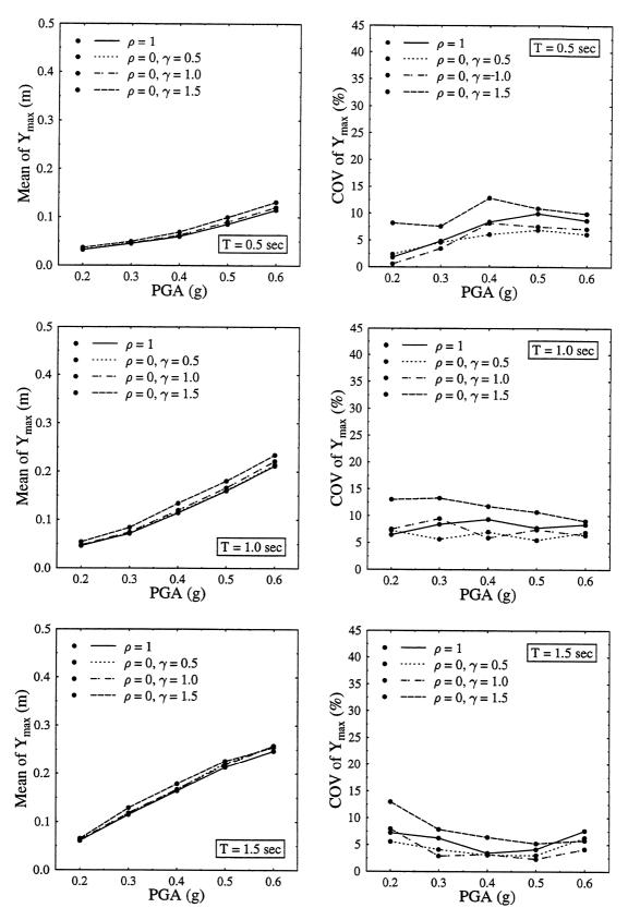
FIGURE 3-30 Mean and COV of  $Y_{\text{max}}$ . MC model. Input: El Centro.
