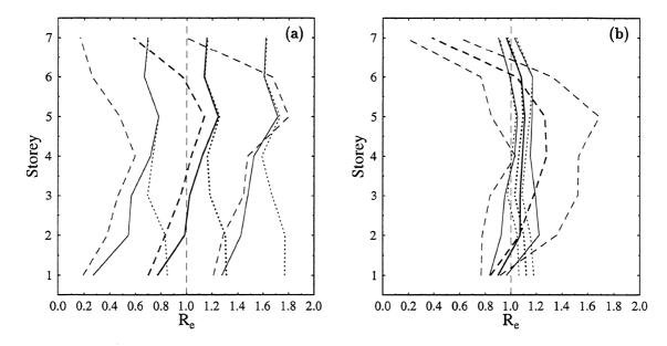
FIGURE 4-14 Ratio of dissipated energy of MC to EP model. (a) Input: El Centro. (b) Input: Parkfield. (····· frames; -- walls; --- total.)
