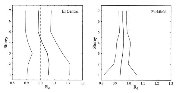
FIGURE 4-10 Ratio of maximum interstorey displacement of MC to EP model.
