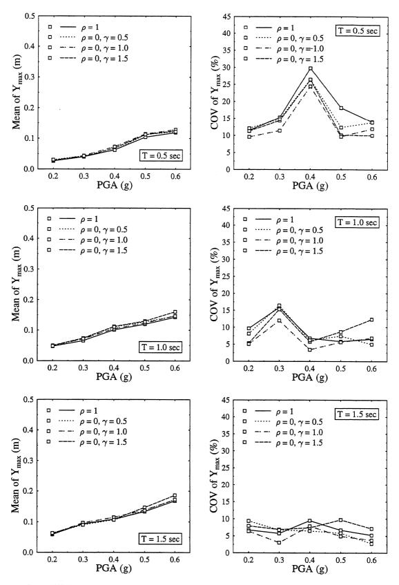
FIGURE 3-7 Mean and COV of  $Y_{\text{max}}$ . EP model. Input: Taft.
