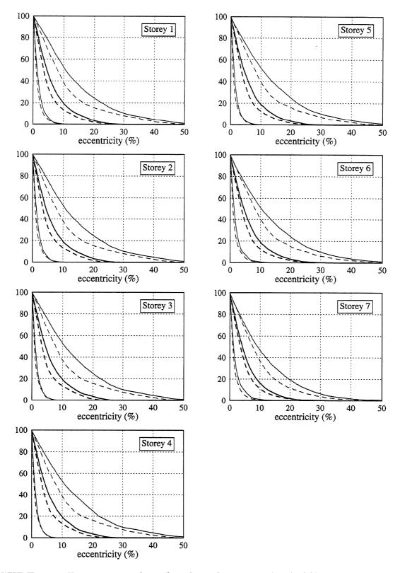
FIGURE 5-19 Percentage of motion duration for which  $|\Theta(t)|$  exceeds specified eccentricity levels. Input: El Centro. (—— EP model; --- MC model)
