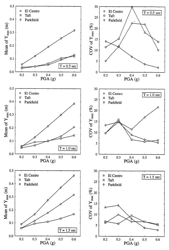
FIGURE 3-9 Mean and COV of  $Y_{\text{max}}$  for perfectly correlated yield strengths. EP model.
