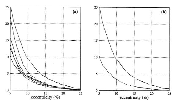
FIGURE 5-5 Percentage of absolute dynamic eccentricity values above specified eccentricity levels. Input: Parkfield scaled to PGA = 0.4g. (a) Results for EP and MC models, T=0.5, 1.0, and 1.5 sec, and  $\gamma=1.5$ . (b) Envelopes of results in (a).
