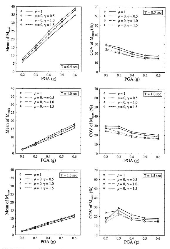
FIGURE 3-19 Mean and COV of  $M_{\text{max}}$ . EP model. Input: Parkfield.
