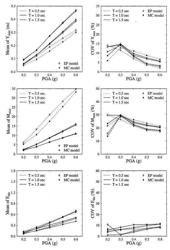
FIGURE 3-56 Mean and COV of  $Y_{\text{max}}$ ,  $M_{\text{max}}$ , and  $E_{\text{dis}}$  for perfectly correlated yield strengths. Input: Parkfield.
