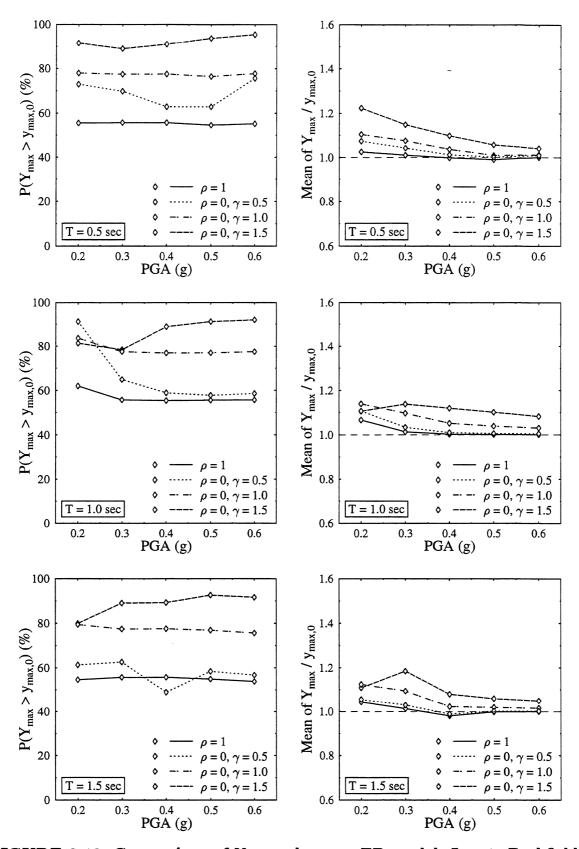
FIGURE 3-13 Comparison of  $Y_{\text{max}}$  and  $y_{\text{max},0}$ . EP model. Input: Parkfield.
