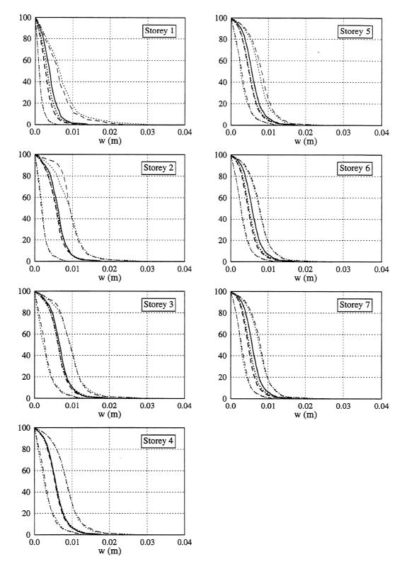
FIGURE 4-5 Percentage of motion duration over which  $|Y_w(t)|$  exceeds level w. MC model. Input: El Centro. (—— symmetric system; ····· wall 1; -- wall 2)
