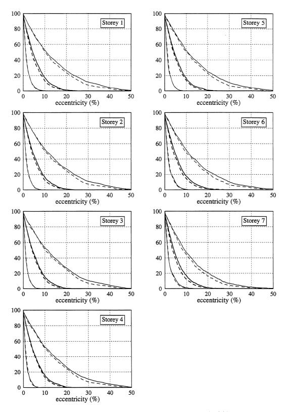
FIGURE 5-20 Percentage of motion duration for which  $|\Theta(t)|$  exceeds specified eccentricity levels. Input: Parkfield. (—— EP model; -- MC model)
