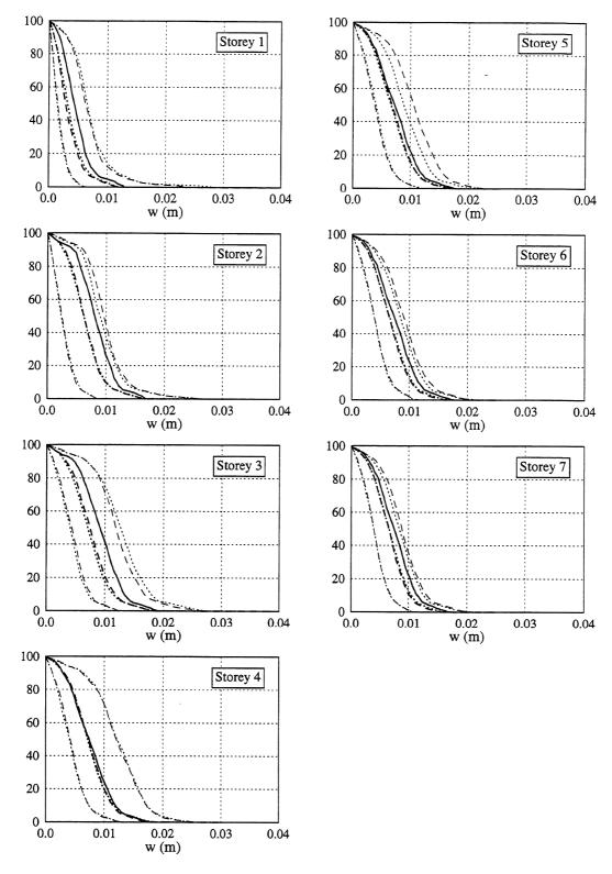
FIGURE 4-4 Percentage of motion duration over which  $|Y_w(t)|$  exceeds level w. EP model. Input: El Centro. (—— symmetric system; · · · · · wall 1; - - · wall 2)
