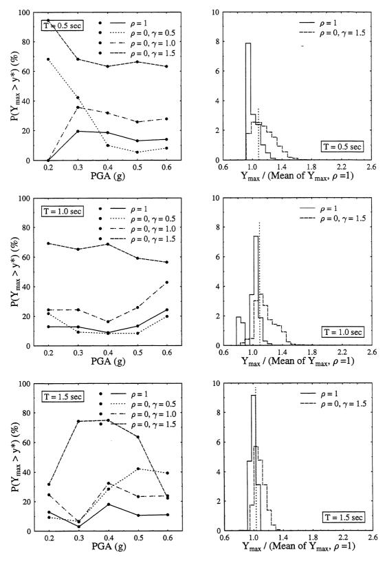
FIGURE 3-38 Probability of exceedence of level  $y^*$  and histograms of normalized maximum displacement. MC model. Input: El Centro.
