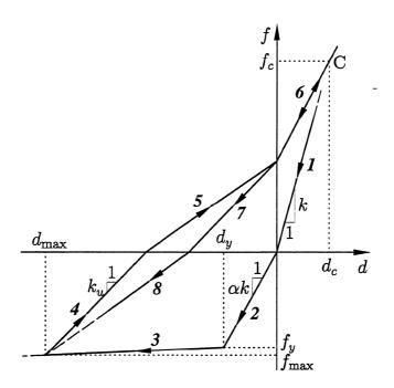
FIGURE 4-3 Axial restoring force model.
