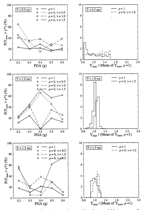
FIGURE 3-15 Probability of exceedence of level  $y^*$  and histograms of normalized maximum displacement. EP model. Input: Taft.
