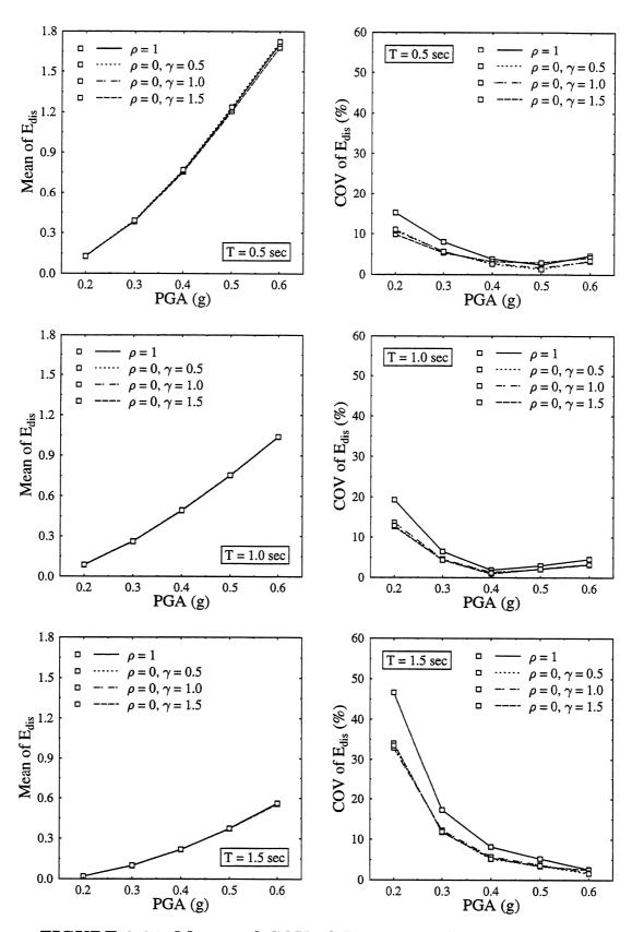
FIGURE 3-24 Mean and COV of  $E_{\rm dis}$ . EP model. Input: Taft.
