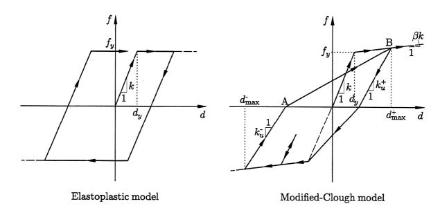
FIGURE 3-2 Restoring force models.
