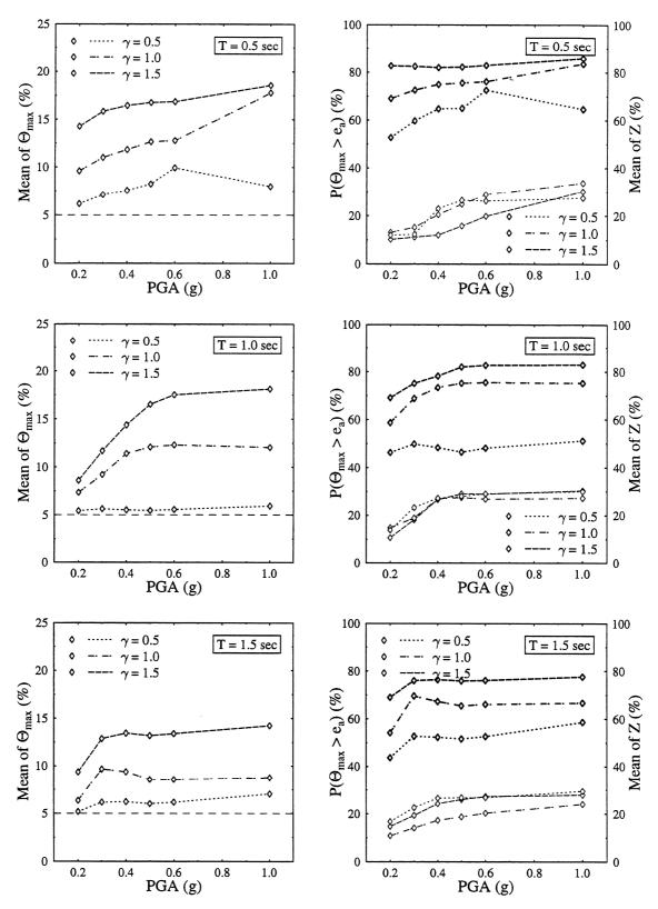
FIGURE 5-8 Mean of  $\Theta_{\max}$ , probability of exceedence of  $e_a$  by  $\Theta_{\max}$ , and mean of Z. EP model. Input: Parkfield.
