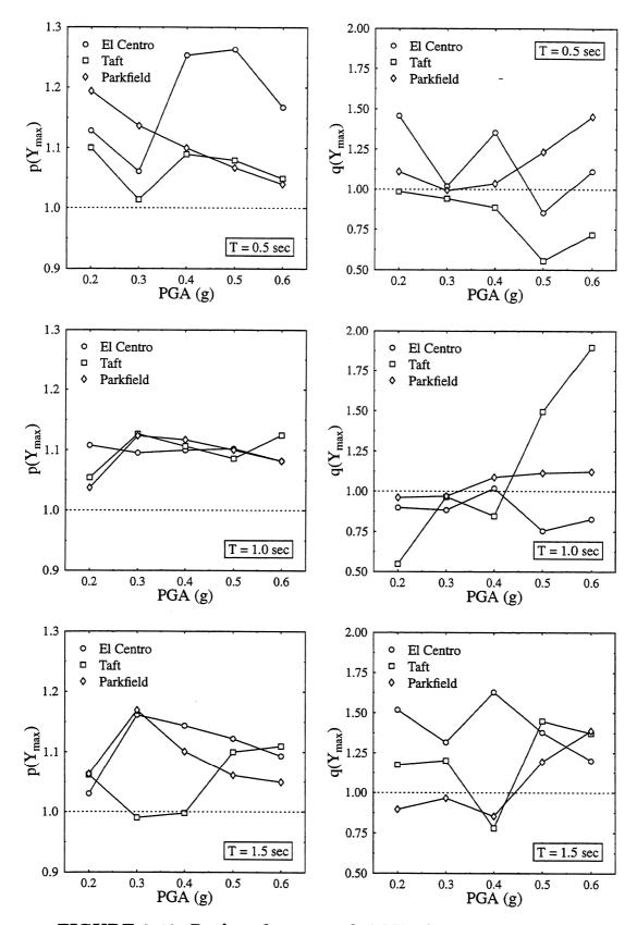
FIGURE 3-10 Ratios of mean and COV of  $Y_{\text{max}}$ . EP model.
