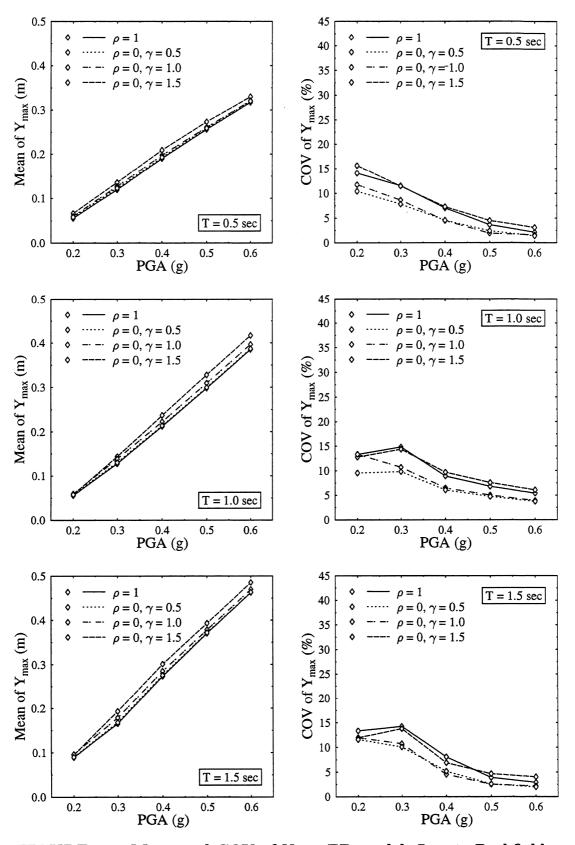
FIGURE 3-8 Mean and COV of  $Y_{\text{max}}$ . EP model. Input: Parkfield.
