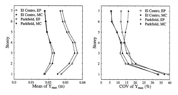
FIGURE 4-9 Mean and COV of maximum interstorey displacement  $Y_{\text{max}}$ .
