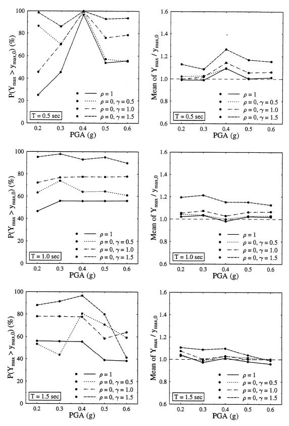
FIGURE 3-35 Comparison of  $Y_{\rm max}$  and  $y_{{\rm max},0}.$  MC model. Input: El Centro.
