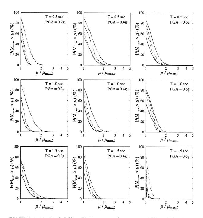
FIGURE 3-44 Probability of  $M_{\text{max}}$  exceeding  $\mu_{\text{max},0}$ . MC model. Input: El Centro. (——  $\rho=1; \cdots \cdot \rho=0, \ \gamma=0.5; -\cdot -\cdot \ \rho=0, \ \gamma=1.0; ---- \ \rho=0, \ \gamma=1.5$ )
