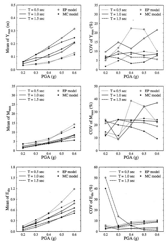
FIGURE 3-54 Mean and COV of  $Y_{\text{max}}$ ,  $M_{\text{max}}$ , and  $E_{\text{dis}}$  for perfectly correlated yield strengths. Input: El Centro.
