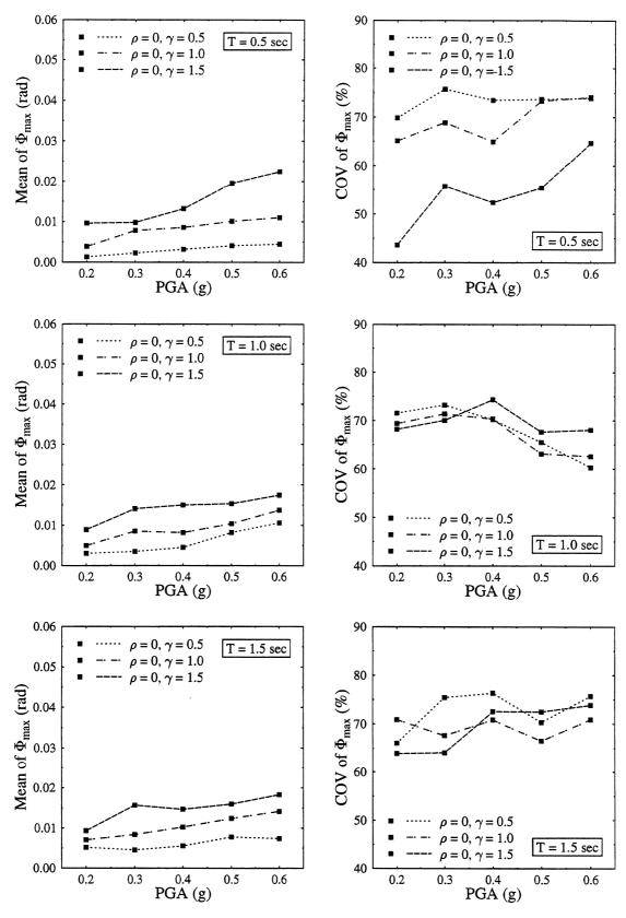
FIGURE 3-52 Mean and COV of  $\Phi_{\text{max}}$ . MC model. Input: Taft.
