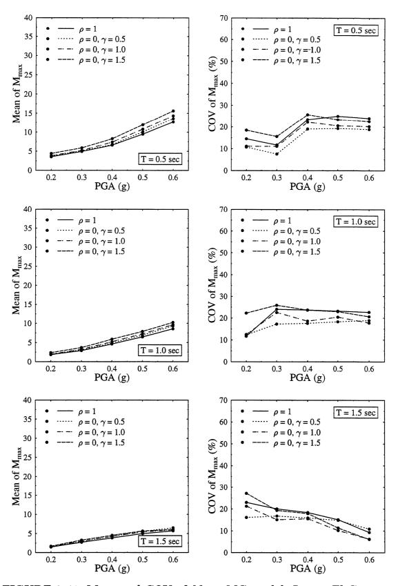
FIGURE 3-41 Mean and COV of  $M_{\text{max}}$ . MC model. Input: El Centro.
