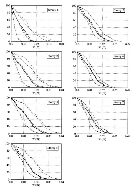
FIGURE 4-7 Percentage of motion duration over which  $|Y_w(t)|$  exceeds level w. MC model. Input: Parkfield. (—— symmetric system; · · · · · wall 1; - - · wall 2)
