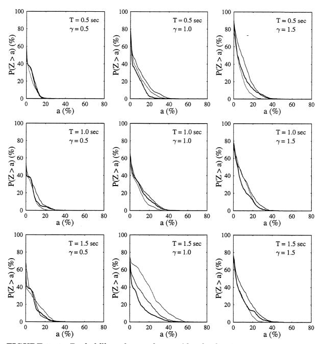
FIGURE 5-15 Probability of exceedence of level a by Z. MC model. Input: El Centro. (Lines in increasing width correspond to PGA = 0.2g, 0.4g, and 0.6g.)
