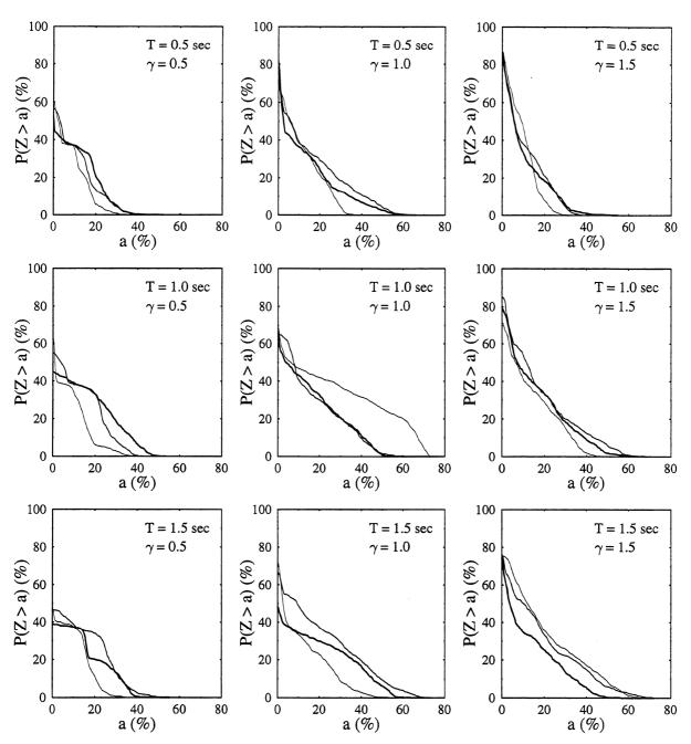
FIGURE 5-17 Probability of exceedence of level a by Z. MC model. Input: Parkfield. (Lines in increasing width correspond to PGA = 0.2g, 0.4g, and 0.6g.)
