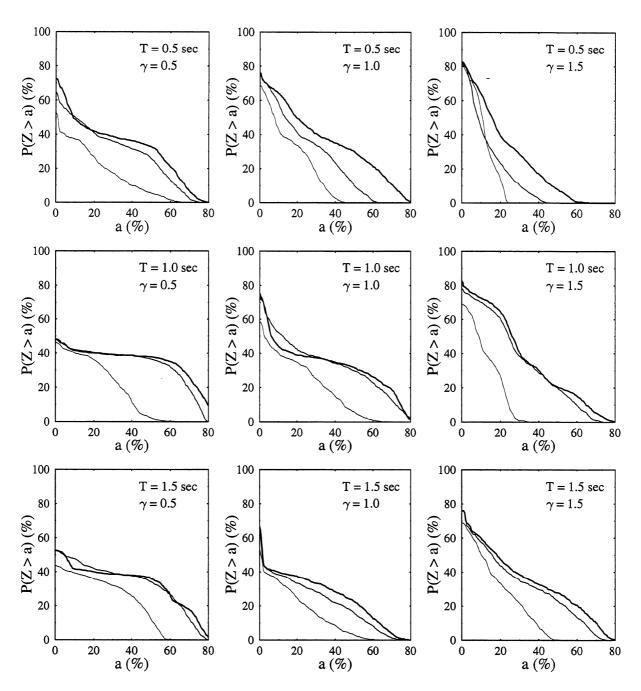
FIGURE 5-14 Probability of exceedence of level a by Z. EP model. Input: Parkfield. (Lines in increasing width correspond to PGA = 0.2g, 0.4g, and 0.6g.)
