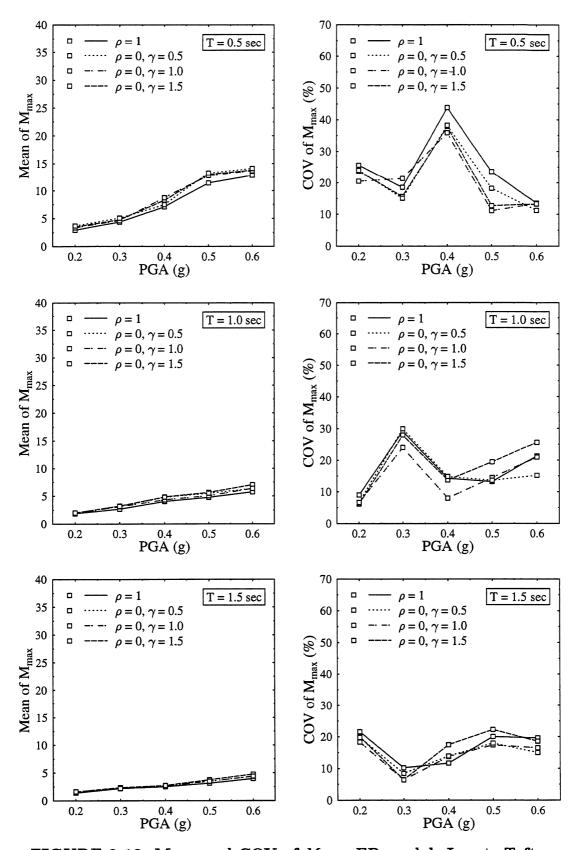
FIGURE 3-18 Mean and COV of  $M_{\text{max}}$ . EP model. Input: Taft.
