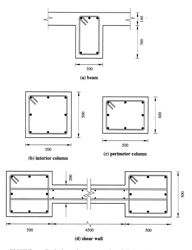
FIGURE 4-2 Typical member cross sections (all dimensions in mm).
