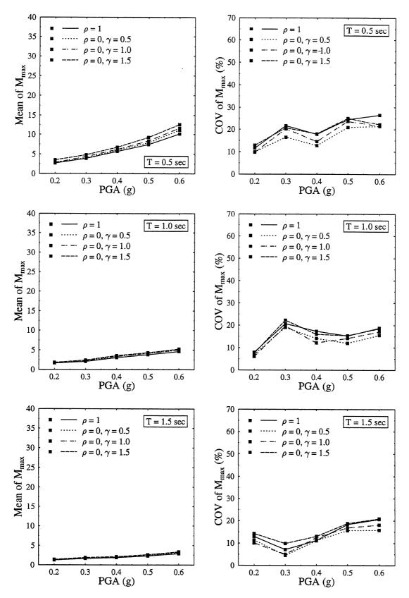
FIGURE 3-42 Mean and COV of  $M_{\text{max}}$ . MC model. Input: Taft.
