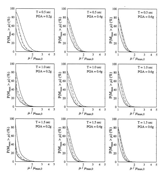
FIGURE 3-46 Probability of  $M_{\text{max}}$  exceeding  $\mu_{\text{max},0}$ . MC model. Input: Parkfield. (——  $\rho = 1; \cdots \rho = 0, \gamma = 0.5; - \rho = 0, \gamma = 1.0; - - \rho = 0, \gamma = 1.5)$
