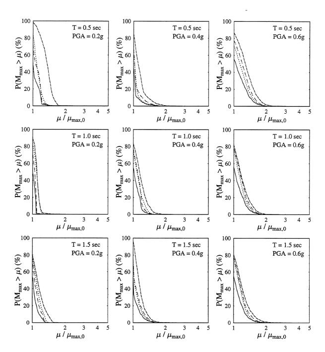
FIGURE 3-45 Probability of  $M_{\rm max}$  exceeding  $\mu_{\rm max,0}$ . MC model. Input: Taft. (——  $\rho=1;$  ·····  $\rho=0,$   $\gamma=0.5;$  -··  $-\cdot$   $\rho=0,$   $\gamma=1.0;$  ---  $\rho=0,$   $\gamma=1.5)$
