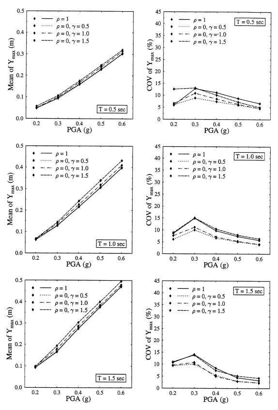
FIGURE 3-32 Mean and COV of  $Y_{\text{max}}$ . MC model. Input: Parkfield.
