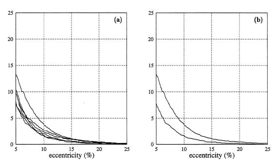
FIGURE 5-3 Percentage of absolute dynamic eccentricity values above specified eccentricity levels. Input: El Centro scaled to PGA = 0.4g. (a) Results for EP and MC models, T=0.5, 1.0, and 1.5 sec, and  $\gamma=1.5$ . (b) Envelopes of results in (a).
