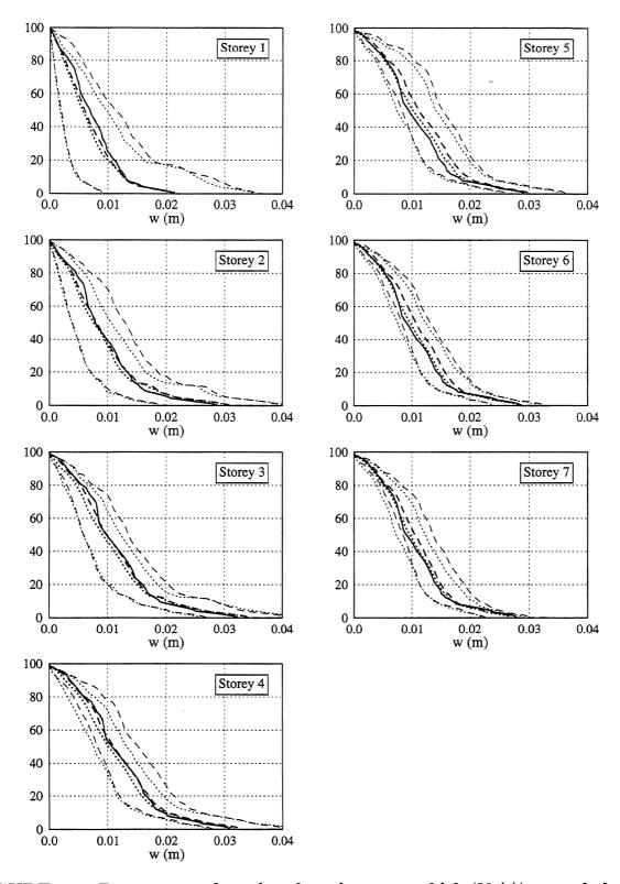
FIGURE 4-6 Percentage of motion duration over which  $|Y_w(t)|$  exceeds level w. EP model. Input: Parkfield. (—— symmetric system; · · · · · wall 1; - - - wall 2)
