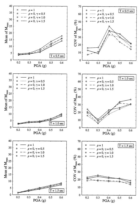
FIGURE 3-17 Mean and COV of  $M_{\rm max}$ . EP model. Input: El Centro.
