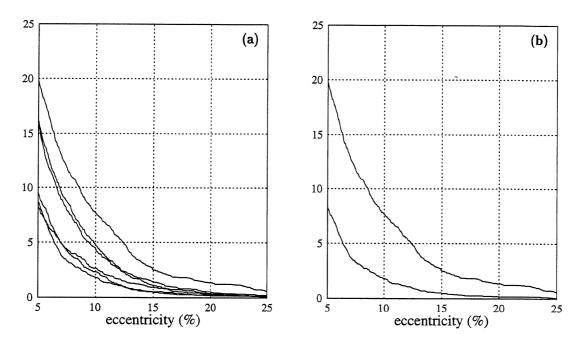
FIGURE 5-4 Percentage of absolute dynamic eccentricity values above specified eccentricity levels. Input: Taft scaled to PGA = 0.4g. (a) Results for EP and MC models, T=0.5, 1.0, and 1.5 sec, and  $\gamma=1.5$ . (b) Envelopes of results in (a).
