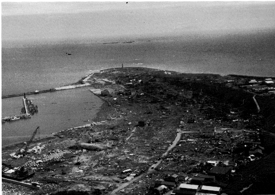
Figure 6-4: The sea-level southern tip of Aonae showing near total destruction of buildings. All destroyed buildings, mostly two-story, were wood frame. Note that the area is completely surrounded by protective, up to 4.5-m tsunami walls. They were ineffective in preventing the destruction, although they probably moderated the height of the run-up, which was 10 to 15 m high. The lower photograph shows much of Aonae, looking south. Photographs by K. Kawashima.
