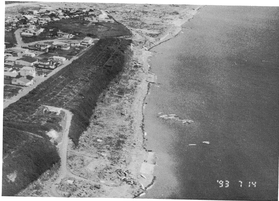
Figure 5-3: Evidence of tsunami inundation along the western shoreline of Okushiri Island just north of Aonae town. The run-up is about 15 m. All the telephone power lines are new; the old ones were destroyed. The vegetation remains along the road railing are from the tsunami. All buildings in this area along the coast at or near sea level were destroyed (lower photograph; courtesy of K. Kawashima).
