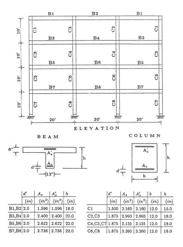
FIGURE 5-1 Details of a Three Bay Four Story Building Frame (1 in = 2.54 cm; 1 kip = 4.448 kN)
