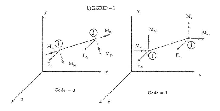
FIGURE 3-6 Fixed End Forces and Initial Force Patterns
