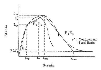
FIGURE 3-3 Stress-Strain Curve for Concrete
