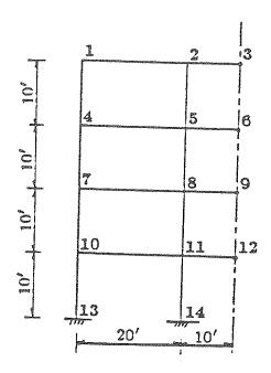
FIGURE 5-3 Half of Four Story Three Bay Building Frame
