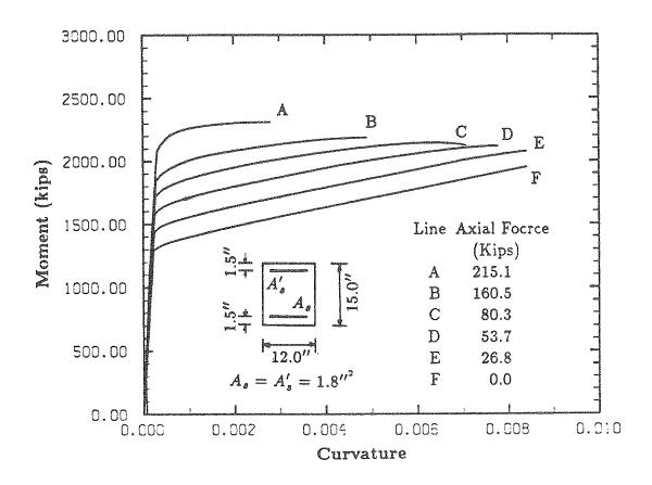
FIGURE 2-1 Effect of Axial Force on the Primary Moment-Curvature Curve
