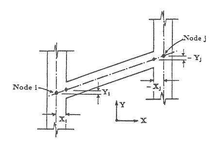
FIGURE 3-5 End Eccentricities of Frame Element
