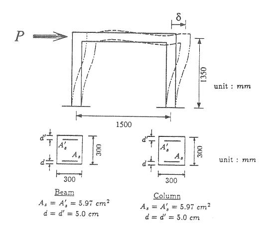
FIGURE 5-4 Details of Ohno's Experimental Frame
