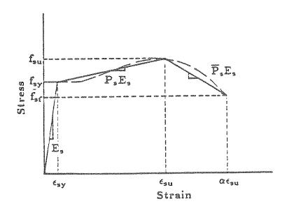
FIGURE 3-2 Stress-Strain Curve for Reinforcing Steel
