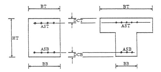
FIGURE 3-4 Idealized Concrete Cross Sections
