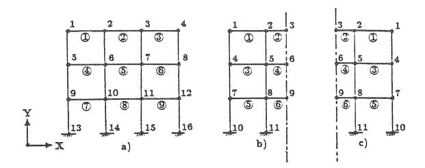
FIGURE 3-1 Node and Element Numbering Sequence
