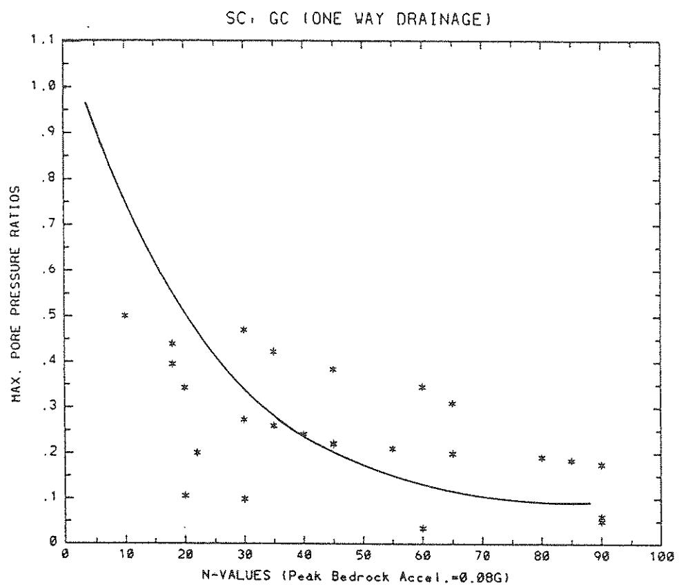
FIGURE 3-1 Pore Pressure Ratios vs. In Situ N-Values for SC-GC
