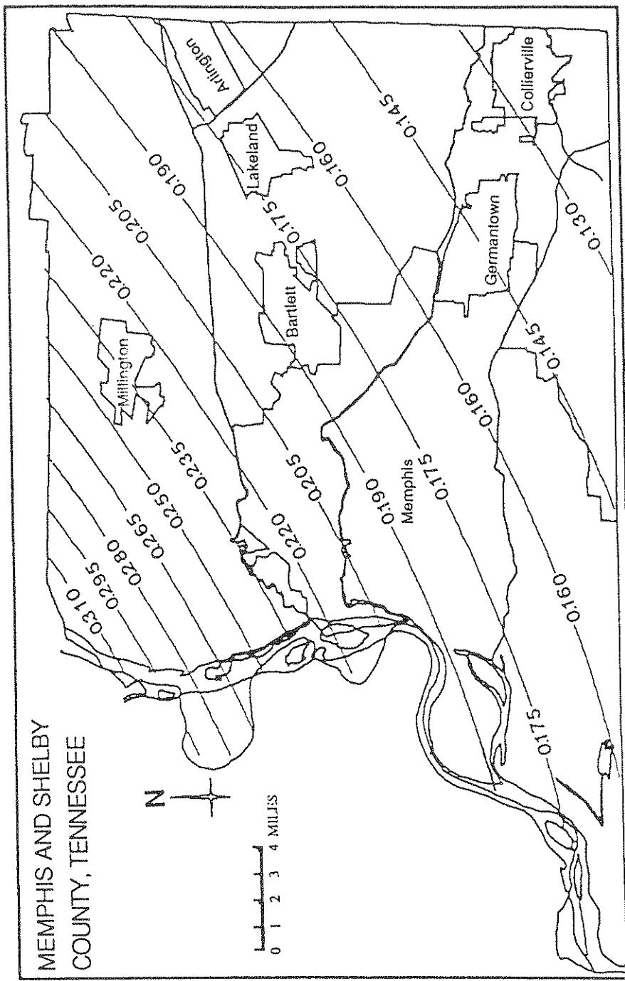
FIGURE 4-2 Bedrock Acceleration ( $g$ ) Contour Map of Mean + S.D.
