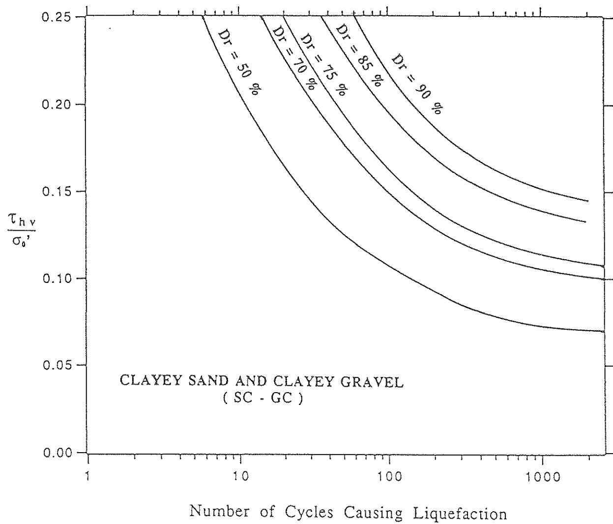
FIGURE 2-4 Cyclic Loading Test Data for Clayey Sand and Clayey Gravel
