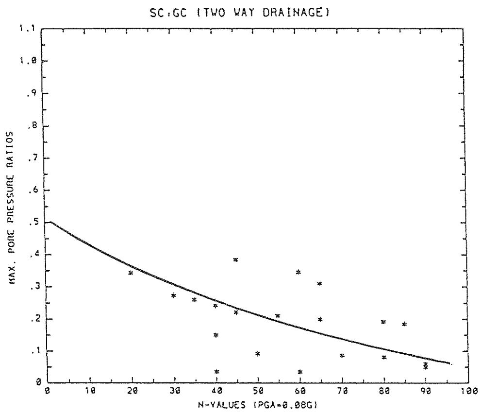
FIGURE A-9 Pore Pressure Ratios vs. In Situ N-Values for SC-GC
