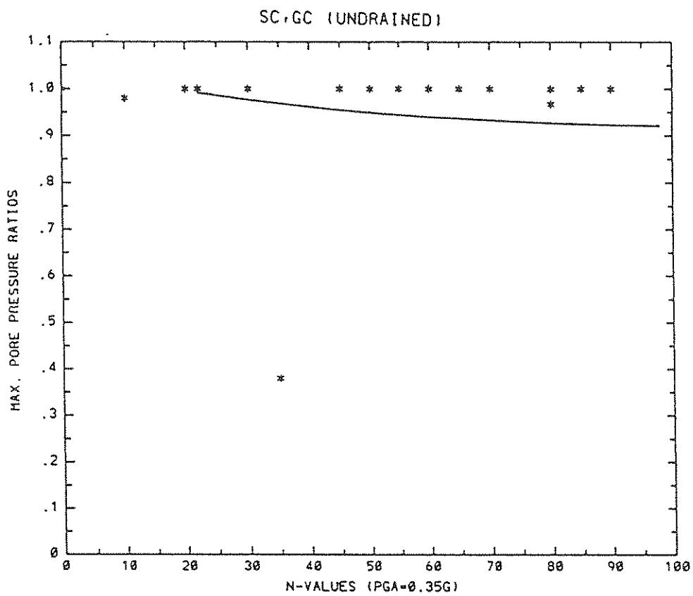
FIGURE A-16 Pore Pressure Ratios vs. In Situ N-Values for SC-GC
