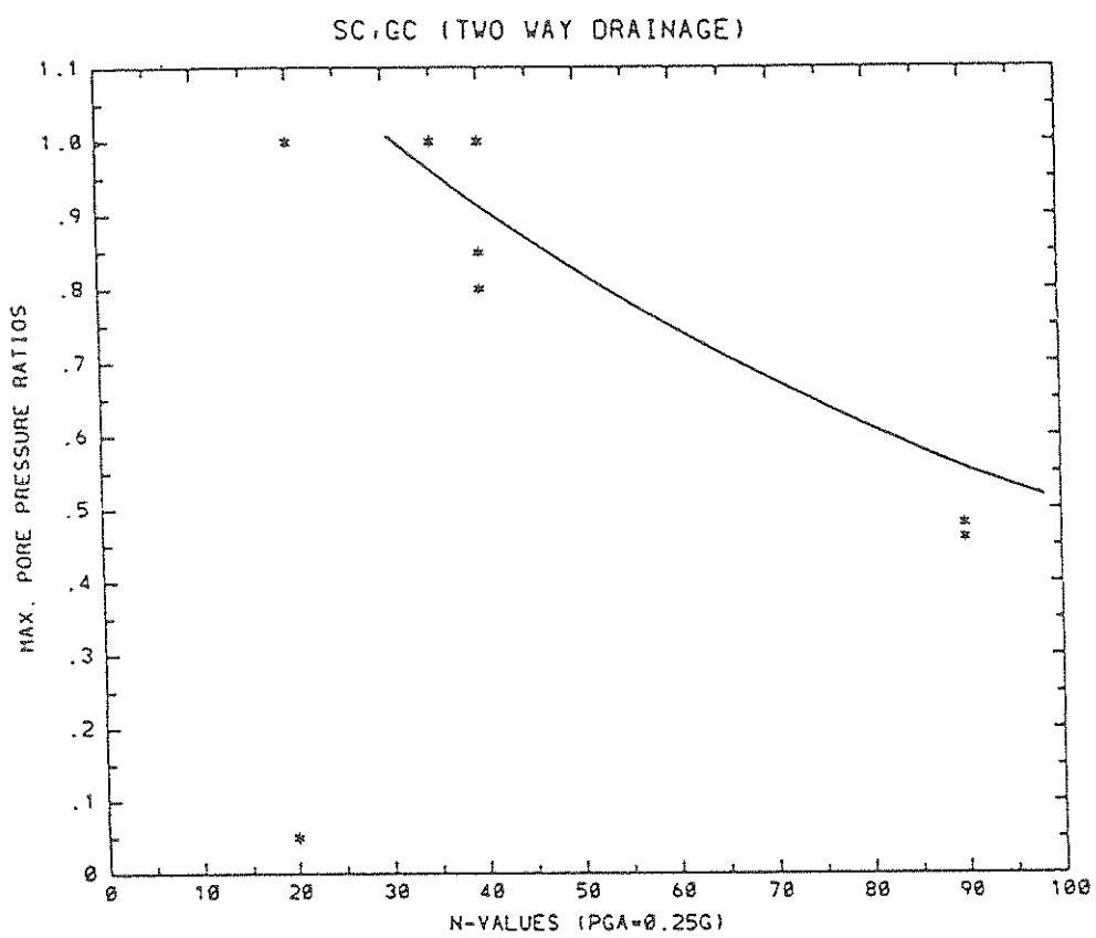
FIGURE A-11 Pore Pressure Ratios vs. In Situ N-Values for SC-GC
