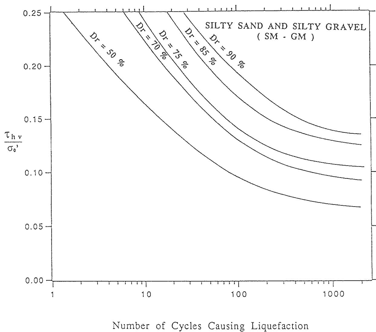
FIGURE 2-3 Cyclic Loading Test Data for Silty Sand and Silty Gravel
