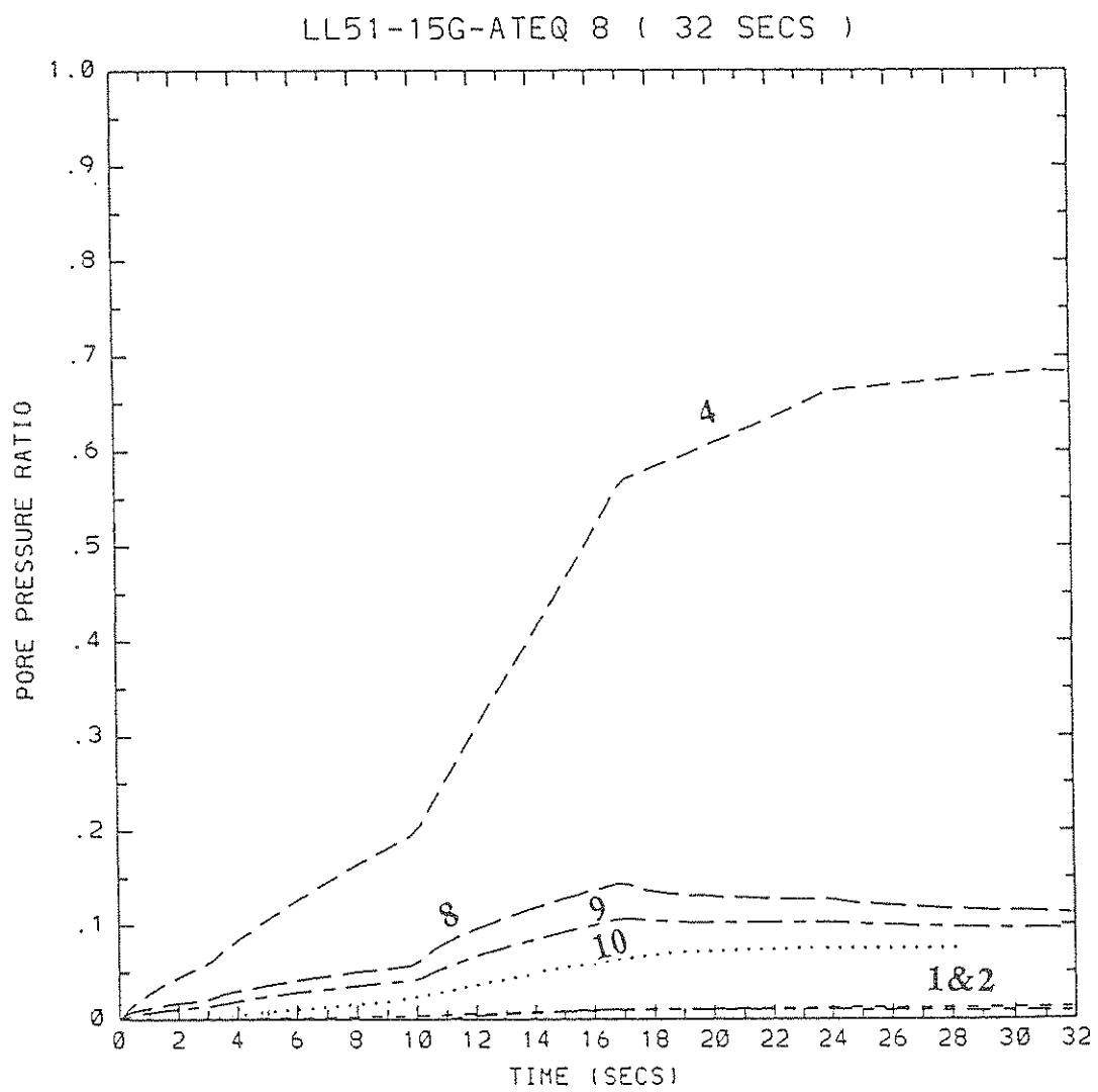
FIGURE 2-8 Pore Pressure Buildup with Time of Granular Soil Elements Number 1, 2, 4, 8, 9, and 10 of Site LL51 Subjected to 0.15 g Earthquake Expressed in Terms of Pore Pressure Ratio
