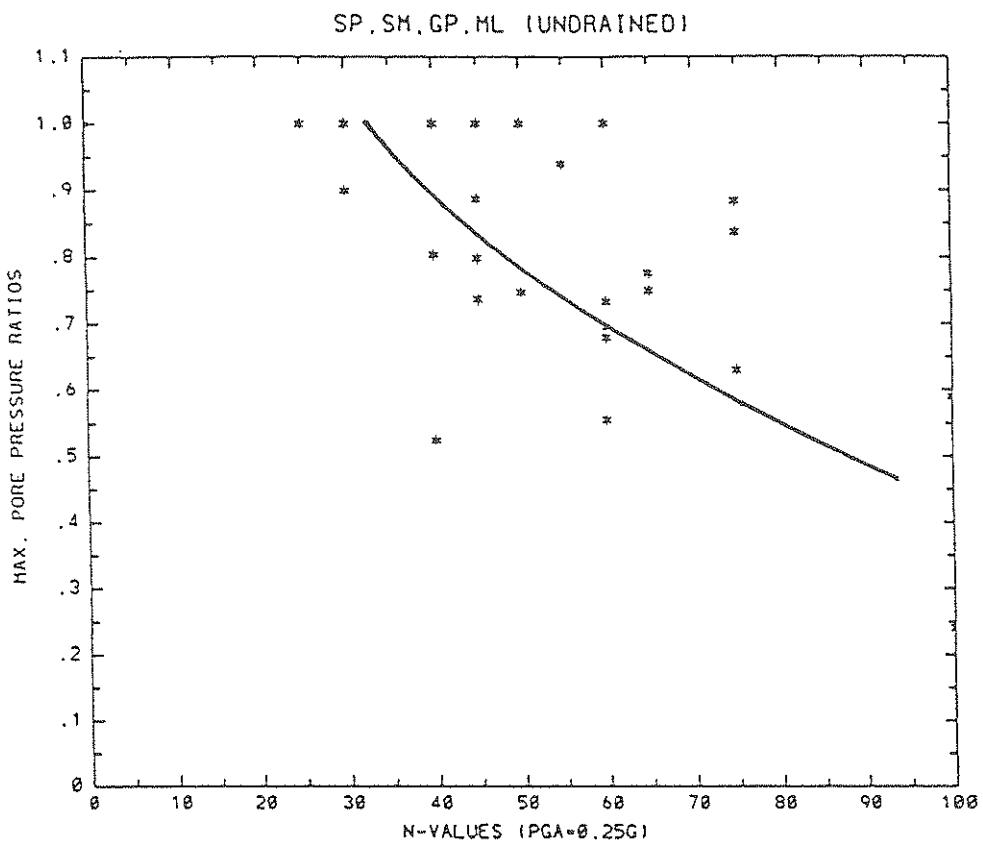
FIGURE A-7 Pore Pressure Ratios vs. In Situ N-Values for SP-SM-GP-ML (Undrained, 0.25 g)
