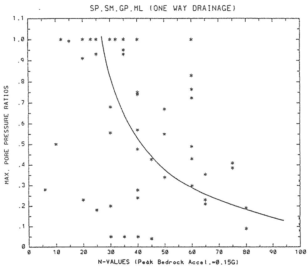
FIGURE 3-6 Pore Pressure Ratios vs. In Situ N-Values for
