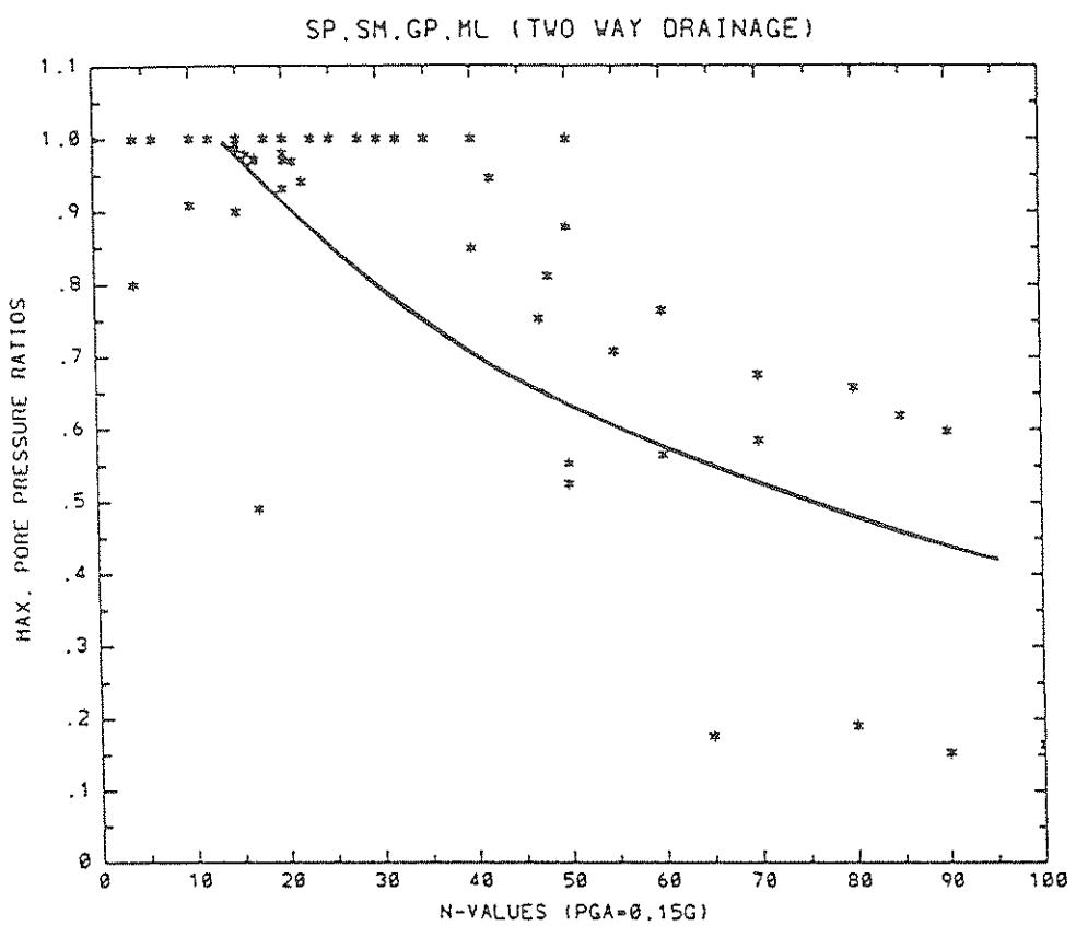
FIGURE A-2 Pore Pressure Ratios vs. In Situ N-Values for
