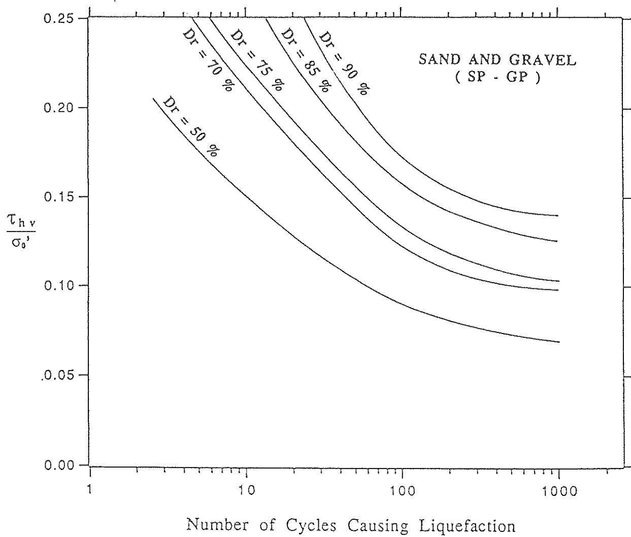
FIGURE 2-2 Cyclic Loading Test Data for Sand and Gravel
