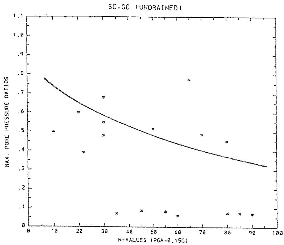
FIGURE A-14 Pore Pressure Ratios vs. In Situ N-Values for SC-GC
