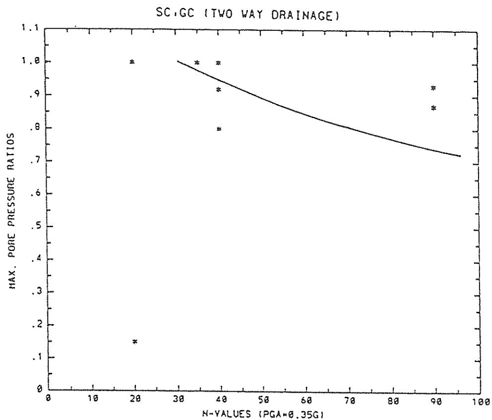
FIGURE A-12 Pore Pressure Ratios vs. In Situ N-Values for SC-GC
