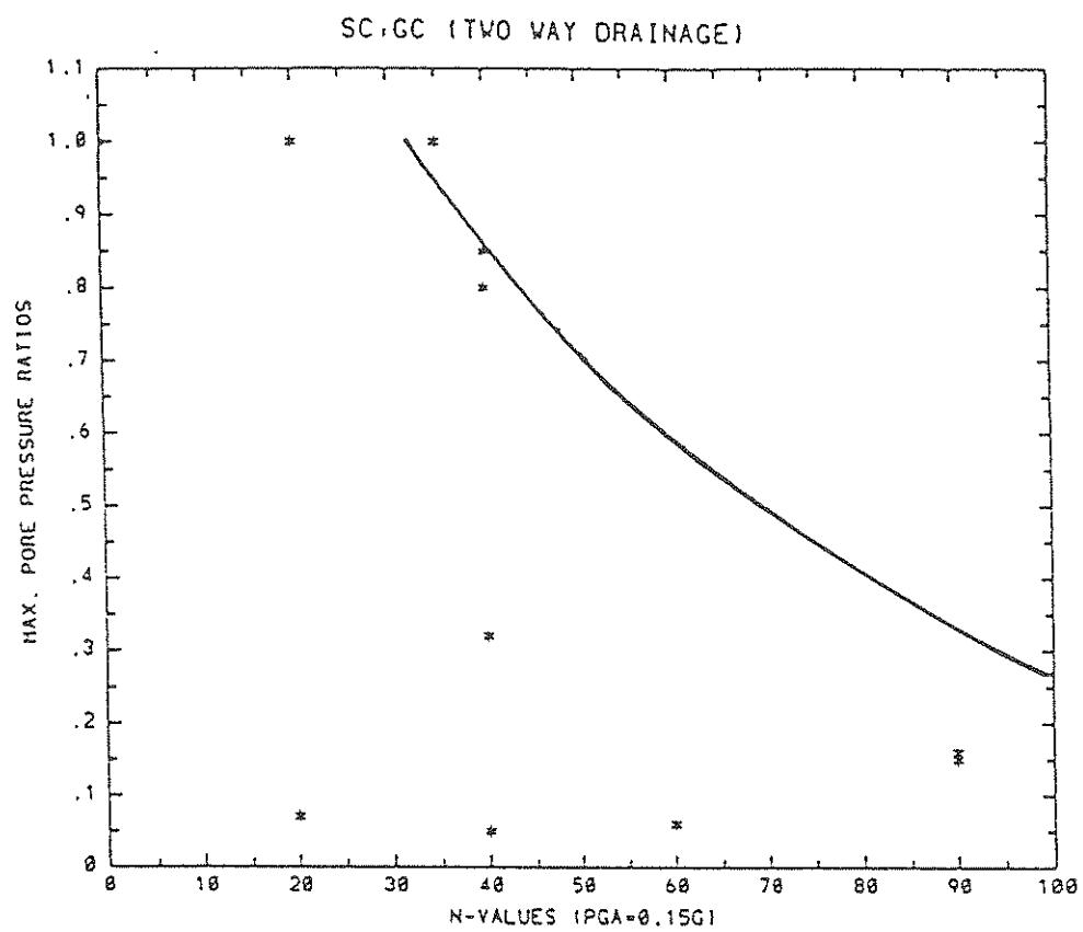
FIGURE A-10 Pore Pressure Ratios vs. In Situ N-Values for SC-GC
