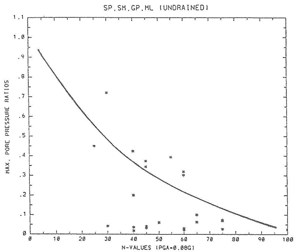
FIGURE A-5 Pore Pressure Ratios vs. In Situ N-Values for
