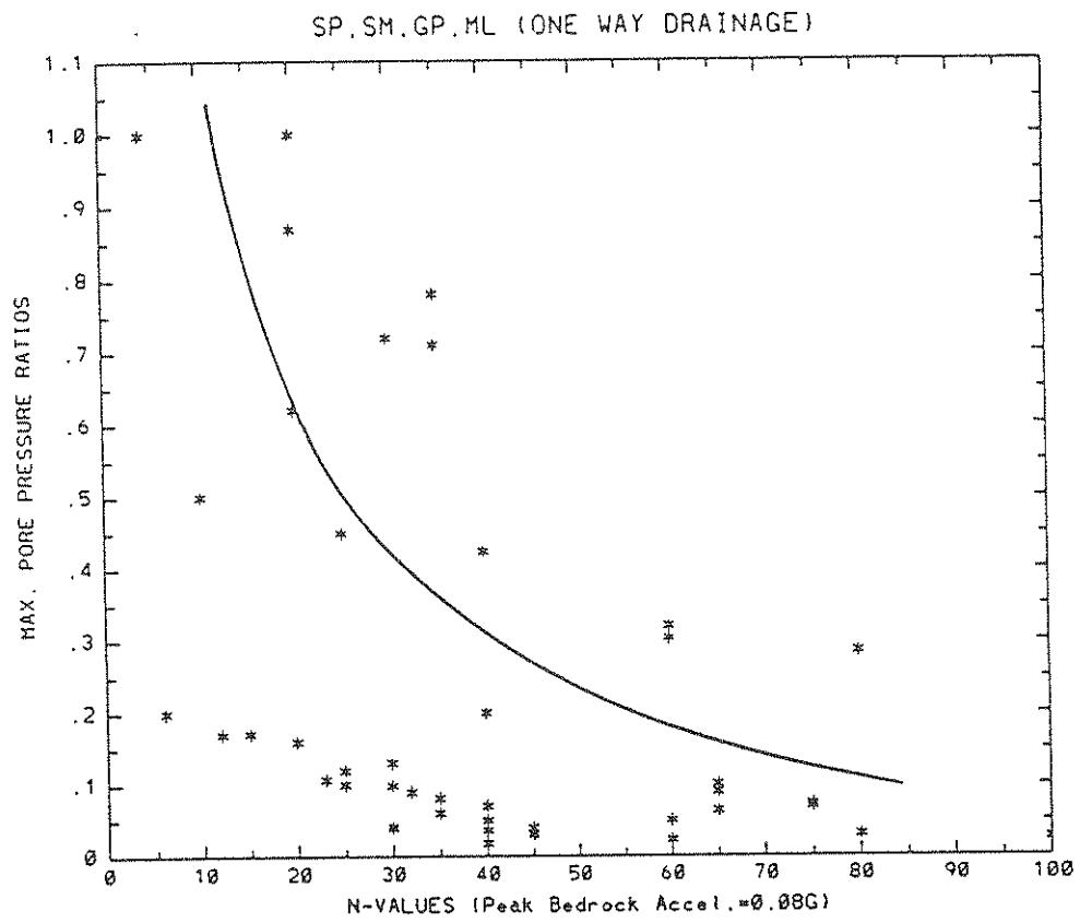
FIGURE 3-5 Pore Pressure Ratios vs. In Situ N-Values for
