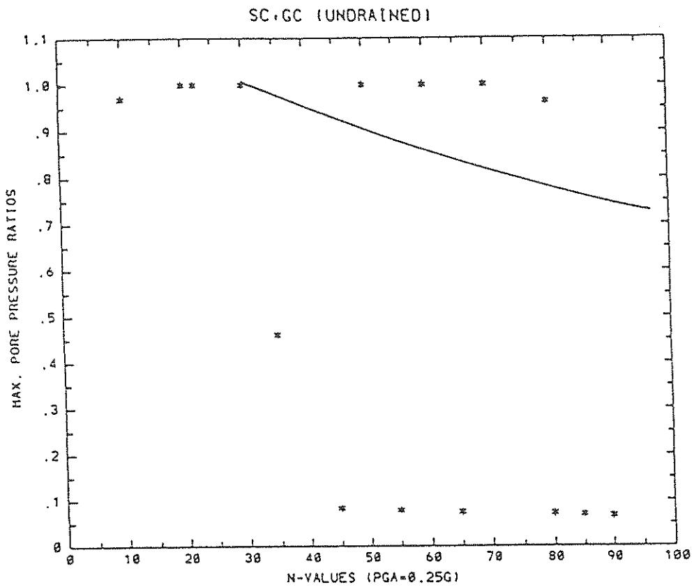
FIGURE A-15 Pore Pressure Ratios vs. In Situ N-Values for SC-GC
