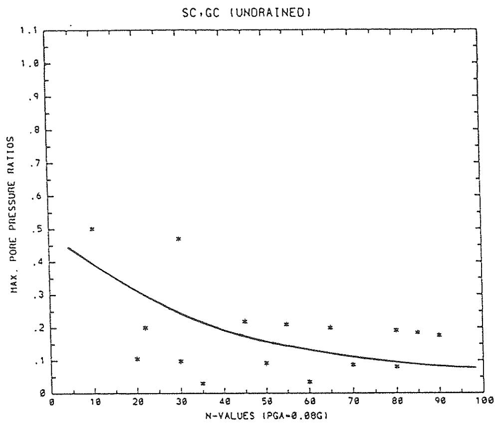
FIGURE A-13 Pore Pressure Ratios vs. In Situ N-Values for SC-GC
