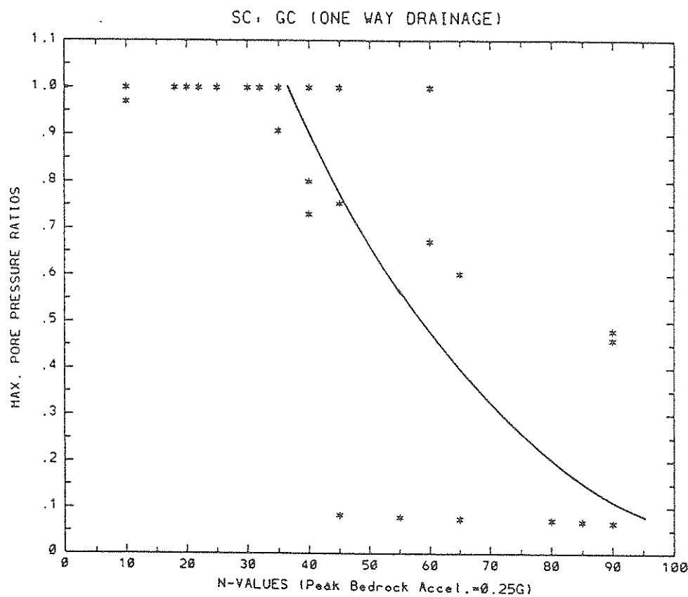
FIGURE 3-3 Pore Pressure Ratios vs. In Situ N-Values for SC-GC
