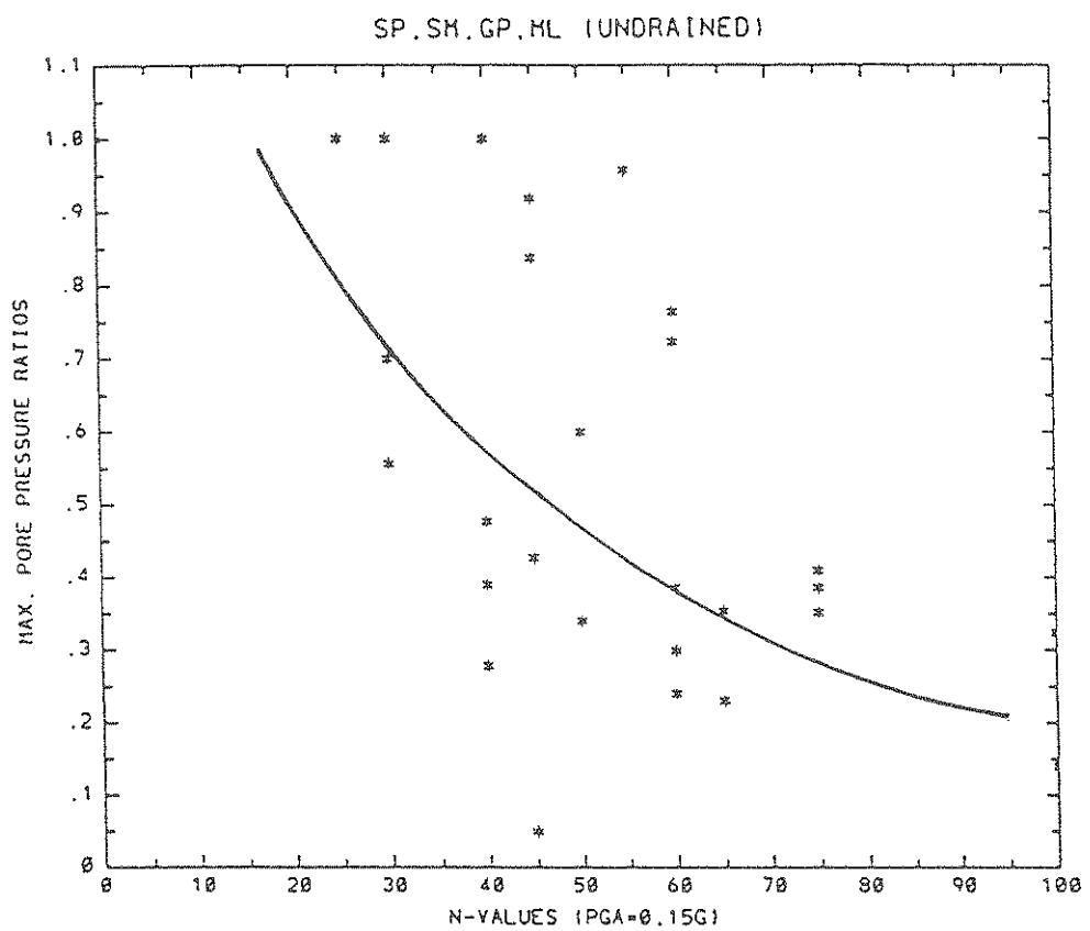
FIGURE A-6 Pore Pressure Ratios vs. In Situ N-Values for
