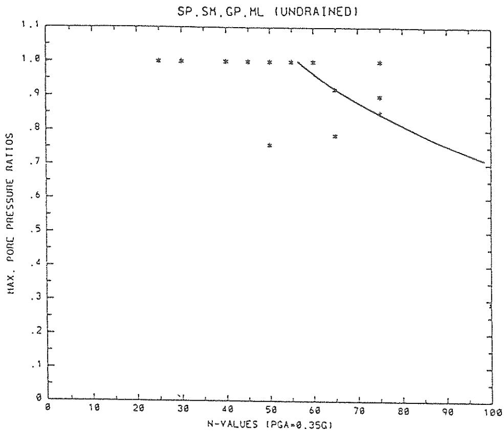
FIGURE A-8 Pore Pressure Ratios vs. In Situ N-Values for
