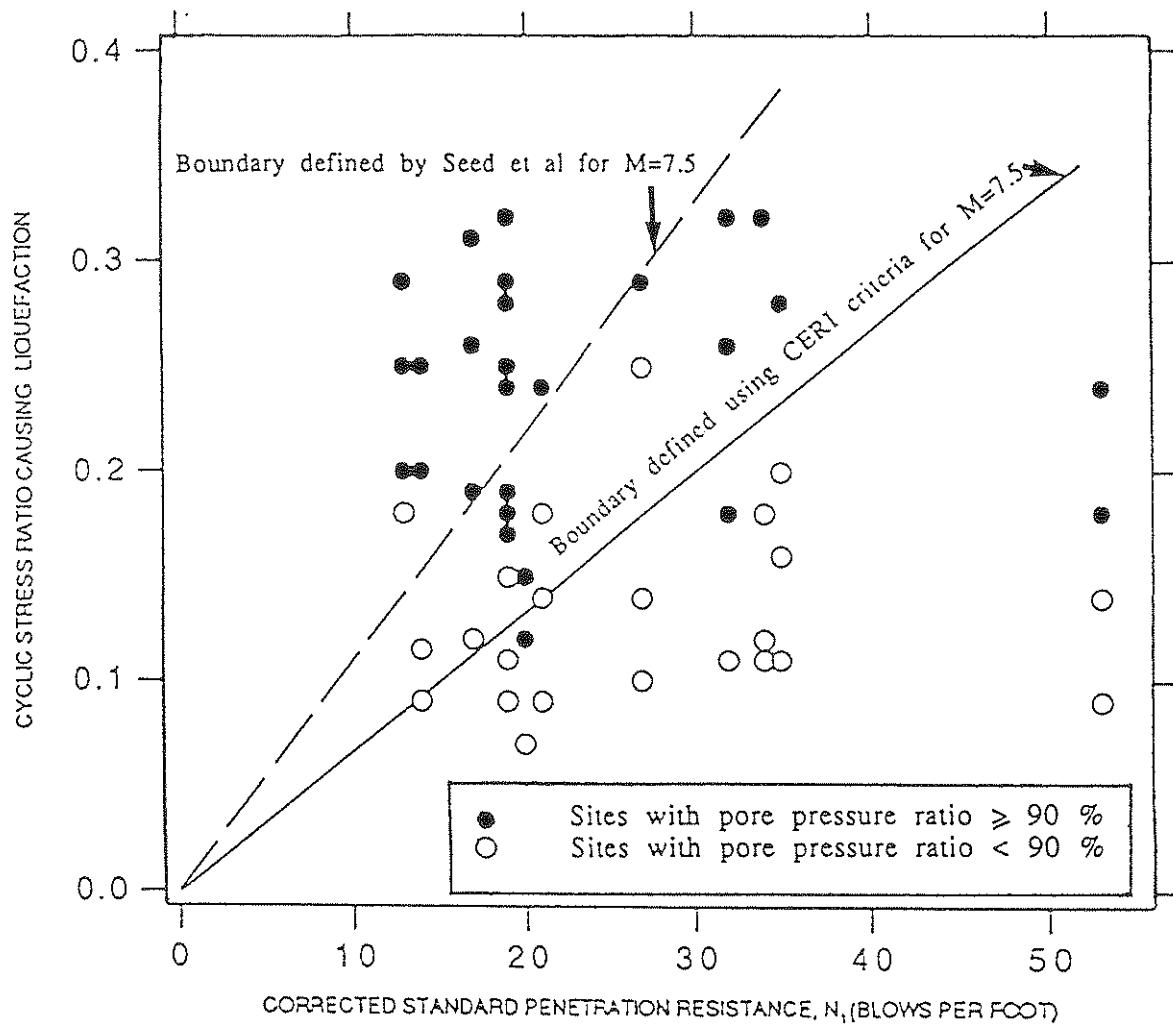
FIGURE 3-14 Comparison between the CERI Liquefaction Correlation and Seed's Field Liquefaction Correlation
