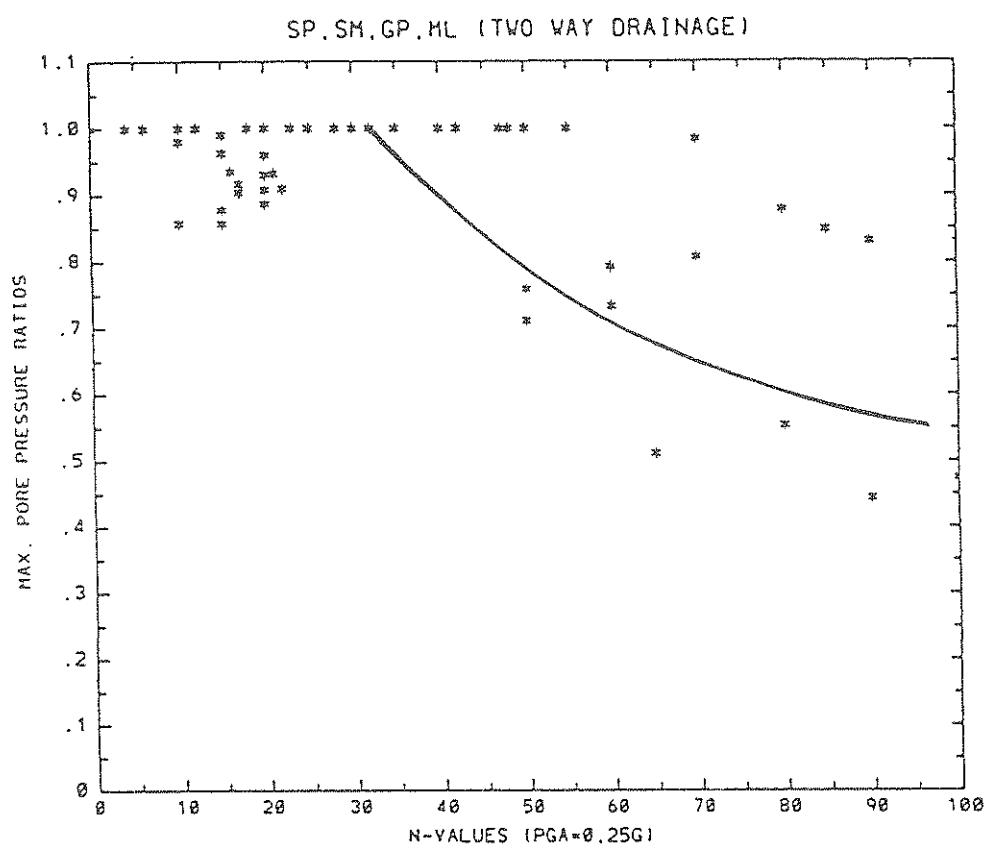
FIGURE A-3 Pore Pressure Ratios vs. In Situ N-Values for
