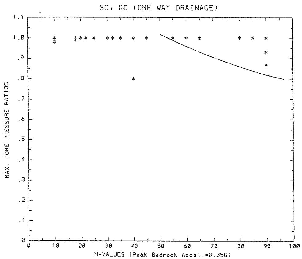
FIGURE 3-4 Pore Pressure Ratios vs. In Situ N-Values for SC-GC
