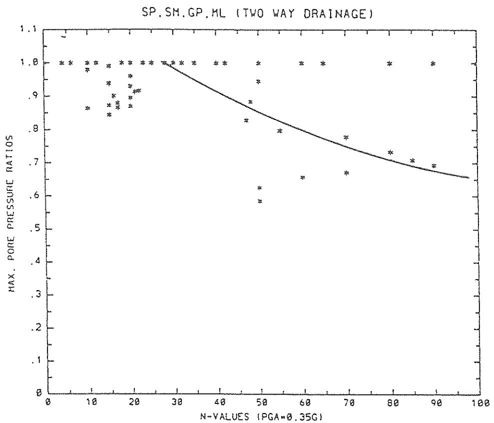
FIGURE A-4 Pore Pressure Ratios vs. In Situ N-Values for
