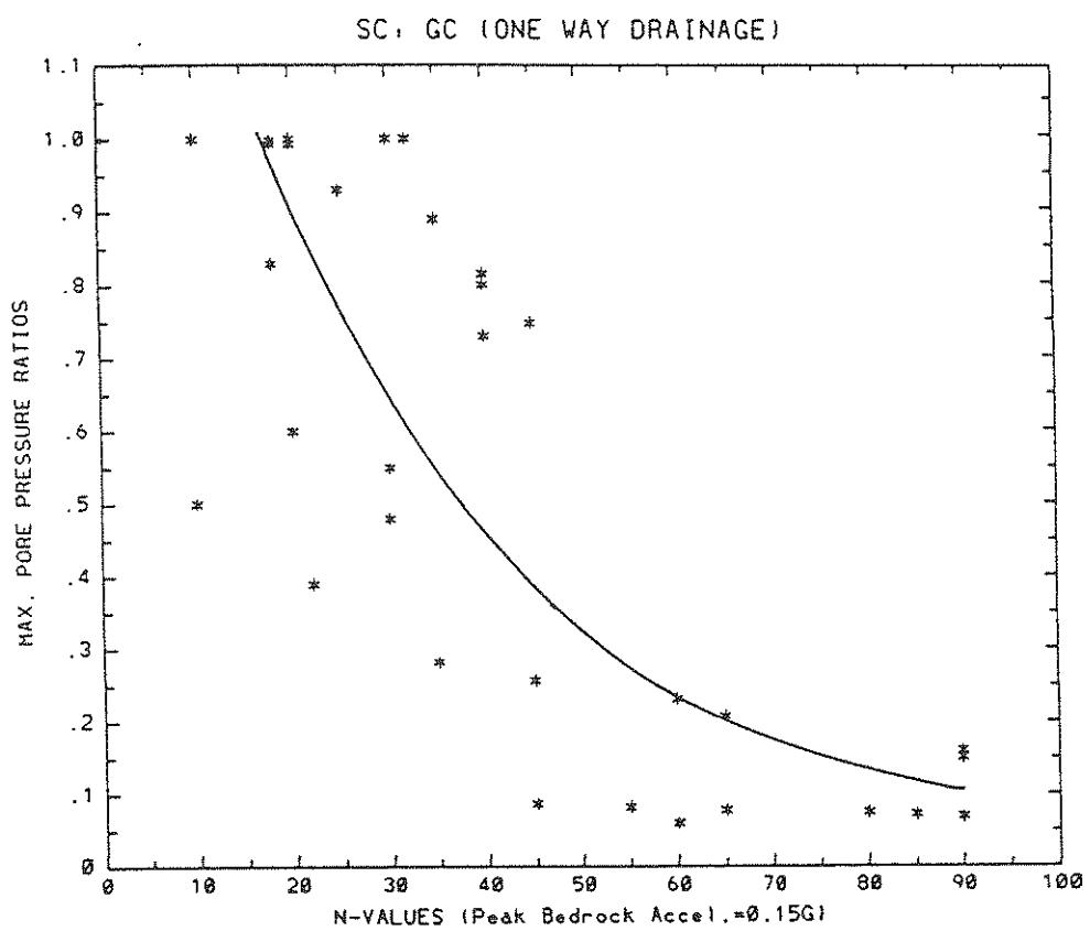
FIGURE 3-2 Pore Pressure Ratios vs. In Situ N-Values for SC-GC
