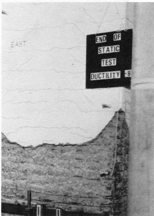
(c) End of quasi-static testing, after 2 cycles at \mu = \pm 8
