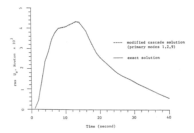
FIGURE 4-4. ROOT-MEAN-SQUARE SHEAR FORCE ACTING AT THE EQUIPMENT-BUILDING INTERFACE: MODIFIED CASCADE VS. EXACT SOLUTION. EQUIPMENT ON 4-TH FLOOR TUNED TO NINTH MODE OF BUILDING. (RIGID SOIL AND VISCOELASTIC CUSHION WITH PARAMETER  $a=66.0 \times 10^{-3} \text{ m}$ ).
