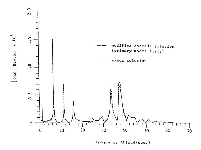
FIGURE 4-5. MODULUS OF FREQUENCY RESPONSE FUNCTION FOR INTERACTIVE FORCE ACTING AT THE EQUIPMENT-BUILDING INTERFACE: MODIFIED CASCADE VS. EXACT SOLUTION. EQUIPMENT ON 4-TH FLOOR "TUNED" TO NINTH MODE OF BUILDING. (COMPLIANT SOIL).
