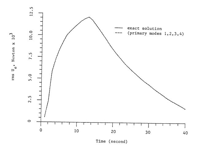
FIGURE 4-12. ROOT-MEAN-SQUARE SHEAR FORCE ACTING AT THE EQUIPMENT-BUILDING INTERFACE: COMPONENT-MODE APPROXIMATION VS. EXACT SOLUTION. EQUIPMENT ON 4-TH FLOOR "DETUNED" MIDWAY BETWEEN 3RD AND 4TH MODES OF BUILDING. (RIGID SOIL AND VISCOELASTIC CUSHION WITH PARAMETER  $a=270 \times 10^{-3} \text{ m}$ , TO EFFECT A FIRST MODE TUNING).
