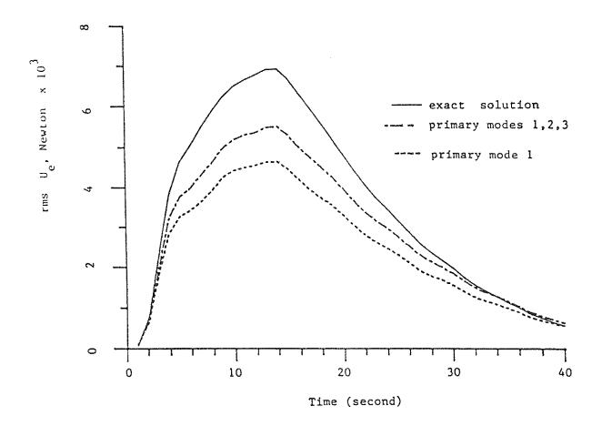
FIGURE 4-8. ROOT-MEAN-SQUARE SHEAR FORCE ACTING AT THE EQUIPMENT-BUILDING INTERFACE: COMPONENT-MODE APPROXIMATION VS. EXACT SOLUTION. EQUIPMENT ON 4-TH FLOOR "TUNED" TO FIRST MODE OF BUILDING. (COMPLIANT SOIL).
