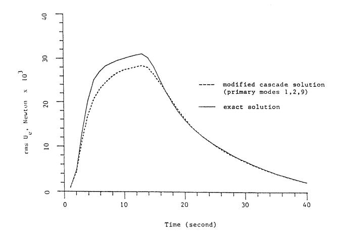
FIGURE 4-6. ROOT-MEAN-SQUARE SHEAR FORCE ACTING AT THE EQUIPMENT-BUILDING INTERFACE: MODIFIED CASCADE VS. EXACT SOLUTION. EQUIPMENT ON 4-TH FLOOR "TUNED" TO NINTH MODE OF BUILDING. (COMPLIANT SOIL).
