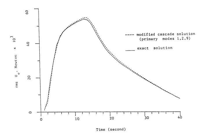
FIGURE 4-2. ROOT-MEAN-SQUARE SHEAR FORCE ACTING AT THE EQUIPMENT-BUILDING INTERFACE: MODIFIED CASCADE VS. EXACT SOLUTION. EQUIPMENT ON 4-TH FLOOR TUNED TO NINTH MODE OF BUILDING. (RIGID SOIL).
