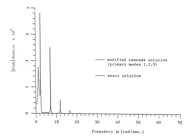
FIGURE 4-3. MODULUS OF FREQUENCY RESPONSE FUNCTION FOR INTERACTIVE FORCE ACTING AT THE EQUIPMENT-BUILDING INTERFACE: MODIFIED CASCADE VS. EXACT SOLUTION. EQUIPMENT ON 4-TH FLOOR TUNED TO NINTH MODE OF BUILDING. (RIGID SOIL AND VISCOELASTIC CUSHION WITH PARAMETER a=66.0 x  $10^{-3}$  m).
