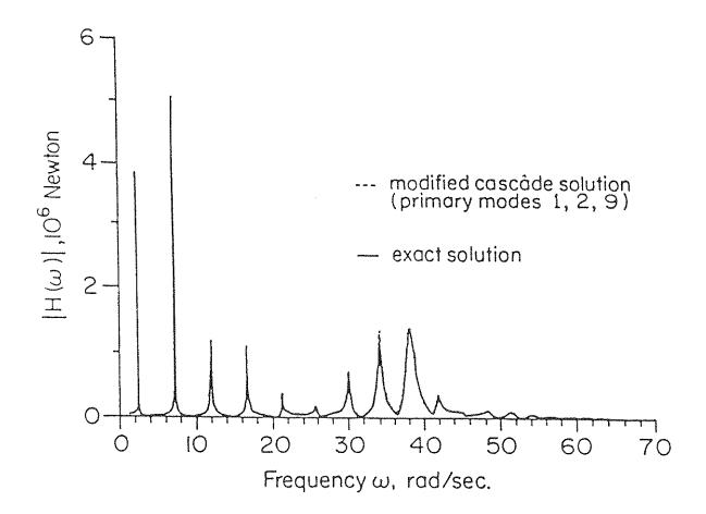
FIGURE 4-1. MODULUS OF FREQUENCY RESPONSE FUNCTION FOR INTERACTIVE FORCE ACTING AT THE EQUIPMENT-BUILDING INTERFACE: MODIFIED CASCADE VS. EXACT SOLUTION. EQUIPMENT ON 4-TH FLOOR TUNED TO NINTH MODE OF BUILDING. (RIGID SOIL).
