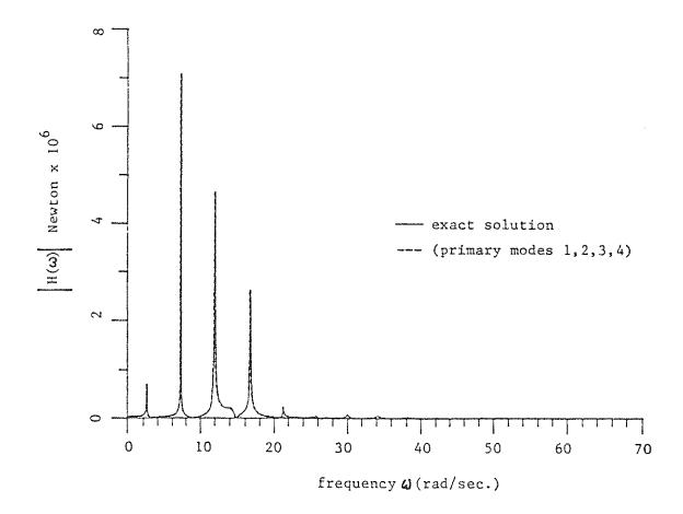
FIGURE 4-9. MODULUS OF FREQUENCY RESPONSE FUNCTION FOR INTERACTIVE FORCE ACTING AT THE EQUIPMENT-BUILDING INTERFACE: COMPONENT-MODE APPROXIMATION VS. EXACT SOLUTION. EQUIPMENT ON 4-TH FLOOR "DETUNED" MID-WAY BETWEEN 3RD AND 4TH MODES OF BUILDING. (RIGID SOIL).
