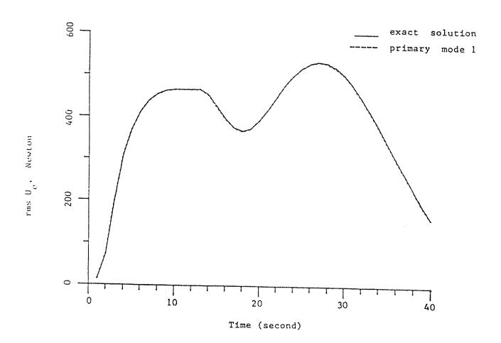
FIGURE 4-7. ROOT-MEAN-SQUARE SHEAR FORCE ACTING AT THE EQUIPMENT-BUILDING INTERFACE: COMPONENT-MODE APPROXIMATION VS. EXACT SOLUTION. EQUIPMENT ON 4-TH FLOOR TUNED TO FIRST MODE OF BUILDING. (RIGID SOIL AND VISCOELASTIC CUSHION WITH PARAMETER  $a=66.0 \times 10^{-3} \, \text{m}$ ).
