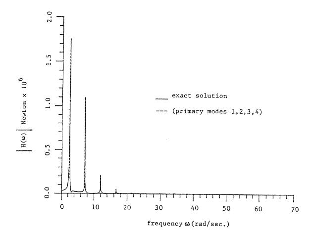
FIGURE 4-11. MODULUS OF FREQUENCY RESPONSE FUNCTION FOR INTERACTIVE FORCE ACTING AT THE EQUIPMENT-BUILDING INTERFACE: COMPONENT-MODE APPROXIMATION VS. EXACT SOLUTION. EQUIPMENT ON 4-TH FLOOR "DETUNED" MID-WAY BETWEEN 3RD AND 4TH MODES OF BUILDING. (RIGID SOIL AND VISCOELASTIC CUSHION WITH PARAMETER  $a=270 \times 10^{-3}$  m, TO EFFECT A FIRST MODE TUNING).
