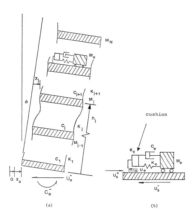
FIGURE 2-1. STRUCTURAL MODEL: (a) N+3 DEGREE-OF-FREEDOM COMBINED P-S SYSTEM, (b) FORCES ON THE S-TH FLOOR.
