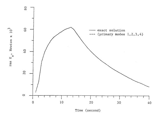
FIGURE 4-10. ROOT-MEAN-SQUARE SHEAR FORCE ACTING AT THE EQUIPMENT-BUILDING INTERFACE: COMPONENT-MODE APPROXIMATION VS. EXACT SOLUTION. EQUIPMENT ON 4-TH FLOOR "DETUNED" MIDWAY BETWEEN 3RD AND 4TH MODES OF BUILDING. (RIGID SOIL).
