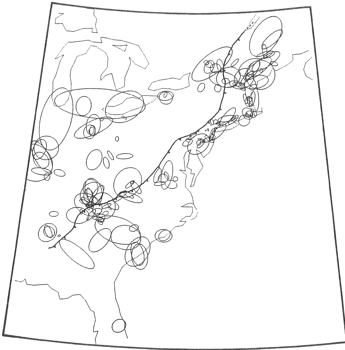
Figure 6. Seismicity (1928-1981) in the eastern U.S. from the NOAA Earthquake Effect File of intensity data (revised by the authors); only events with at least 10 intensity points are shown. The ellipses are isoseismal contours from MACRO solutions of these events where the model is an elliptical conoid (vertical axis = intensity; horizontal axes = space) with a linear slope. Each event is represented by the contour for the intensity level one unit below the conoid maximum intensity. The long axes of the isoseismals tend to be aligned with structural trends along the Appalachians, suggesting a structurally controlled attenuation anisotropy. The size of the ellipses is inversely proportional to the rate of intensity fall-off. This rate tends to scatter; nevertheless, regional patterns are detected.
