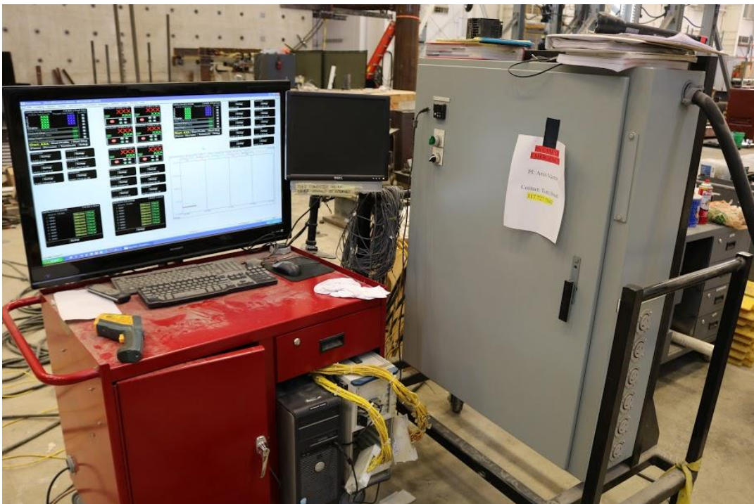
Figure 3-14. Heating control system and display
