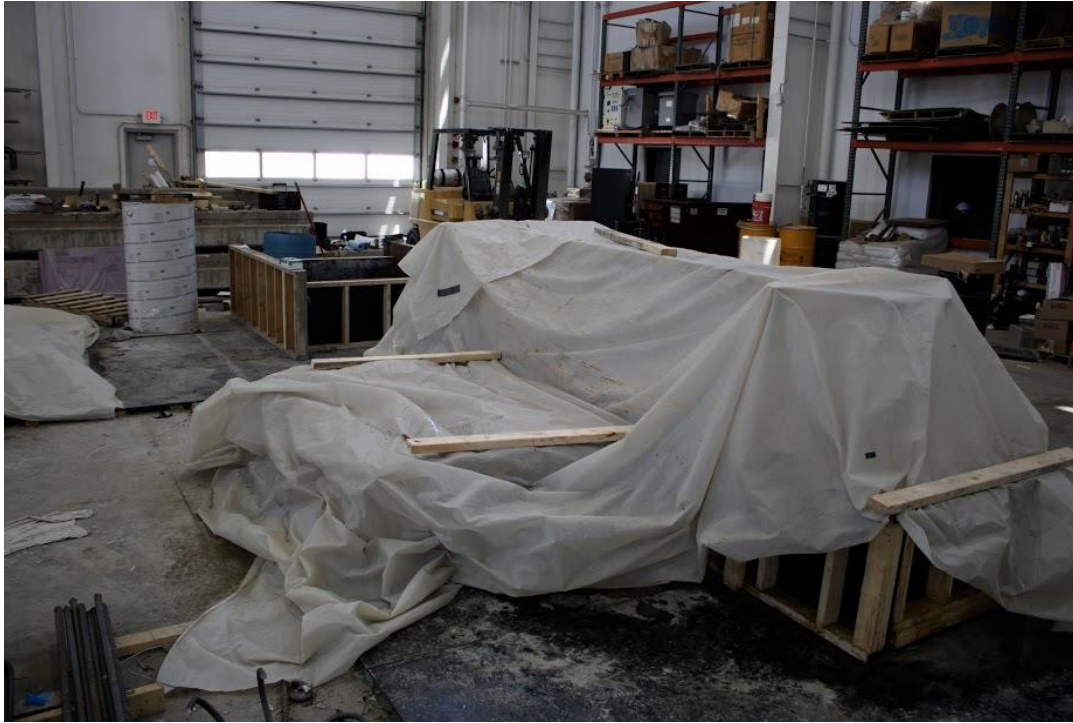
Figure 3-11. Polythene cover placed over specimen for curing period
