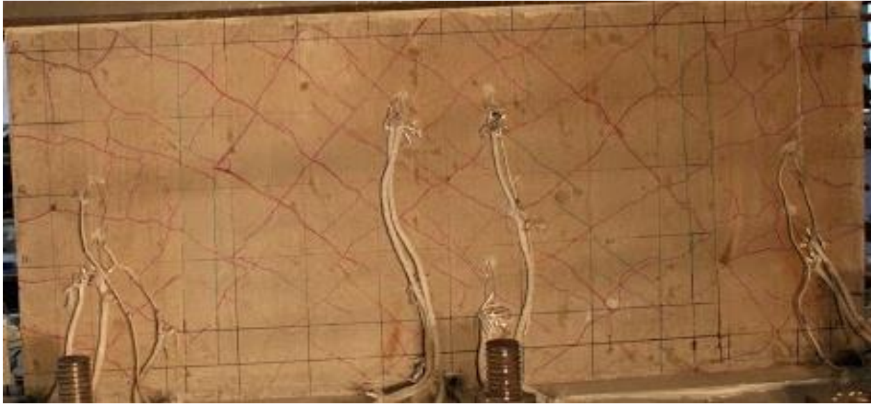
Figure 4-13. Crack pattern on West face of Wall 2 after LC14
