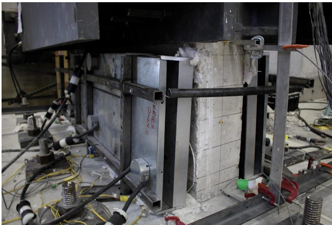
Figure 3-16. Heaters installed on wall specimen
