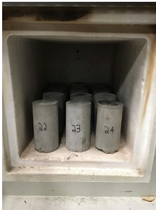
Figure 5-3. Cylinders in the furnace
