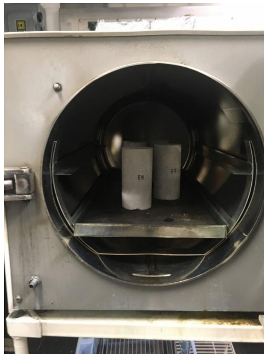
Figure 6-3. Placement of concrete cylinders in the autoclave
