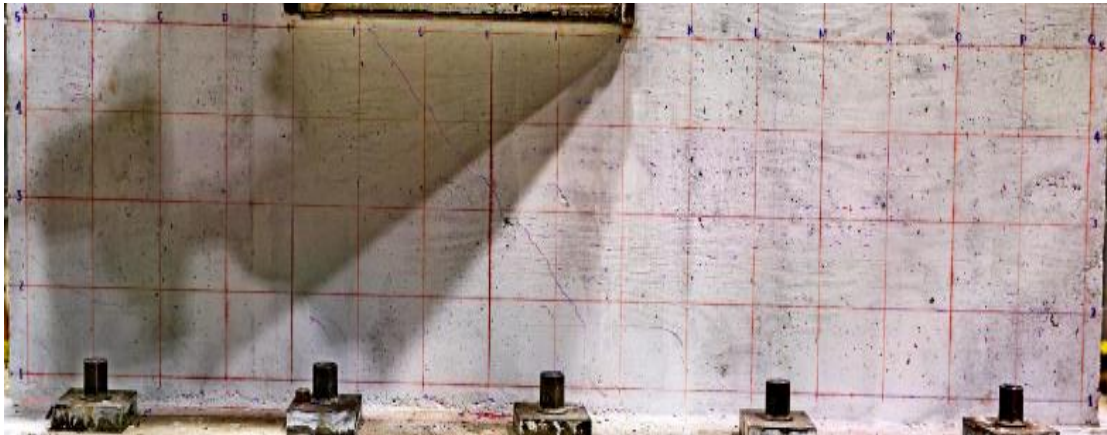
Figure 4-37. Onset of visible cracks, SW7, after LS3 (peak transient drift ratio of 0.08%)
