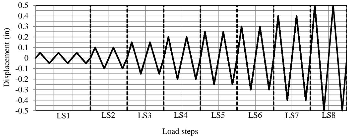
Figure D.4. Loading protocol for SW2
