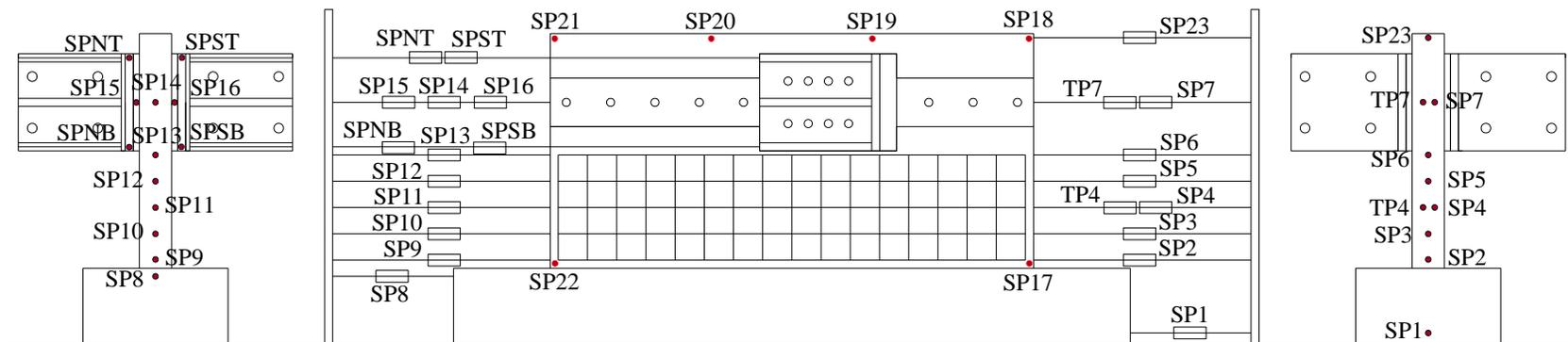
Figure C.41. In-plane and out-of-plane string potentiometers and Temposonics for SW5
