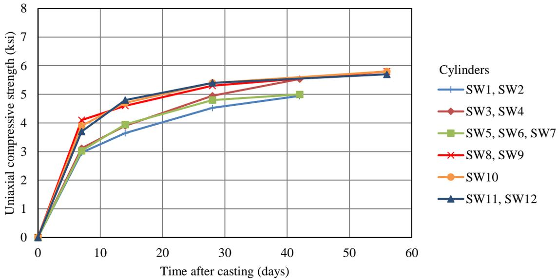
Figure 3.17. Concrete compressive strength from cylinder tests: foundations
