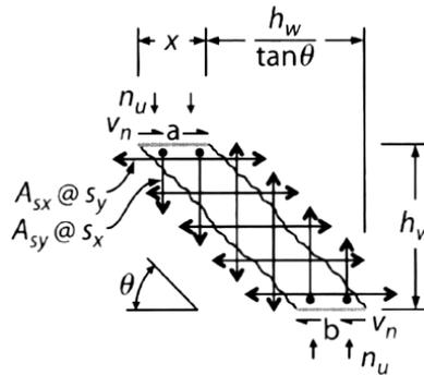
b) Free-body diagram of compression strut a-b
