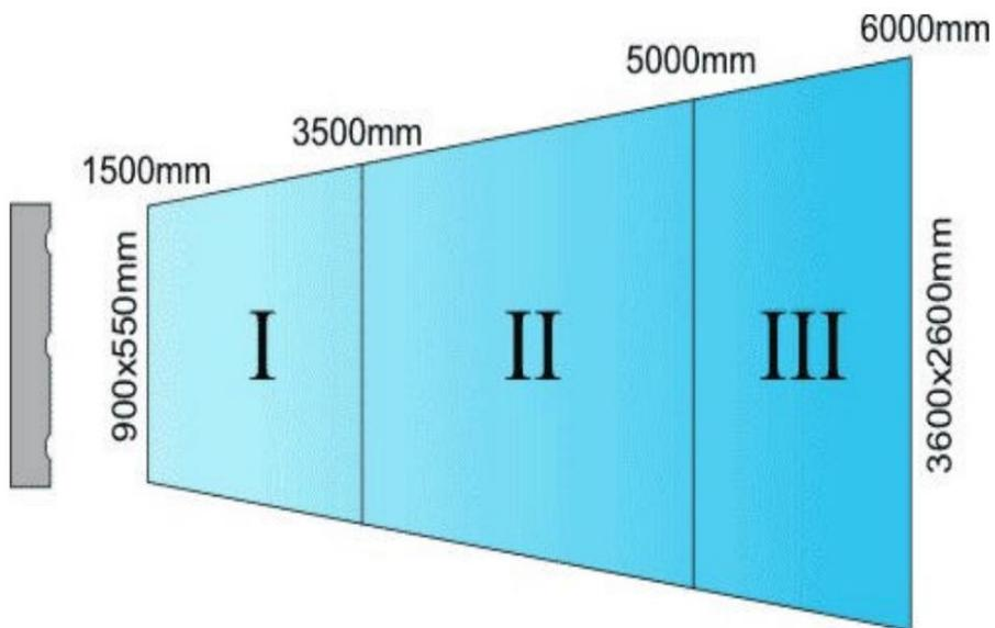
Figure C.55. Krypton K600 camera field of view
