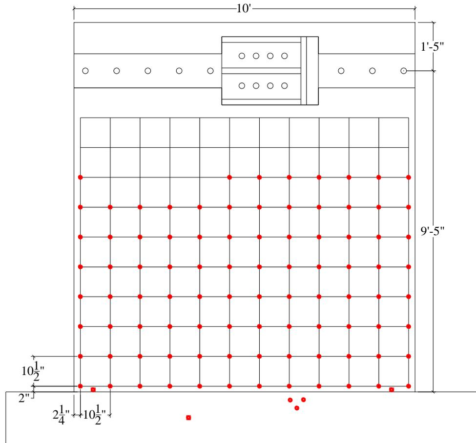
Figure C.1. Krypton LED sensors for SW1
