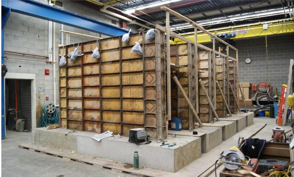
Figure 3.14. Phase II specimens prior to pouring of concrete on the walls
