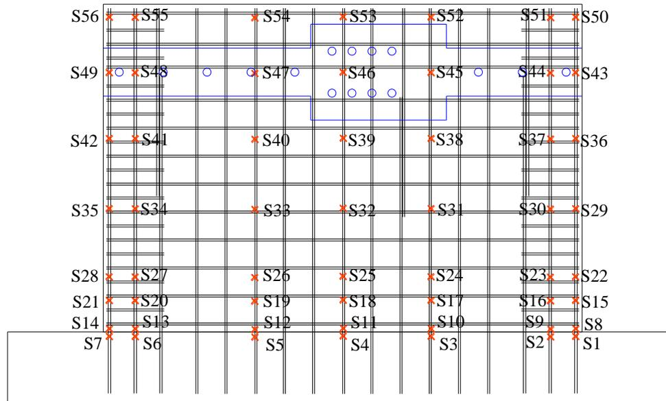
Figure C.23. Strain gages on the vertical reinforcements for SW11
