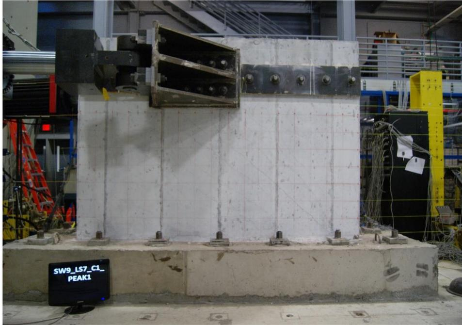
Figure E.73. Damage to SW9 at 0.76% drift ratio
