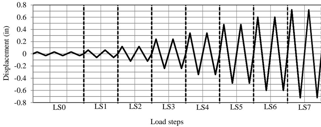
Figure D.24. Loading protocol for SW12
