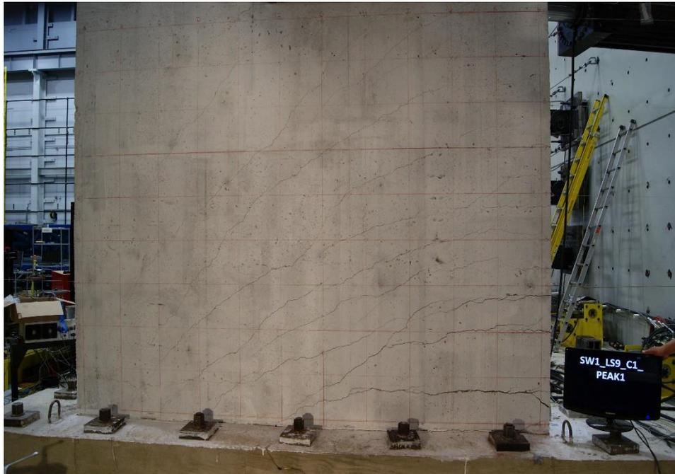
Figure E.4. Damage to SW1 at 1.30% drift ratio (peak strength)
