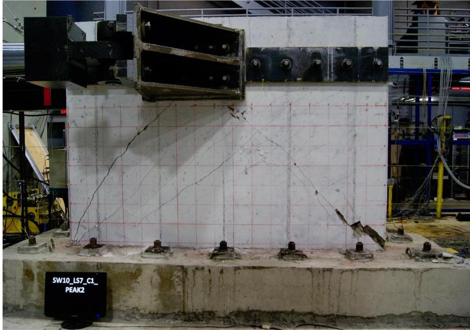
Figure E.86. Damage to SW10 at -0.87% drift ratio
