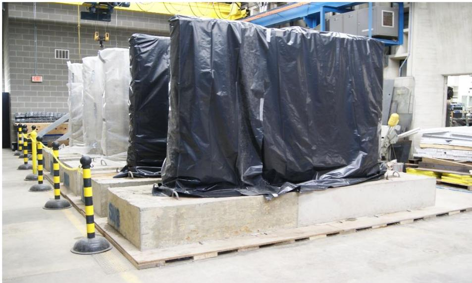
Figure 3.15. Curing of Phase II wall specimens
