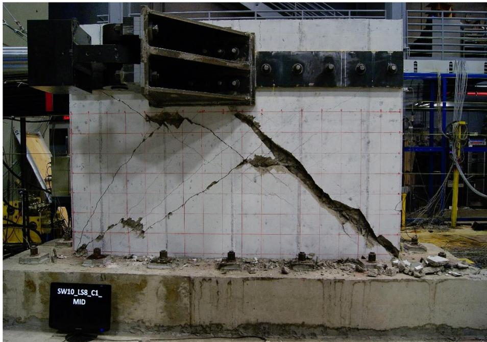
Figure 2.2. Diagonal tension failure
