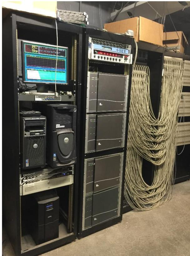
Figure C.59. Pacific Instruments model 6000 data acquisition system
