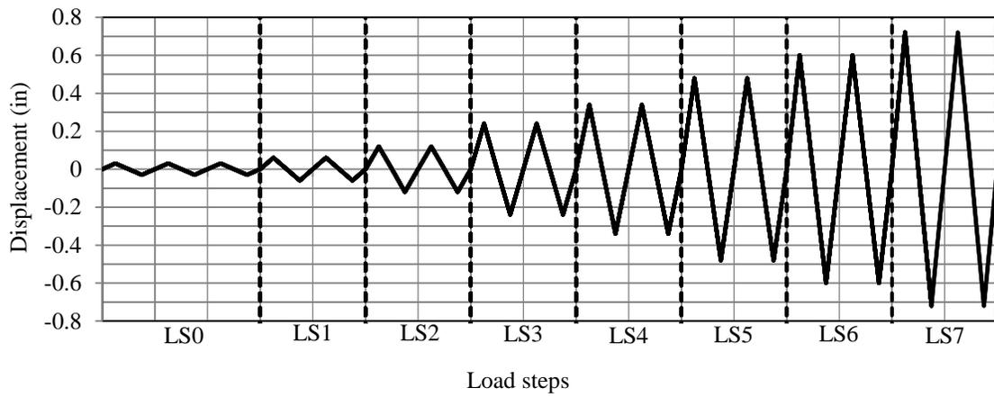
Figure D.22. Loading protocol for SW11
