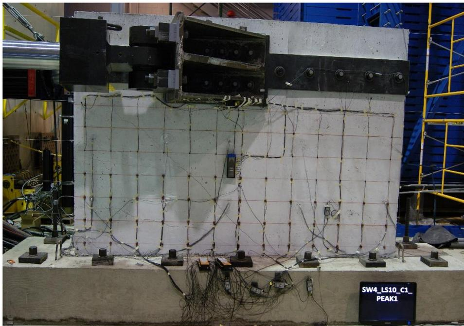
Figure E.27. Damage to SW4 at 0.60% drift ratio
