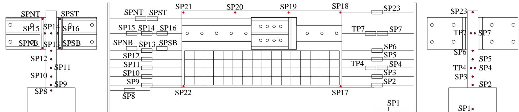
Figure C.43. In-plane and out-of-plane string potentiometers and Temposonics for SW7
