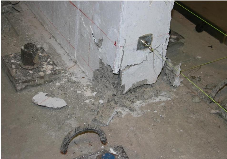
Figure 0.1. Damage to SW8 at -0.86% drift ratio
