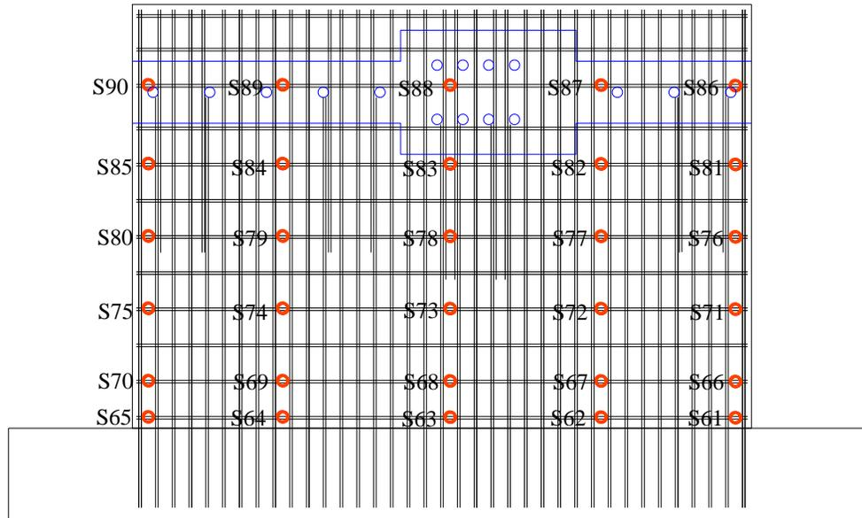
Figure C.33. Strain gages on the horizontal reinforcements for SW9
