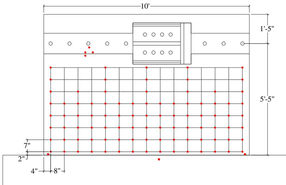
Figure C.2. Krypton LED sensors for SW2
