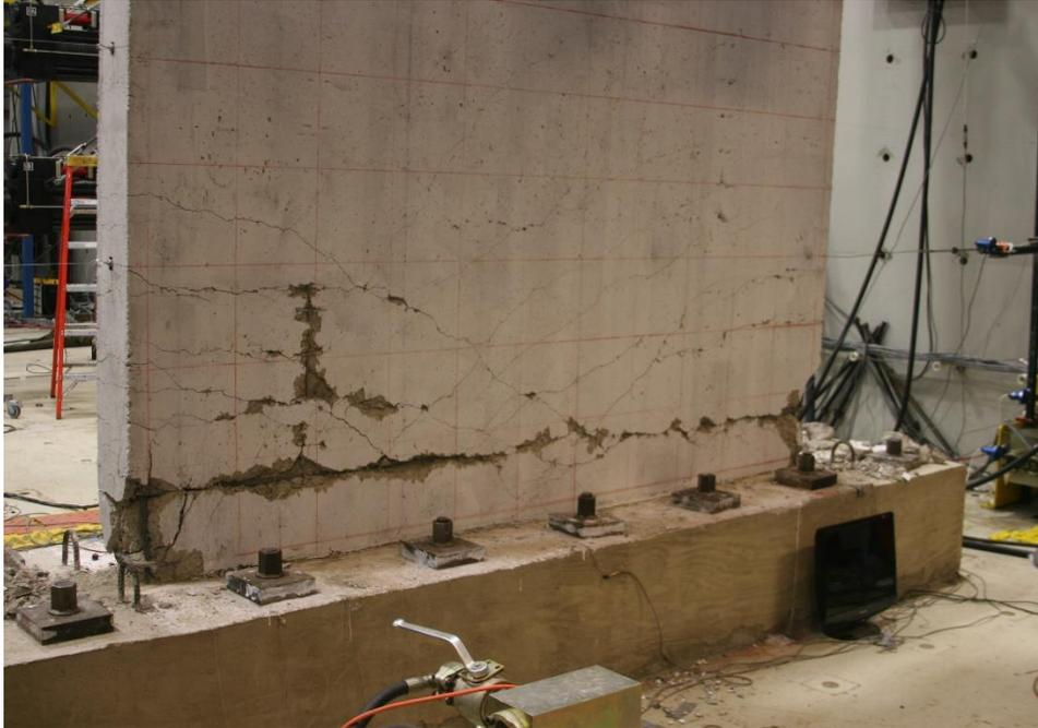
Figure E.8. Damage to SW1 at the end of testing
