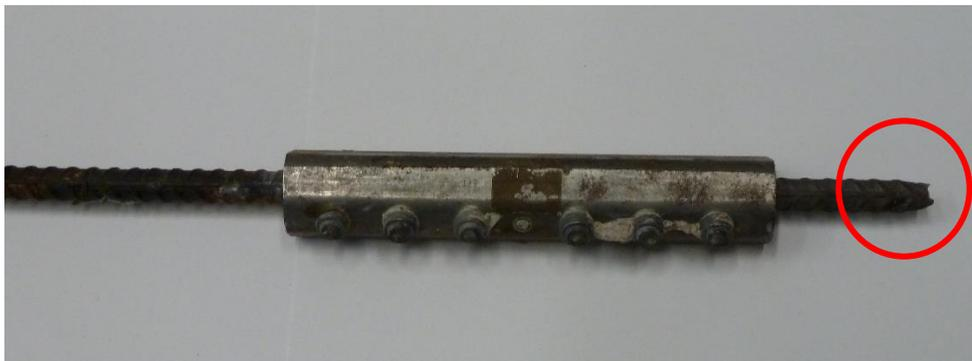
Figure 3.18. Rupture zone in the Type-2 mechanical coupler tensile test
