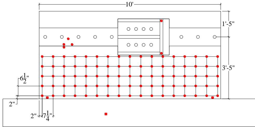
Figure C.7. Krypton LED sensors for SW7
