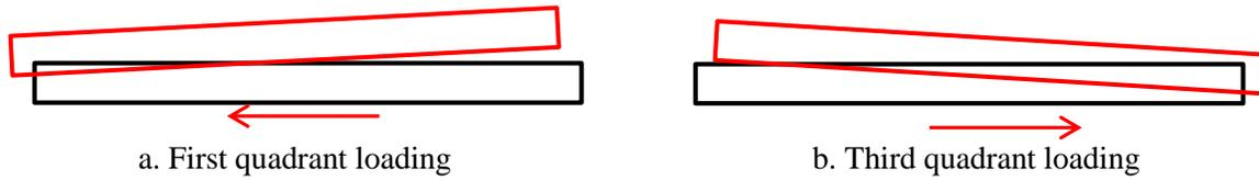
Figure 6.2. Typical out-of-plane displacement and twisting of the walls at peak strength
