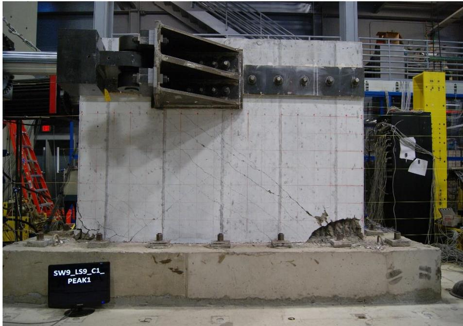
Figure E.75. Damage to SW9 at 1.72% drift ratio
