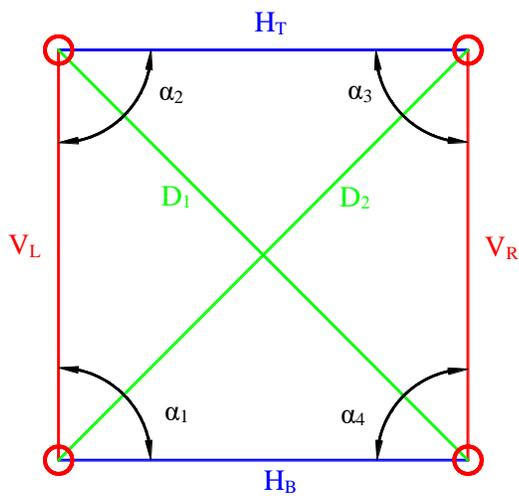
Figure 4.12. Notation for the quadrilateral panel used to calculate strain fields
