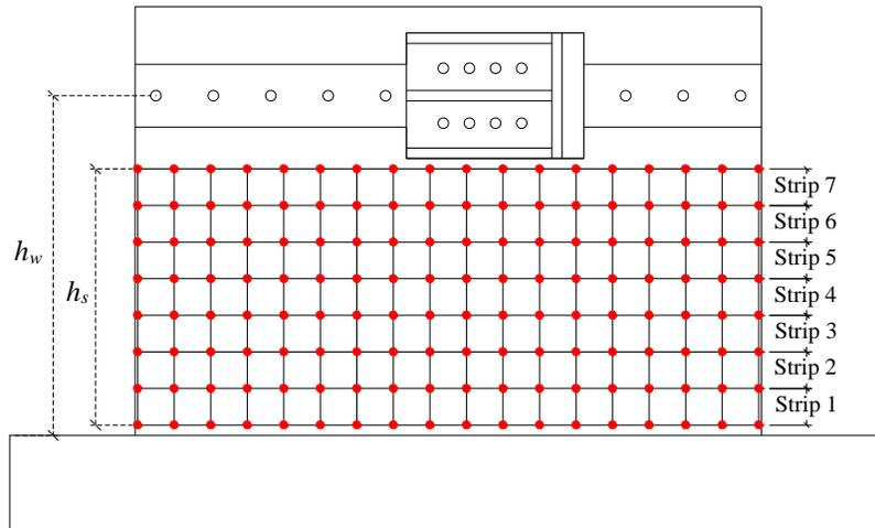
Figure 4.22. Typical grid of Krypton LED sensors
