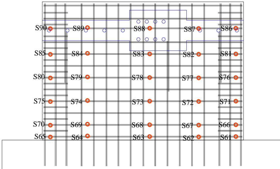
Figure C.35. Strain gages on the horizontal reinforcements for SW11
