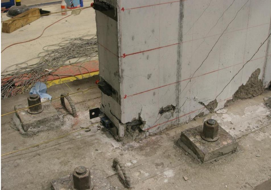
Figure E.109. Damage to SW12 at the end of testing
