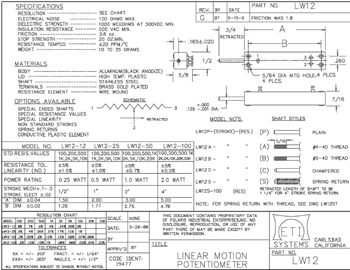
Figure C.54. LW12 linear potentiometer data sheet
