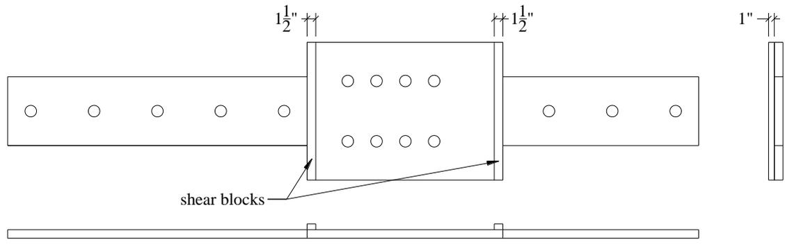
Figure A.20. Loading plate with the additional shear blocks
