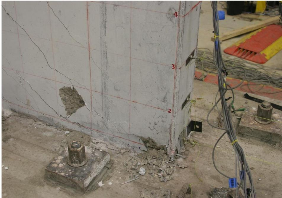
Figure 0.2. Damage to SW12 at -1.64% drift ratio
