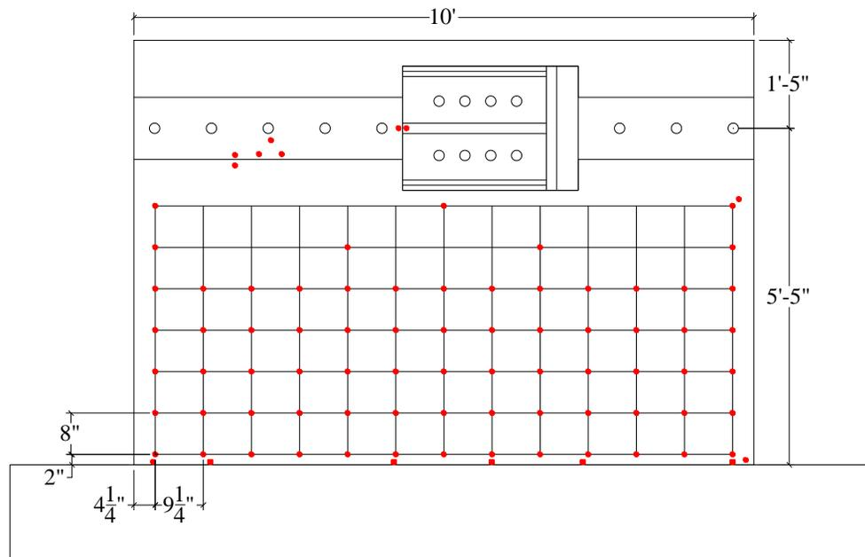
Figure C.4. Krypton LED sensors for SW4
