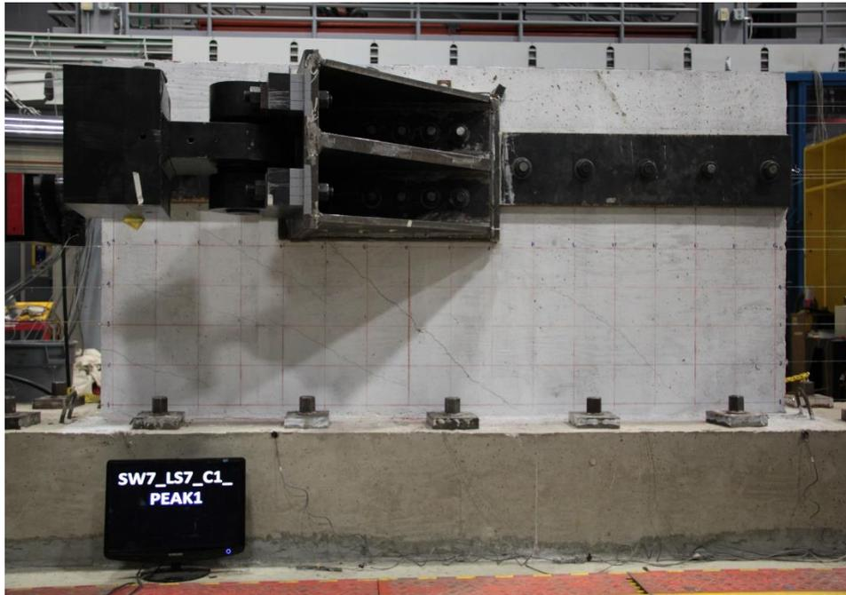
Figure E.51. Damage to SW7 at 0.45% drift ratio (peak strength)
