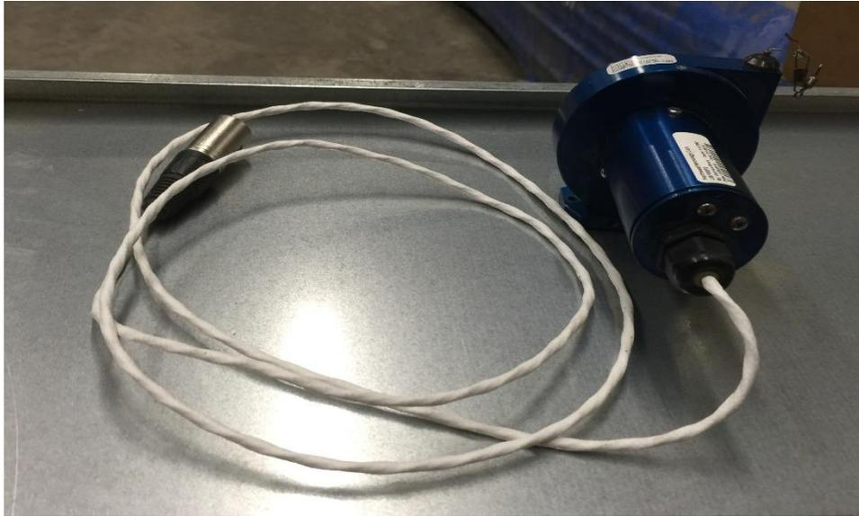
Figure C.51. Series D62 string potentiometer
