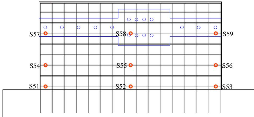
Figure C.30. Strain gages on the horizontal reinforcements for SW6
