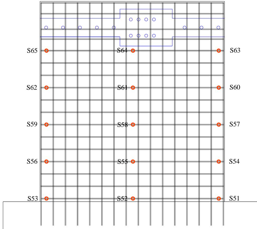
Figure C.25. Strain gages on the horizontal reinforcements for SW1
