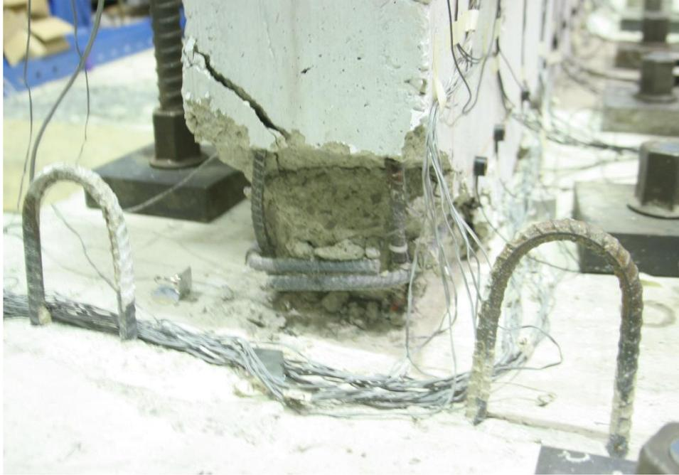
Figure E.34. Damage to SW4 at the end of testing
