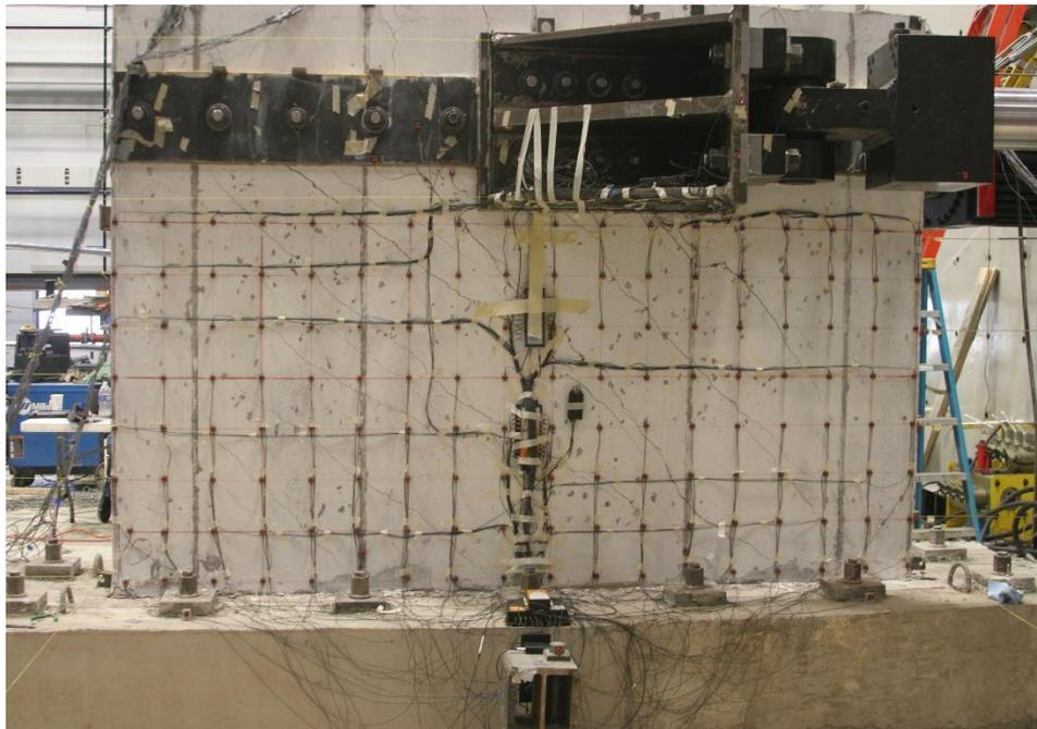
Figure E.104. Damage to SW12 at 1.63% drift ratio
