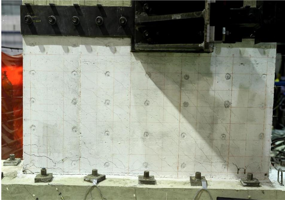
Figure E.14. Damage to SW2 at -1.28% drift ratio
