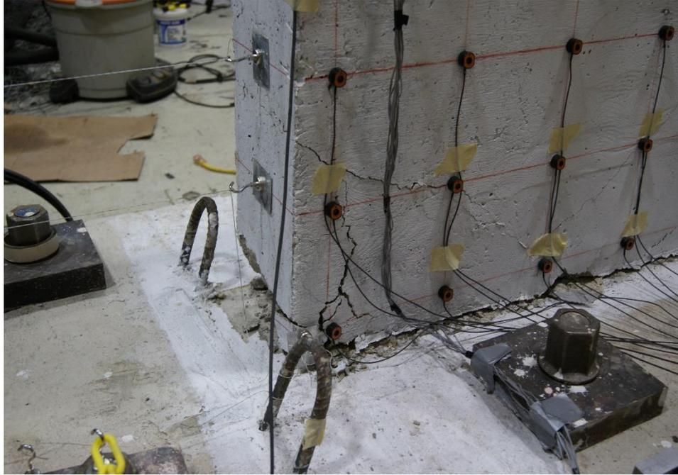
Figure E.57. Damage to SW7 at the end of testing
