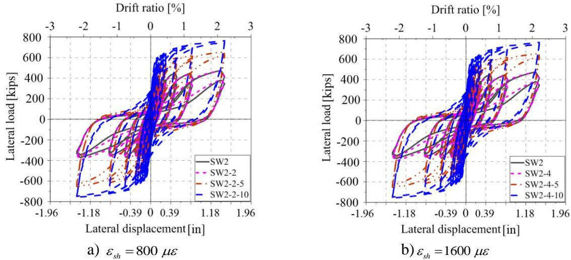
Figure 5.4. Cyclic force-displacement relationships of RC walls
