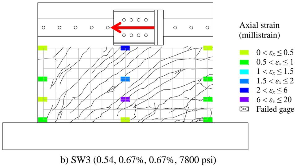
Figure 4.11. Strains on horizontal reinforcement of SW2 and SW3 at 0.7% drift ratio
