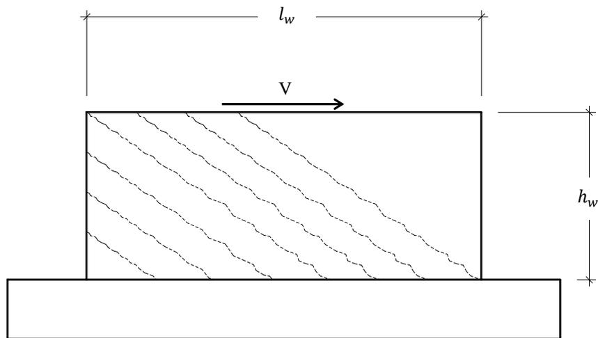
Figure 6.4. Observed cracking pattern (idealized) of a rectangular low aspect ratio RC wall without boundary elements
