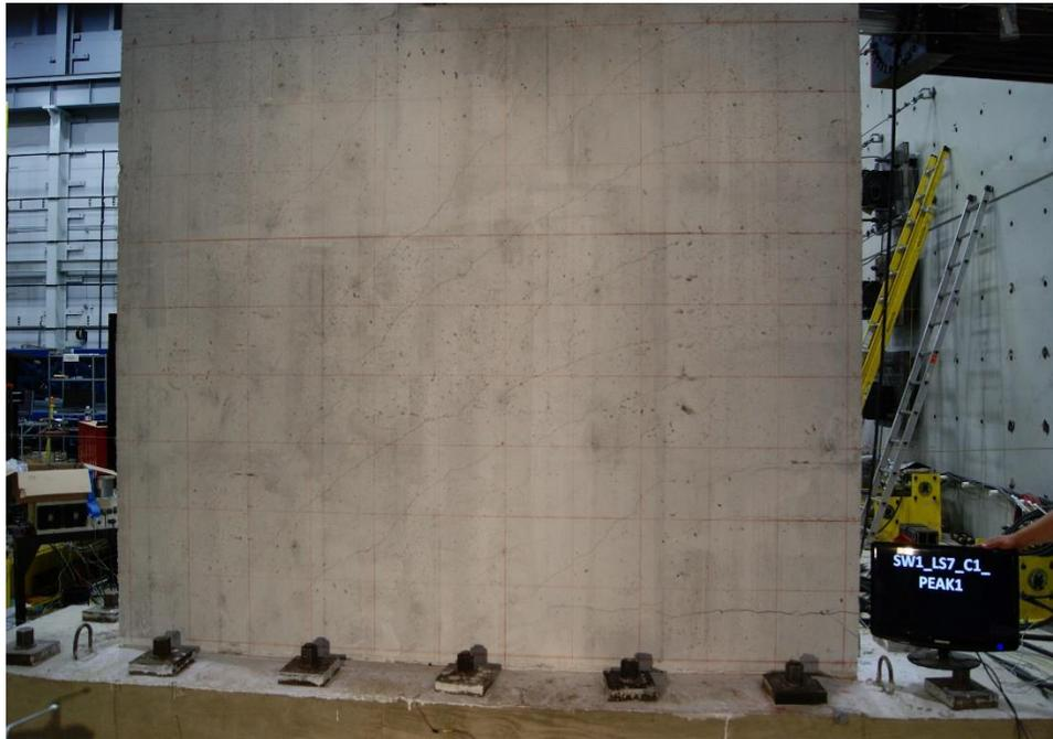
Figure E.2. Damage to SW1 at 0.62% drift ratio
