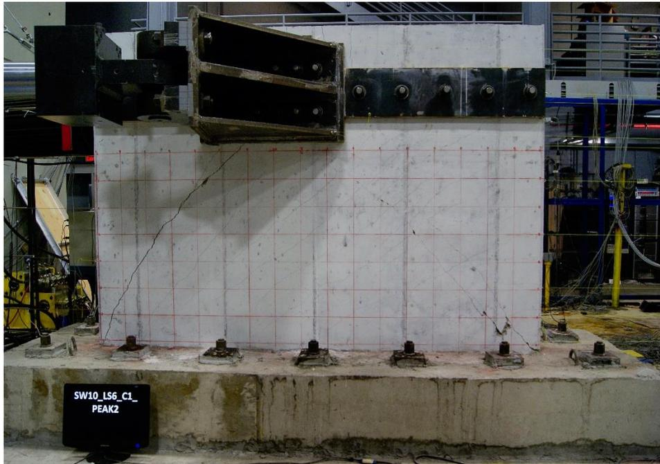
Figure E.84. Damage to SW10 at -0.58% drift ratio (peak strength)
