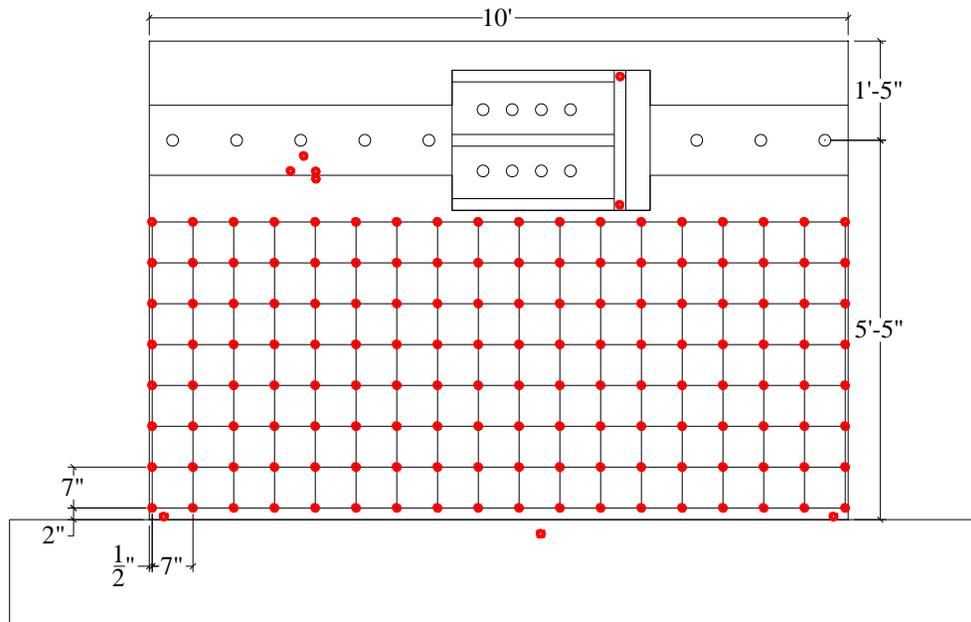
Figure C.11. Krypton LED sensors for SW11
