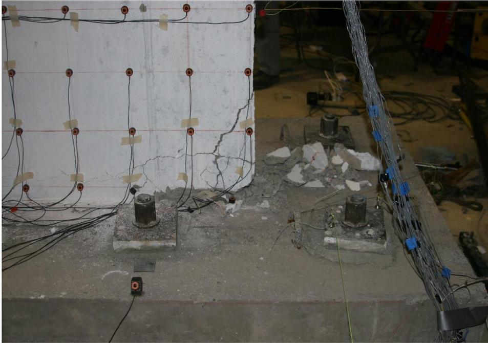
Figure E.69. Damage to SW8 following two cycles to 1.3% drift ratio
