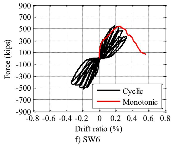
Figure 3.1. VecTor2 predicted force-displacement relationships
