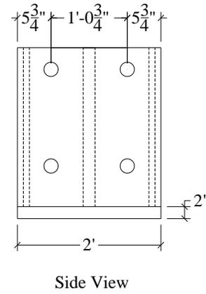
Figure A.21. Loading bracket details
