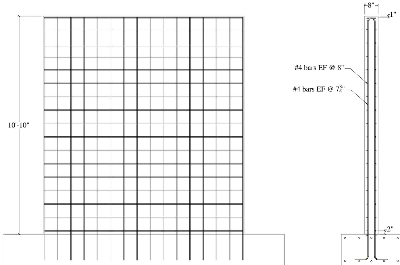
Figure A.7. Reinforcement details for SW1
