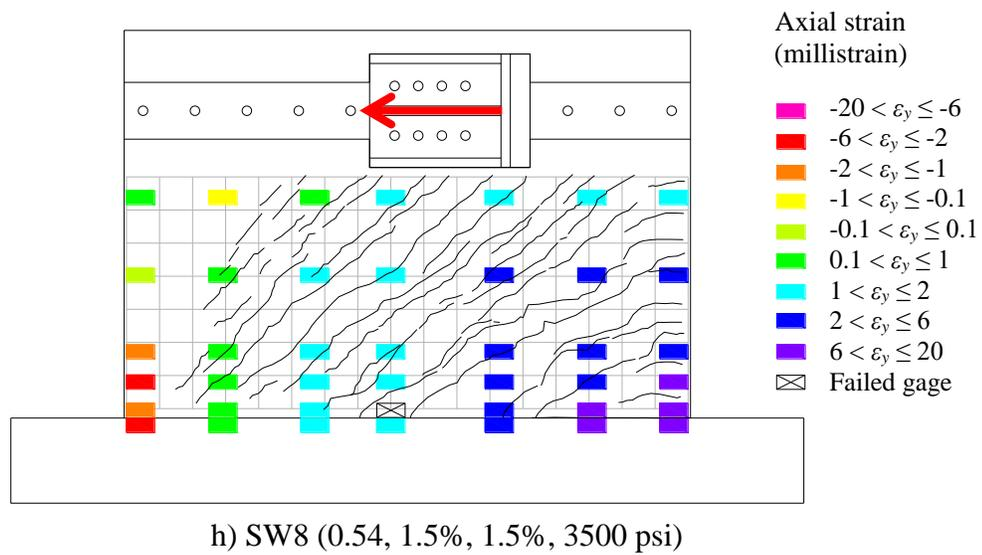
Figure 4.8. Strains on vertical reinforcement at peak strength (continued)
