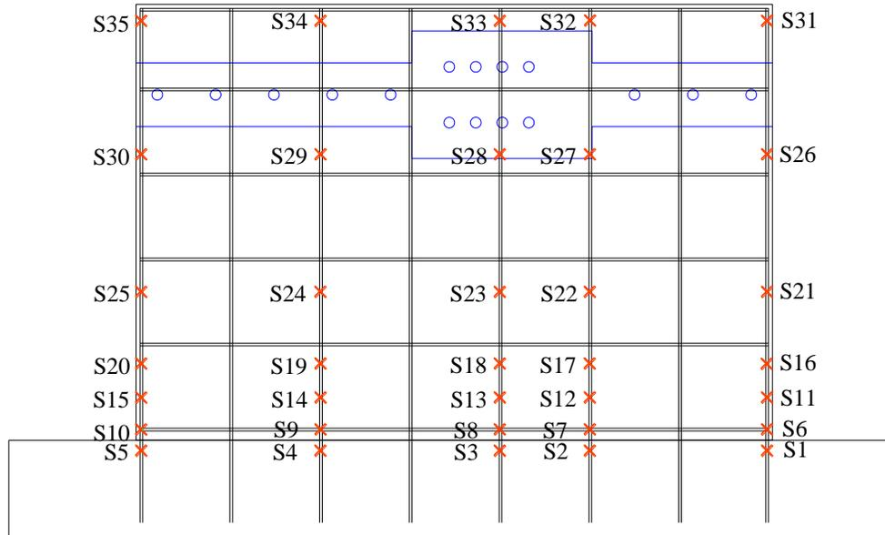
Figure C.16. Strain gages on the vertical reinforcements for SW4
