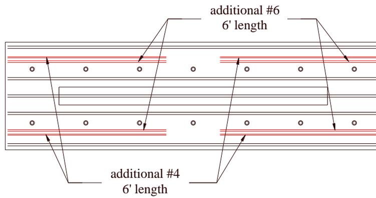
Figure B.5. Supplemental longitudinal reinforcement on the top section of rebar cage (SW8)
