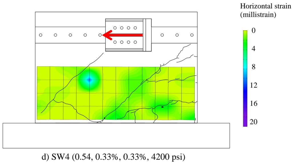
Figure 4.14. Horizontal strain fields at peak strength (continued)
