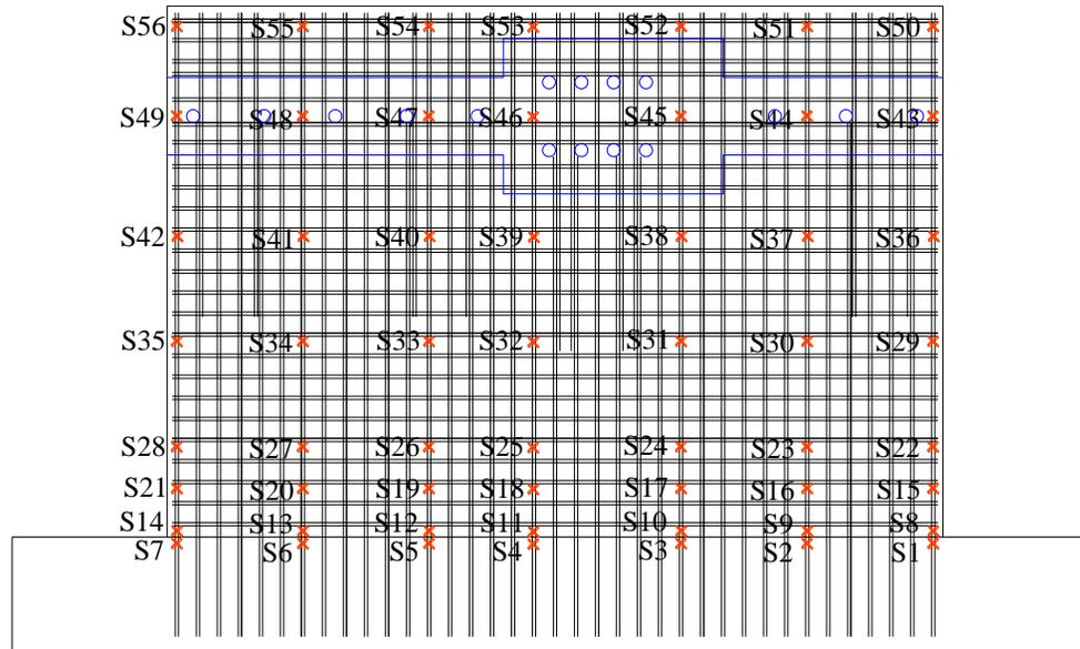
Figure C.20. Strain gages on the vertical reinforcements for SW8
