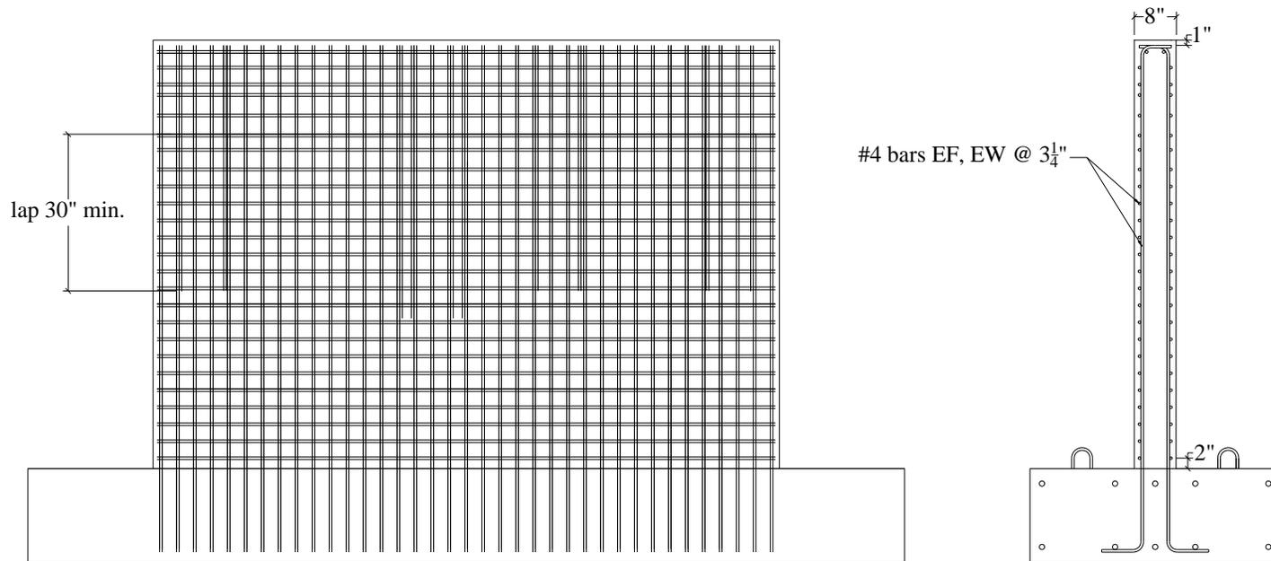
Figure A.14. Reinforcement details for SW8
