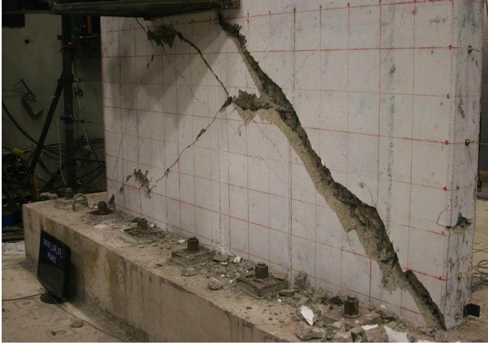
Figure E.90. Damage to SW10 at the end of testing
