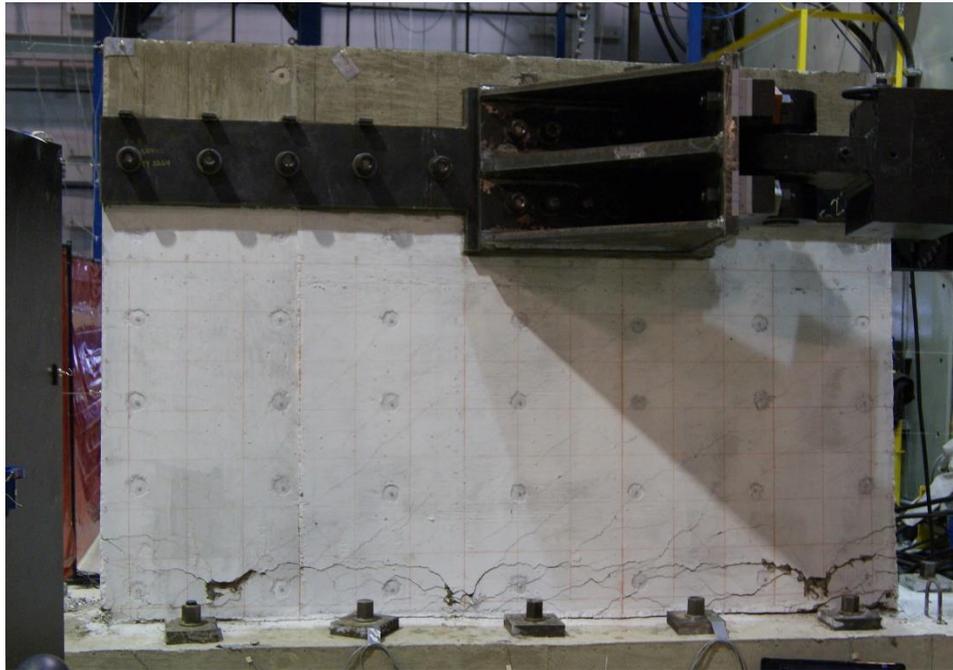
Figure E.15. Damage to SW2 at the end of testing
