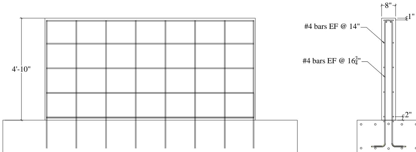
Figure A.13. Reinforcement details for SW7
