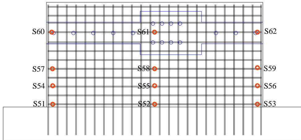
Figure C.29. Strain gages on the horizontal reinforcements for SW5
