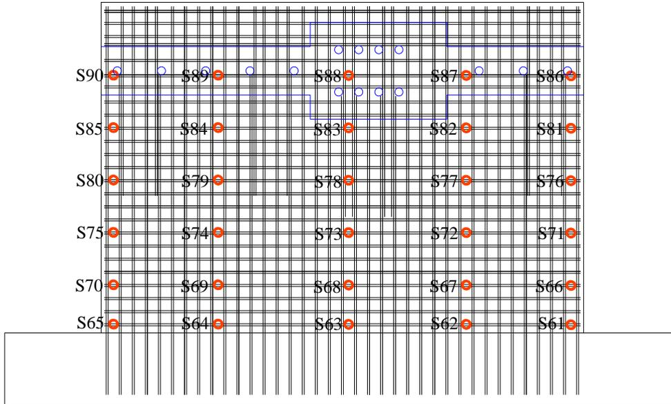
Figure C.32. Strain gages on the horizontal reinforcements for SW8
