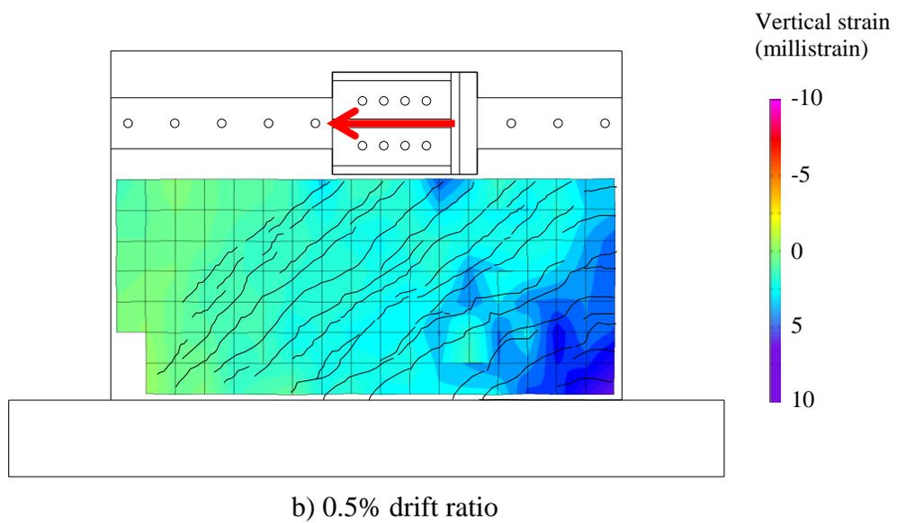
Figure 4.16. Vertical strain fields on SW8 calculated from Krypton LED sensors
