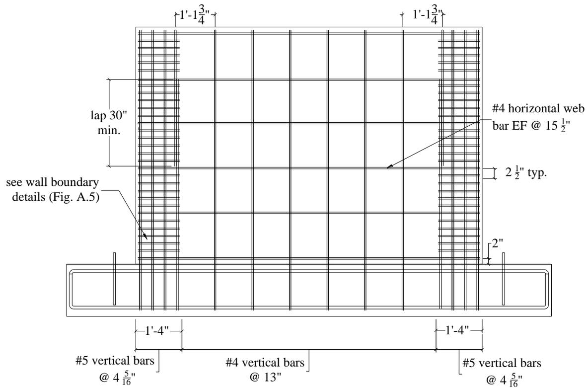
Figure A.18. Reinforcement details for SW12
