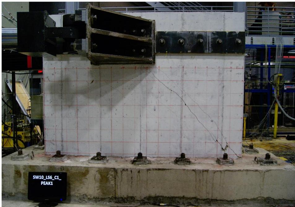
Figure E.83. Damage to SW1 at 0.52% drift ratio
