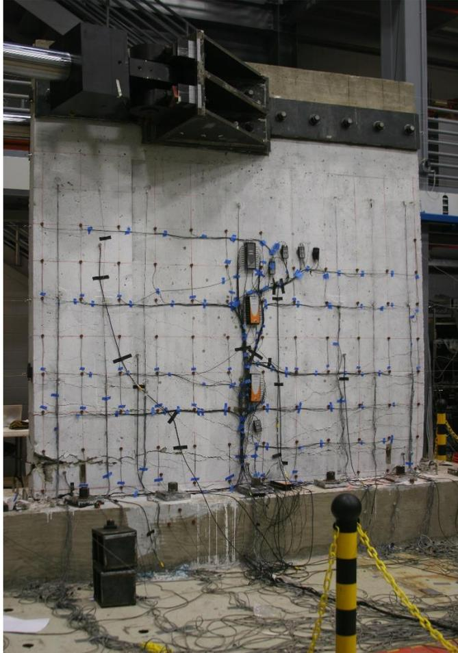
Figure E.7. Damage to SW1 at the end of testing
