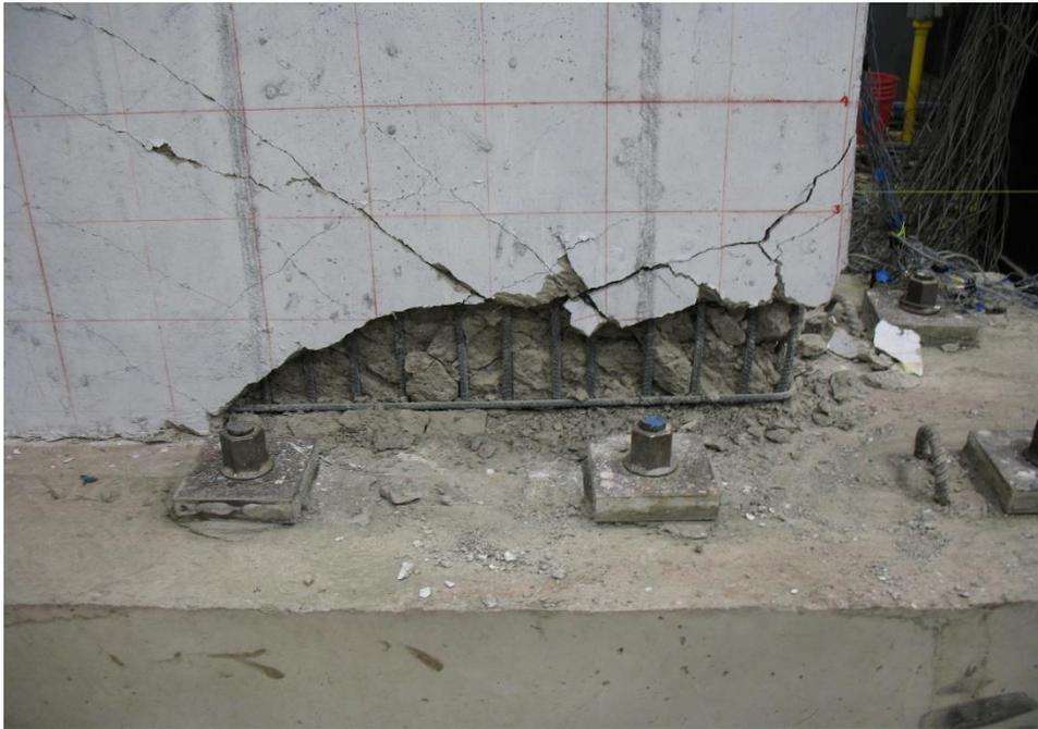
Figure E.78. Damage to SW9 at the end of testing
