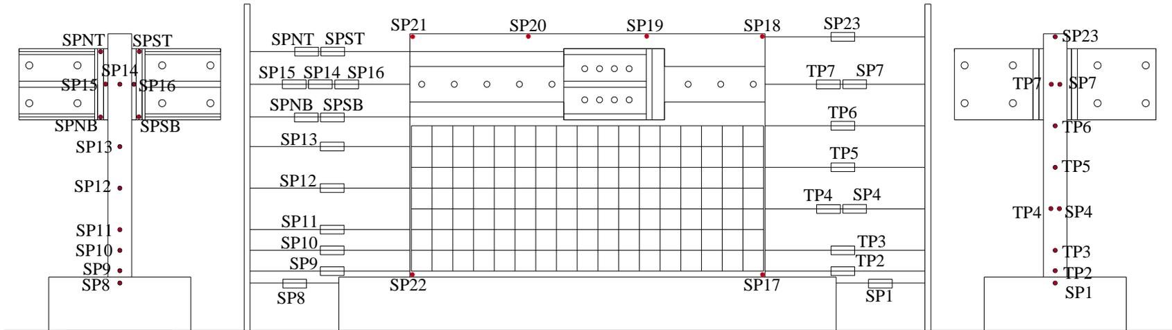
Figure C.48. In-plane and out-of-plane string potentiometers and Temposonics for SW12
