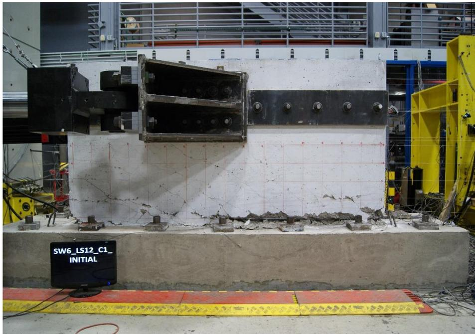
Figure E.46. Damage to SW6 at the end of testing
