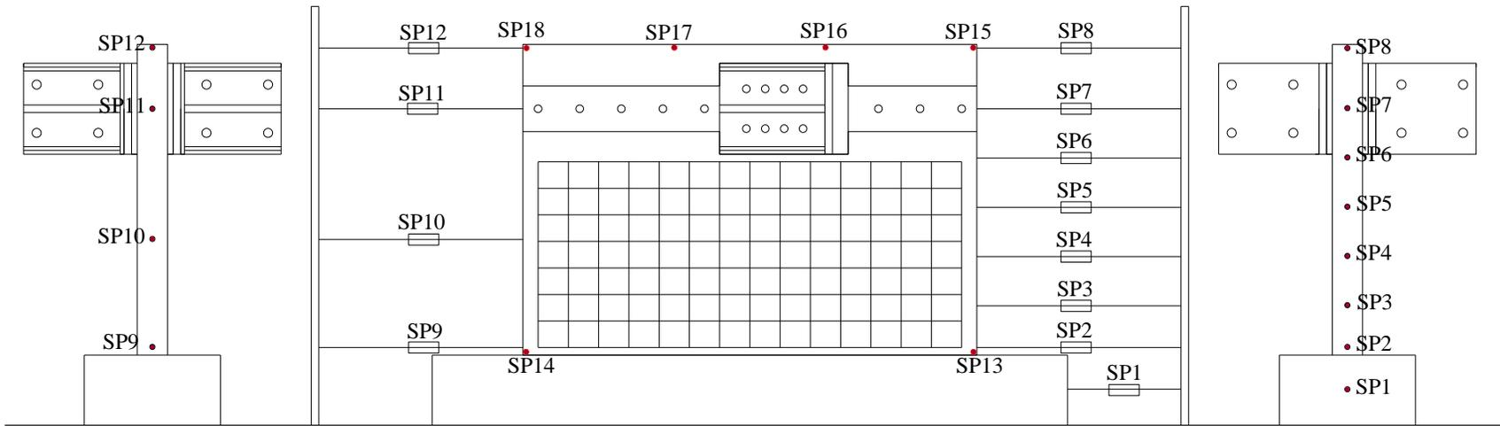
Figure C.39. In-plane and out-of-plane string potentiometers and Temposonics for SW3
