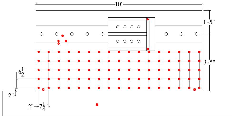
Figure C.5. Krypton LED sensors for SW5
