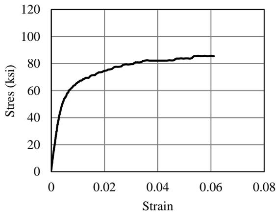
c) ASTM A706 rebar with Type-2 mechanical coupler
