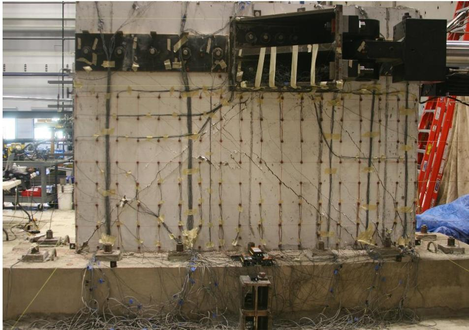
Figure E.87. Damage to SW10 at -0.87% drift ratio
