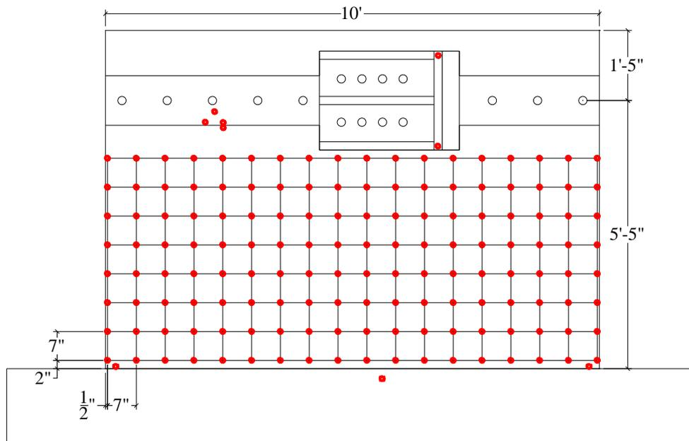
Figure C.12. Krypton LED sensors for SW12
