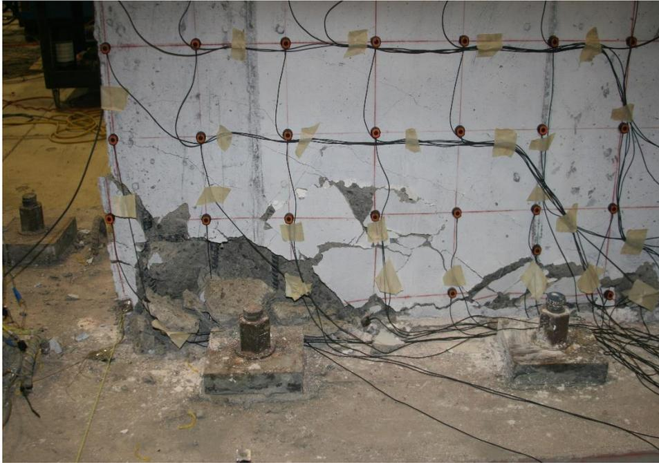
Figure E.97. Damage to SW11 at the end of testing
