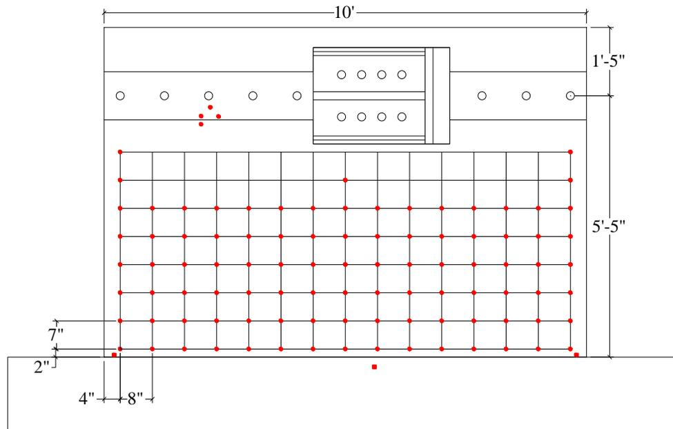
Figure C.3. Krypton LED sensors for SW3
