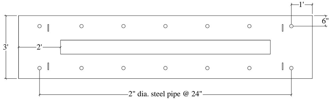
Figure A.3. Typical foundation thru-hole layout for the installation of Dywidag bars (Phase I specimens)
