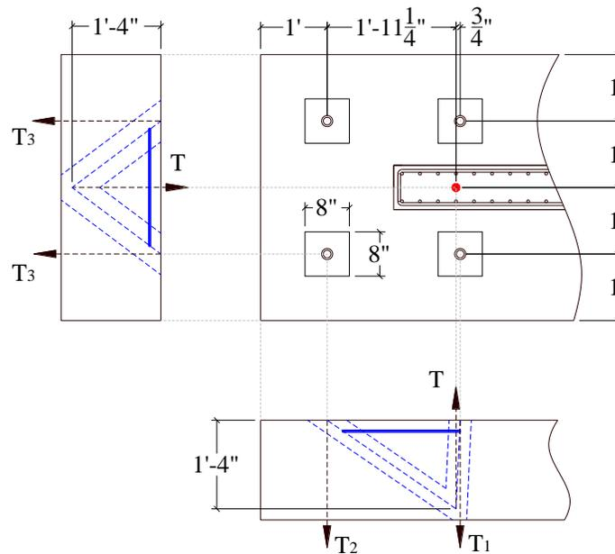
Figure B.2. Strut-and-tie model of the critical zone (longitudinal and transverse directions)
