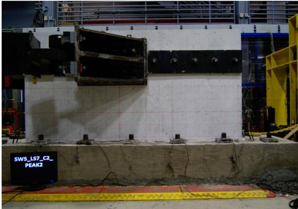
Figure E.37. Damage to SW5 at -0.59% drift ratio
