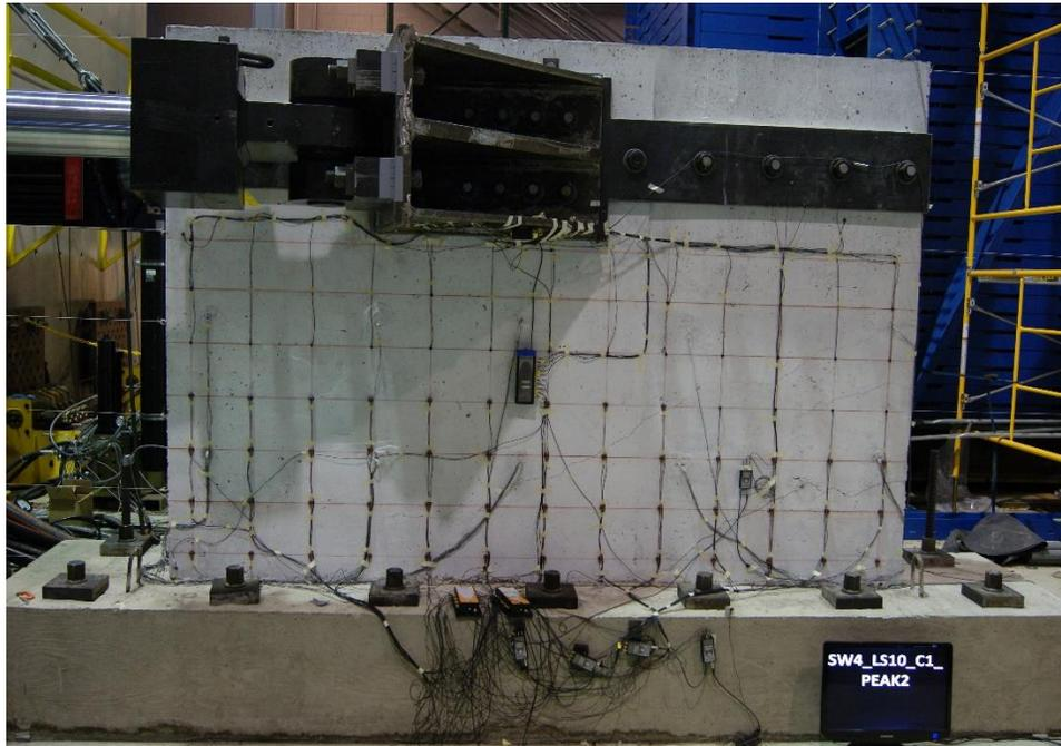
Figure E.28. Damage to SW4 at -0.55% drift ratio
