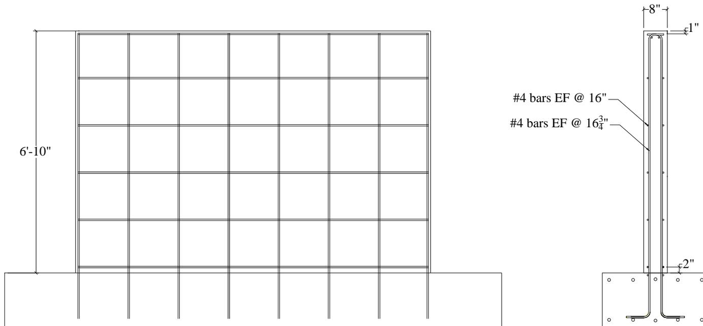
Figure A.10. Reinforcement details for SW4
