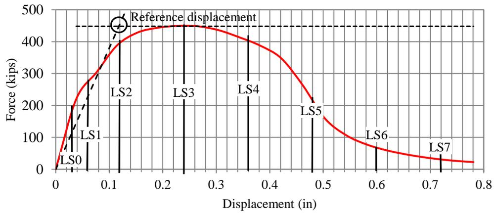
Figure D.21. Reference displacement for SW11
