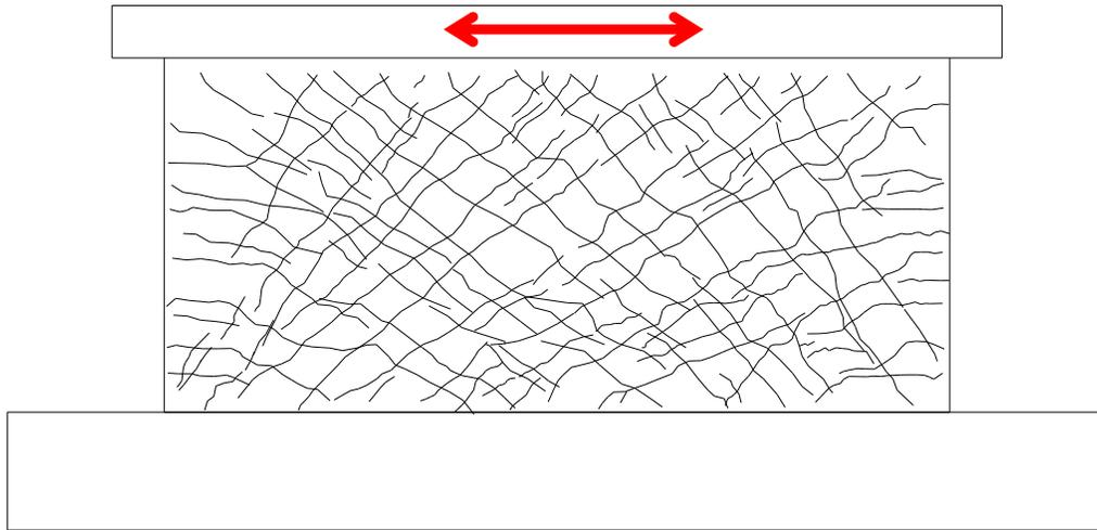
Figure 2.1. Typical cracking pattern for a low aspect ratio shear wall subjected to reversed cyclic lateral loading
