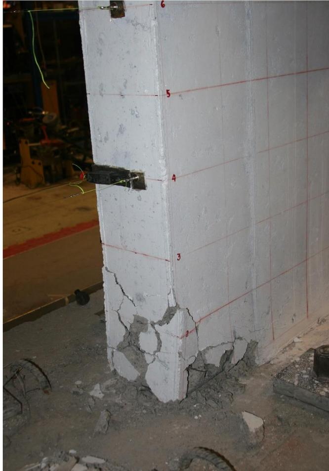
Figure E.66. Damage to SW8 following two cycles to 1.3% drift ratio
