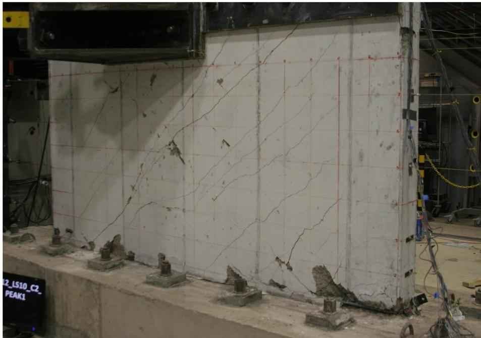
Figure E.108. Damage to SW12 at the end of testing
