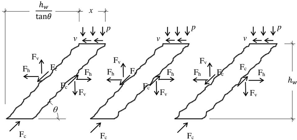
a) Forces in the concrete compression struts
