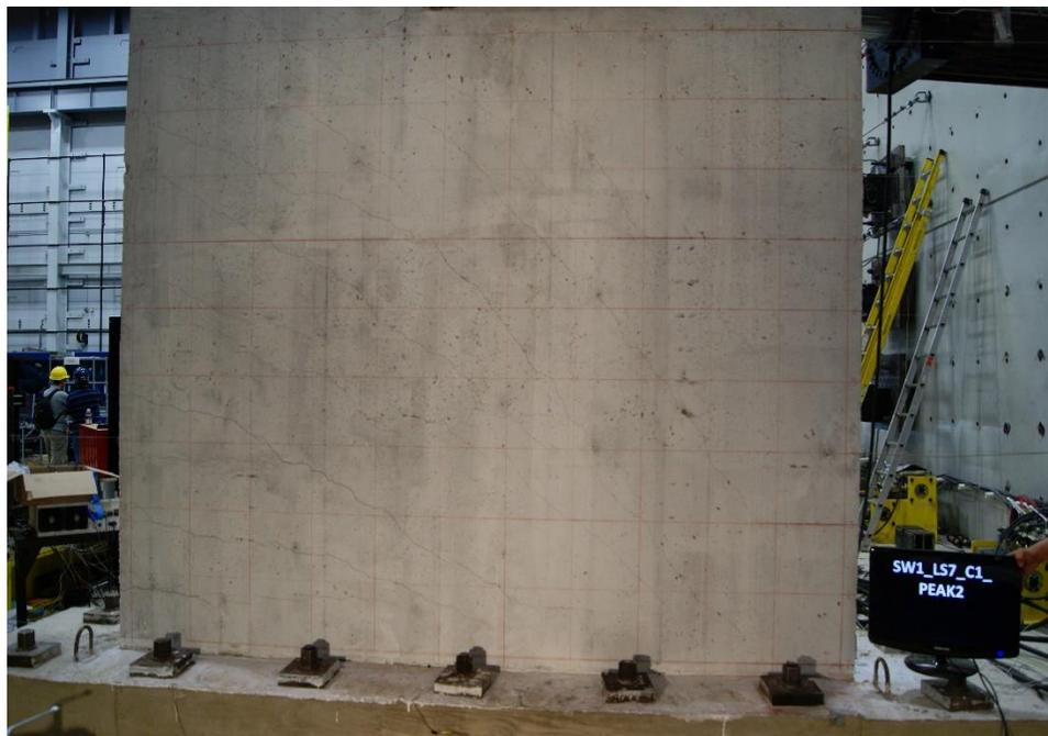
Figure E.3. Damage to SW1 at -0.61% drift ratio
