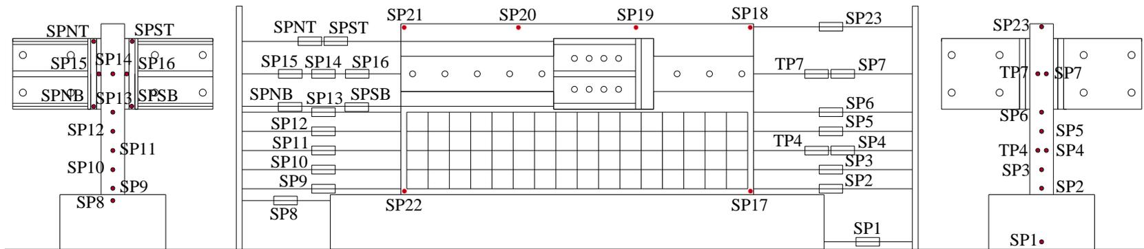
Figure C.42. In-plane and out-of-plane string potentiometers and Temposonics for SW6
