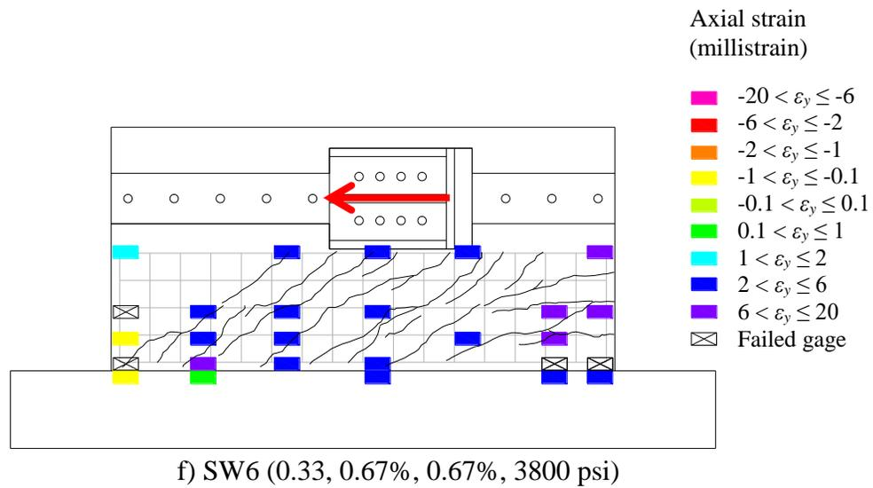
Figure 4.8. Strains on vertical reinforcement at peak strength (continued)
