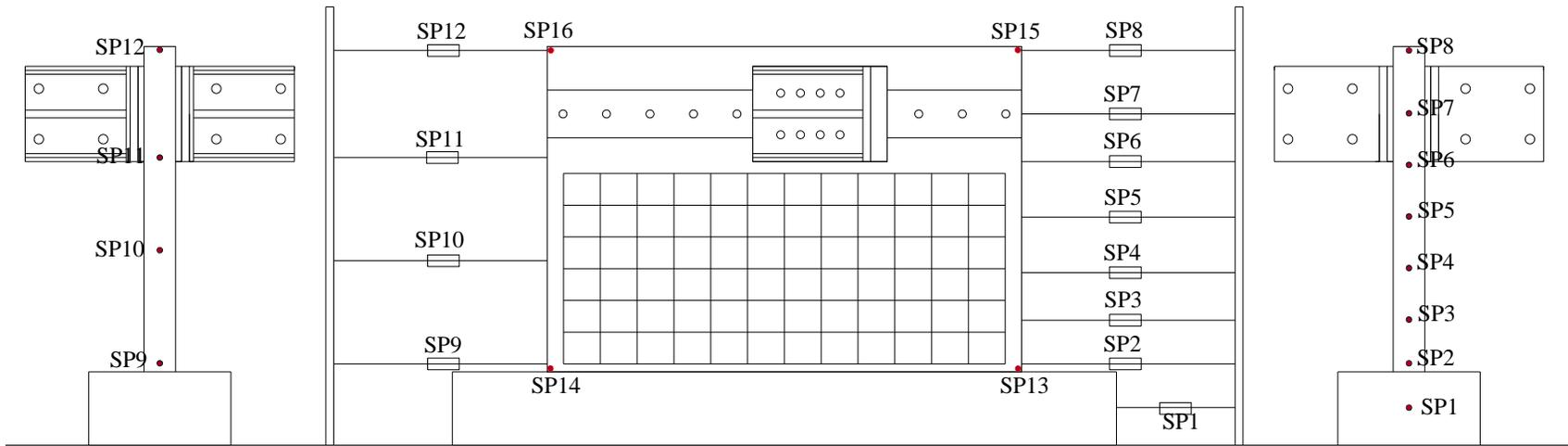
Figure C.40. In-plane and out-of-plane string potentiometers and Temposonics for SW4
