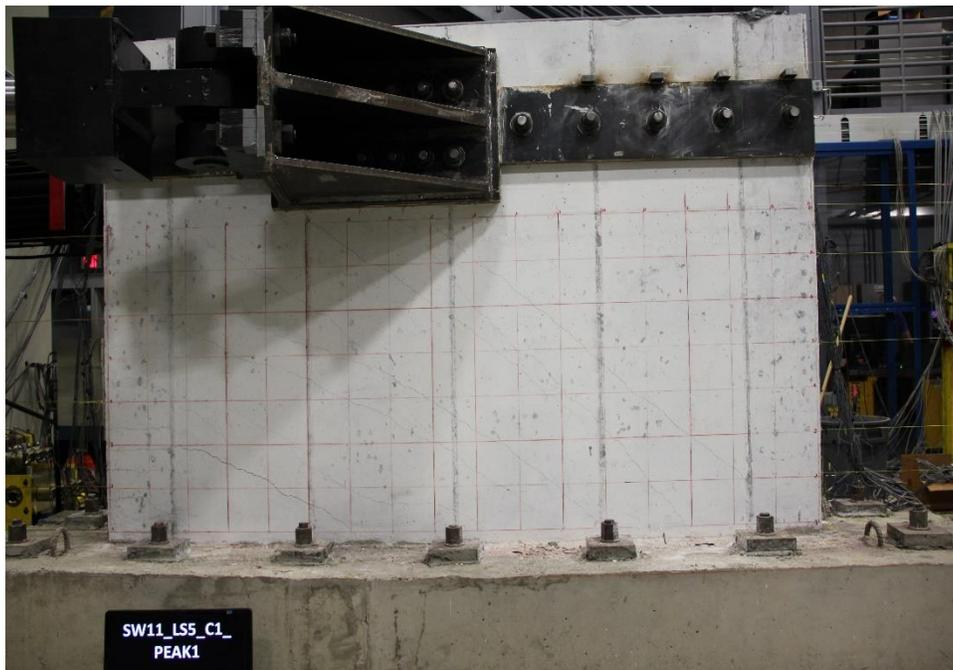
Figure E.92. Damage to SW11 at 0.56% drift ratio (peak strength)
