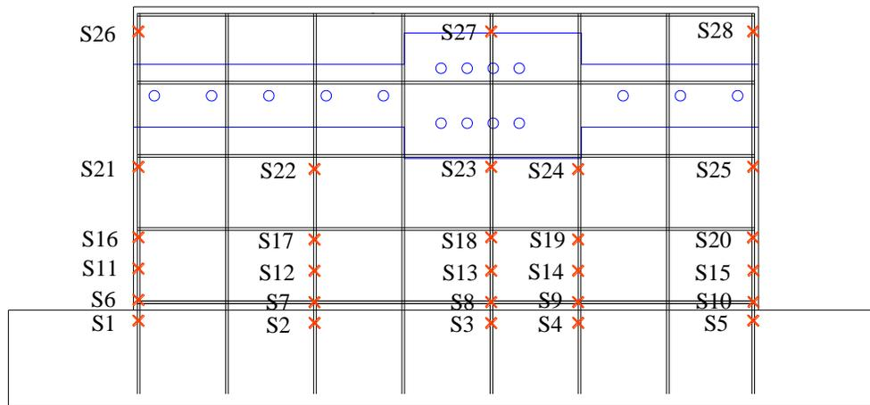
Figure C.19. Strain gages on the vertical reinforcements for SW7
