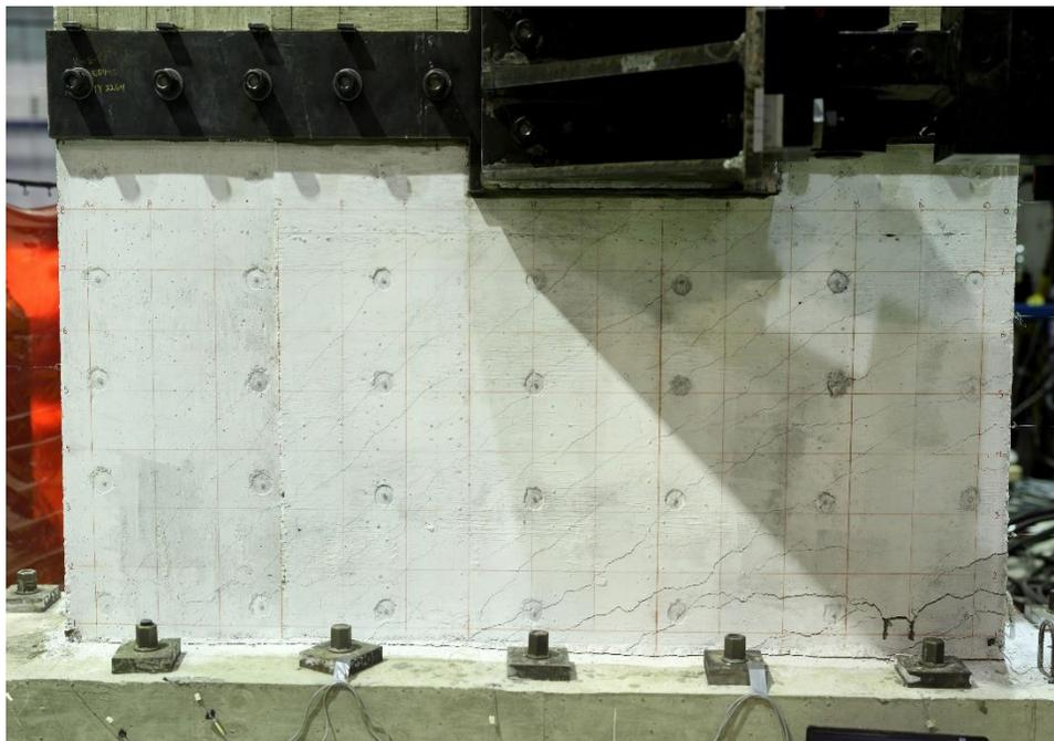
Figure E.13. Damage to SW2 at 1.25% drift ratio (peak strength)
