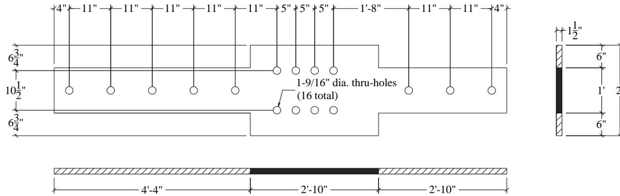
Figure A.19. Loading plate details
