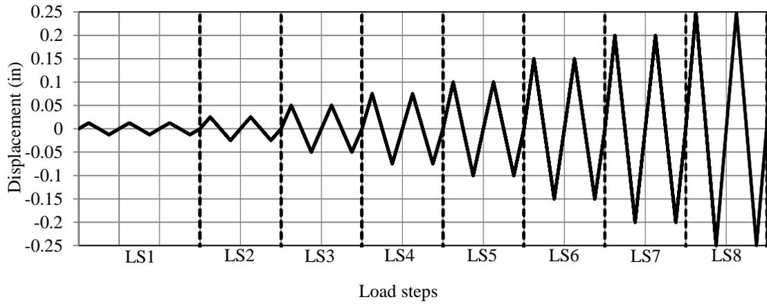
Figure D.8. Loading protocol for SW4
