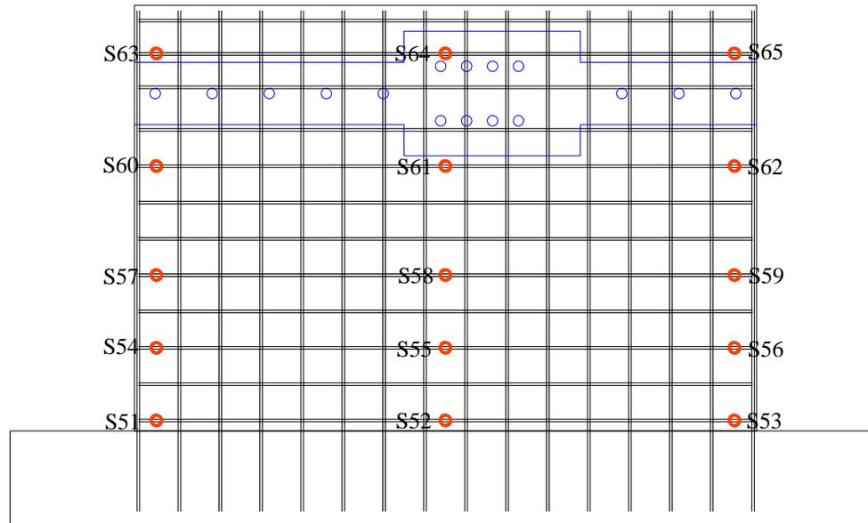
Figure C.27. Strain gages on the horizontal reinforcements for SW3
