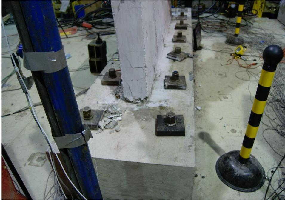
Figure E.16. Damage to SW2 at the end of testing
