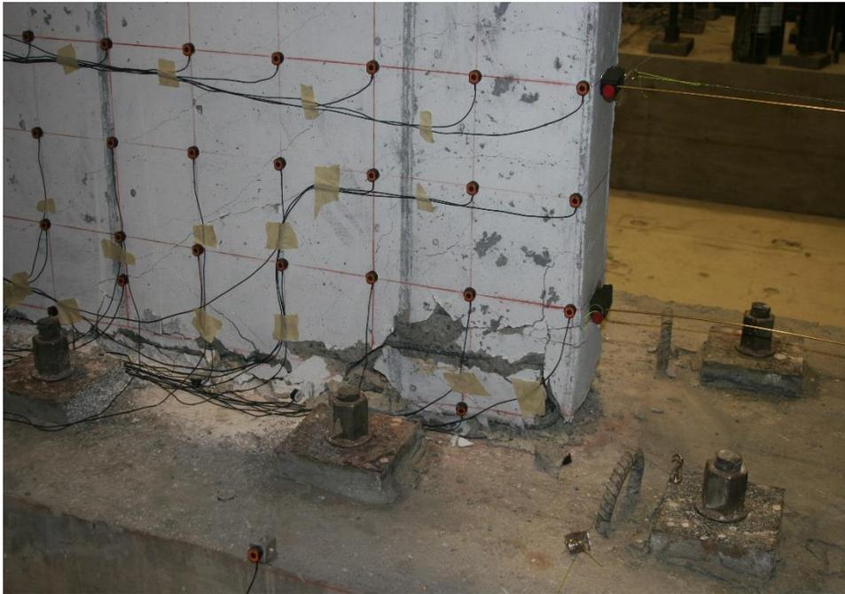
Figure E.98. Damage to SW11 at the end of testing
