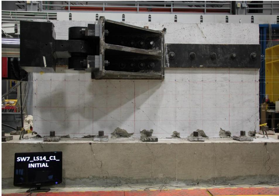
Figure E.53. Damage to SW7 at the end of testing
