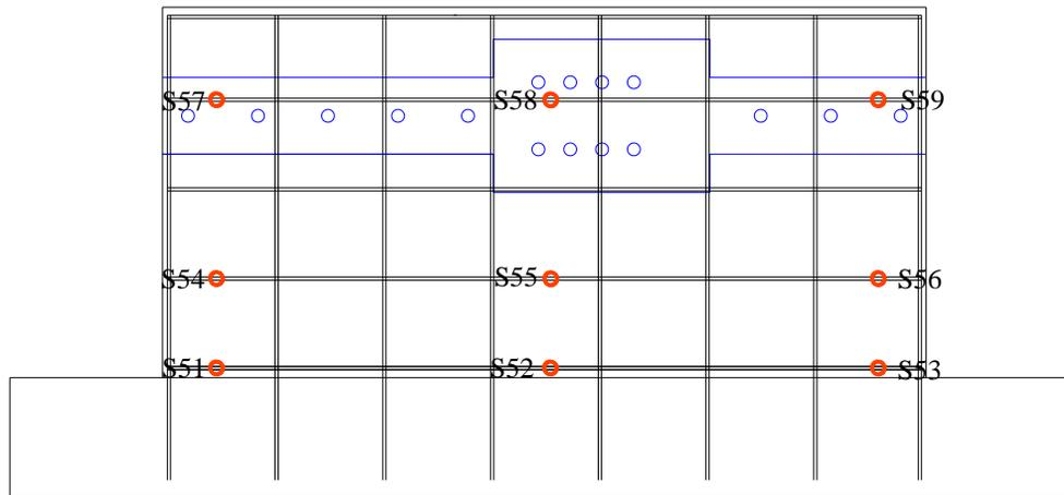
Figure C.31. Strain gages on the horizontal reinforcements for SW7
