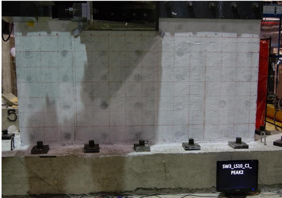
Figure E.20. Damage to SW3 at -0.76% drift ratio
