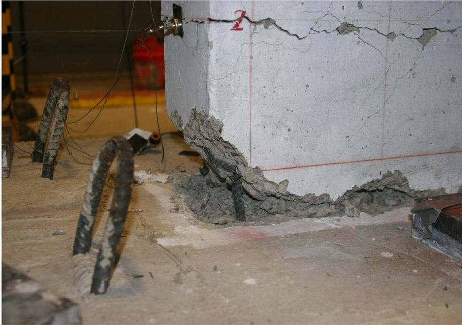
Figure E.47. Damage to SW6 at the end of testing
