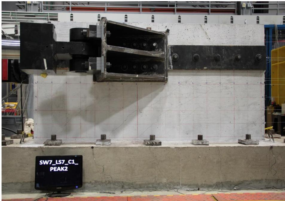
Figure E.52. Damage to SW7 at -0.41% drift ratio
