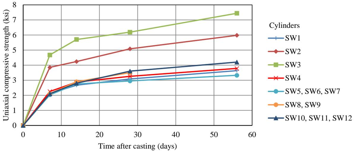
Figure 3.16. Concrete compressive strength from cylinder tests: walls
