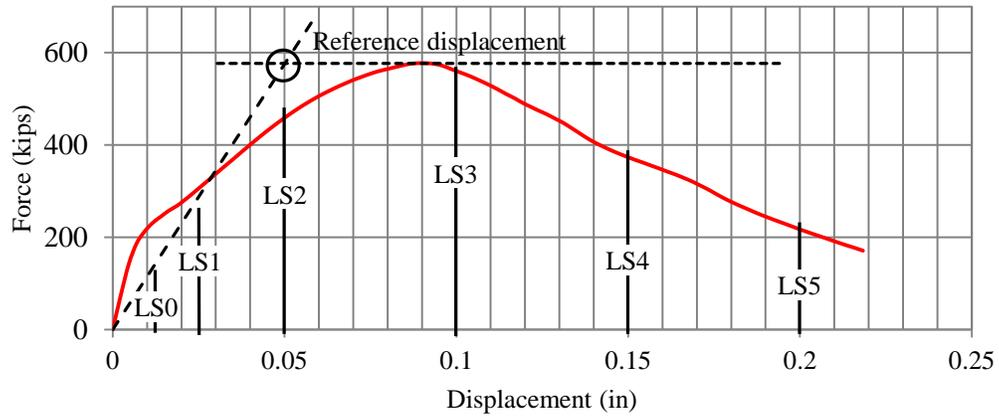
Figure D.9. Reference displacement for SW5
