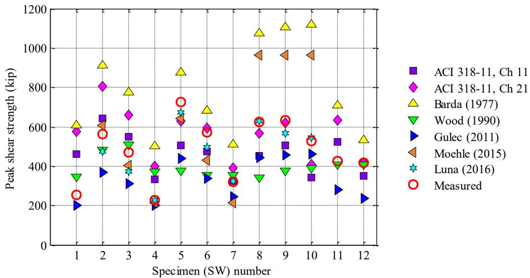
Figure 6.1. Measured and predicted peak shear strength
