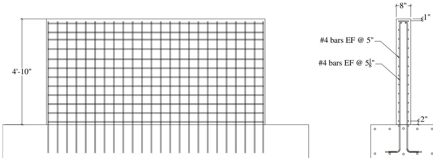
Figure A.11. Reinforcement details for SW5
