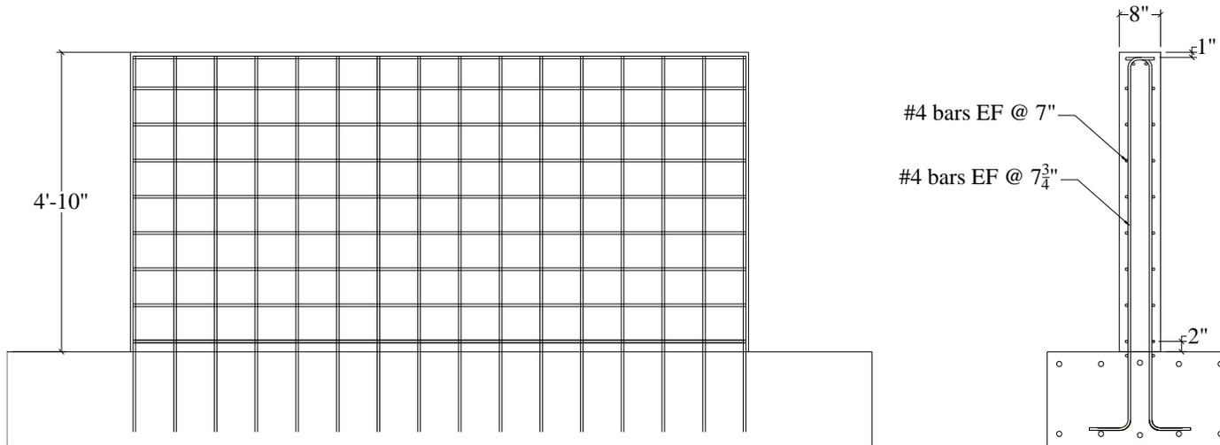
Figure A.12. Reinforcement details for SW6
