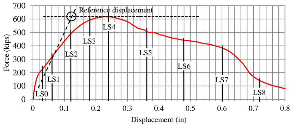
Figure D.17. Reference displacement for SW9
