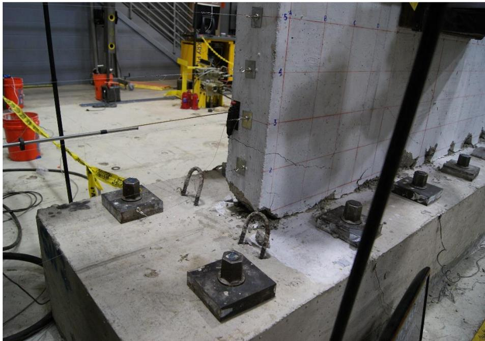
Figure E.54. Damage to SW7 at the end of testing
