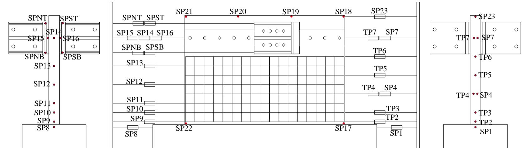
Figure C.47. In-plane and out-of-plane string potentiometers and Temposonics for SW11
