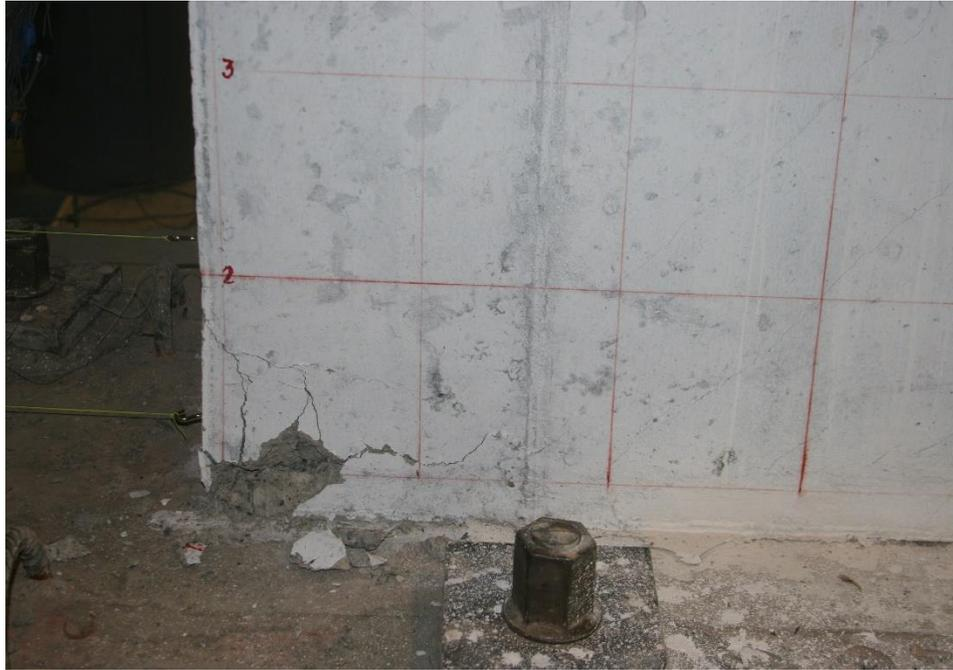
Figure E.62. Damage to SW8 at 0.91% drift ratio
