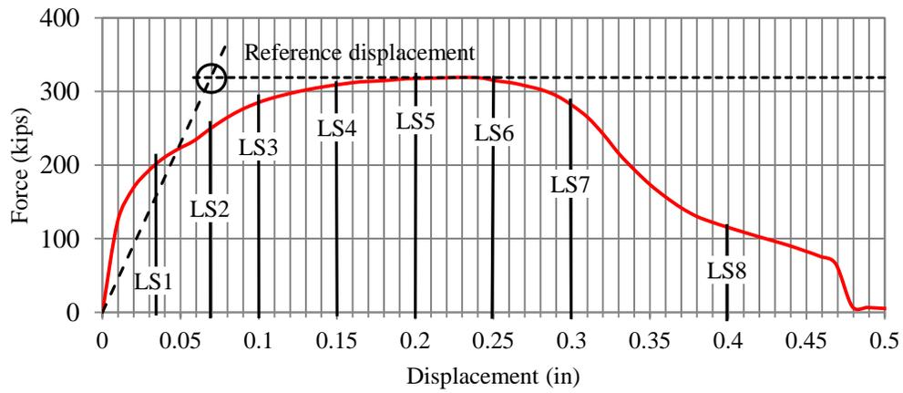
Figure D.5. Reference displacement for SW3
