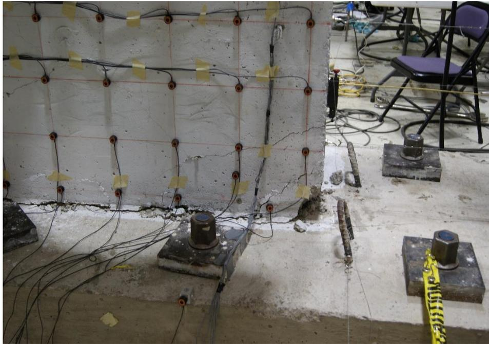
Figure E.56. Damage to SW7 at the end of testing
