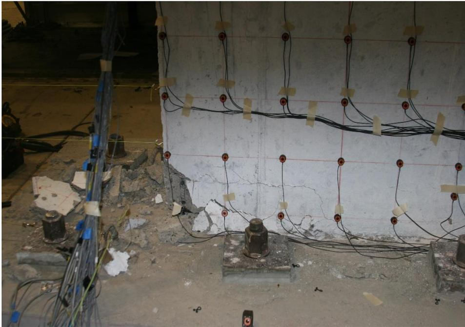
Figure E.68. Damage to SW8 following two cycles to 1.3% drift ratio
