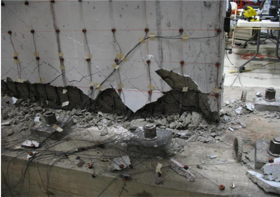
Figure E.79. Damage to SW9 at the end of testing
