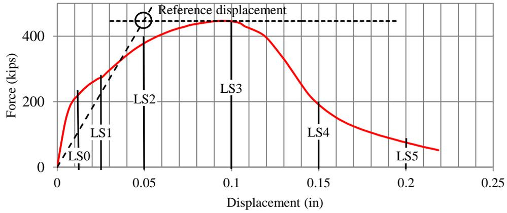
Figure D.11. Reference displacement for SW6
