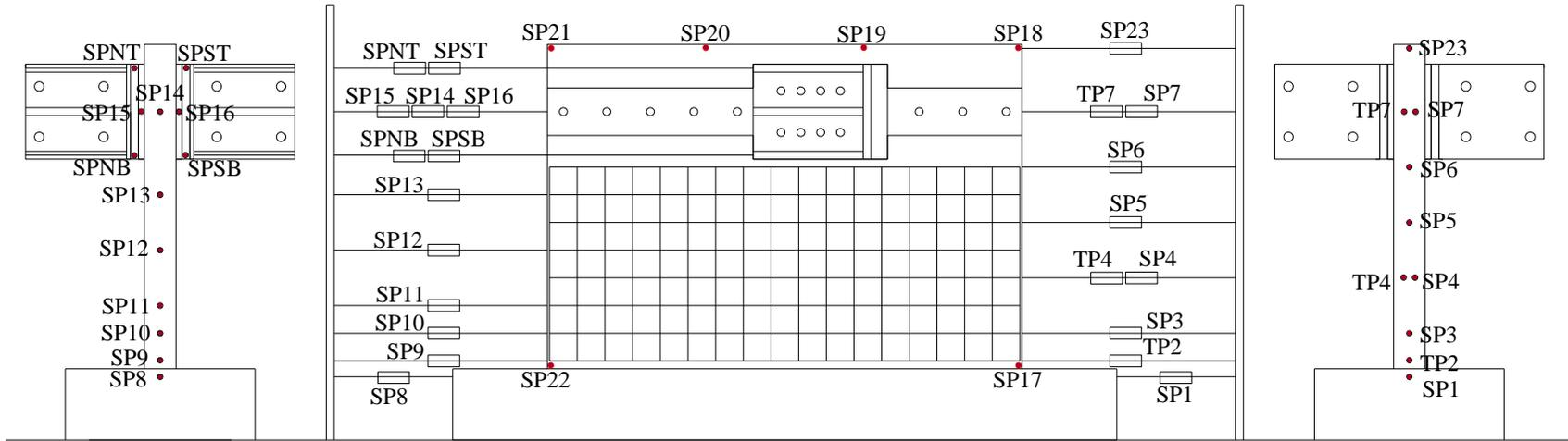
Figure C.45. In-plane and out-of-plane string potentiometers and Temposonics for SW9
