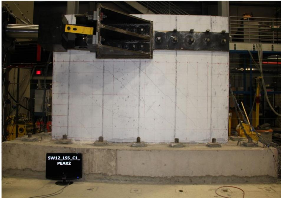
Figure E.101. Damage to SW12 at -0.54% drift ratio
