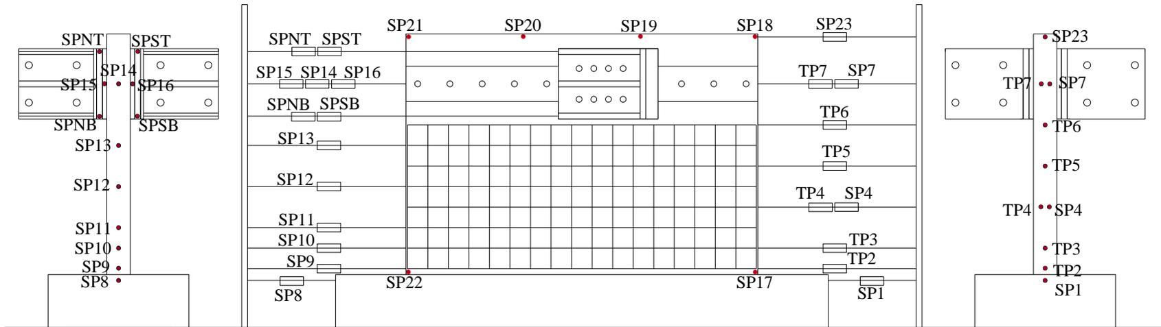
Figure C.46. In-plane and out-of-plane string potentiometers and Temposonics for SW10
