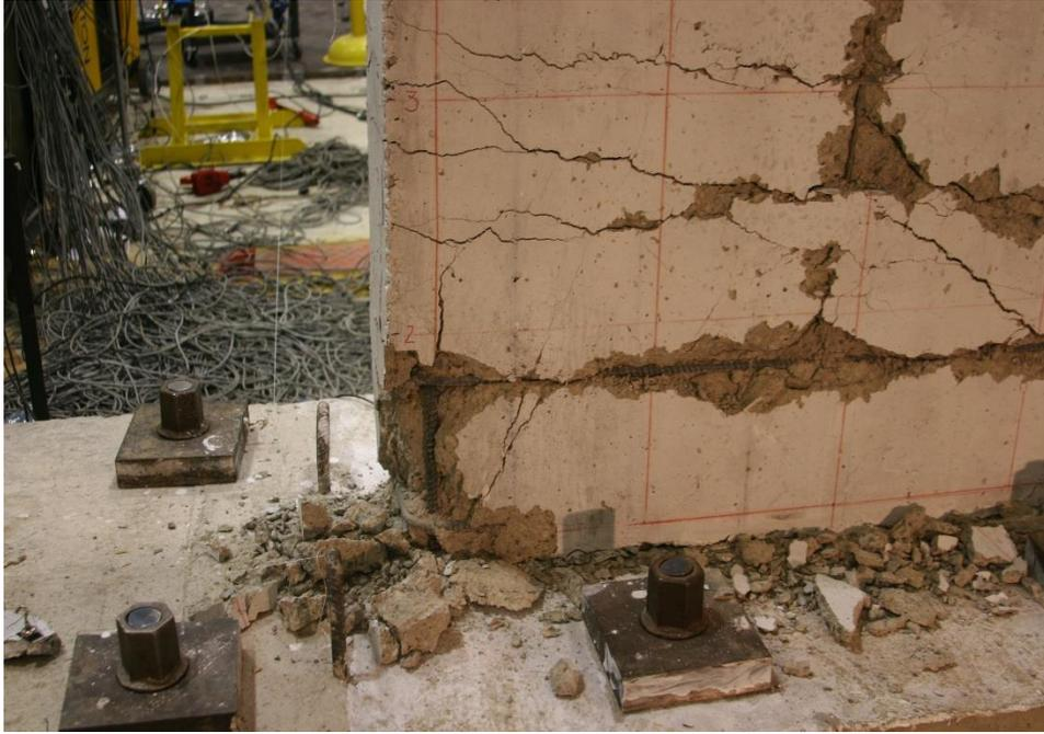
Figure E.10. Damage to SW1 at the end of testing
