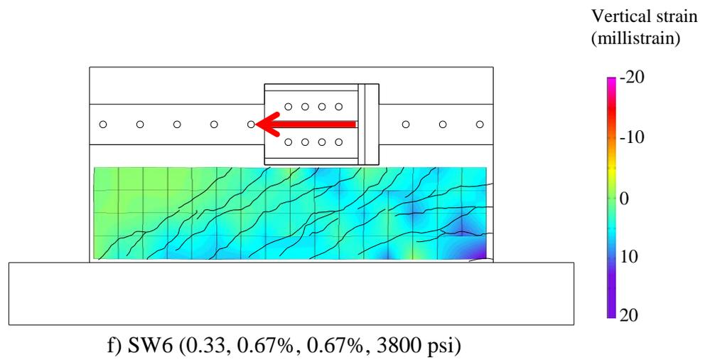
Figure 4.13. Vertical strain fields at peak strength (continued)
