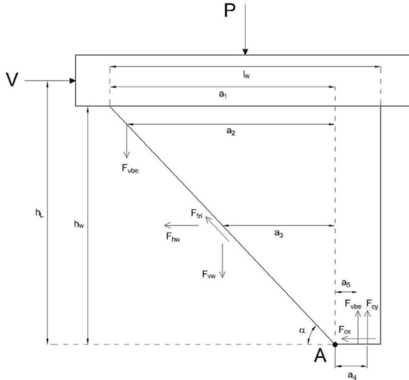
Figure 6.3. Free body diagram used to identify the functional form of Gulec and Whittaker equation for peak strength (reproduced from Gulec and Whittaker, 2009)
