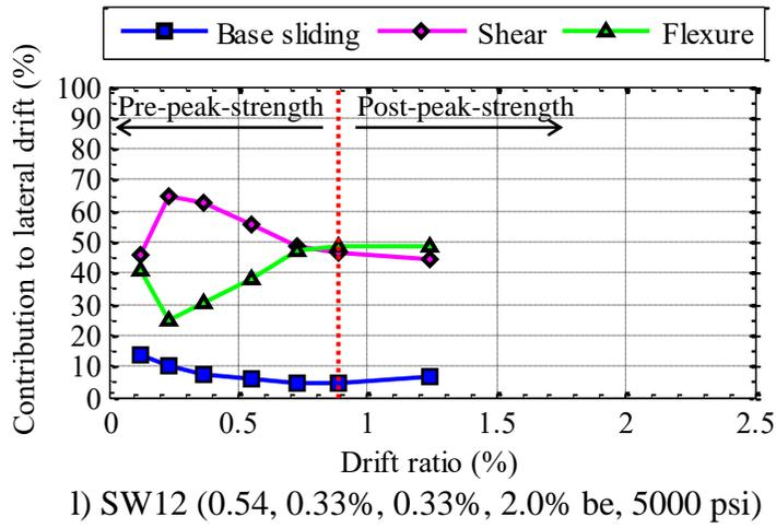
Figure 4.23. Components of the total lateral displacement (continued)
