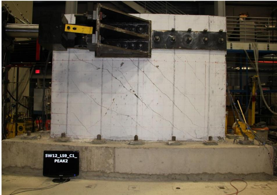
Figure E.107. Damage to SW12 at -1.64% drift ratio
