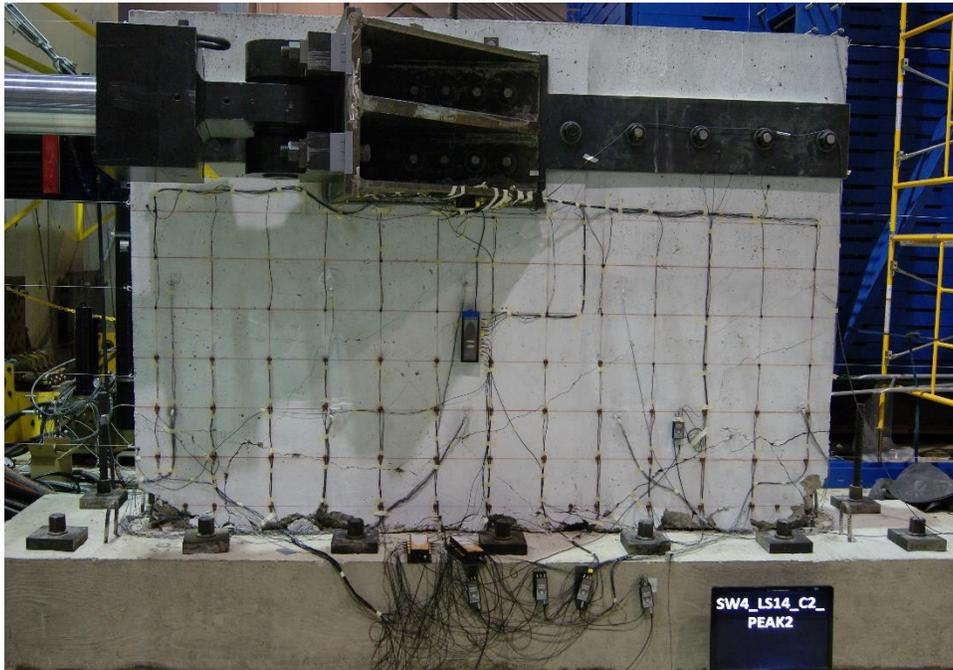
Figure E.31. Damage to SW4 at the end of testing
