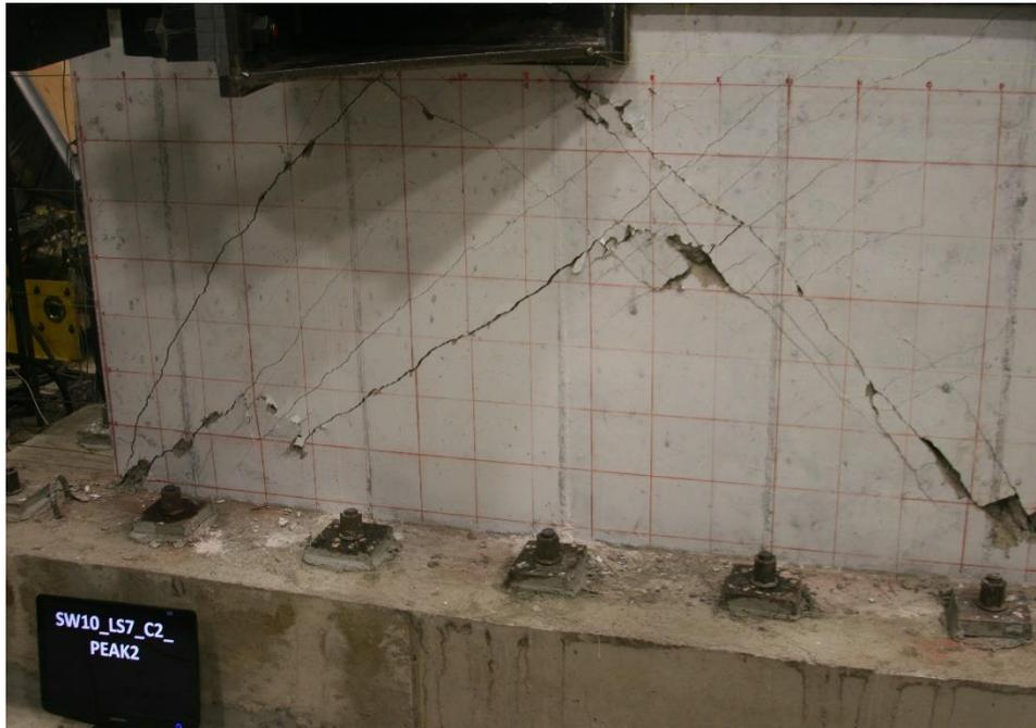
Figure E.88. Damage to SW10 at -0.87% drift ratio
