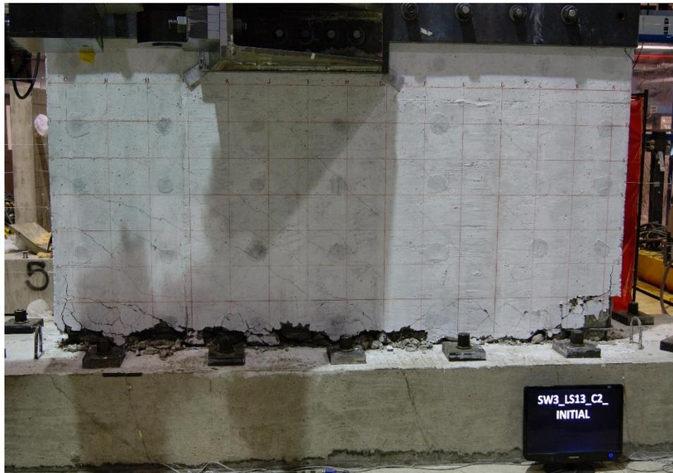
Figure E.23. Damage to SW3 at the end of testing
