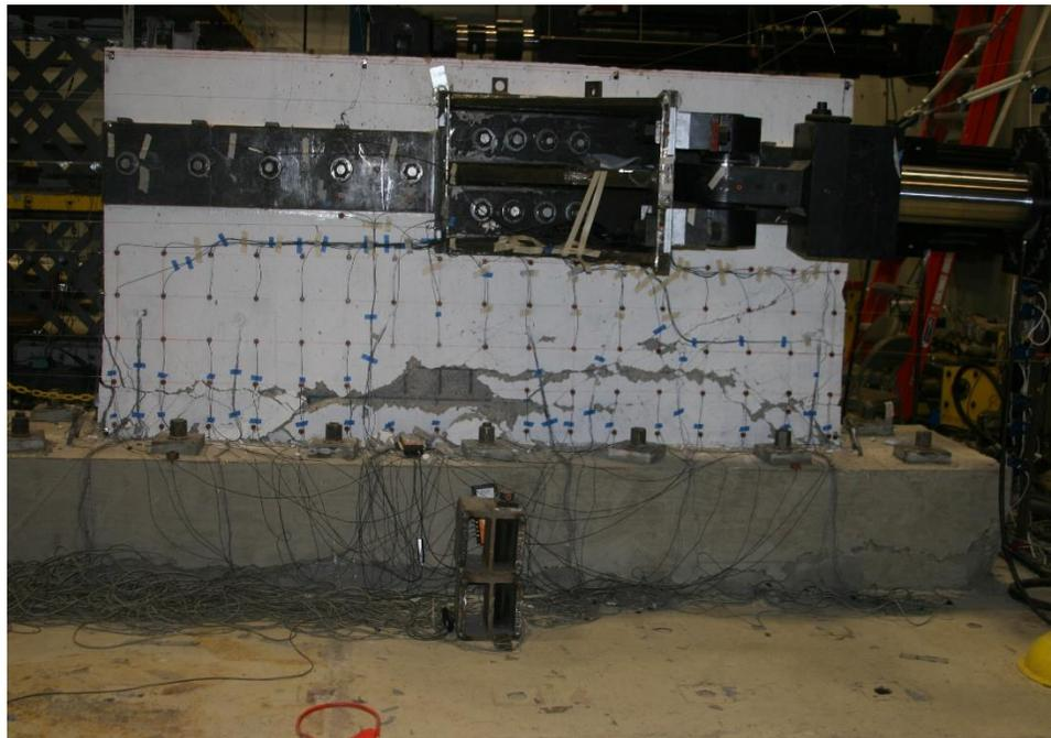
Figure E.40. Damage to SW5 at the end of testing
