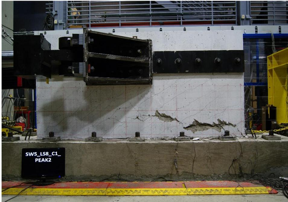
Figure E.39. Damage to SW5 at -1.31% drift ratio
