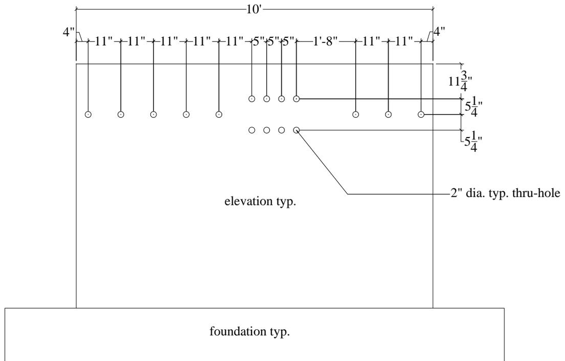
Figure A.5. Typical thru-hole layout for the installation of loading apparatus
