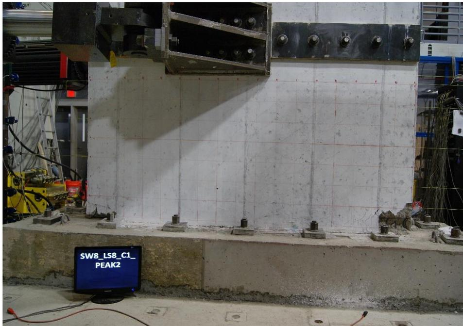
Figure E.65. Damage to SW8 at -1.28% drift ratio
