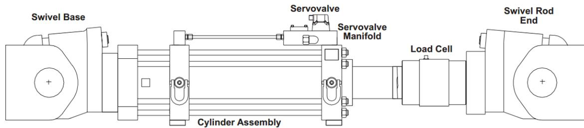
Figure C.49. MTS 243.90T actuator assembly
