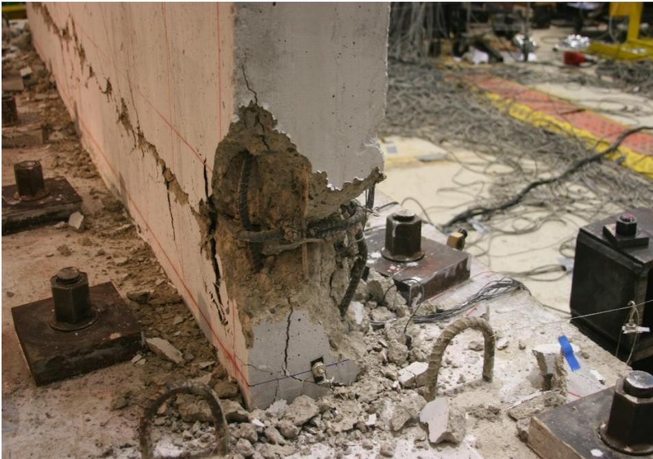
Figure E.11. Damage to SW1 at the end of testing
