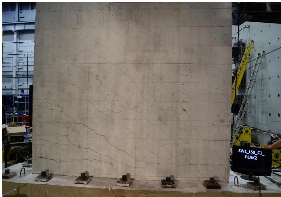
Figure E.5. Damage to SW1 at -1.28% drift ratio
