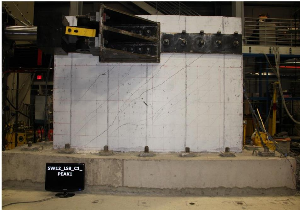
Figure E.102. Damage to SW12 at 1.24% drift ratio
