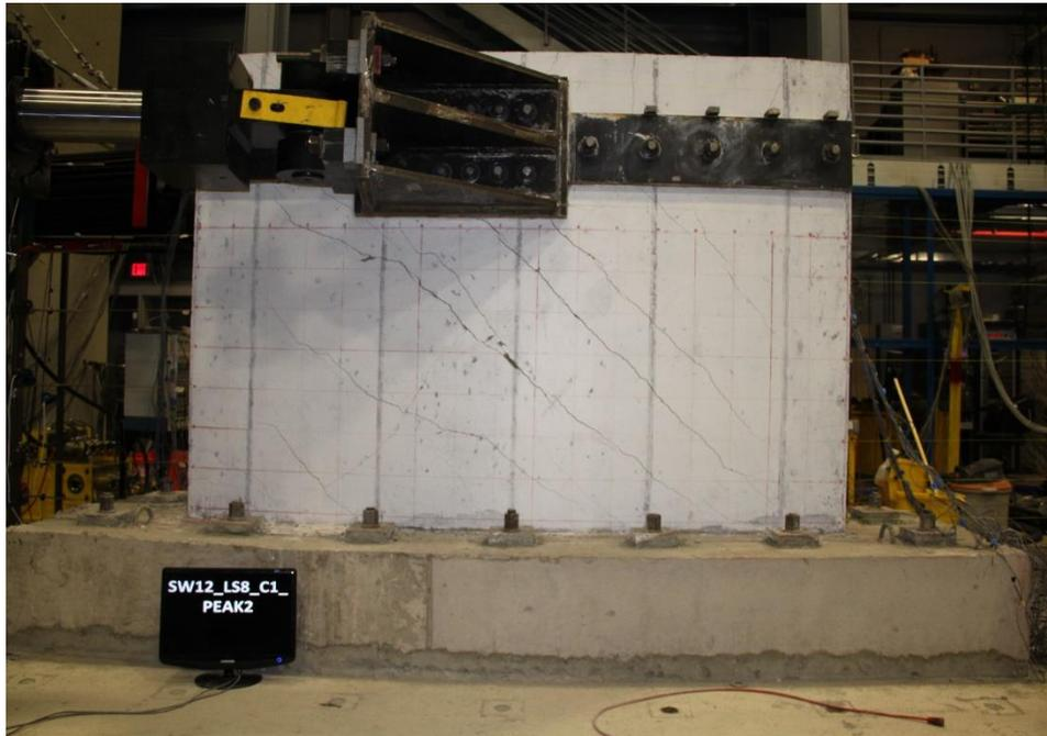
Figure E.103. Damage to SW12 at -1.24% drift ratio (peak strength)
