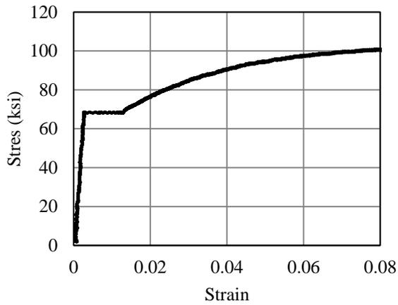
a) ASTM A615 rebar
