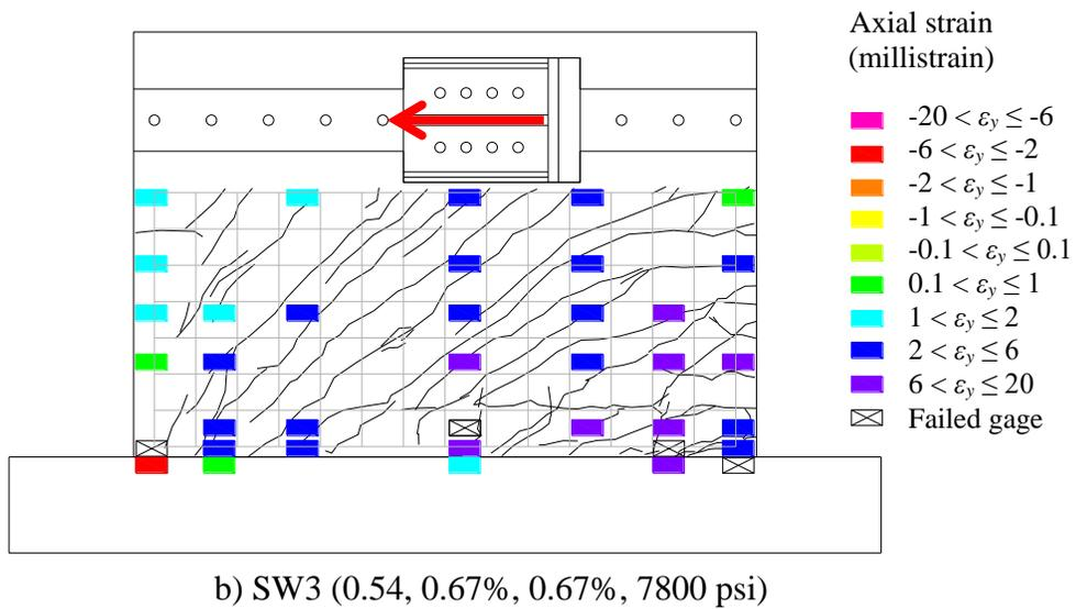
Figure 4.10. Strains on vertical reinforcement of SW2 and SW3 at 0.7% drift ratio
