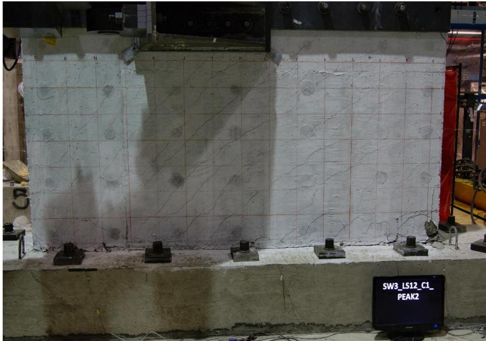
Figure E.22. Damage to SW3 at -1.96% drift ratio
