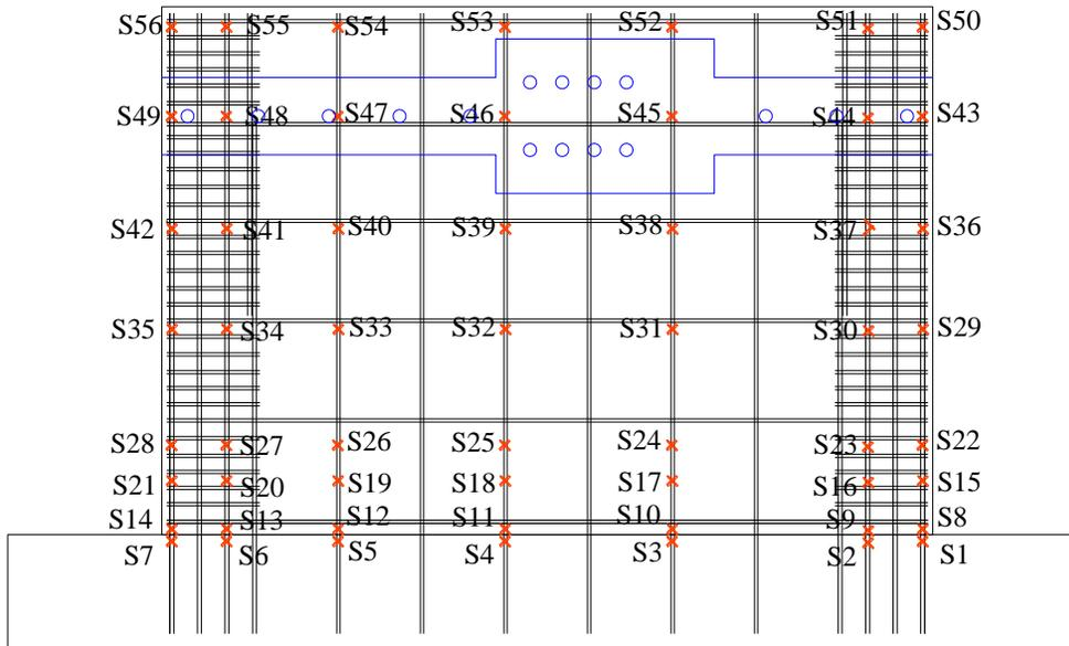
Figure C.24. Strain gages on the vertical reinforcements for SW12
