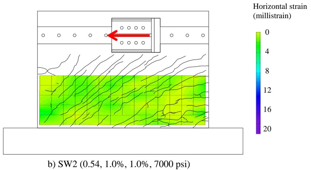
Figure 4.14. Horizontal strain fields at peak strength
