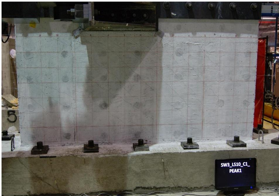
Figure E.19. Damage to SW3 at 0.75% drift ratio
