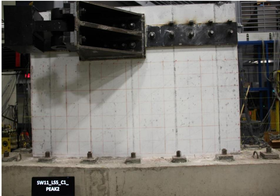
Figure E.93. Damage to SW11 at -0.57% drift ratio
