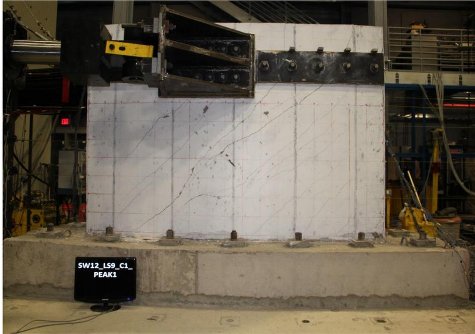
Figure E.105. Damage to SW12 at 1.63% drift ratio
