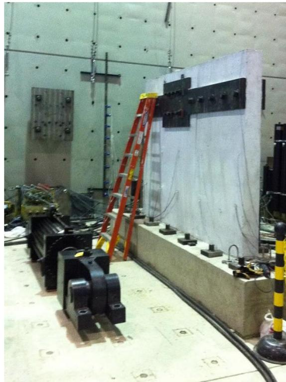
Figure 3.20. Loading plate installation
