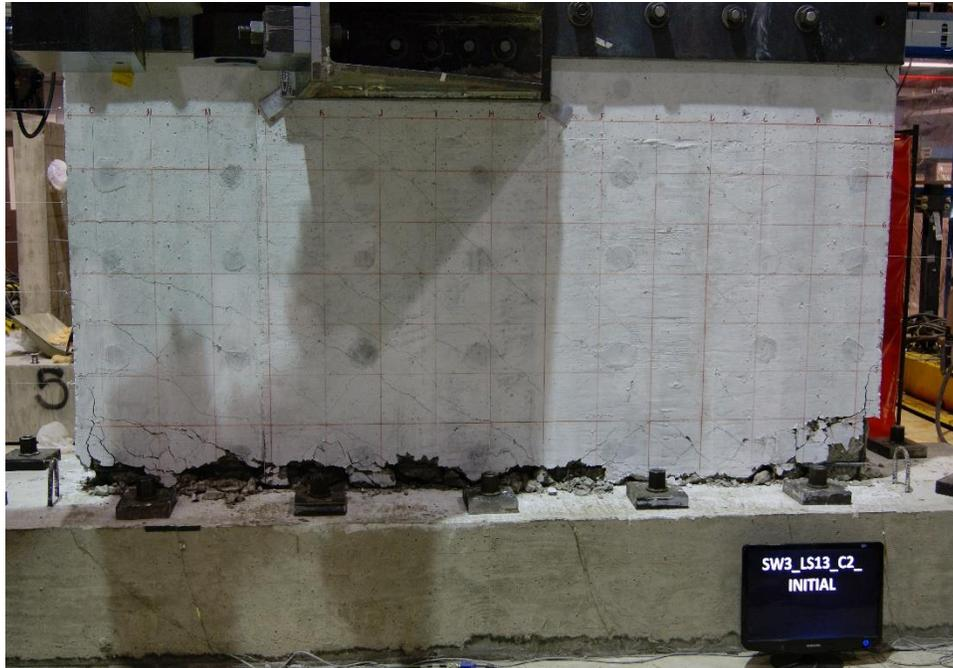
Figure 2.4. Sliding shear failure
