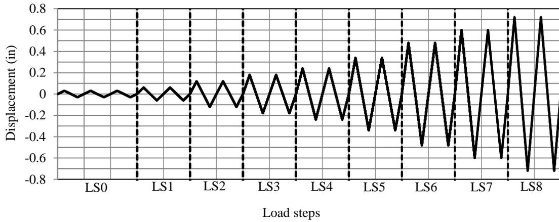
Figure D.18. Loading protocol for SW9
