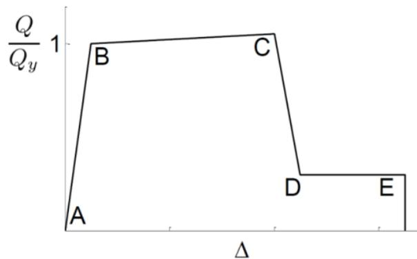
Figure 5.1. ASCE 41-13 force-deformation relationship (ASCE, 2013)
