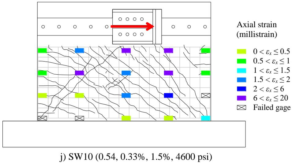
Figure 4.9. Strains on horizontal reinforcement at peak strength (continued)
