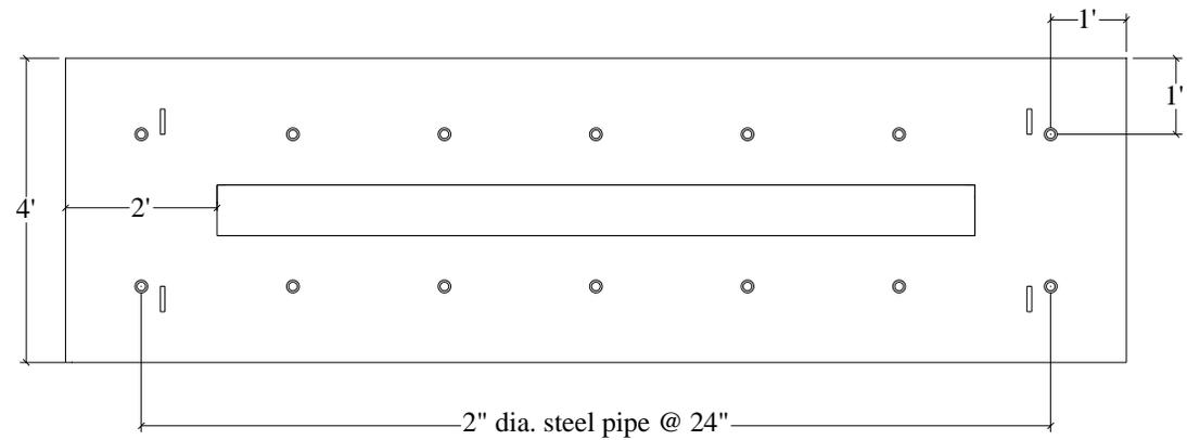
Figure A.4. Typical foundation thru-hole layout for the installation of Dywidag bars (Phase II specimens)
