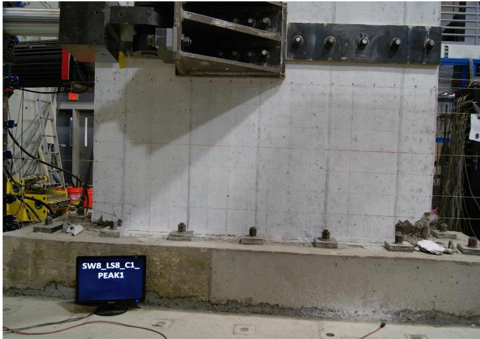
Figure E.64. Damage to SW8 at 1.31% drift ratio
