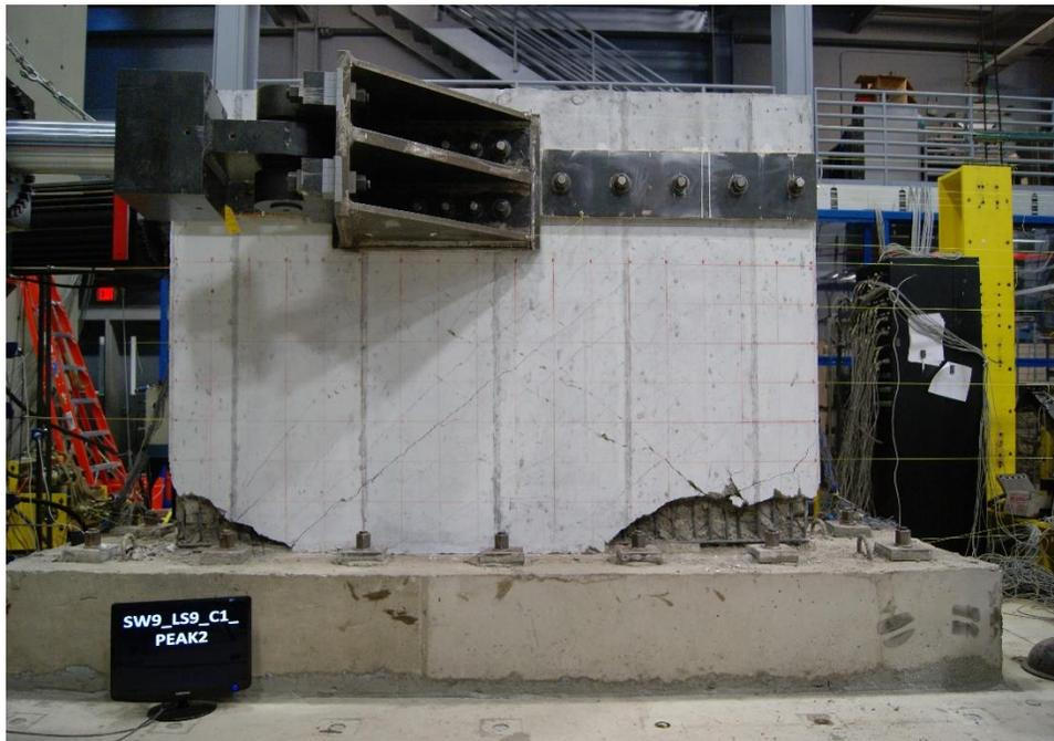
Figure E.76. Damage to SW9 at -1.72% drift ratio
