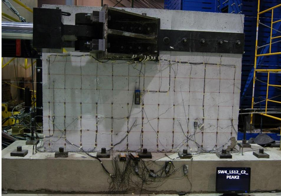
Figure E.30. Damage to SW4 at -1.06% drift ratio
