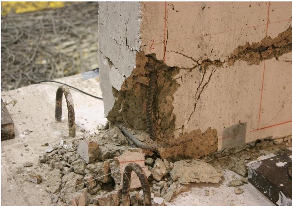
Figure E.9. Damage to SW1 at the end of testing
