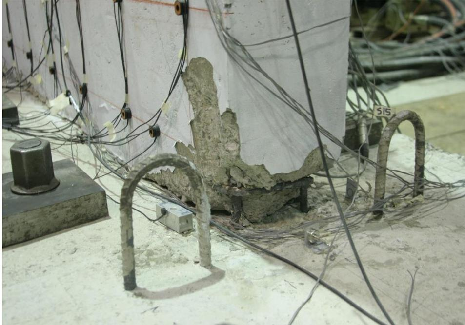
Figure E.32. Damage to SW4 at the end of testing
