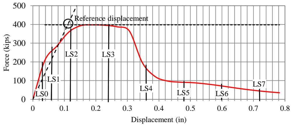
Figure D.23. Reference displacement for SW12
