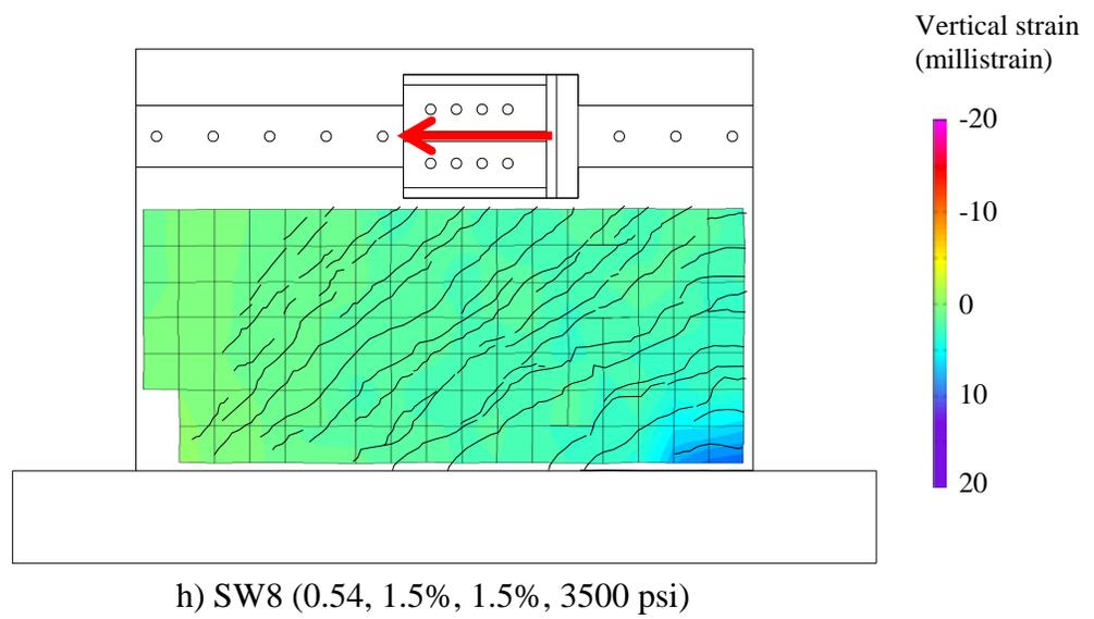
Figure 4.13. Vertical strain fields at peak strength (continued)
