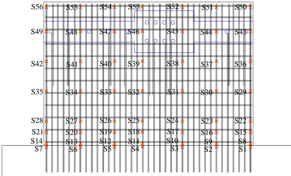
Figure C.21. Strain gages on the vertical reinforcements for SW9
