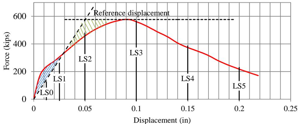
Figure 3.25. Reference displacement for SW5
