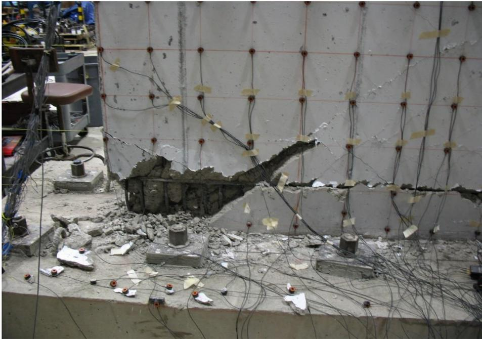
Figure E.80. Damage to SW9 at the end of testing
