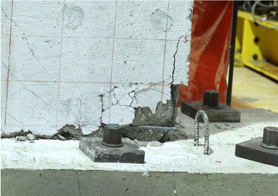
Figure E.25. Damage to SW3 at the end of testing
