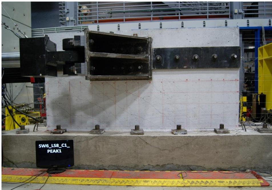
Figure E.44. Damage to SW6 at 0.81% drift ratio (peak strength)
