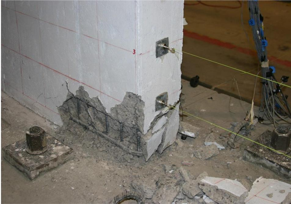
Figure E.67. Damage to SW8 following two cycles to 1.3% drift ratio
