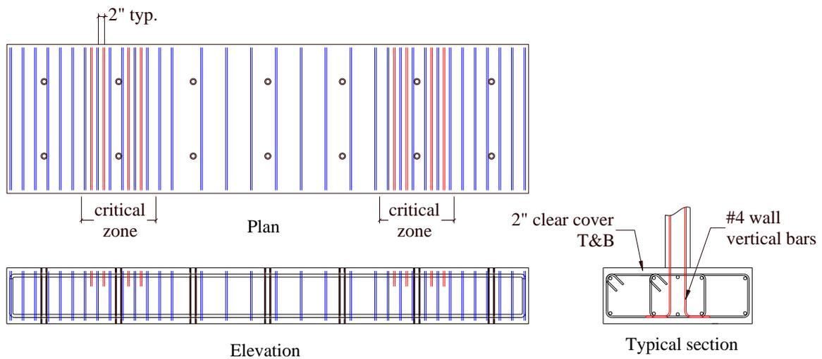
Figure B.4. Supplemental transverse reinforcement
