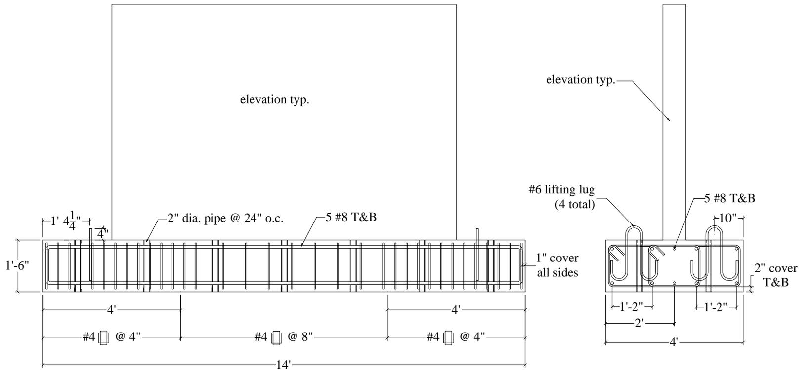
Figure A2. Typical foundation drawings (Phase II specimens)
