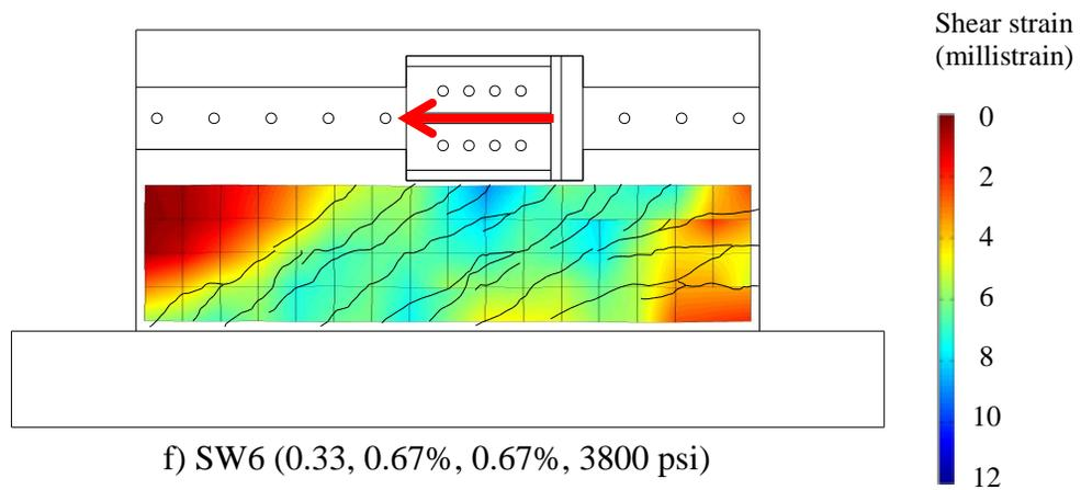
Figure 4.17. Shear strain fields at peak strength (continued)
