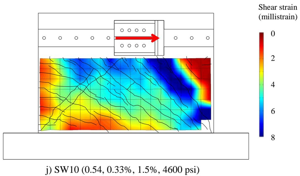
Figure 4.17. Shear strain fields at peak strength (continued)
