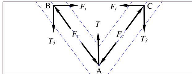
Figure B.3. Idealized free-body diagram of the nodes of the strut-and-tie model (transverse direction)
