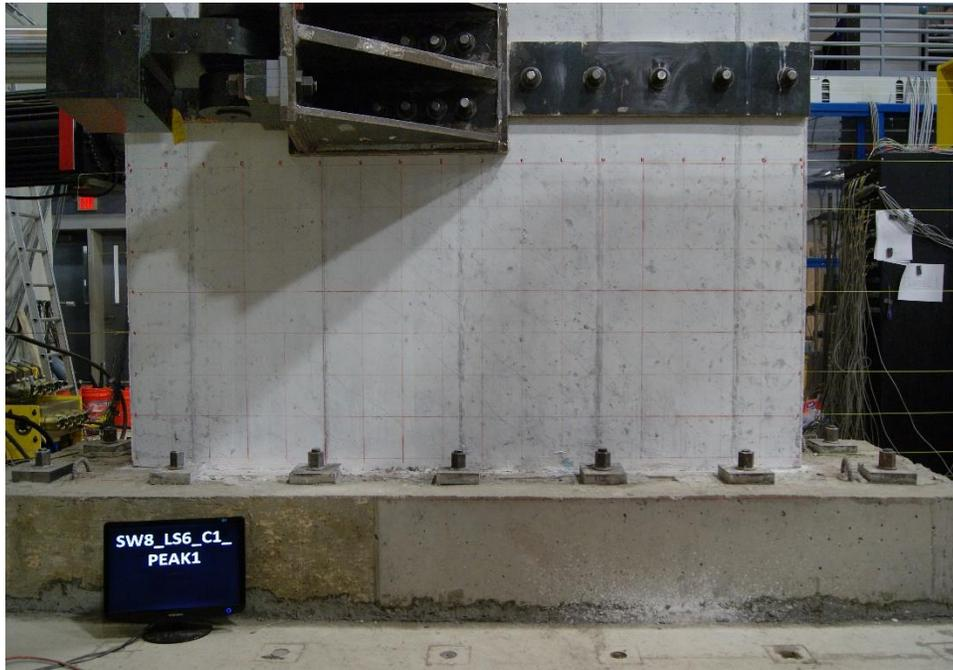
Figure E.60. Damage to SW8 at 0.70% drift ratio (peak strength)
