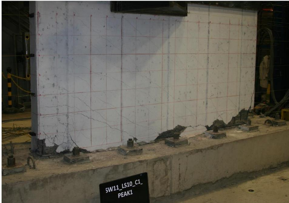
Figure E.95. Damage to SW11 at 2.4% drift ratio
