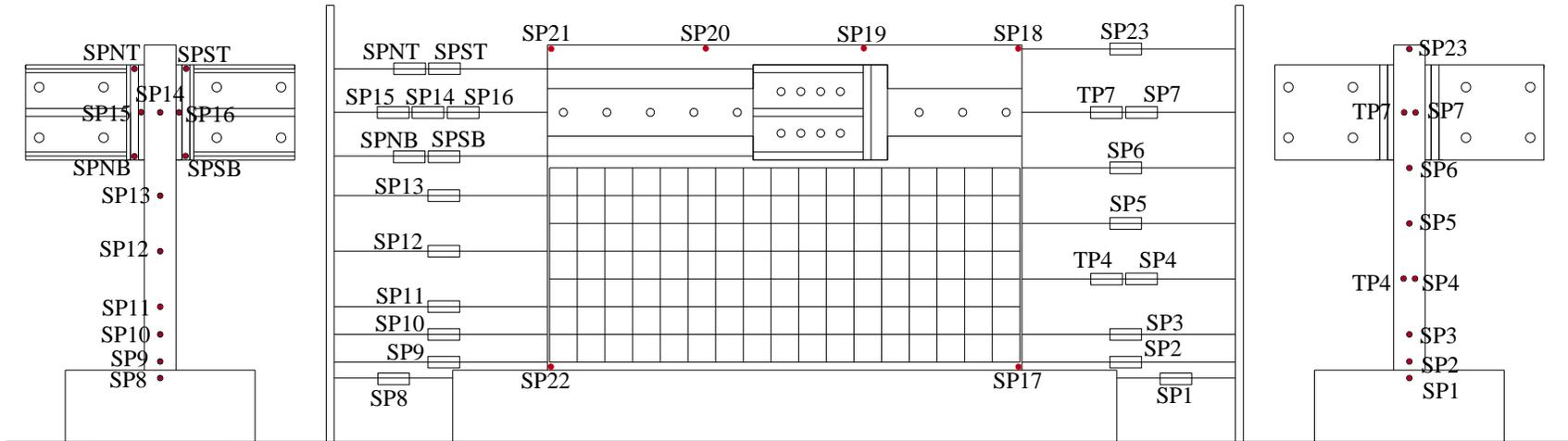
Figure C.44. In-plane and out-of-plane string potentiometers and Temposonics for SW8
