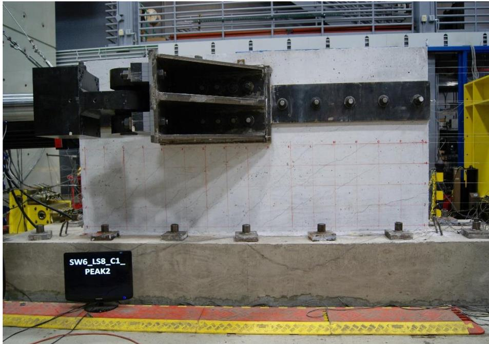
Figure E.45. Damage to SW6 at -0.81% drift ratio
