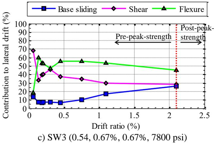
Figure 4.23. Components of the total lateral displacement
