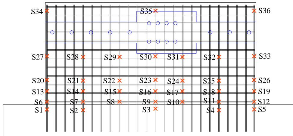
Figure C.17. Strain gages on the vertical reinforcements for SW5
