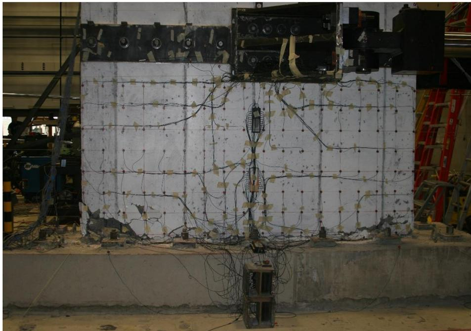
Figure E.96. Damage to SW11 at the end of testing
