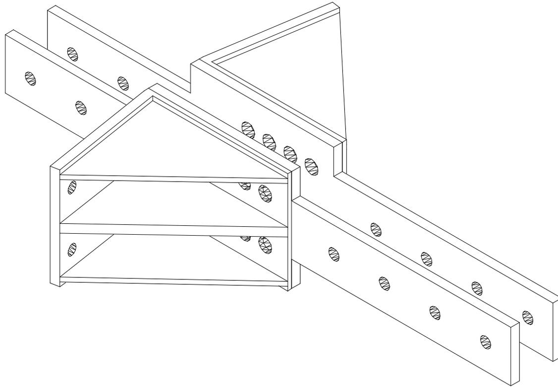
Figure A.22. Isometric drawing of the loading apparatus
