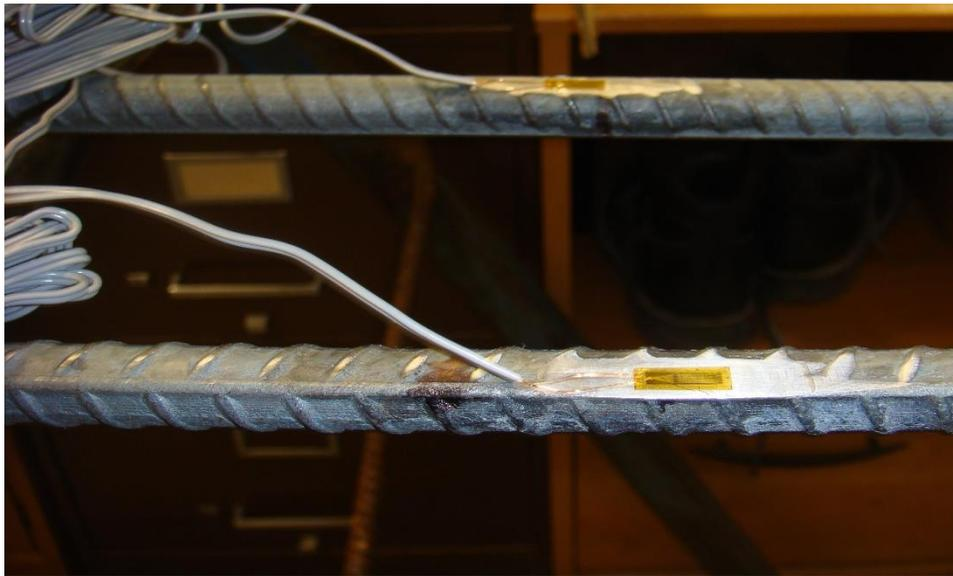
Figure C.57. YFLA-5-5L strain gages
