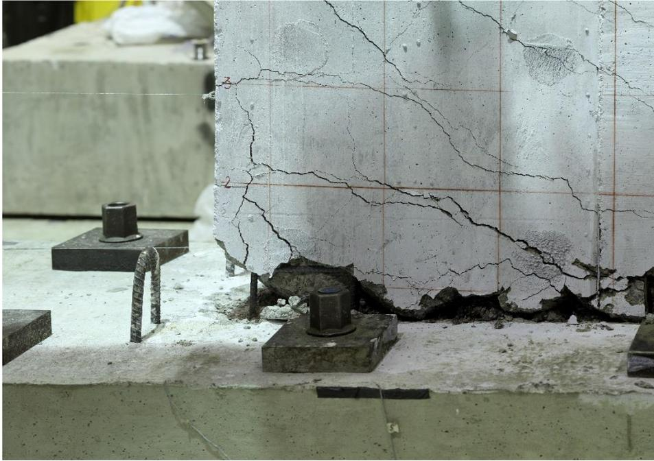
Figure E.24. Damage to SW3 at the end of testing
