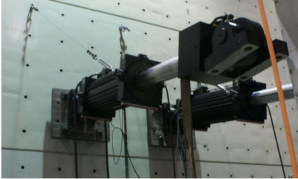
Figure C.50. MTS 243.90T actuators attached to the SEESL strong wall (pistons extended)
