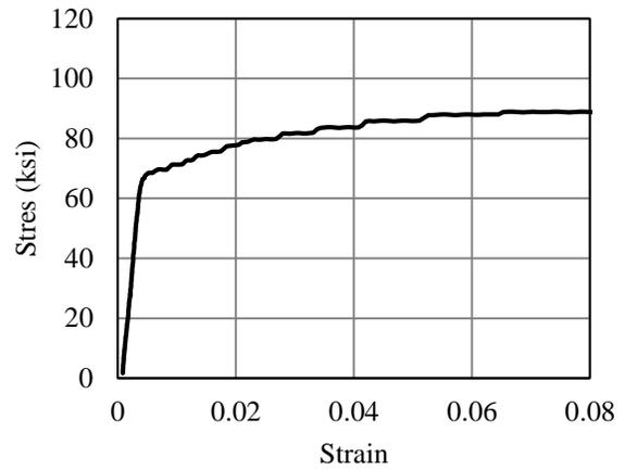
b) ASTM A706 rebar
