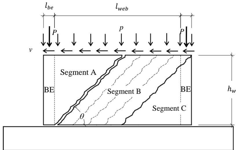
Figure 6.11. Different sections and idealized cracking pattern of a low aspect ratio rectangular RC wall with boundary elements
