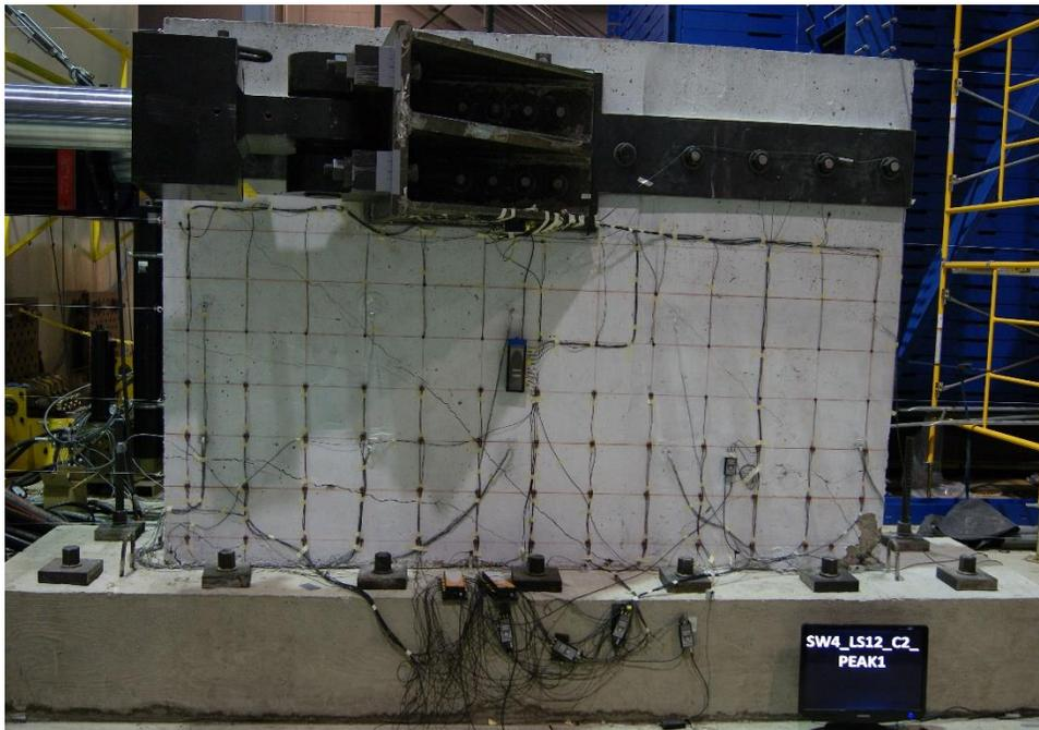
Figure E.29. Damage to SW4 at 1.08% drift ratio (peak strength)
