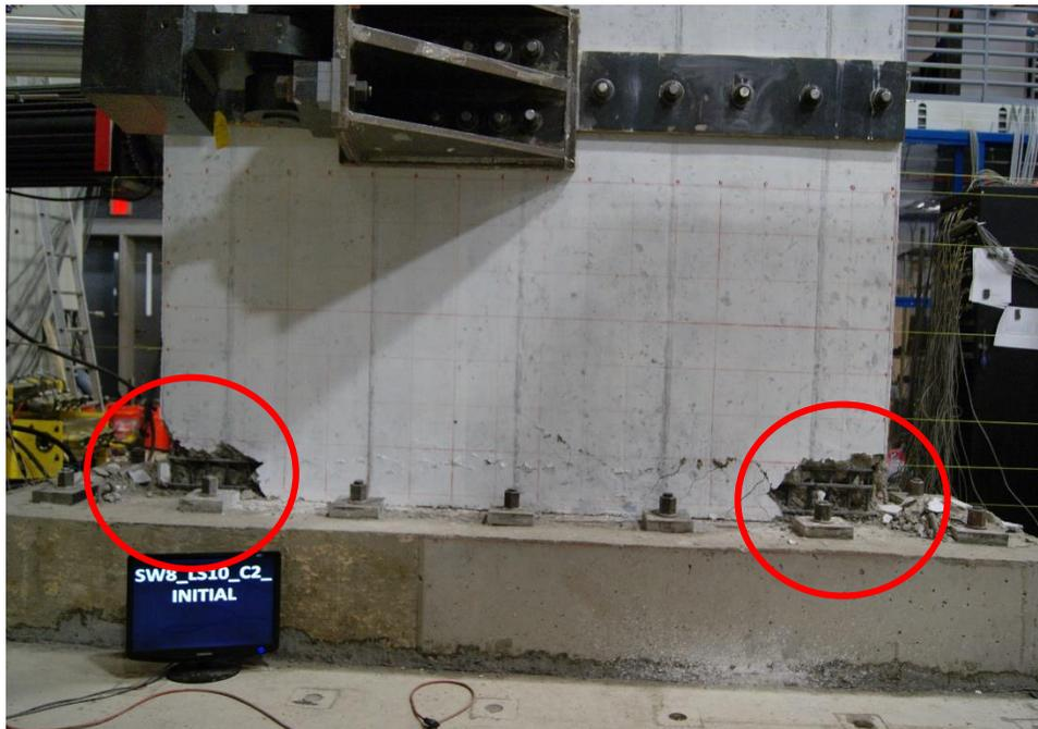
Figure 2.3. Diagonal compression failure
