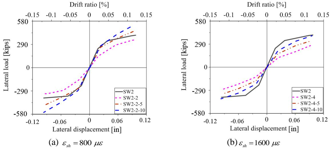
Figure 5.5. Cyclic backbone curves for RC walls
