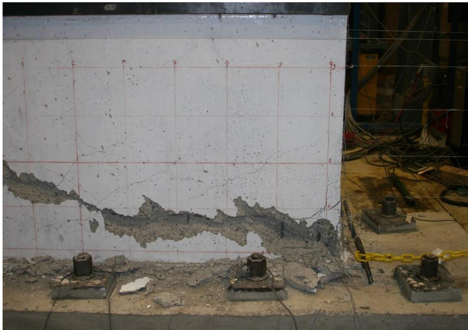
Figure E.42. Damage to SW5 at the end of testing
