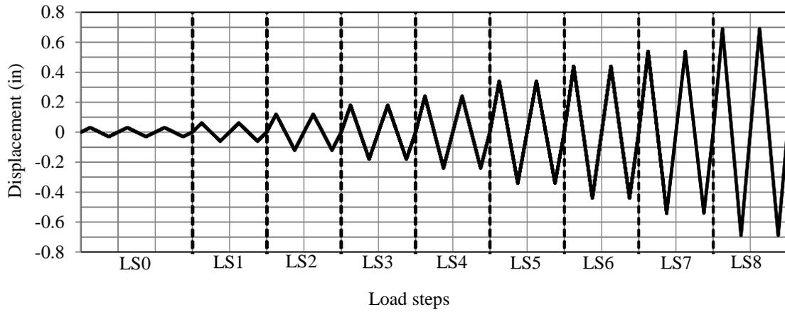
Figure D.16. Loading protocol for SW8
