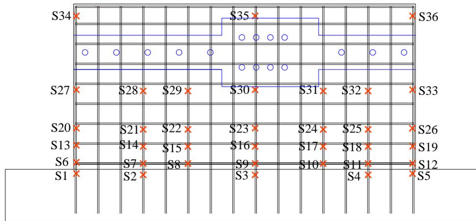
Figure C.18. Strain gages on the vertical reinforcements for SW6
