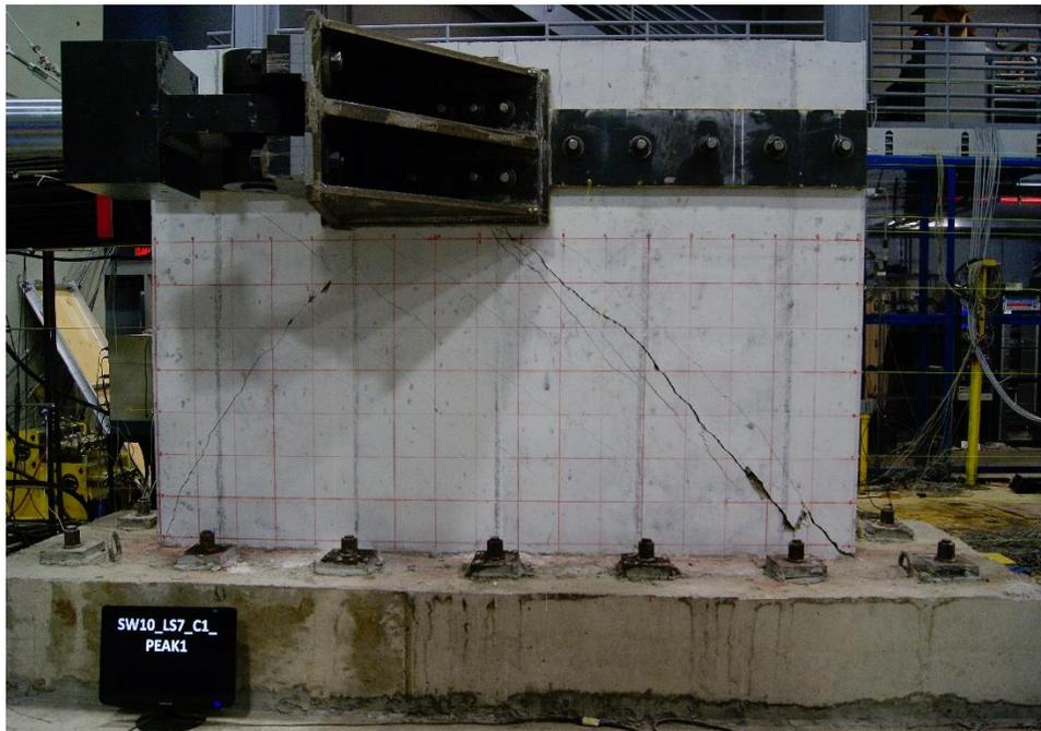
Figure E.85. Damage to SW10 at 0.93% drift ratio
