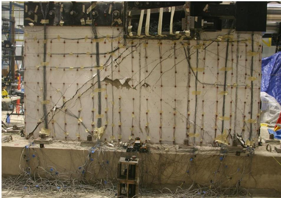
Figure E.89. Damage to SW10 at the end of testing
