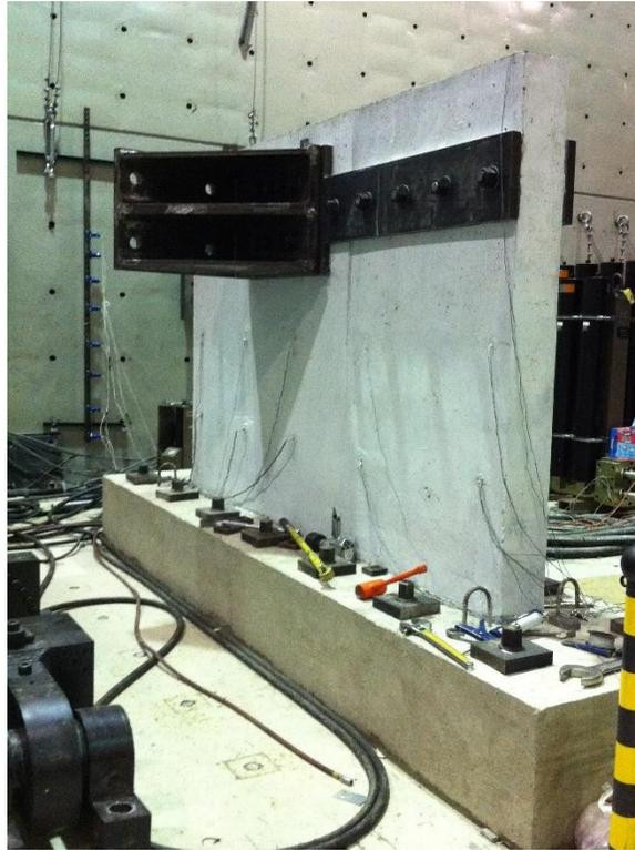
Figure 3.21. Loading bracket installation
