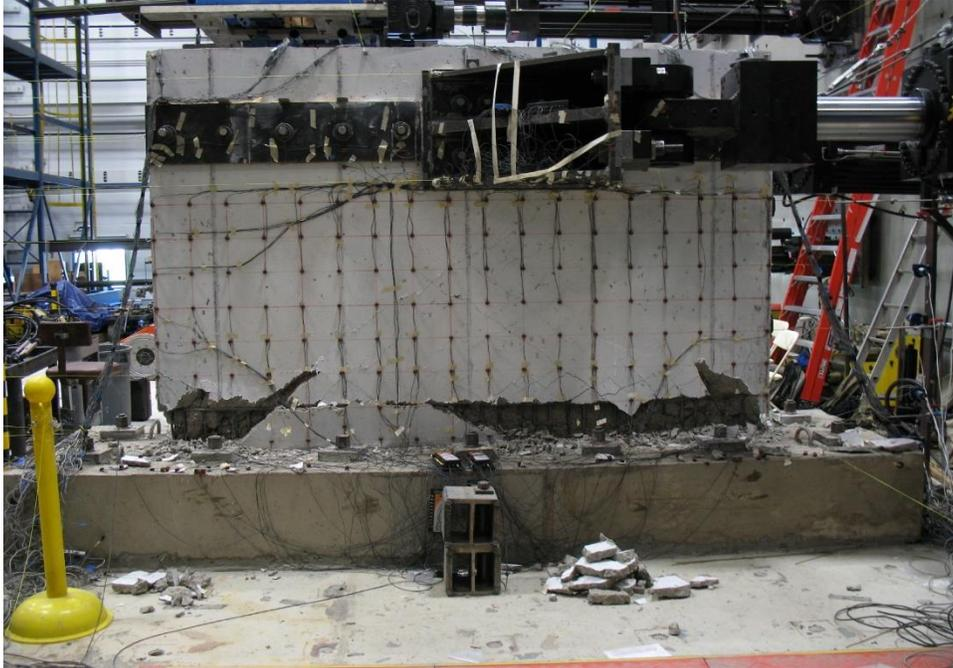
Figure E.81. Damage to SW9 at the end of testing
