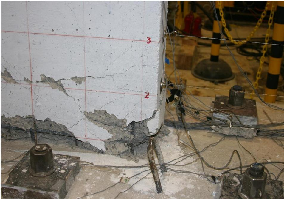
Figure E.48. Damage to SW6 at the end of testing
