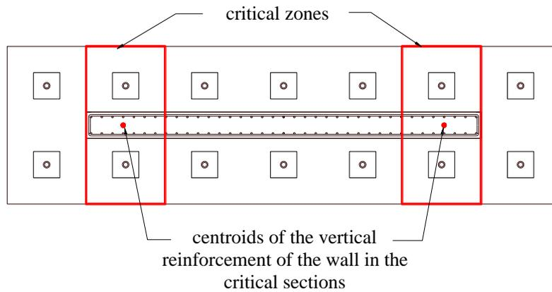
Figure B.1. Critical zones of the foundation of SW8
