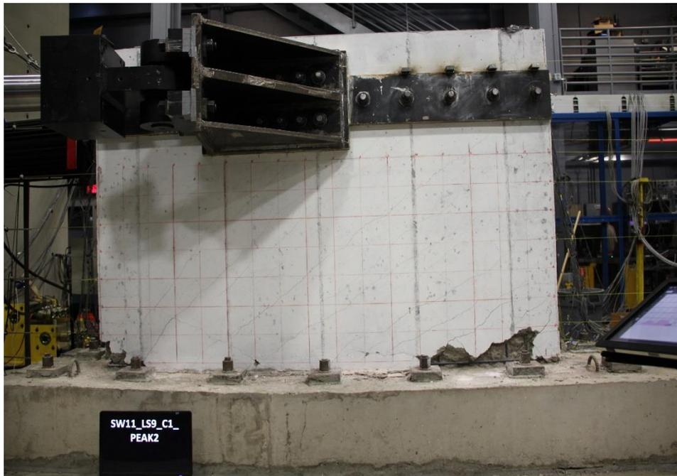
Figure E.94. Damage to SW11 at -1.75% drift ratio
