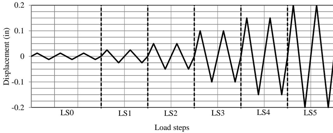
Figure D.12. Loading protocol for SW6
