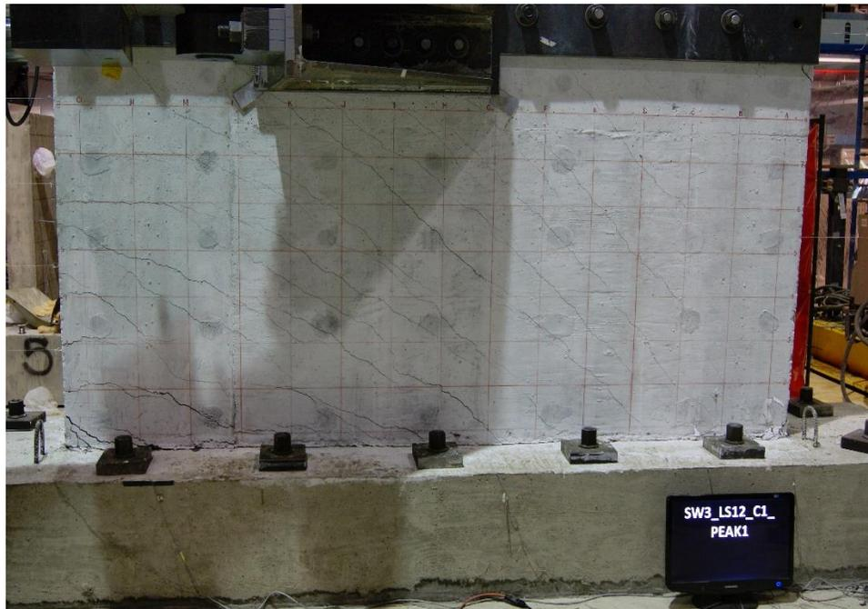
Figure E.21. Damage to SW3 at 2.09% drift ratio (peak strength)
