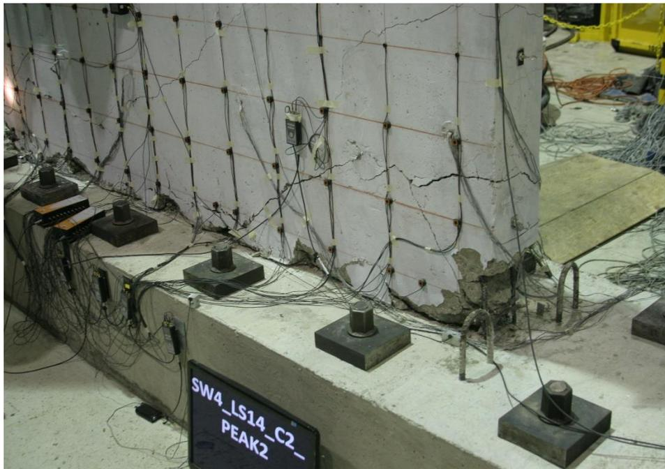
Figure E.33. Damage to SW4 at the end of testing
