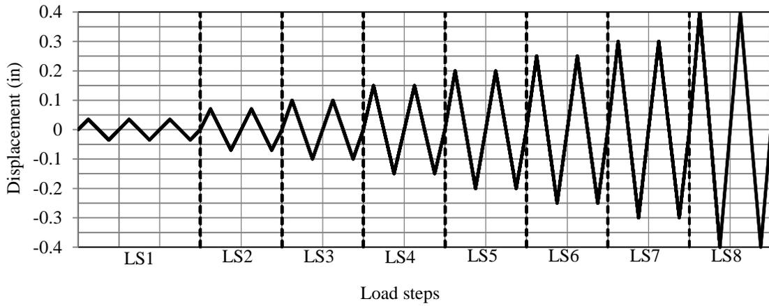
Figure D.6. Loading protocol for SW3
