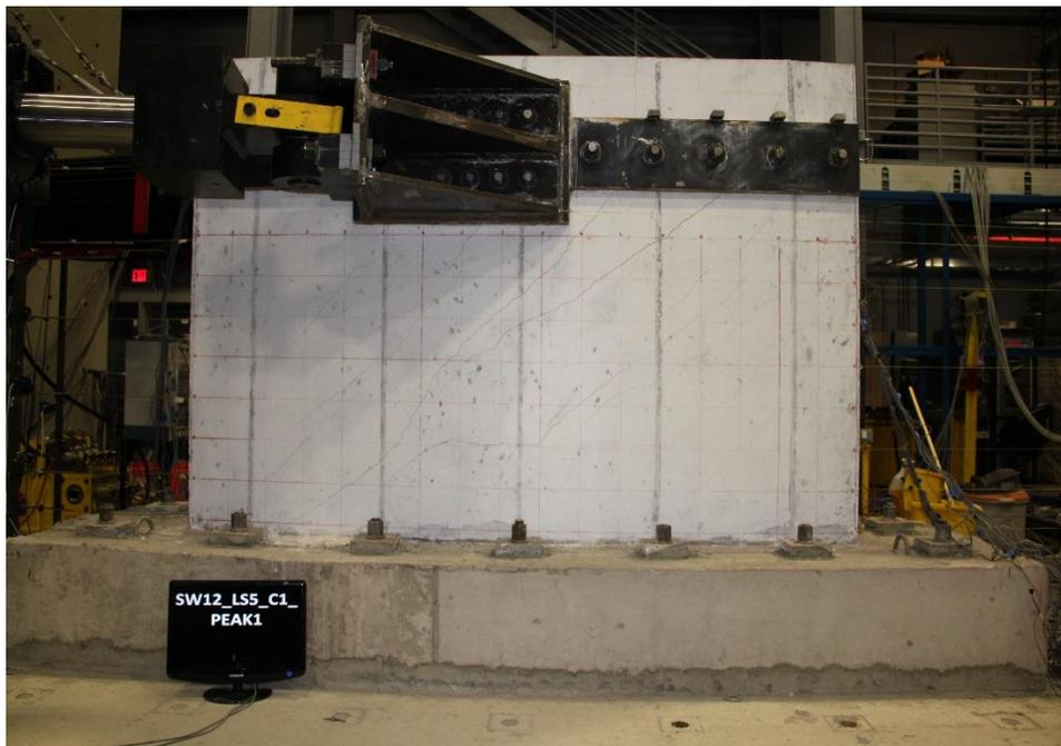
Figure E.100. Damage to SW12 at 0.54% drift ratio
