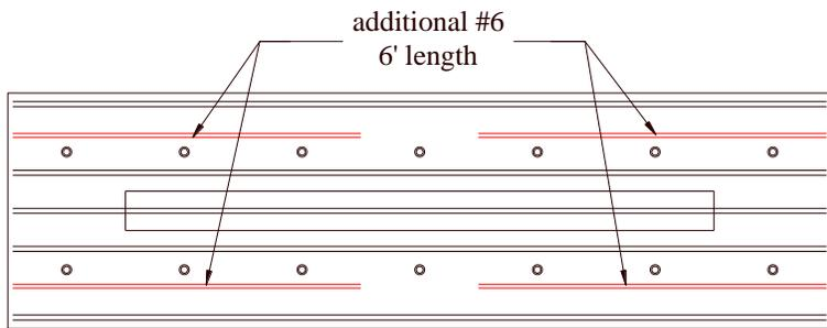
Figure B.6. Supplemental longitudinal reinforcement on the top section of rebar cage (SW9-SW12)
