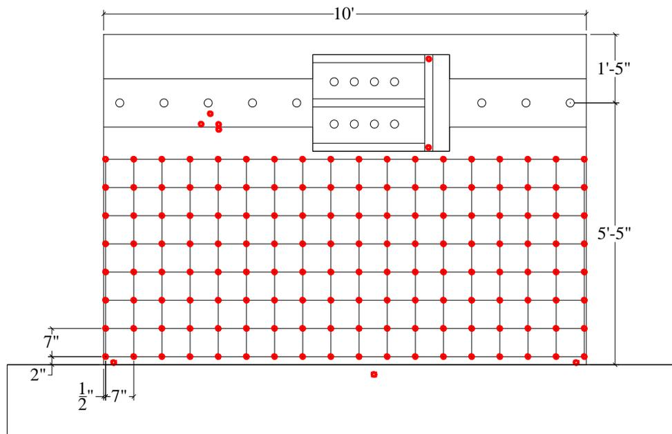
Figure C.10. Krypton LED sensors for SW10
