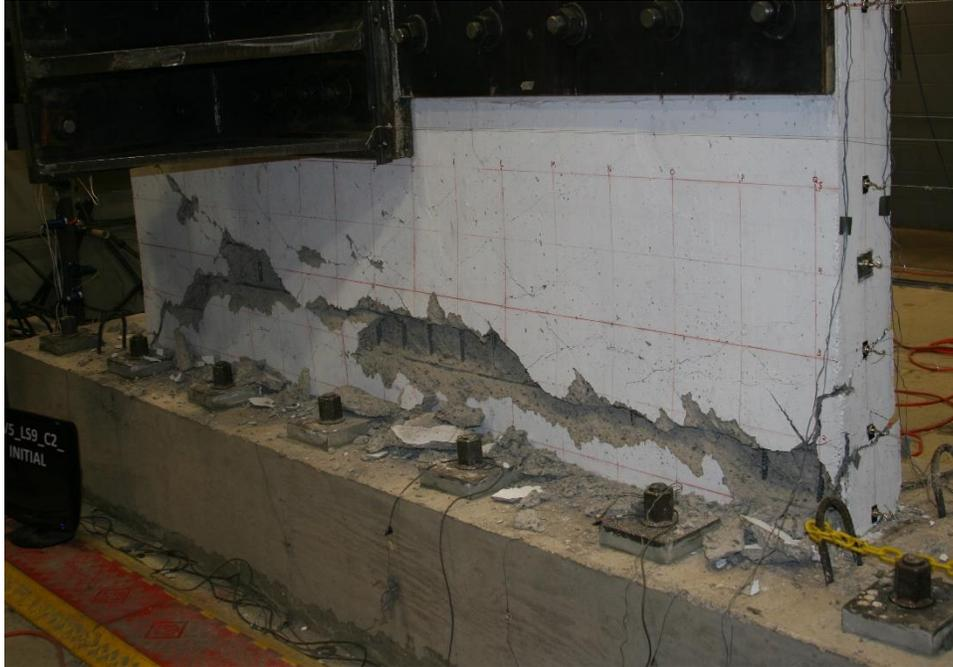
Figure E.41. Damage to SW5 at the end of testing
