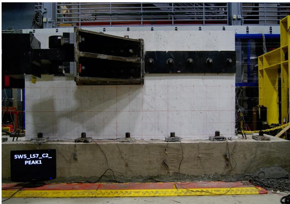
Figure E.36. Damage to SW5 at 0.67% drift ratio
