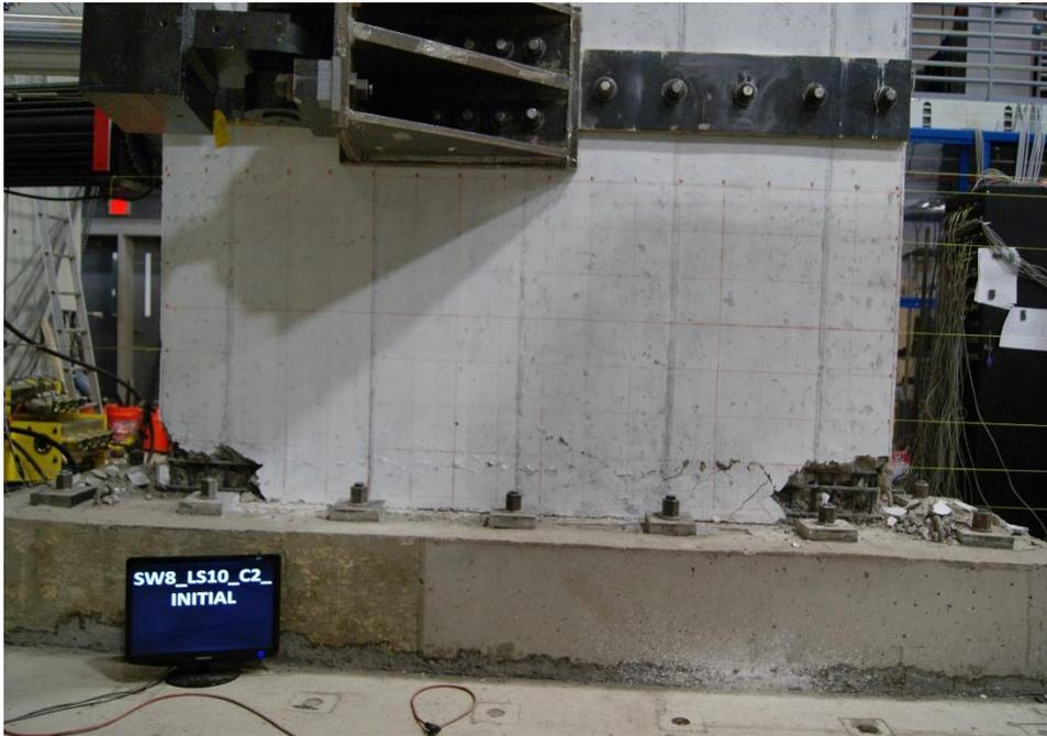
Figure E.70. Damage to SW8 at the end of testing
