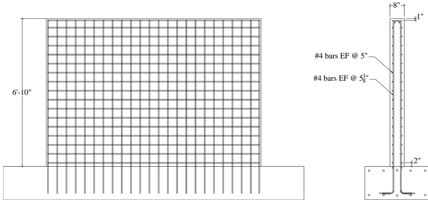
Figure A.8. Reinforcement details for SW2
