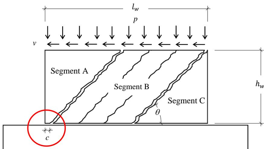
Figure 6.7. Different sections and idealized cracking pattern of a low aspect ratio rectangular RC wall without boundary elements
