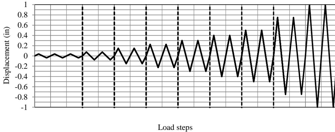
Figure D.2. Loading protocol for SW1
