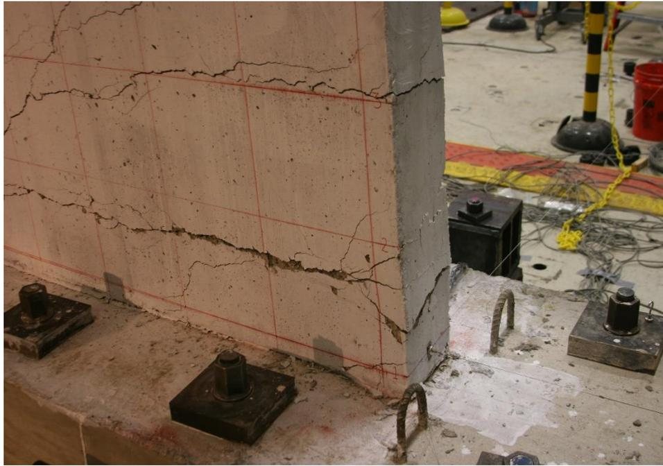
Figure E.6. Damage to SW1 at 1.67% drift ratio
