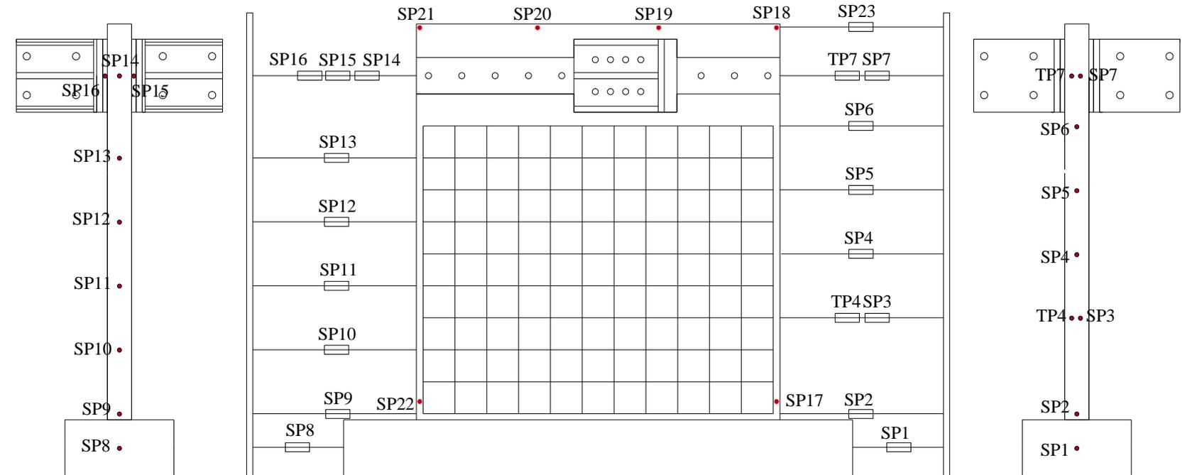
Figure C.37. In-plane and out-of-plane string potentiometers and Temposonics for SW1
