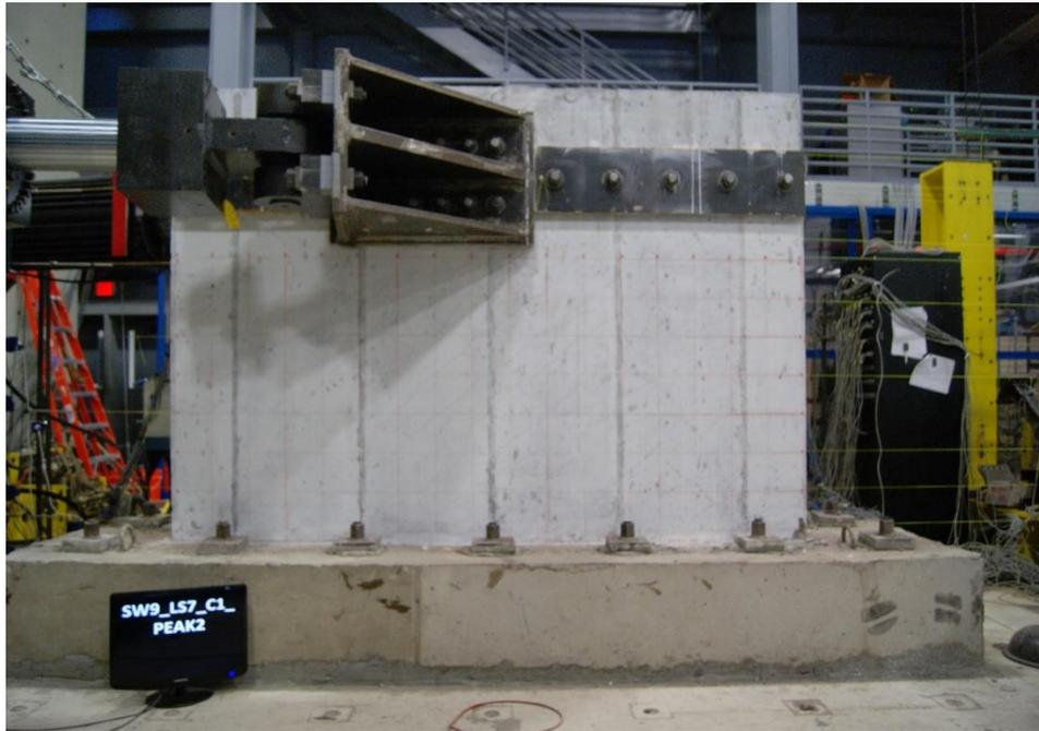
Figure E.74. Damage to SW9 at -0.78% drift ratio (peak strength)
