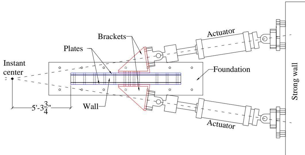
Figure 3.23. Plan view of typical specimen setup
