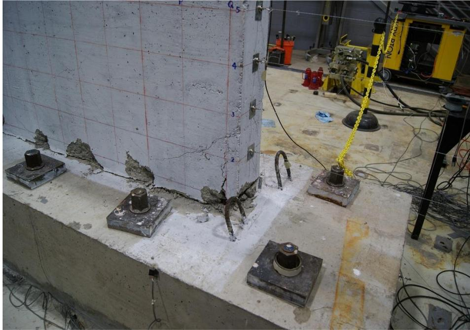
Figure E.55. Damage to SW7 at the end of testing
