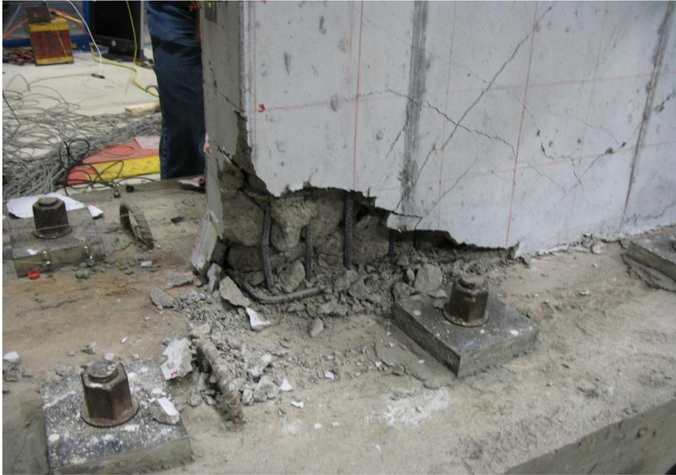
Figure E.77. Damage to SW9 at the end of testing
