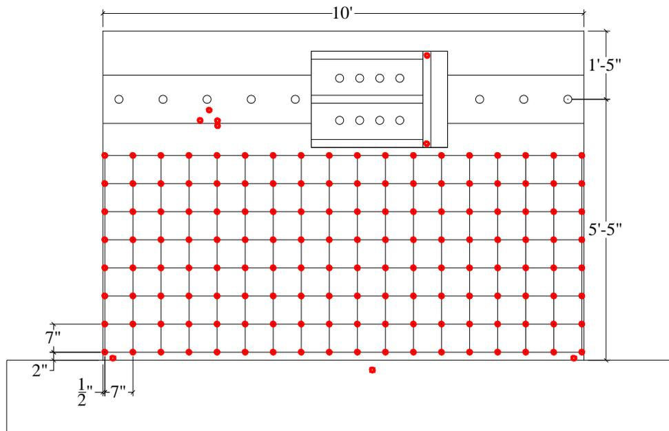
Figure C.8. Krypton LED sensors for SW8
