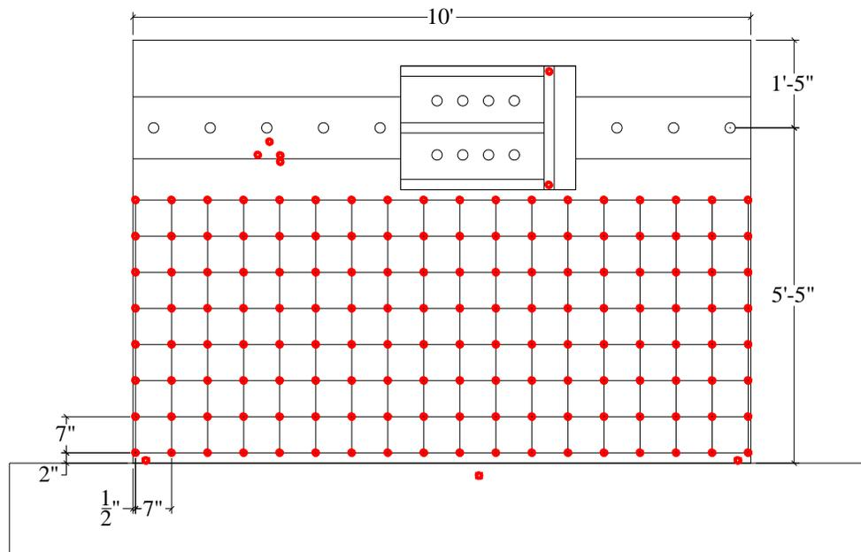
Figure C.9. Krypton LED sensors for SW9
