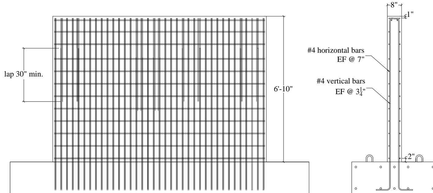
Figure A.15. Reinforcement details for SW9
