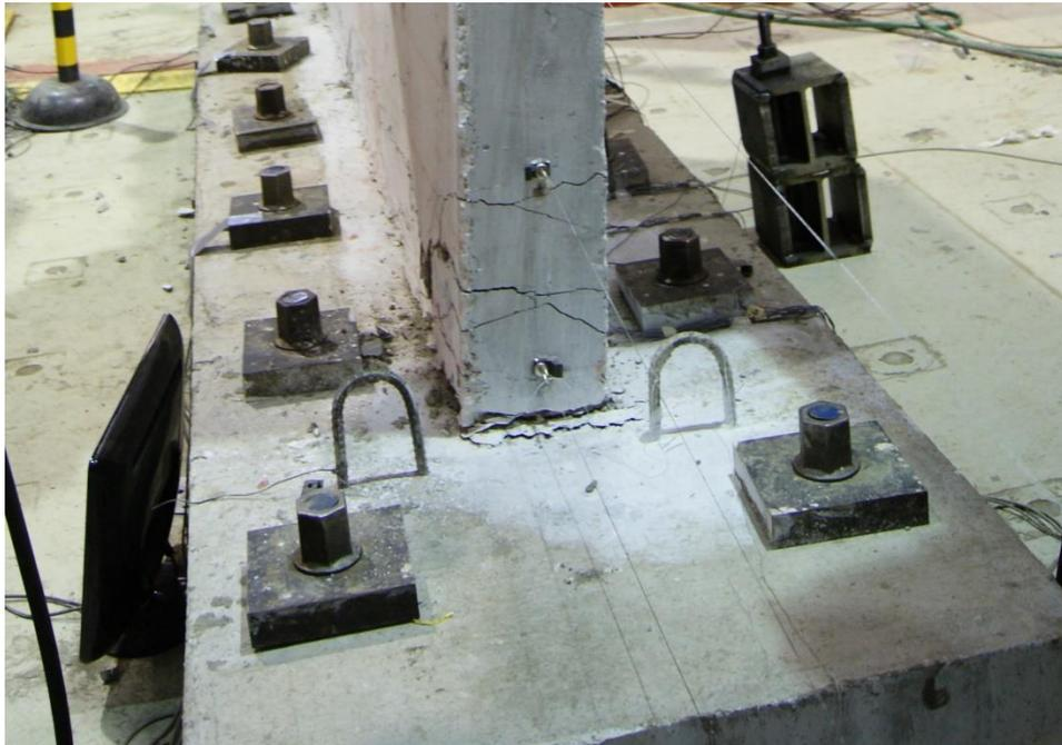
Figure E.17. Damage to SW2 at the end of testing
