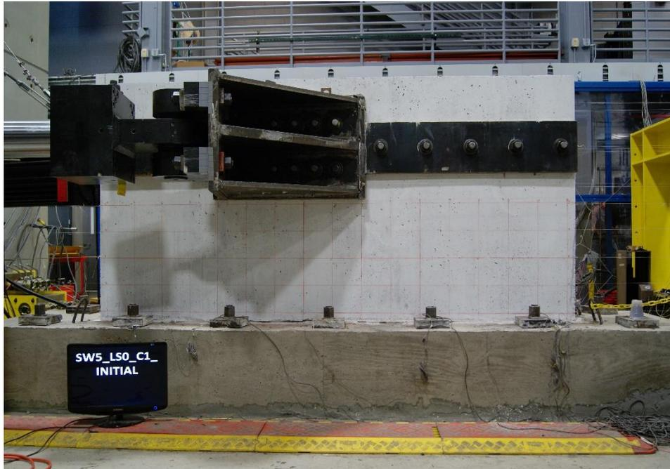
Figure E.35. SW5 before testing
