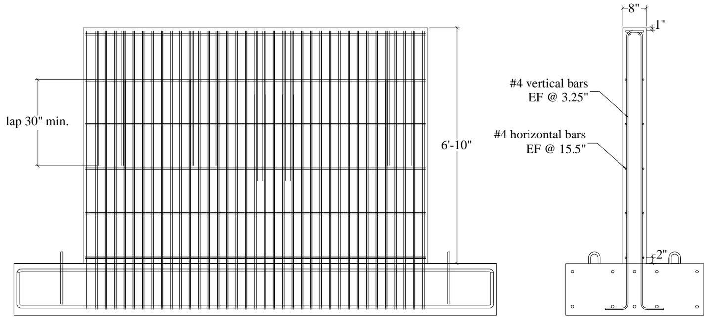
Figure A.16. Reinforcement details for SW10
