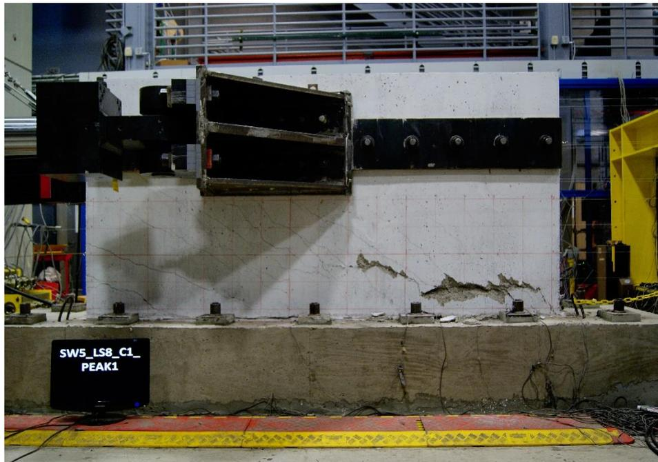
Figure E.38. Damage to SW5 at 0.89% drift ratio (peak strength)
