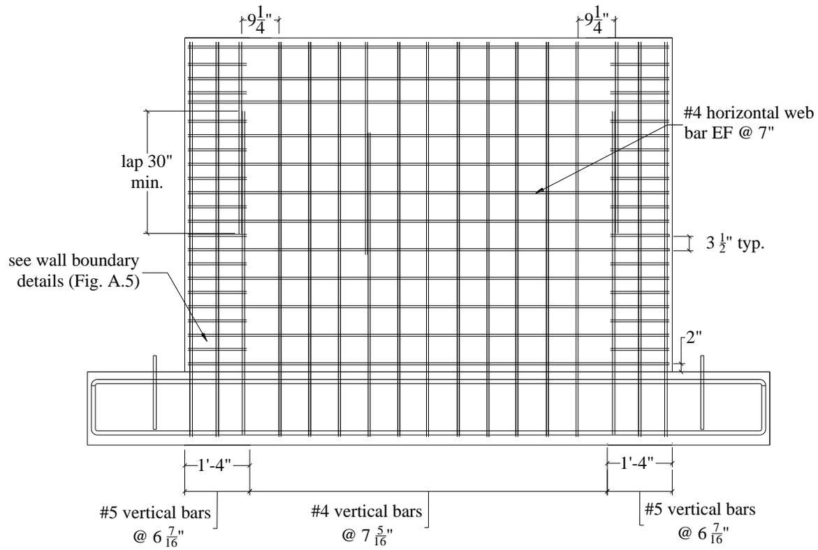
Figure A.17. Reinforcement details for SW11
