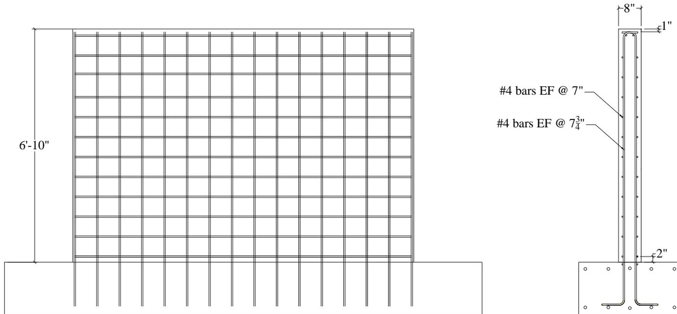
Figure A.9. Reinforcement details for SW3
