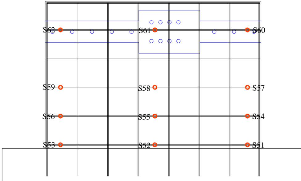
Figure C.28. Strain gages on the horizontal reinforcements for SW4
