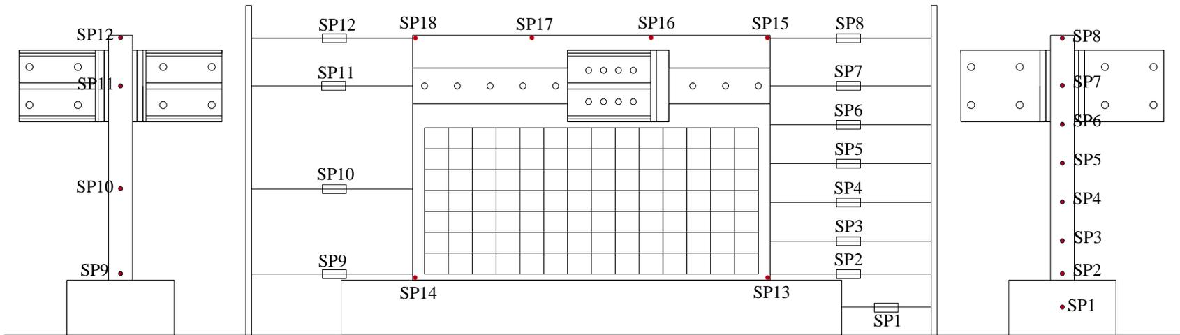
Figure C.38. In-plane and out-of-plane string potentiometers and Temposonics for SW2
