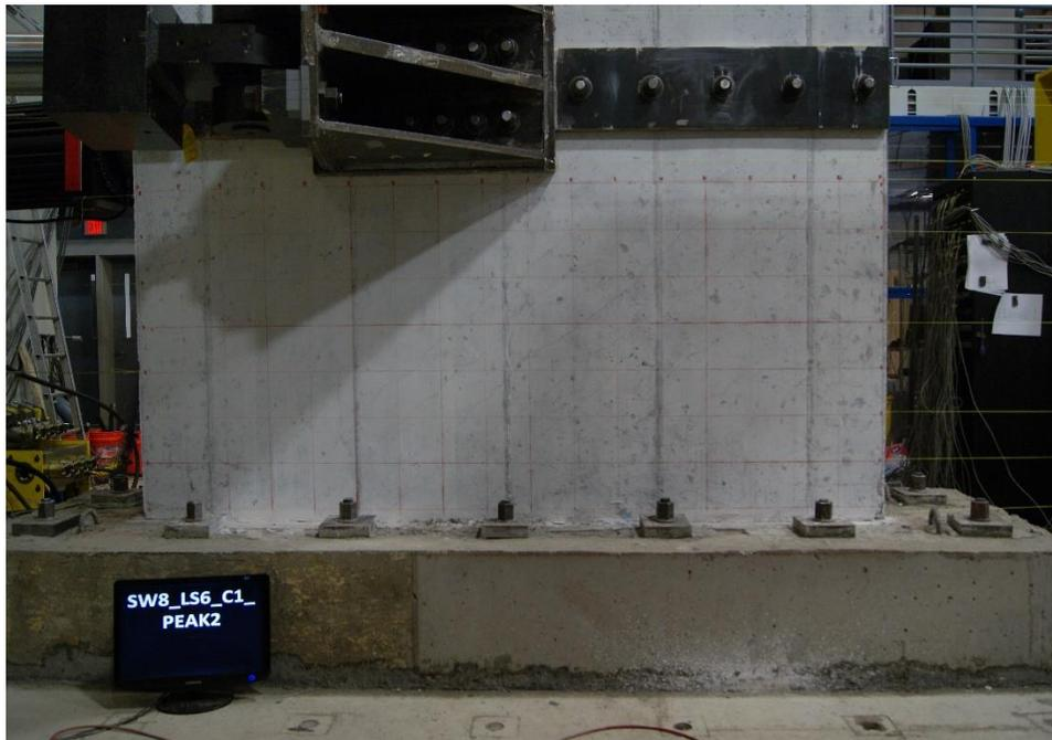
Figure E.61. Damage to SW8 at -0.65% drift ratio
