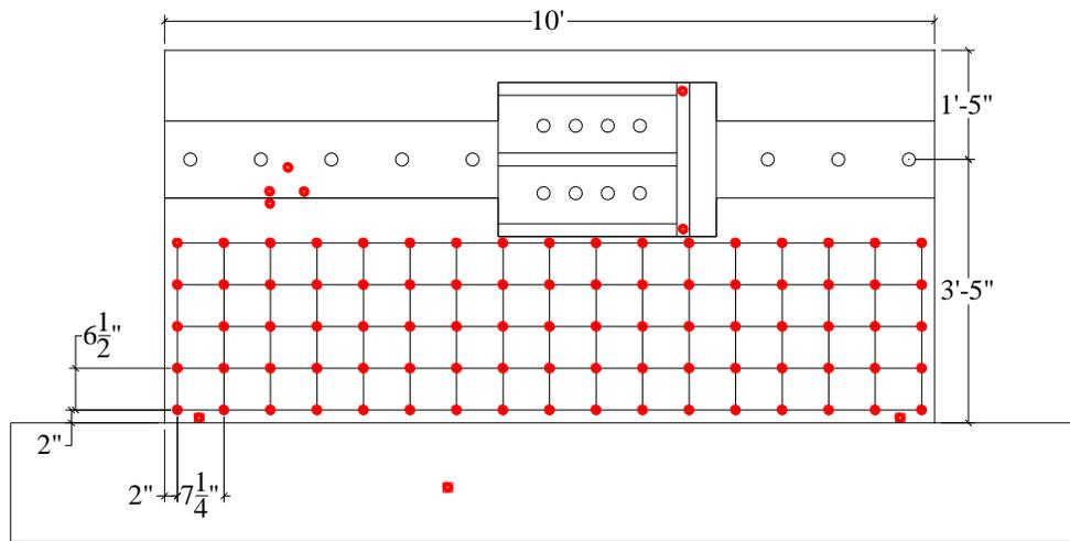
Figure C.6. Krypton LED sensors for SW6
