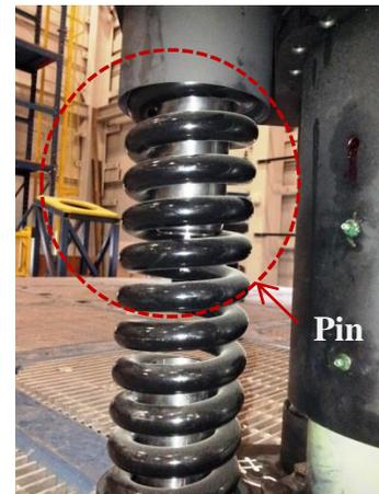
**Figure 3-7 Detail of Spring-Damper Unit for Increasing Shear Spring Stiffness**
