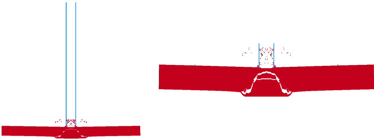
(a) Spalling of concrete and perforation of panel
