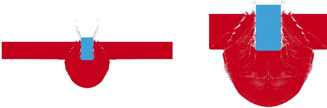
(a) Perforation of panel
