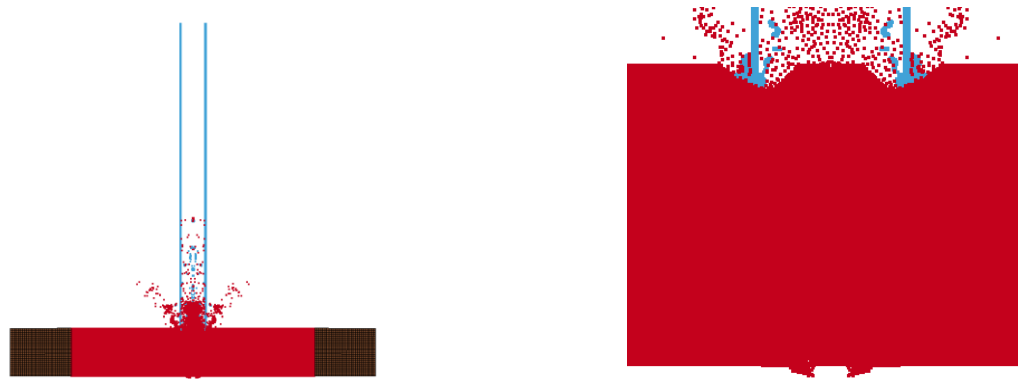
(a) Spalling of concrete on front face
