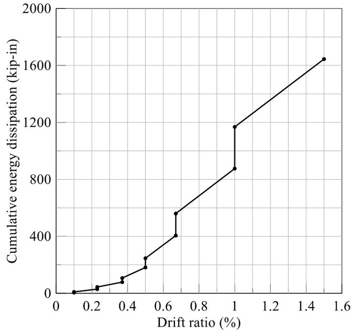
Figure 2-14: Cumulative energy dissipation, CNSC1
