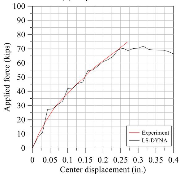
Figure 3-4: Experimental (Bresler) and LS-DYNA results
