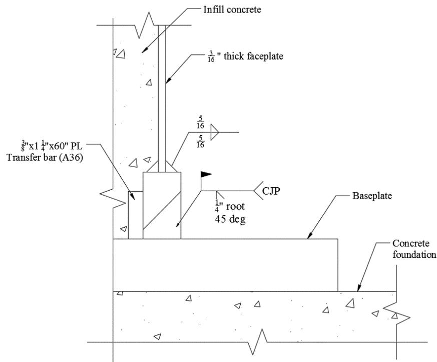
Figure 2-1: Faceplate-to-baseplate connection (courtesy of Purdue University)
