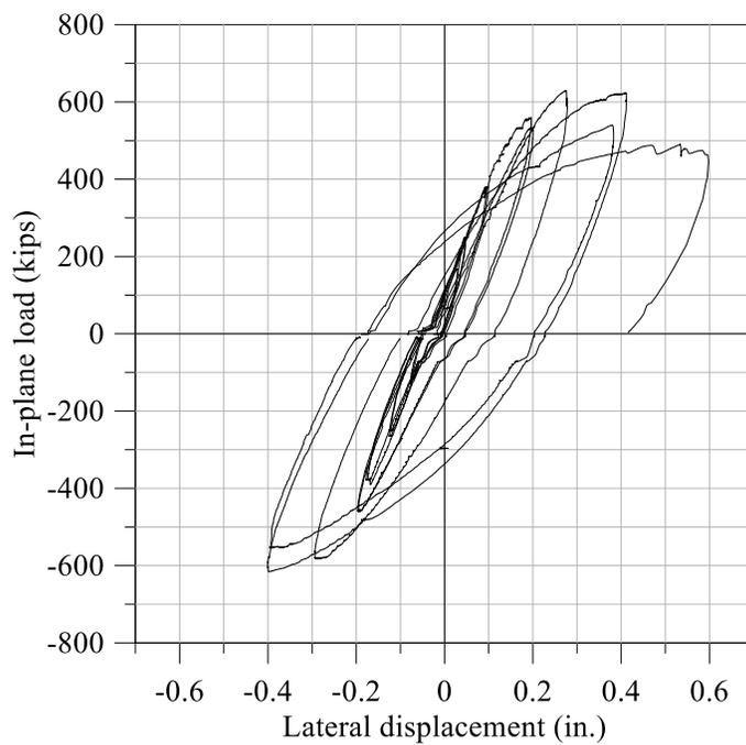
Figure 2-19: In-plane force-displacement relationship, CNSC2
