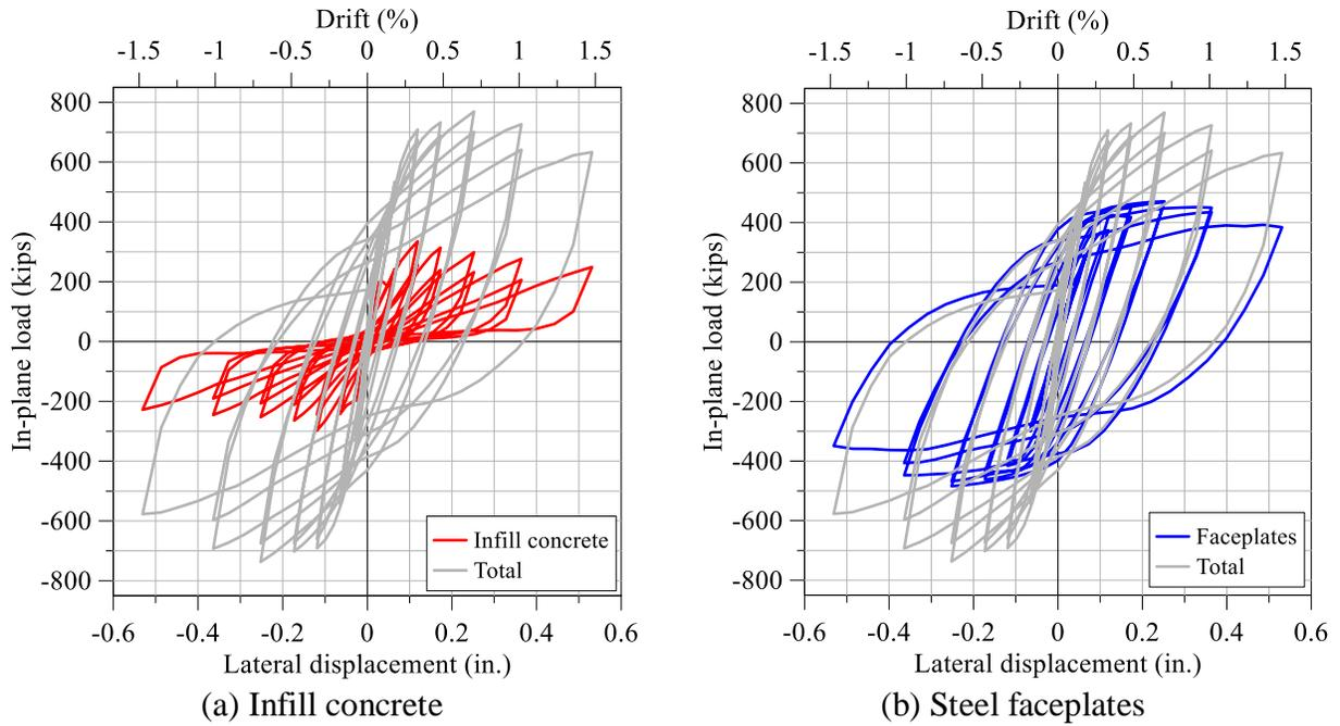
Figure 3-18: LS-DYNA-predicted IP cyclic force-displacement relationships, CNSC1
