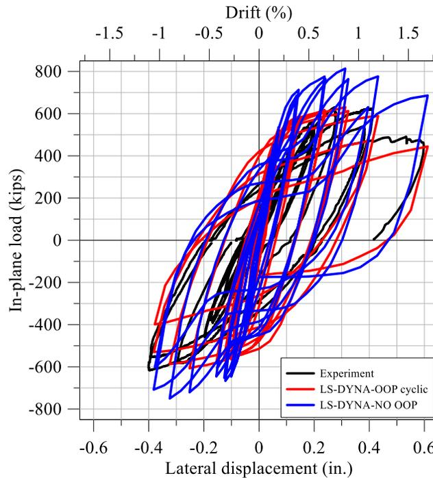
Figure 3-31: IP force-displacement relationships, CNSC2
