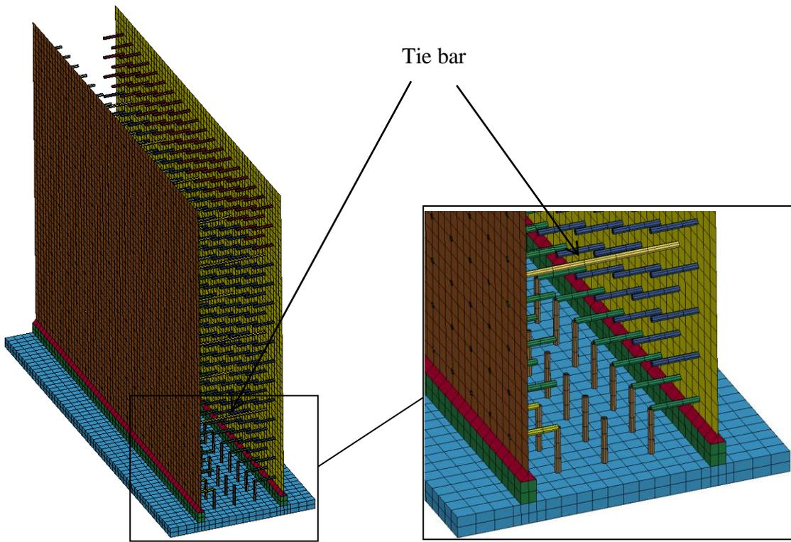
Figure 3-8: CNSC1 and CNSC3 tie bar details
