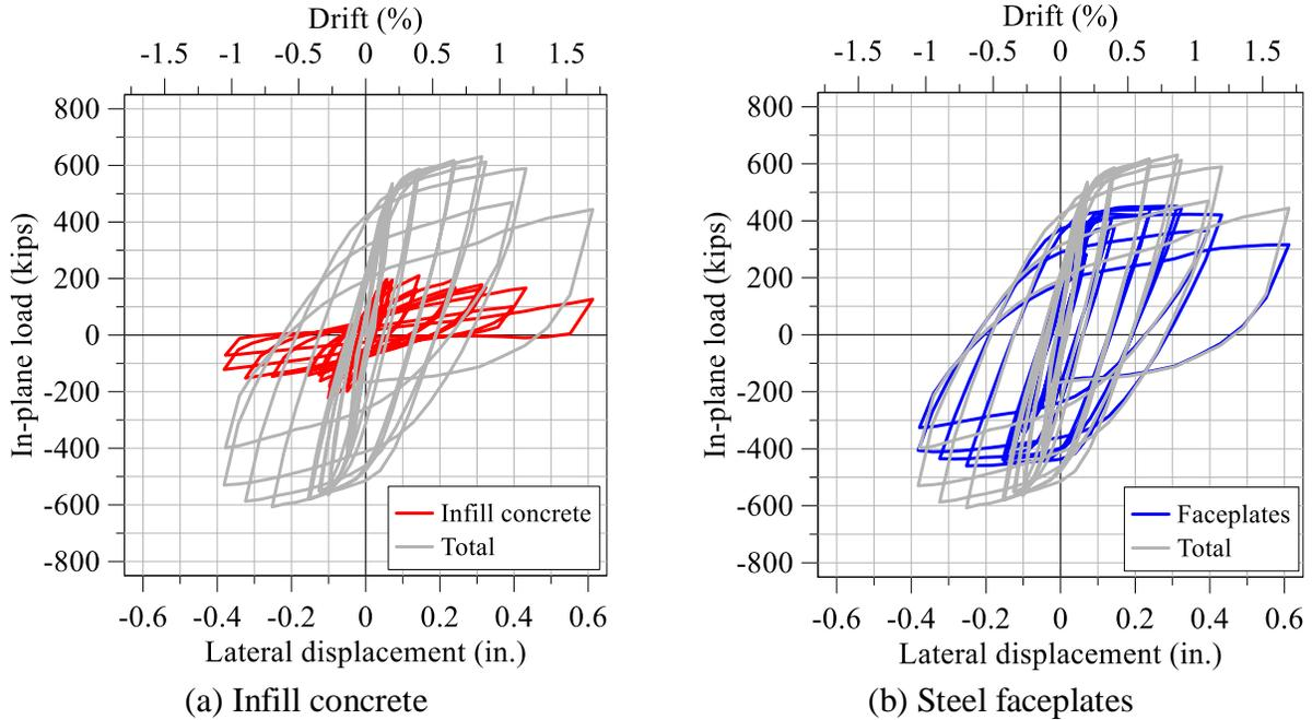
Figure 3-29: LS-DYNA-predicted IP cyclic force-displacement relationships, CNSC2
