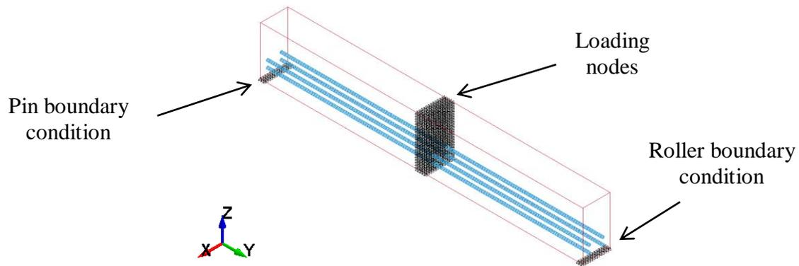
Figure 3-3: LS-DYNA loading and boundary conditions
