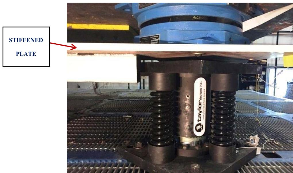
Figure 4-8 View of Isolation System with Installation Method that Restrains Rocking
