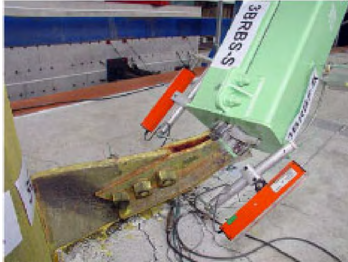
Figure 2-38 Buckling of a BRB gusset plate (Tsai et al, 2008)
