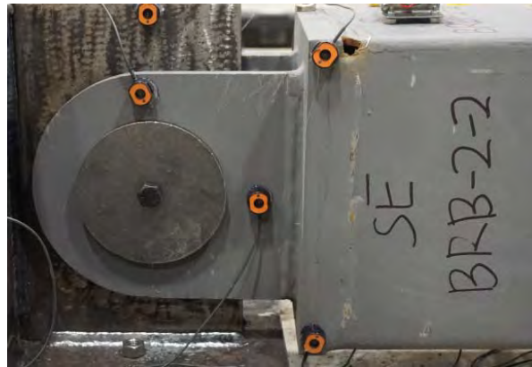
Figure 8-15: Side view of BRB-2 connecting to the gusset plate-2 with pin, washer, and bolts
