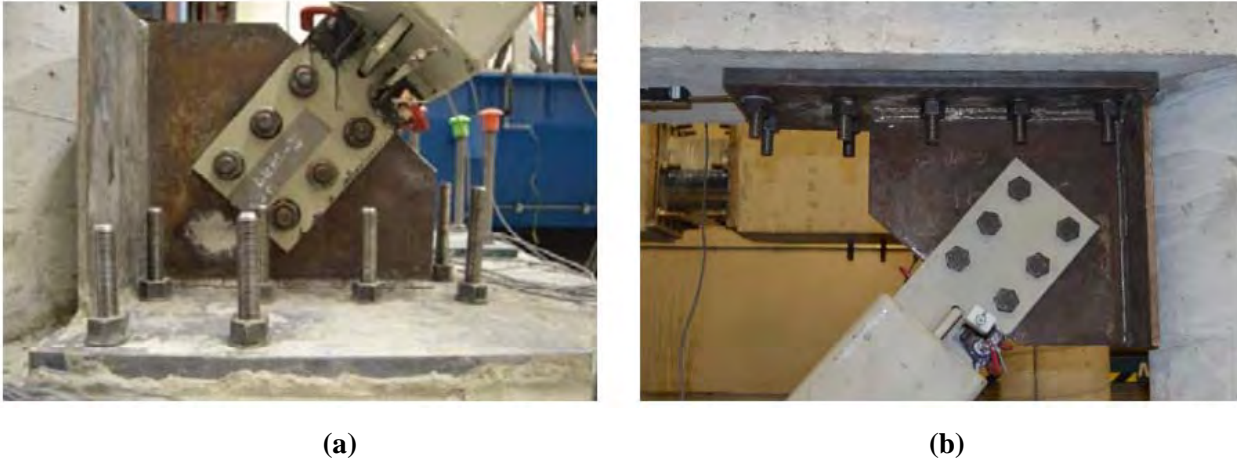
Figure 2-22 Gusset plate to bridge bent connection: (a) bottom connection; (b) top connection
