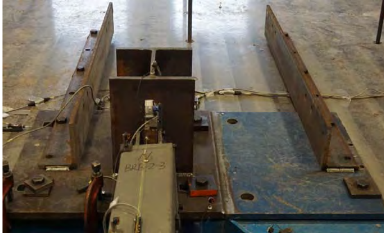
Figure 8-68 Reaction block on the shake table with modification of anchorage using bolted angles
