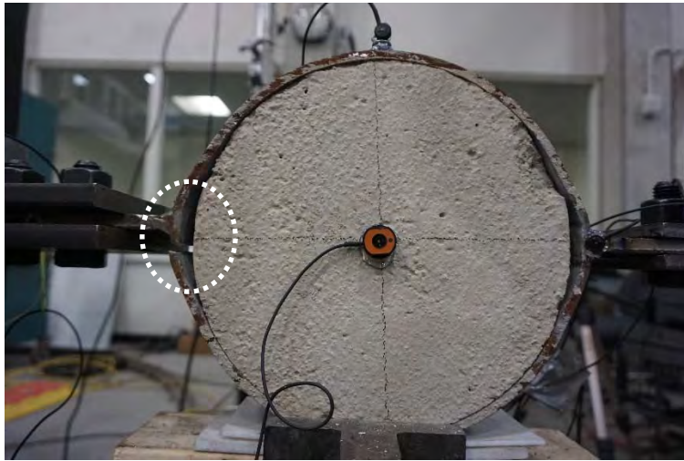
Figure 6-69 Failure of specimen D16L5-2
