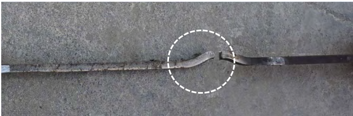
Figure 9-5 Part of the core plate of BRB-2-4 with the fracture
