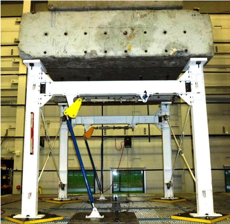
**Figure 4-1 Model Structure on Earthquake Simulator (shown configuration is Model 2, R-R)**
