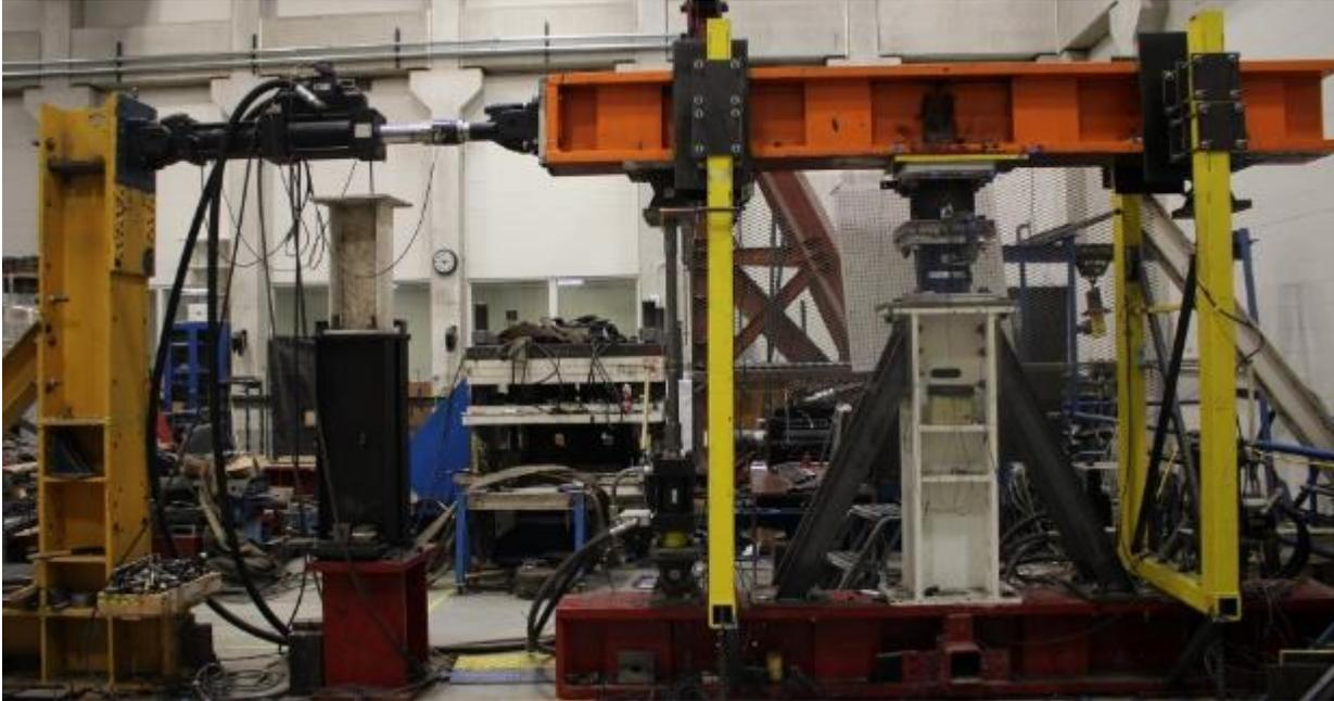
**Figure 6.10: Photograph of Single Bearing Testing Machine**
