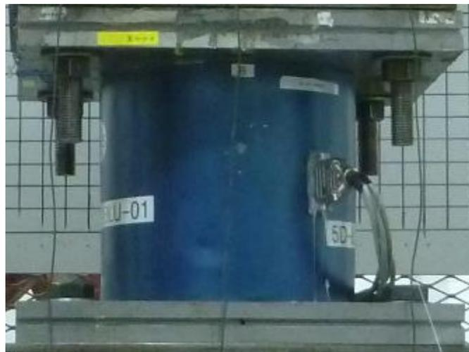
**Figure 6.12: Five channel load cell**
