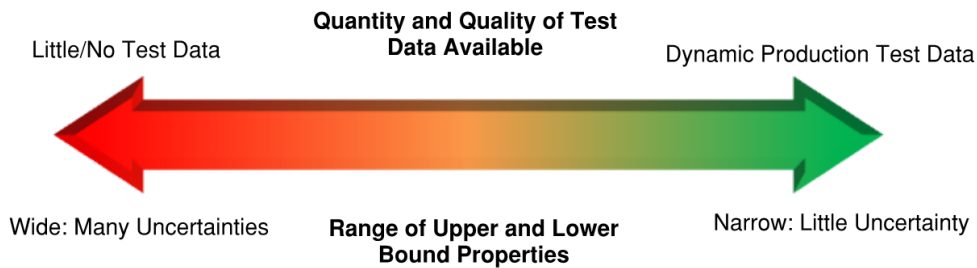
Figure 5-3 Indicative Continuum of Quantity and Quality of Test Data vs. Range in Isolation System Properties
