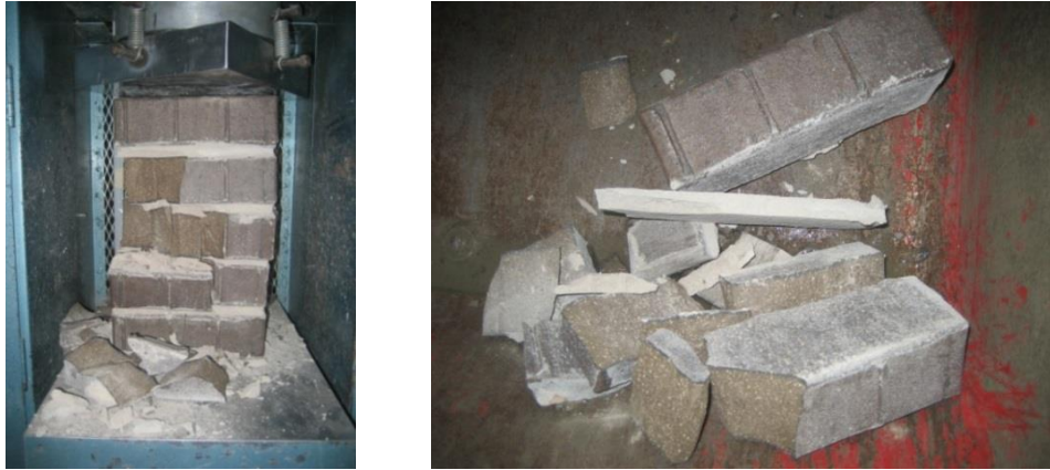
Figure 8-13. A damaged masonry prism after compression test
