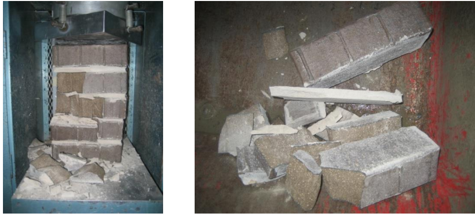
Figure 5-11. The damaged specimen after compression test
