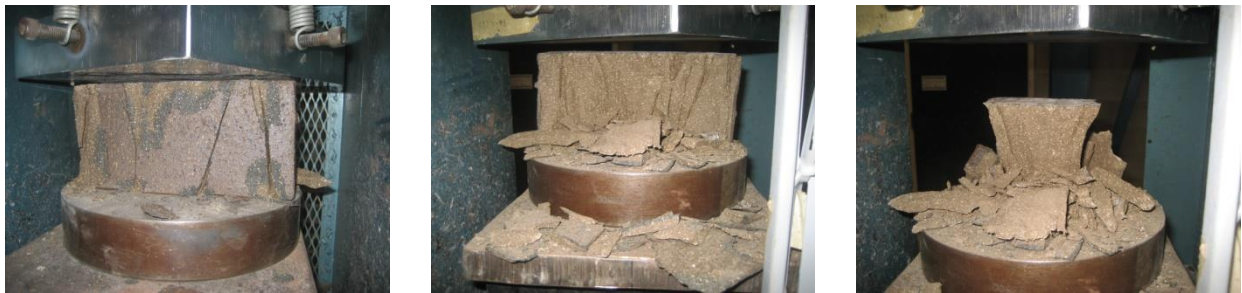
Figure 8-10. A damaged high strength brick after uniaxial compression test
