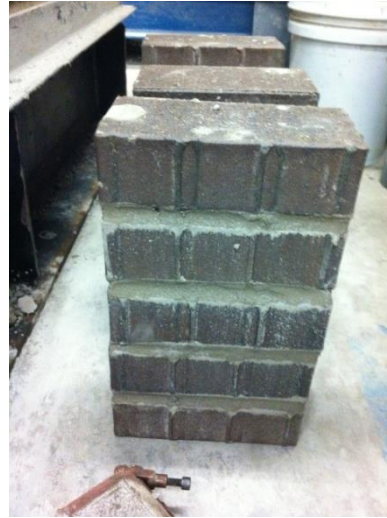
(b) Compression test
