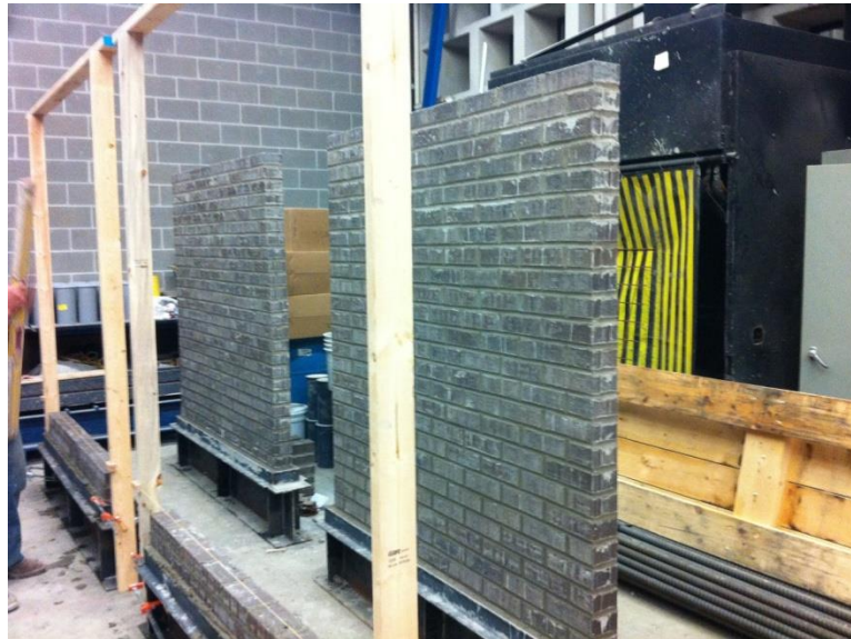
Figure 8-2. Wall type II (the first row of brick is buried into the mortar)
