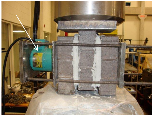
Figure 8-7. Test setup for measuring the shear properties
