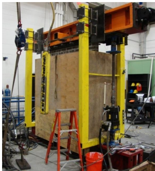
Figure 8-56. Test set-up for out-of-plane load
