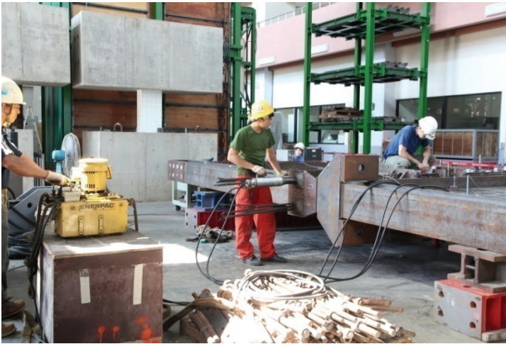
FIGURE 9-1e Specimen NZ construction: Step 5 – install HBE PT strands
