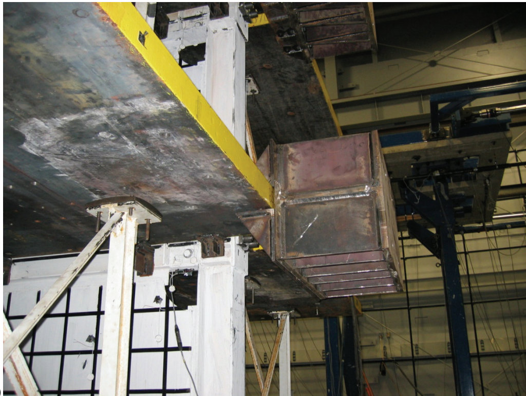
FIGURE 5-5 Actuator shoe: (a) Global view; (b) Close-up view
