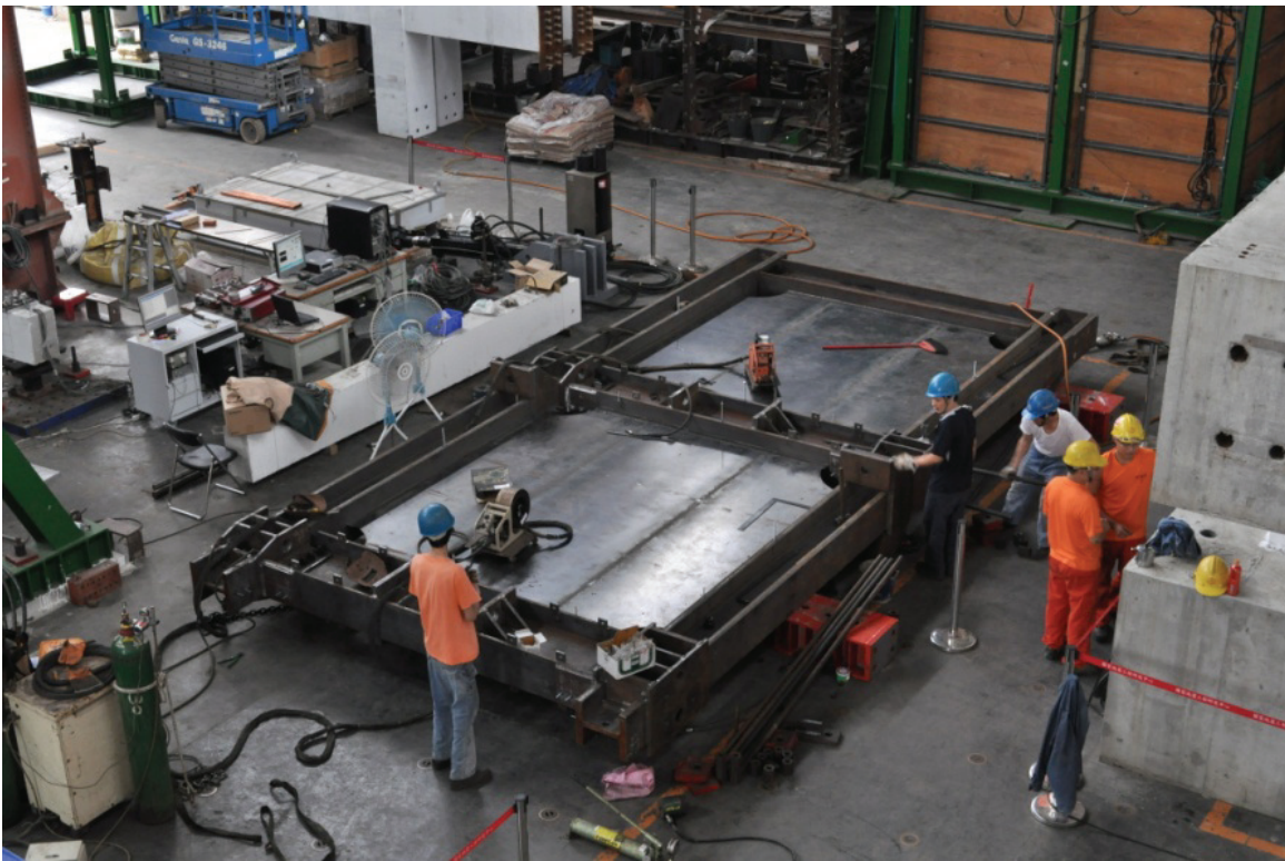
FIGURE 9-1d Specimen NZ construction: Step 4 – remove temporary HBE PT bars
