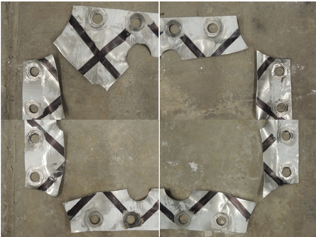
FIGURE 7-69 Post-testing bolt holes at infill web plate corners
