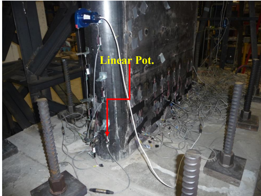
Figure 4-34 Liner Potentiometers Arrangement
