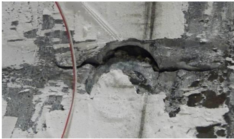
Figure 5-30 Fracture Propagation from Tie Bars Circumference in CFSSP-NB2 at 3.0% Drift
