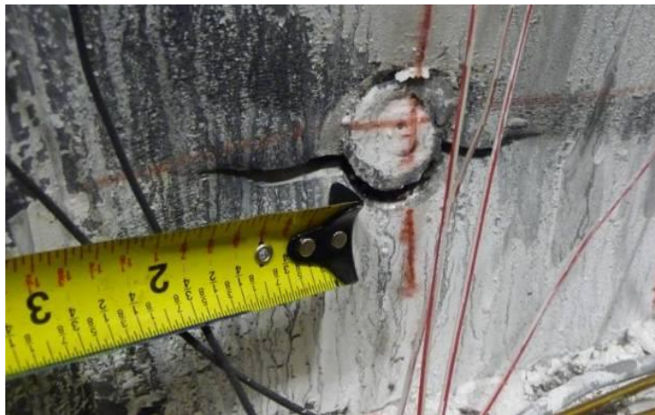
Figure 5-46 Fracture Propagation at Specimen CFSSP-B1 at 3.33% Drift
