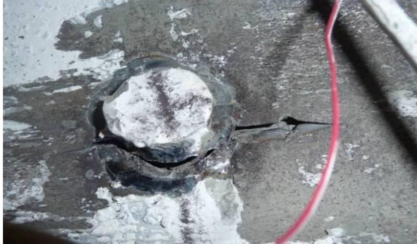
Figure 5-61 Propagation of Cracks at Outer Tie Bars in Specimen CFSSP-B2 at 4% Drift
