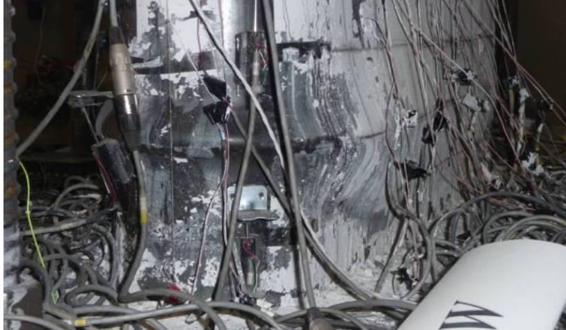
Figure 5-29 Propagation of Local Buckling in Specimen CFSSP-NB2 at 3% Drift
