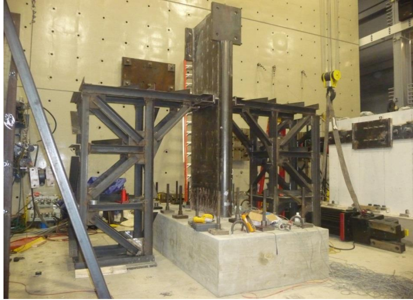
Figure 4-29 Tested CFSSP-Wall Specimen after Erection of Lateral Restraint System
