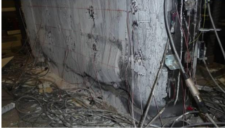
Figure 5-47 Fracture Propagation Pattern in Specimen CFSSP-B1 at 4% Drift
