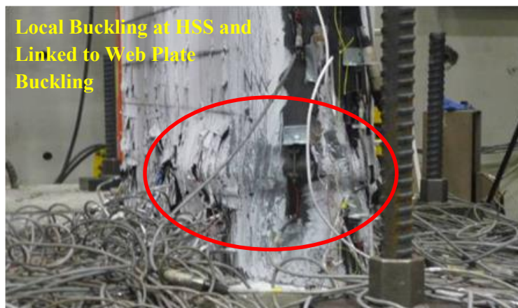
Figure 5-9 Local Buckling of the HSS Part at 2.4% Drift
