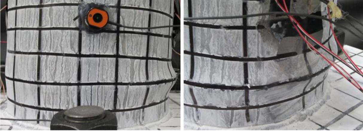
**Figure 4- 26 Local Buckling at the Base of Specimen S2**
