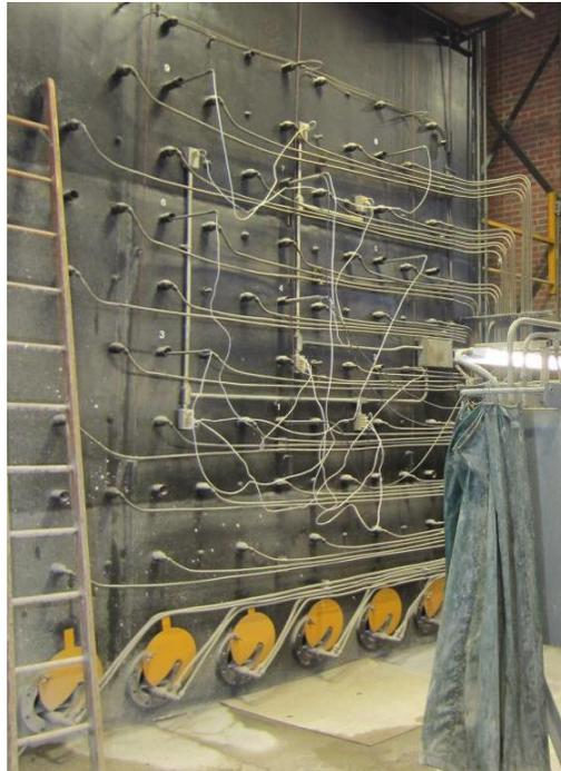
**Figure 5- 7 Wires Carrying Temperature Data Connected to the Channels at the Back of the Furnace Wall**
