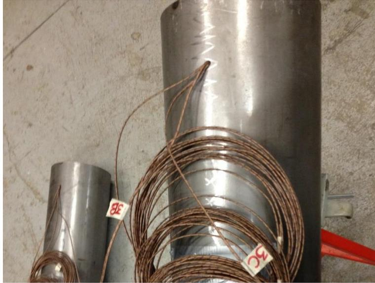
**Figure 4- 14 Thermocouple Wires Coming out of the Specimens**
