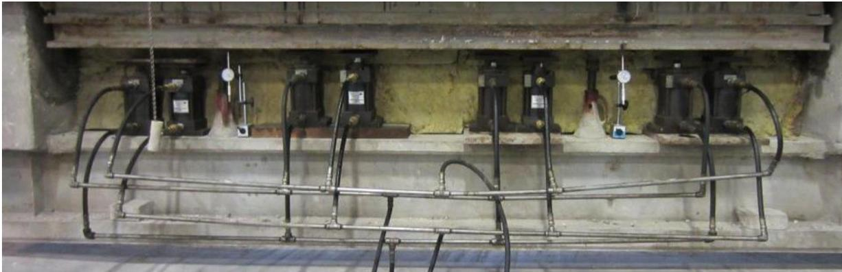
**Figure 5- 9 Mechanical Dial Gauges Placed under the Bottom Beam**
