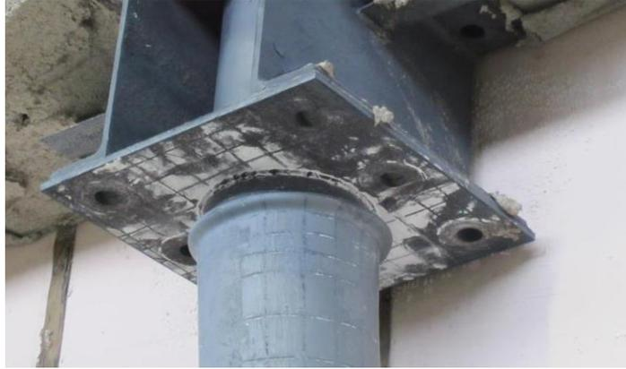
**Figure 5- 23 Local Buckling of Specimen S2 Close to the Top Beam of the Furnace**
