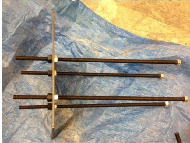
**Figure 4- 15 Threaded Rods fixed on the Cap Plate to Be Embedded in Concrete**
