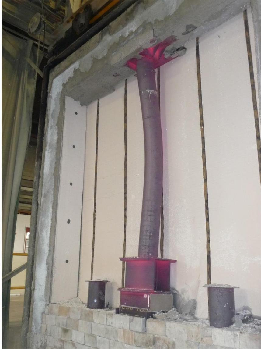
**Figure 5- 20 Out of Plane Global Buckling of Specimen S1**
