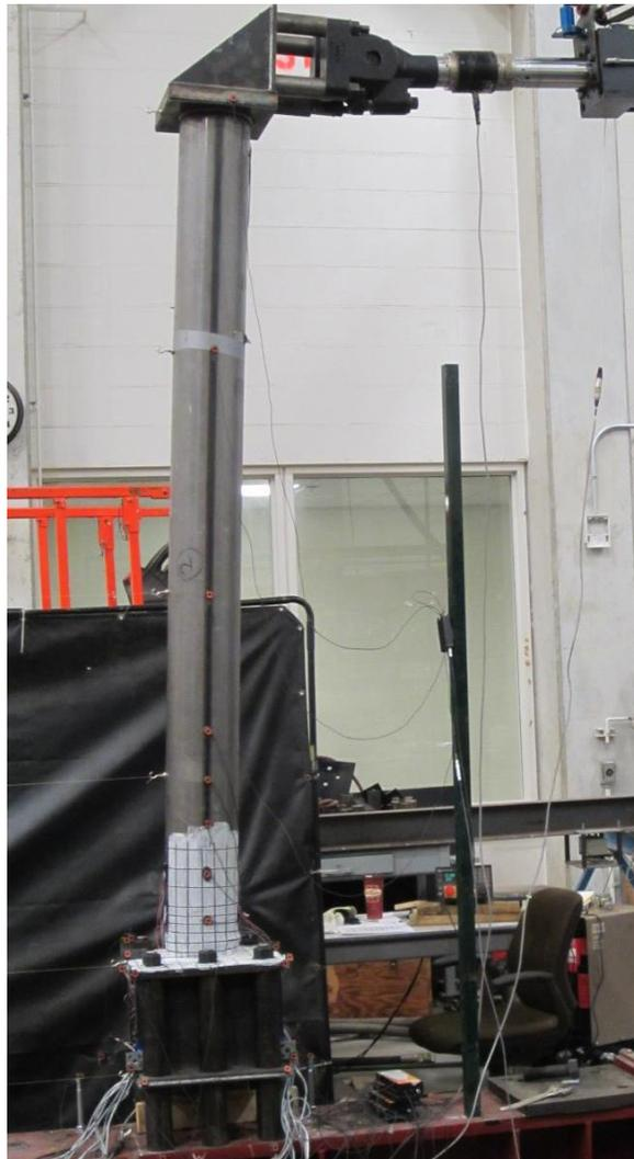
**Figure 4- 27 Specimen S2 at the End of the Cyclic Test**
