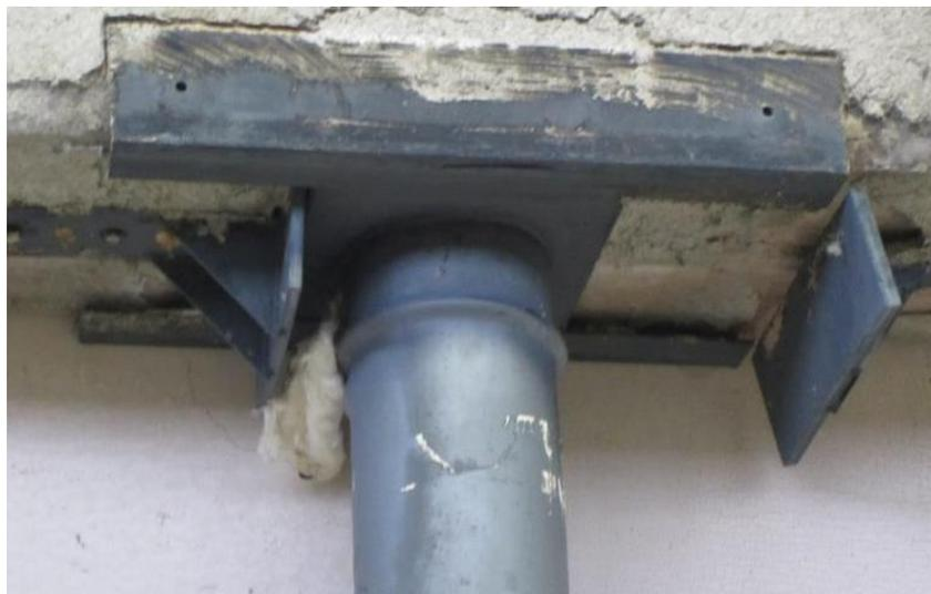
**Figure 5- 13 Local Buckling of Specimen S3 Close to the Top Beam of the Furnace**
