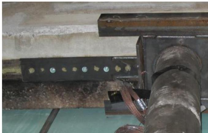
**Figure 5- 4 Built-up Member Used at the Top End Connection**
