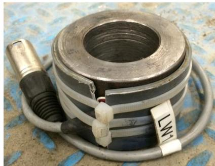
**Figure 4- 20 Load Cell Used to Monitor the Tensile Load of the Threaded Rod**
