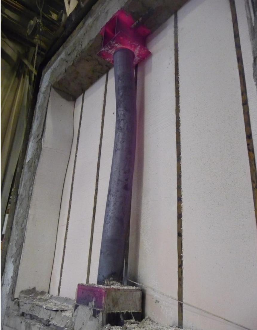
**Figure 5- 24 Out of Plane Global Buckling of Specimen S2**
