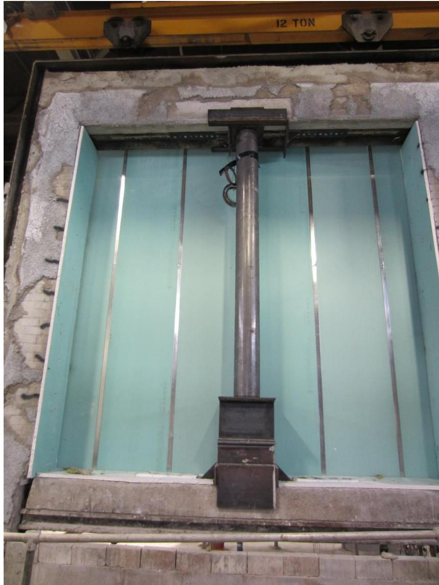
**Figure 5- 1 Specimen S3 in the Vertical Furnace**
