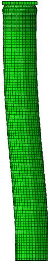
**Figure 3- 29 Visualized final displacement result of the structural analysis – Eurocode steel and concrete models (from ABAQUS)**
