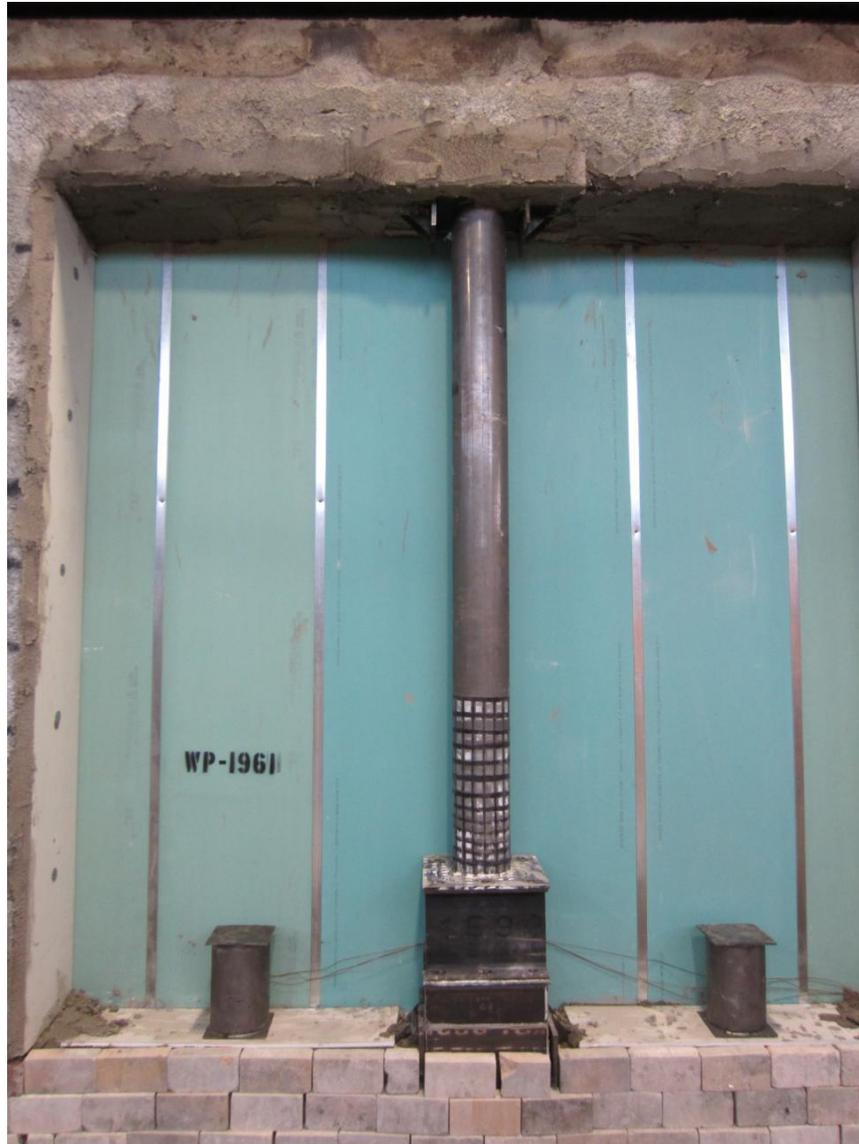
**Figure 5- 16 Specimen S1 Installed in the Furnace in Preparation for the Fire Test**
