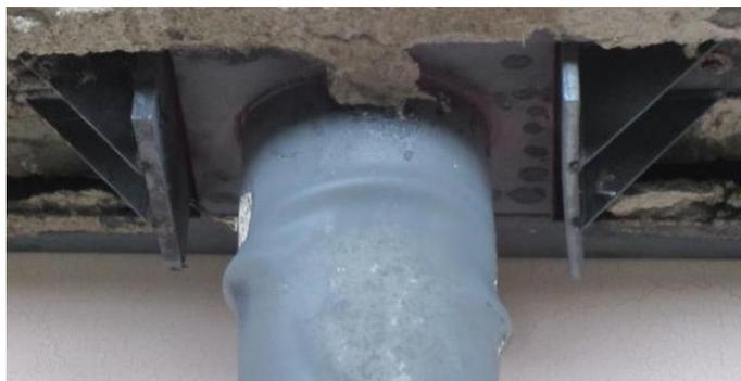
Figure 5- 19 Local Buckling of Specimen S1 Close to the Top Beam of the Furnace
