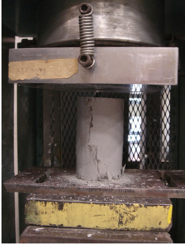
Figure 3-8 Compressive tests of UHPC cylinders
