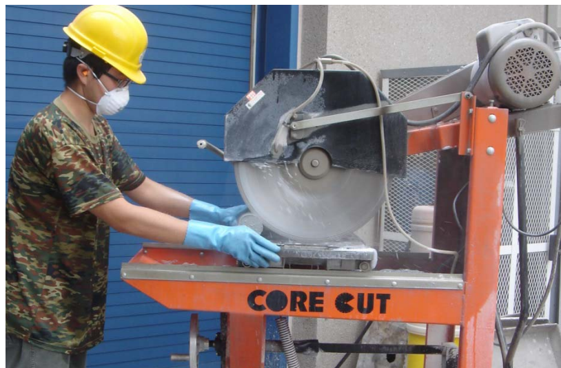
Figure 3-7 Preparation of UHPC cylinders
