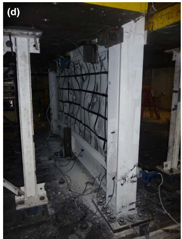
Figure 4-22 Infill Plate Out-of-Plane Buckling at the End of Displacement Step 9 ( \Delta_3 = 3.0\% Drift = 6.38\delta_y ): (a) Overview (North Side); (b) 3 rd Floor; (c) 2 nd Floor; (d); 1 st Floor
