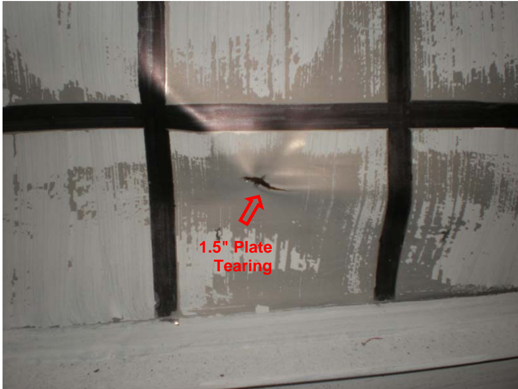
Figure 4-25 New Plate Tearing on the 1 st Story Infill Plate (Displacement Step 9b)
