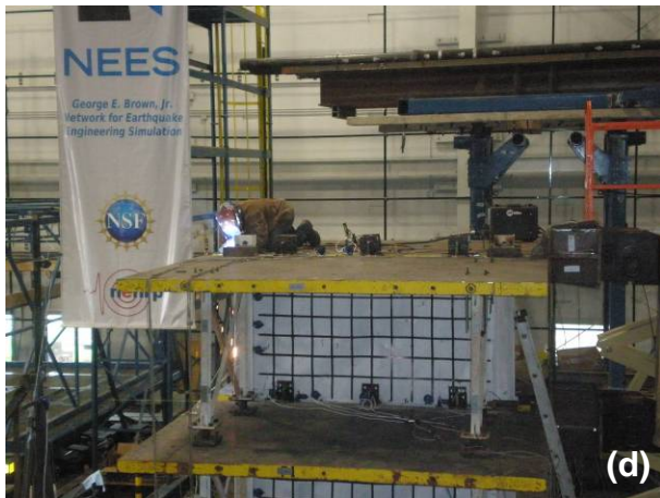
Figure 4-13 HBE3 Connecting Angle Condition in Displacement Step 8 ( \Delta_3 = 2.5\% Drift = 5.32\delta_y ): (a) Connection Prior to Fracture; (b) & (c) Fracture of Both Connecting Angles; (d) Installation of Connecting Channels; (e) Newly Completed Connection at East Column
