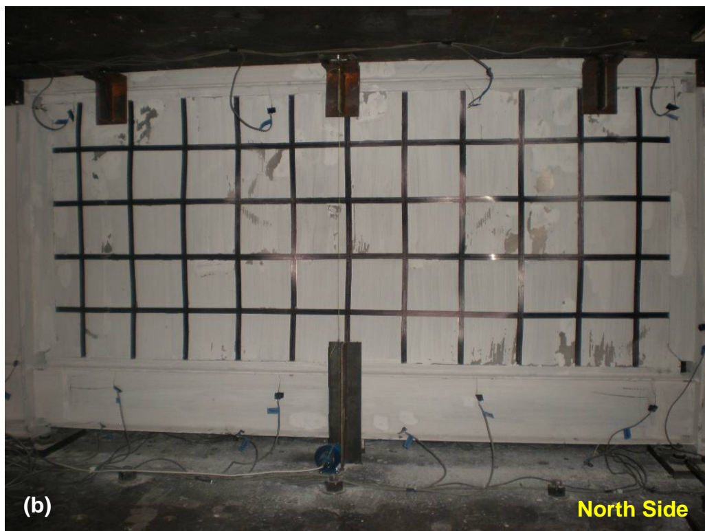
Figure 4-6 Specimen Condition at the End of Displacement Step 6 ( \Delta_3 = 3\delta_y = 1.41\% Drift): (a) Yielding on the 2 nd Floor Infill Plate; (b) Yielding on the 1 st Floor Infill Plate
