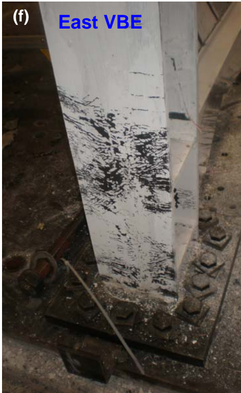
Figure 4-32 Boundary Frame Final Condition – Cont'd: (e) Fracture at HBE1 Top Flange at its Connection to West VBE; (f) & (g) Column Bases
