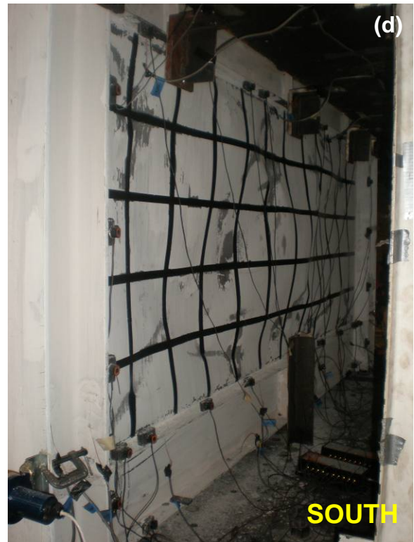
Figure 4-15 Specimen Condition at the End of Displacement Step 7b ( \Delta_3 = 4\delta_y = 1.88\% Drift): (a) & (b) 2 nd Story Infill Plate; (c) & (d) 1 st Story Infill Plate
