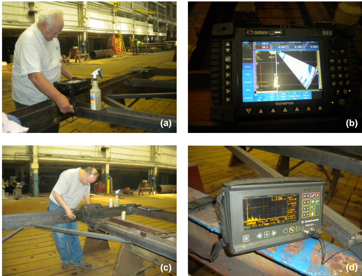
Figure 3-10 Nondestructive Testing: (a) Phase Array (PA) Testing; (b) Real Time Display for PA; (c) Ultrasound Testing (UT); (d) Real Time Display for UT
