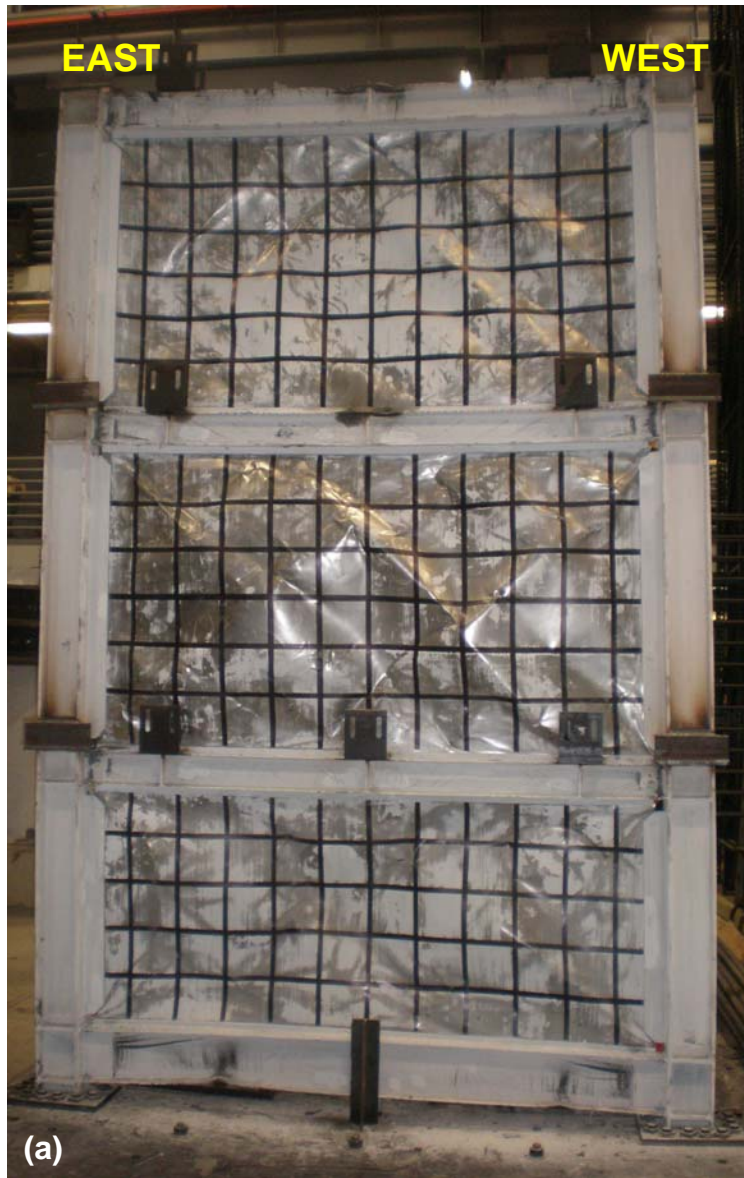
Figure 4-29 Specimen Final Condition (Step 10d: \Delta_3 = 3.33\% Drift = 7.09\delta_y ): a) North Side Overview; (b) South Side Overview
