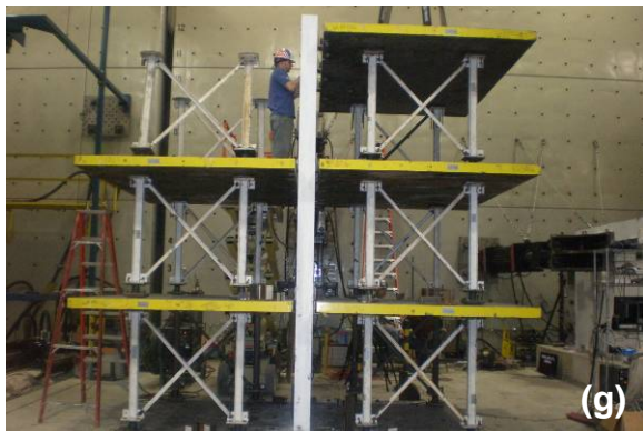
Figure 3-16 Construction Process of Gravity Column System
