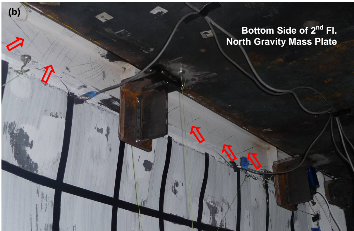
Figure 4-12 Yielding in Displacement Step 7 ( \Delta_3 = 4\delta_y = 1.88\% Drift): (a) Beneath HBE3 Connecting Angles Overview; (b) Yield Lines at a Distinct Angle along HBE2 Web
