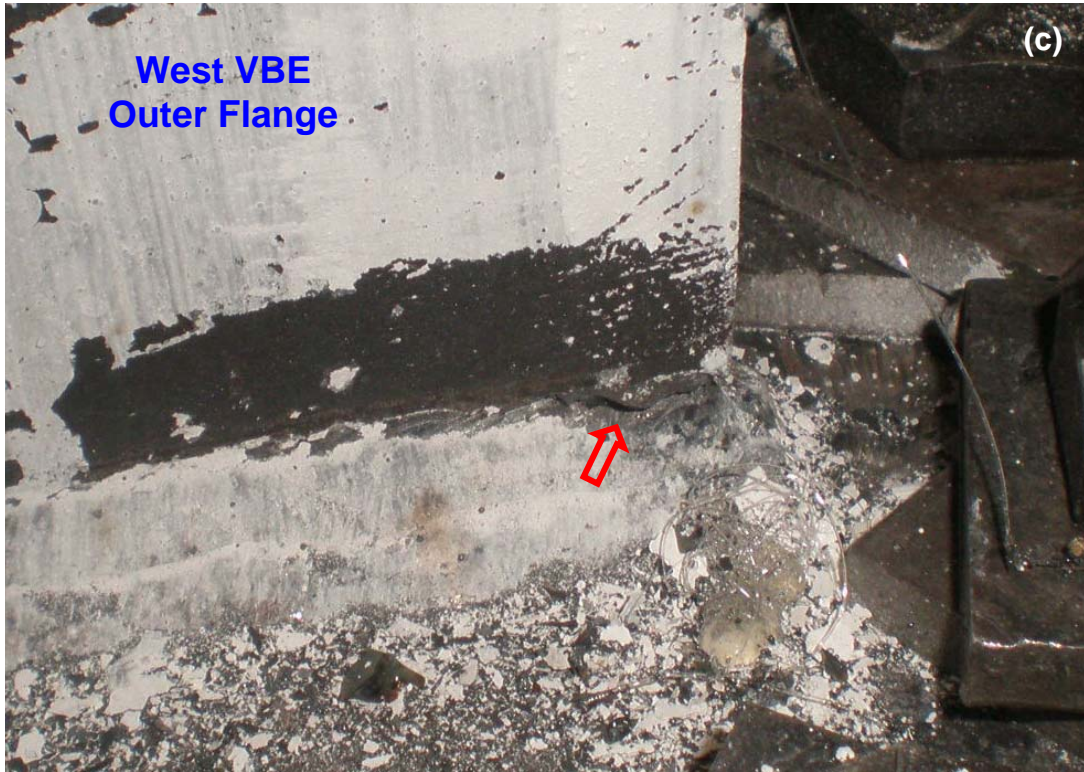
Figure 4-27 Special-Moment Resisting Connection Fractures in Displacement Step 10c ( \Delta_3 = 3.33\% drift = 7.09\delta_y ) – Cont'd: (c) Base of West VBE
