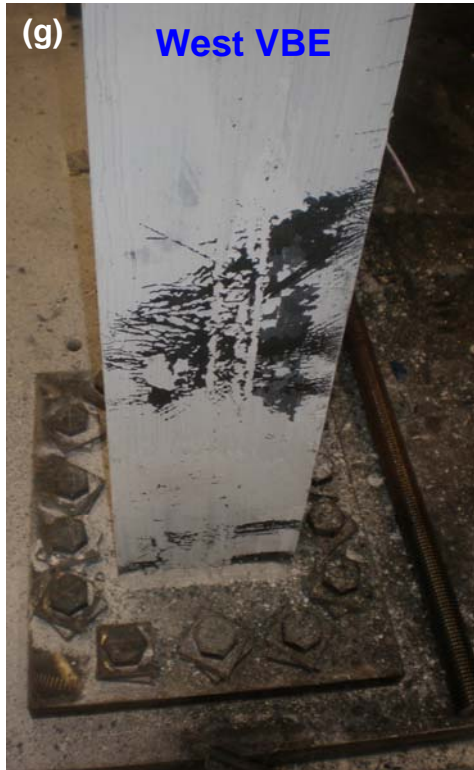
Figure 4-32 Boundary Frame Final Condition – Cont'd: (e) Fracture at HBE1 Top Flange at its Connection to West VBE; (f) & (g) Column Bases
