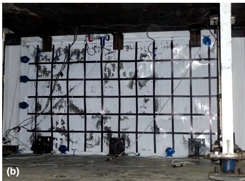
Figure 4-10 Specimen Condition at the End of Displacement Step 6c ( \Delta_3 = 3\delta_y = 1.41\% Drift): (a) Deformed Shape Overview; (b) Yielding on the 2 nd Floor Infill Plate (North View)
