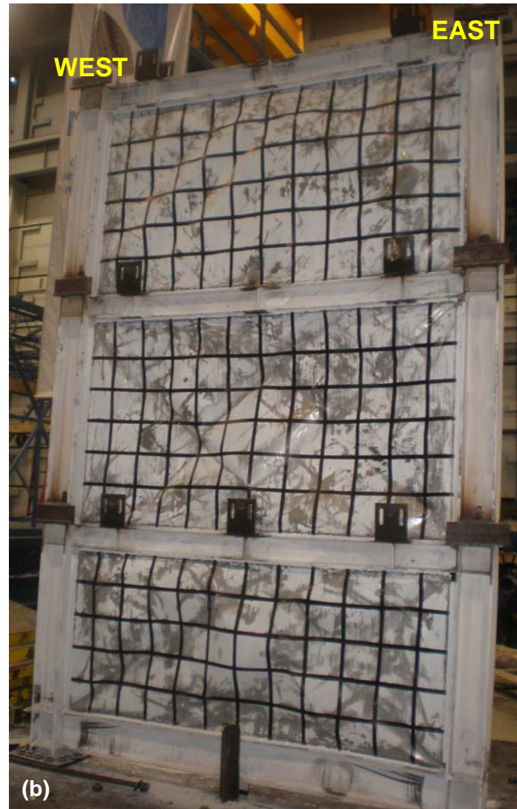
Figure 4-29 Specimen Final Condition (Step 10d: \Delta_3 = 3.33\% Drift = 7.09\delta_y ): a) North Side Overview; (b) South Side Overview
