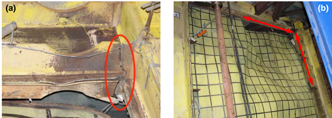
Figure 6-21 Failure Modes in Two-Story SPSW Specimen (Qu and Bruneau 2008): (a) Intermediate HBE Fracture; (b) First Story Web Tearing
