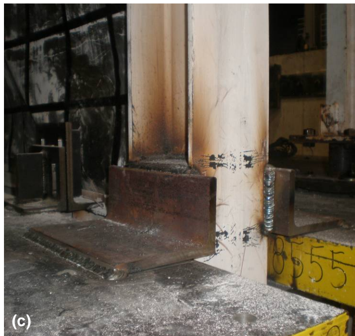
Figure 4-14 Failure and Replacement of Connecting Angles in Displacement Step 7a: (a) Vantage View at Failure; (b) Weld Fractures on Connecting Angles (South Side); (c) Load Transfer Connection at West Column (1 st Story)
