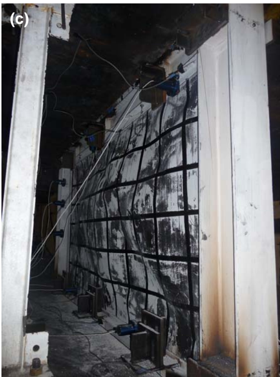
Figure 4-22 Infill Plate Out-of-Plane Buckling at the End of Displacement Step 9 ( \Delta_3 = 3.0\% Drift = 6.38\delta_y ): (a) Overview (North Side); (b) 3 rd Floor; (c) 2 nd Floor; (d); 1 st Floor
