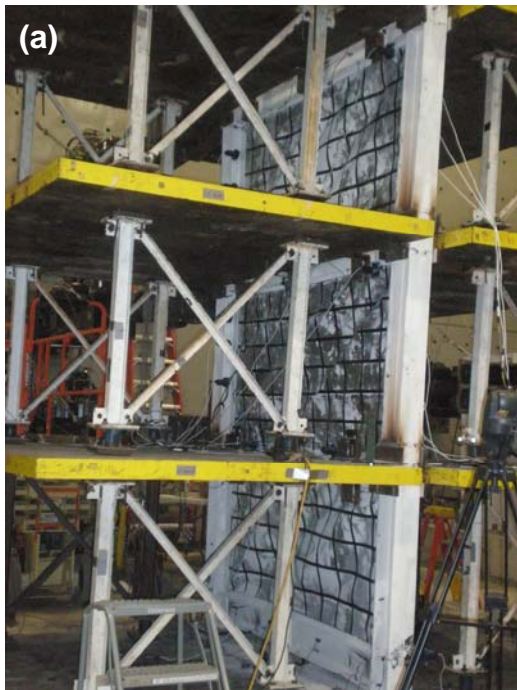
Figure 4-28 Specimen Condition at the End of Displacement Step 10c ( \Delta_3 = 3.33\% Drift = 7.09\delta_y ): (a) Infill Plate Yielding (North Side); (b) Lateral Torsional Buckling
