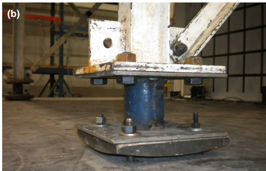
Figure 3-15 Specimen Setup with Gravity Column System: (a) Overview; (b) Detail of Spherically Shape Rocker Support
