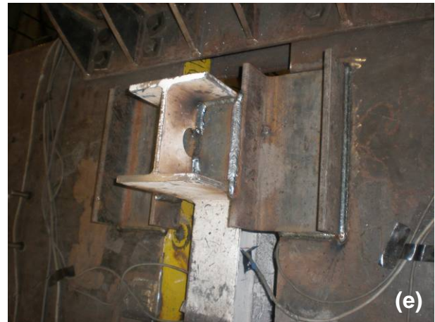
Figure 4-13 HBE3 Connecting Angle Condition in Displacement Step 8 ( \Delta_3 = 2.5\% Drift = 5.32\delta_y ): (a) Connection Prior to Fracture; (b) & (c) Fracture of Both Connecting Angles; (d) Installation of Connecting Channels; (e) Newly Completed Connection at East Column
