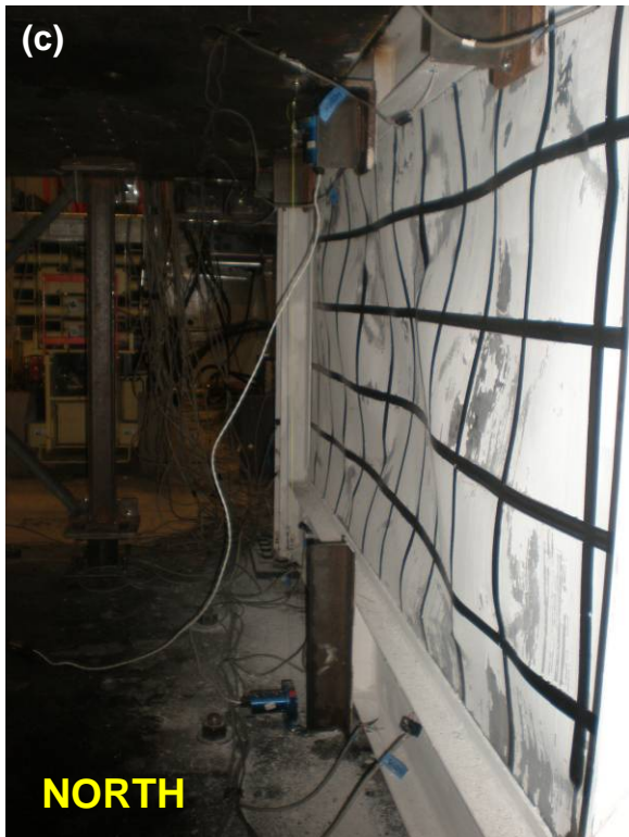
Figure 4-15 Specimen Condition at the End of Displacement Step 7b ( \Delta_3 = 4\delta_y = 1.88\% Drift): (a) & (b) 2 nd Story Infill Plate; (c) & (d) 1 st Story Infill Plate
