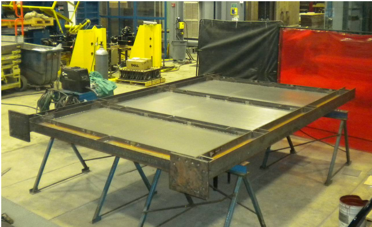
Figure 3-11 Three-Story SPSW Specimen
