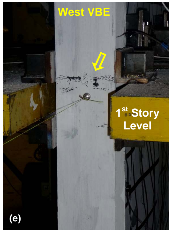
Figure 4-7 New Yielding Pattern Emerged in Displacement Step 6 – Cont'd: (c) Distributed Flange Yielding; (d) & (e) Upper Column Flange Yielding
