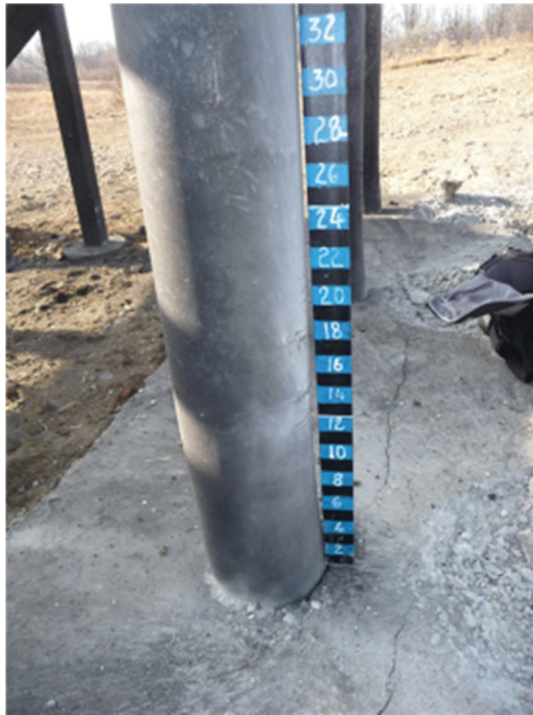
Figure 8-22: Distribution of Deformation near the Base of B6
