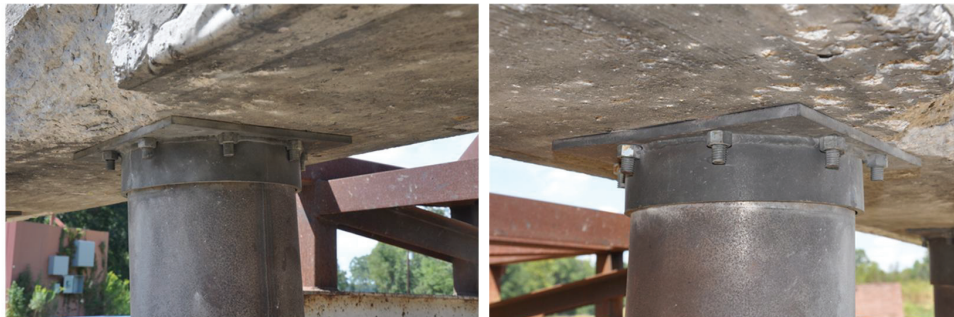
Figure 8-93: State of the Top Collar after the Test
