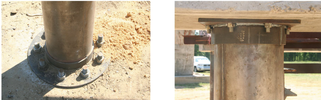
Figure 8-65: Bottom (Left) and Top (Right) Collars of Specimen MSJC4
