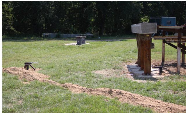
Figure 8-68: View of Specimen MSJC1 Showing the Shorting Pins Arrangement in the Back and the Pressure Probe in the Front
