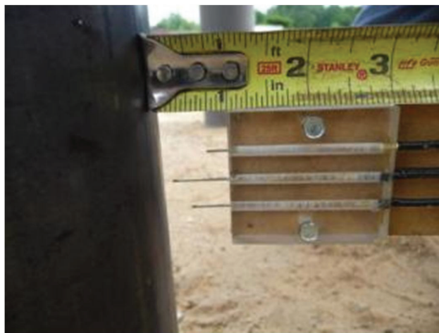
Figure 8-57: Shorting Pins Arrangement on Specimen B10
