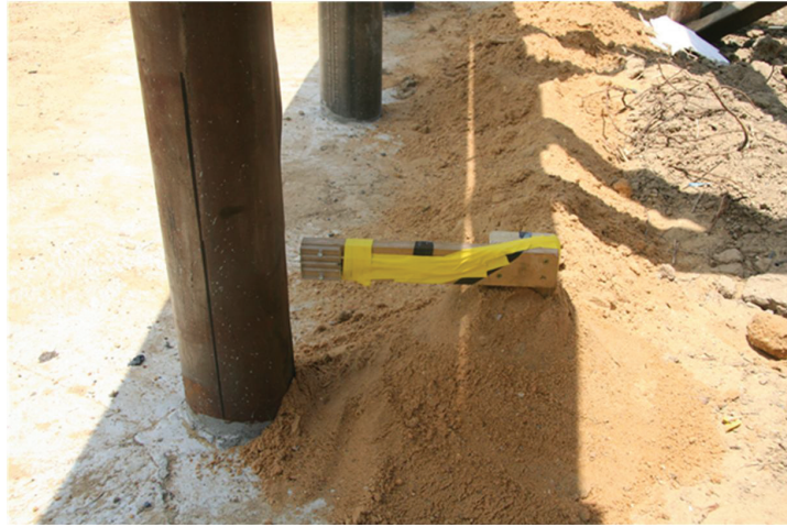
Figure 8-54: Base of Specimen B9 Showing Shorting Pin Mount
