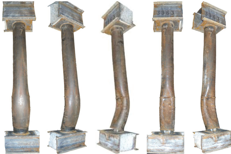
Figure 8-41: Final Deformation of Specimen B6
