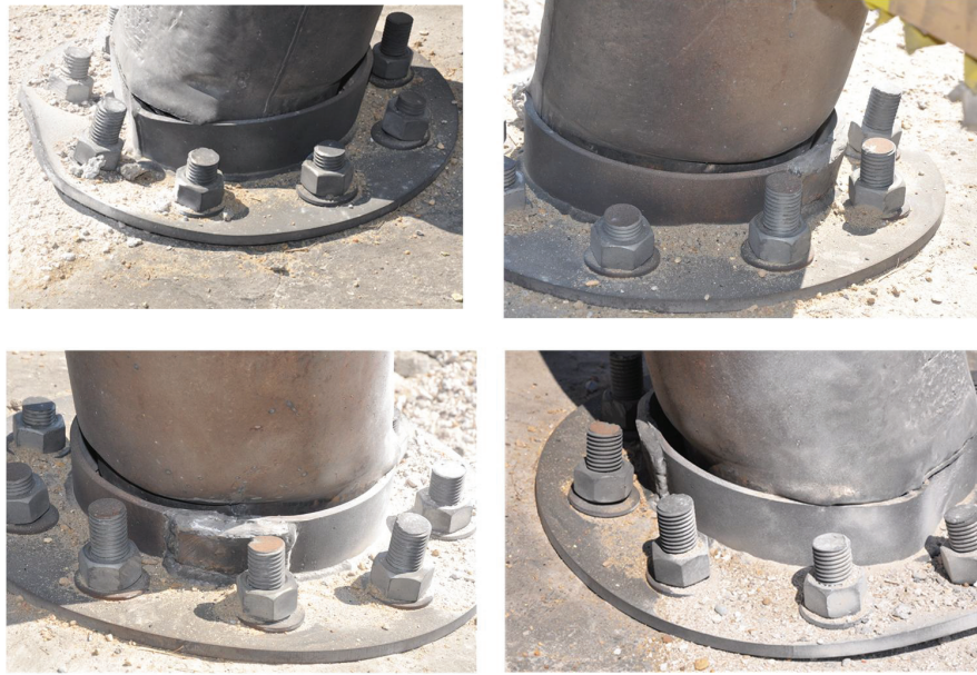
Figure 8-92: State of the Bottom Collar after the Test
