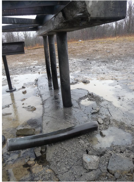
Figure 8-36: Failure of Specimen B8
