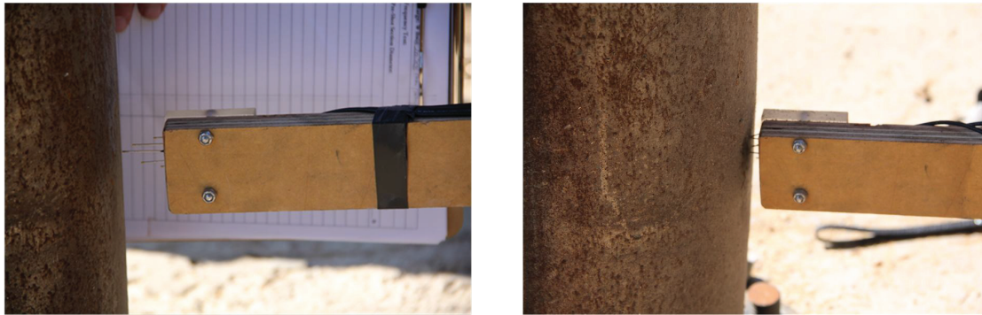
Figure 8-75: Pre and Post-shot View of the Shorting Pin Assembly on the Back of Specimen MSJC3
