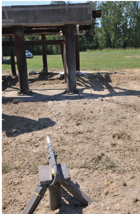
Figure 8-60: Pressure Probe After Test 1 on Specimen MSJC1
