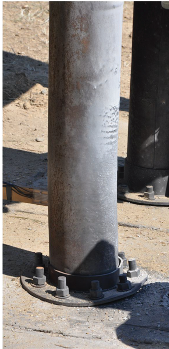
Figure 8-74: Post-shot View of MSJC3 Showing Lip Deformation
