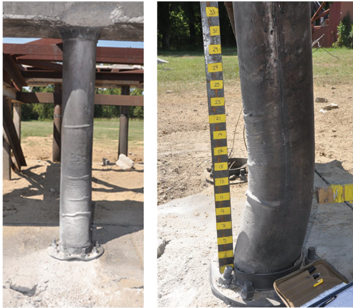
Figure 8-91: Deformation of Specimen MSJC3
