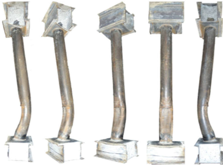
Figure 8-44: Final Deformed Shape of Specimen B4
