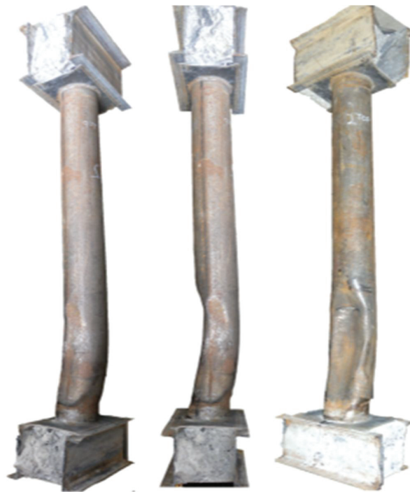
Figure 8-26: Final Deformed Shape of Specimen B7
