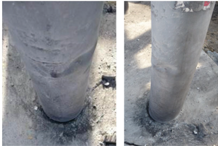
Figure 8-19: Dent in Specimen B2
