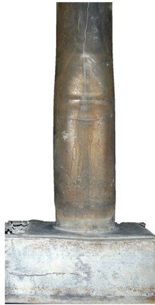
Figure 8-33: Flattening of the Front Face of Specimen B3
