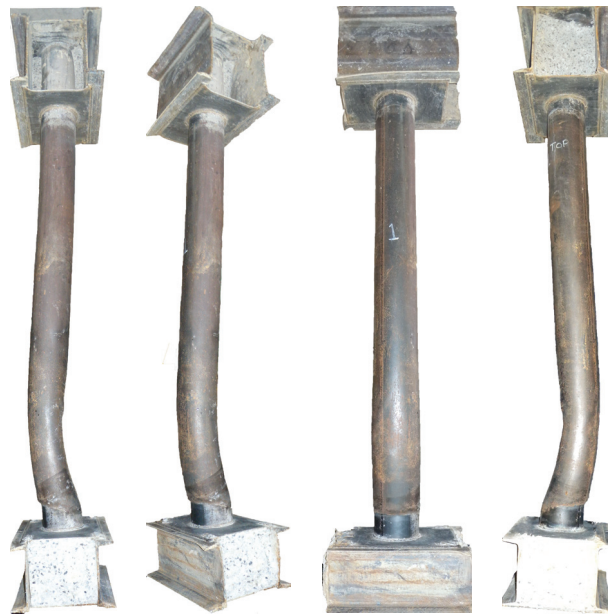
Figure 8-31: Final Deformed Shape of Specimen B1
