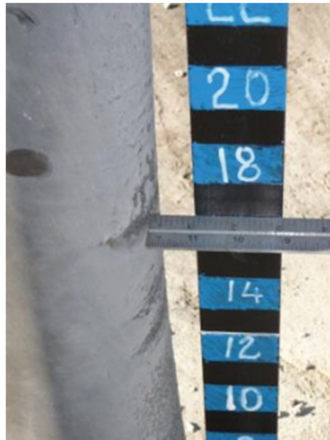
Figure 8-17: Measurement of the Maximum Deformation of Specimen B8
