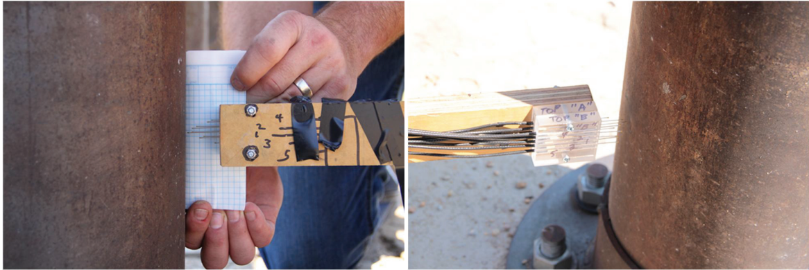
Figure 8-77: Shorting Pins on the Back of Specimen MSJC2
