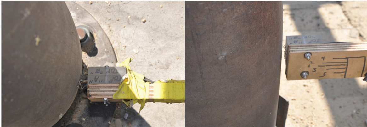
Figure 8-78: Post-Shot View of the Pin Assembly on Specimen MSJC2
