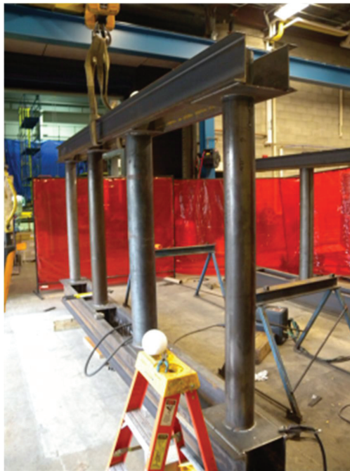
Figure 8-11: Assembly of the Foundation Beam to the Tubes
