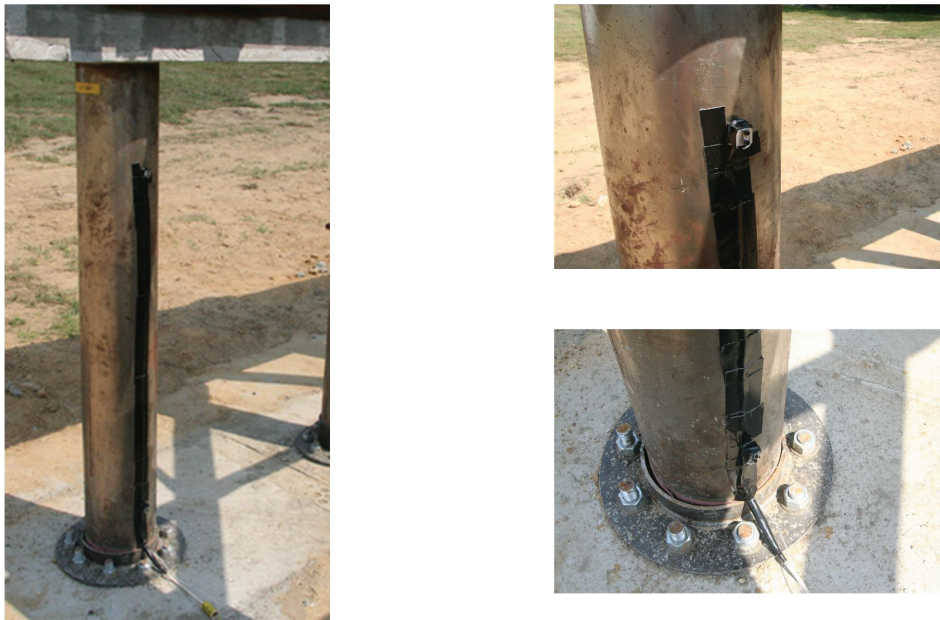
Figure 8-61: Shock Accelerometers on Specimen MSJC1
