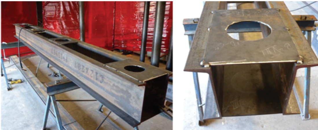
Figure 8-7: Cap-Beam and Plates to C-Channel Connections in the Cap Beam
