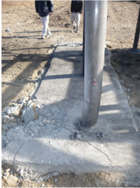
Figure 8-18: Deformation of Specimen B2 After the Test
