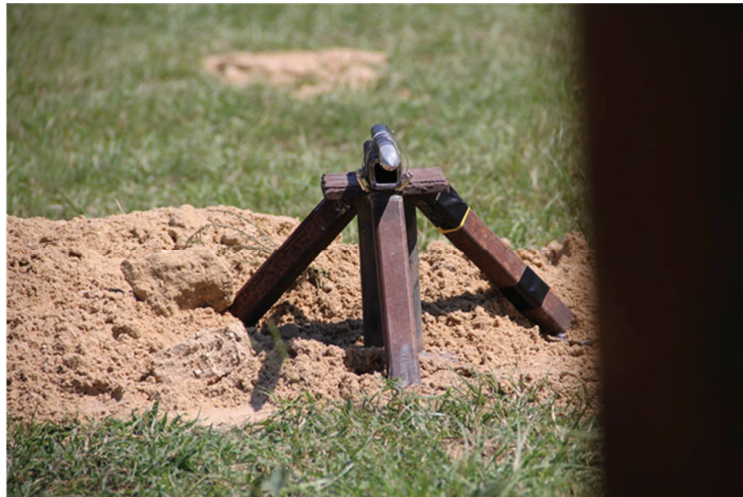
Figure 8-53: Pressure Probe and Supporting Mount
