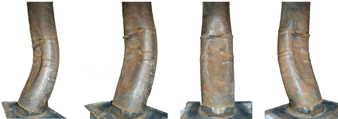
Figure 8-42: Denting and Fracture of Specimen B6
