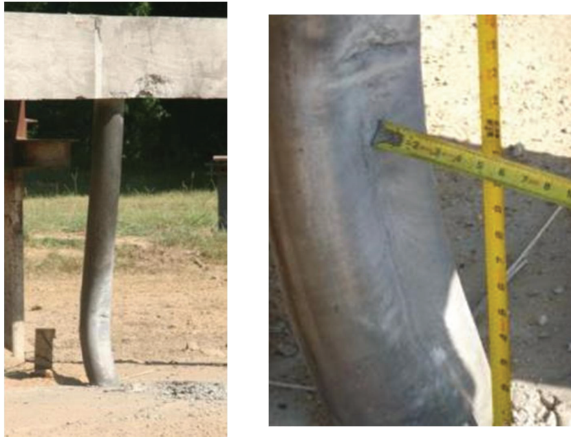
Figure 8-56: Observed Deformation of Specimen B9
