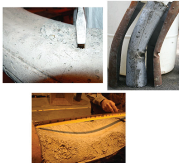
Figure 8-94: Concrete Core of CFDST after Opening
