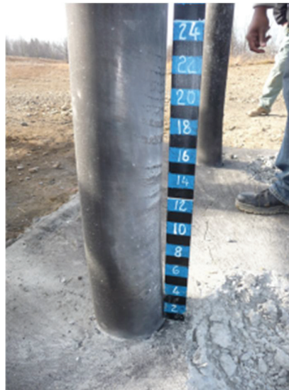
Figure 8-20: Deformation of Specimen B4 after the Test
