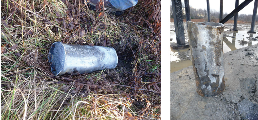
Figure 8-35: Torn Base of Specimen B8
