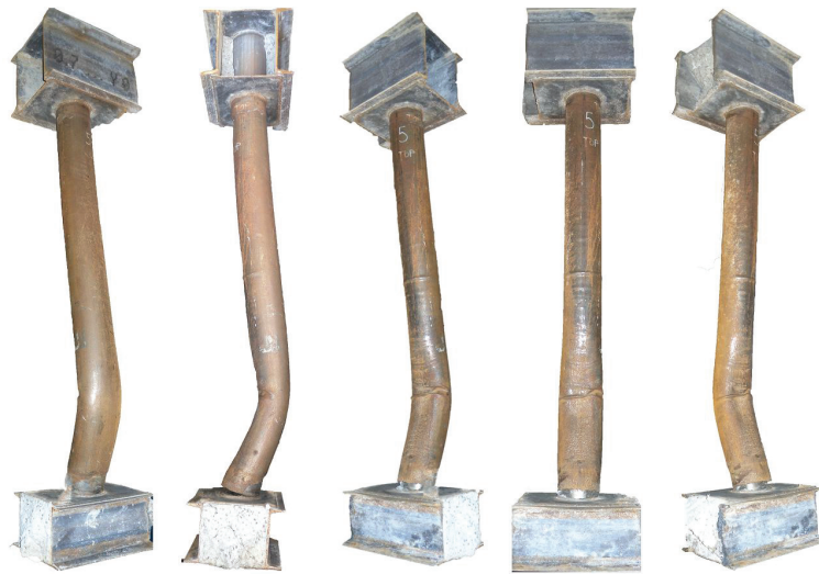
Figure 8-38: Final Deformed Shape of Specimen B2
