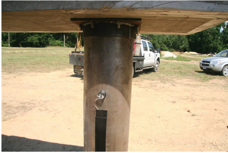
Figure 8-66: Accelerometer of the Back Side of Specimen MSJC4
