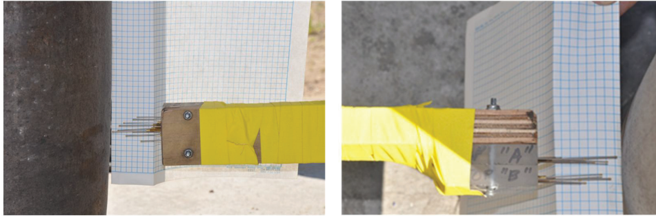
Figure 8-90: Shorting Pin Arrangement for MSJC3
