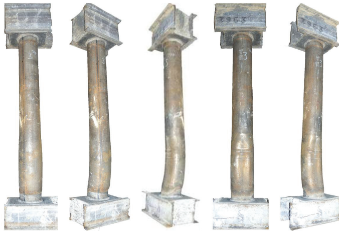
Figure 8-32: Final Deformed Shape of Specimen B3
