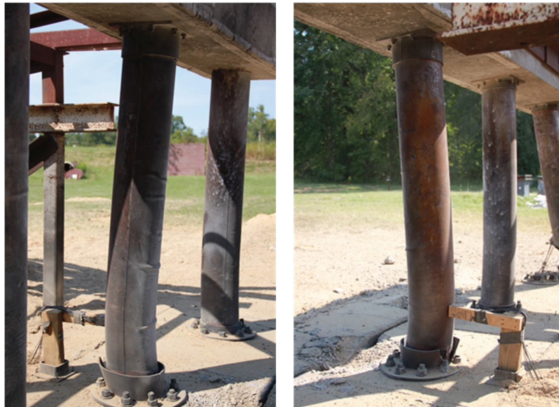
Figure 8-80: Post-Shot Views of on Specimen MSJC2
