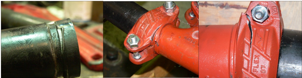
Figure 2-5 Observed Damage in Grooved Tee Joints (Tian et al., 2012)
