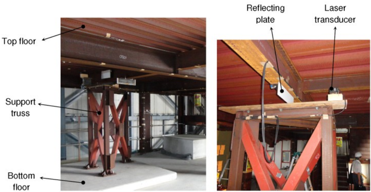
Figure 4-32 Instrumentation for Measuring Story Drift
