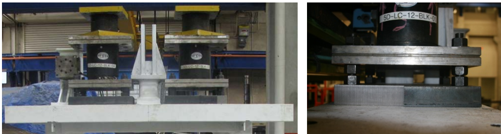
Figure 3.8. Elastomeric bearings supported on load cells (Left) and close-up view showing bolt/nut leveling system (Right)
