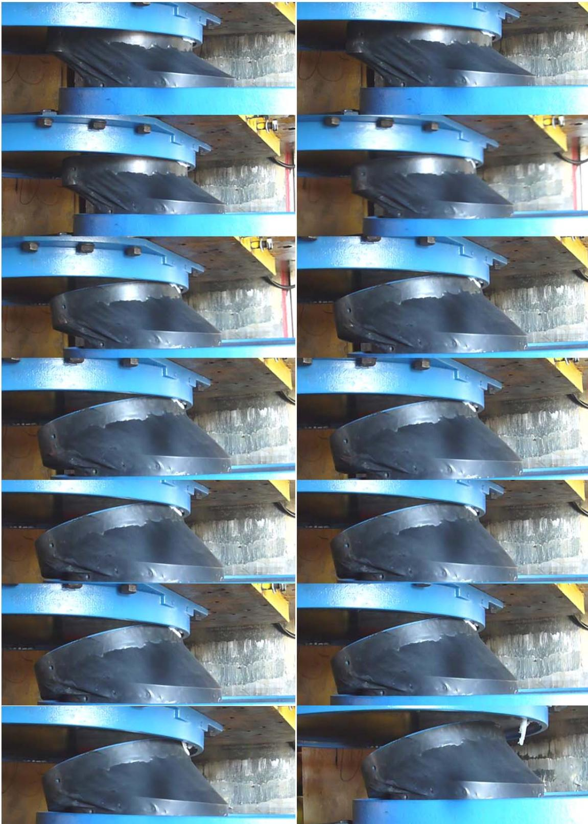
**Figure 8-31: Captured frames in the uplift experiment of Example 6 during the uplift episode (read row by row)**
