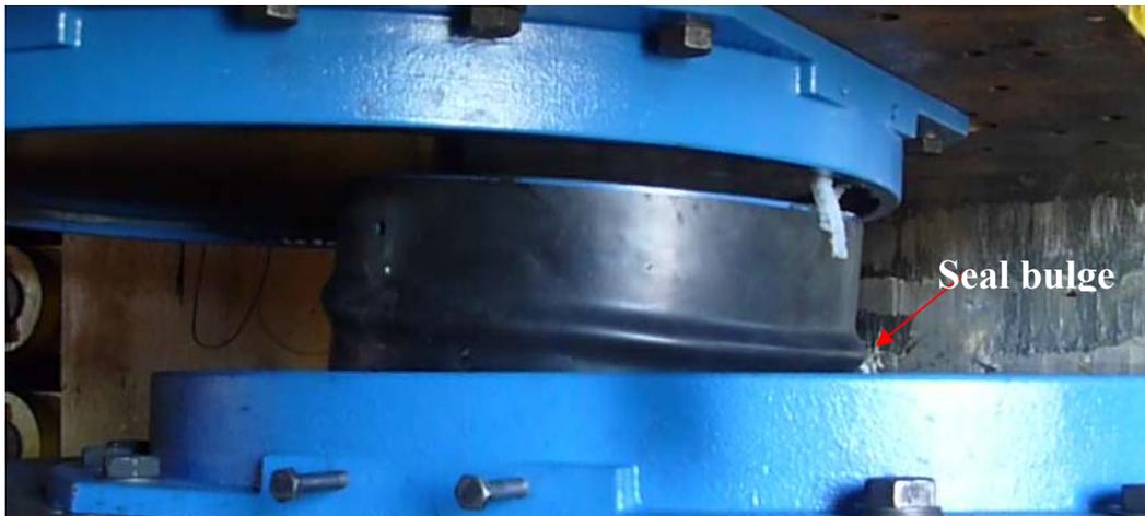
**Figure 5-5: Slider assembly of an un-deformed Triple FP bearing that shows the existence of bulging of the seal**
