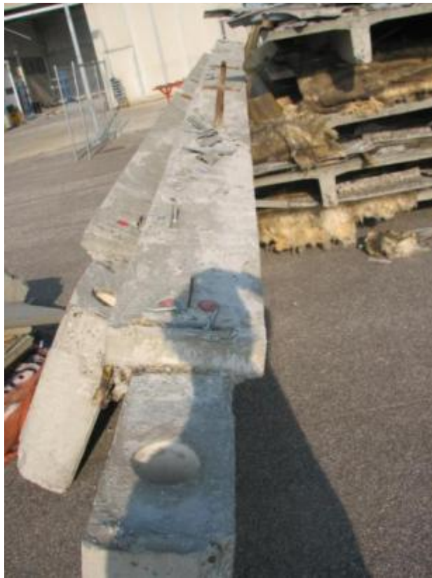
Figure 6-37 Probable roof collapse due to the slip of the beam from the shear key
