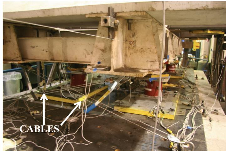
**Figure 5-10: View of transverse cables used for torsional stability in tests of NSD without the GSA**
