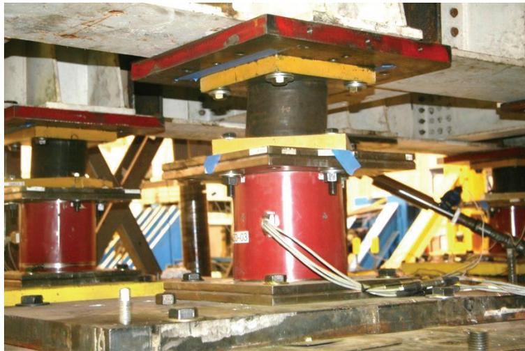
**Figure 5-16: View of load cells below elastomeric bearings**
