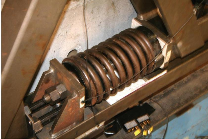
**Figure 2-7: Photograph of un-deformed GSA installed at the NSD**
