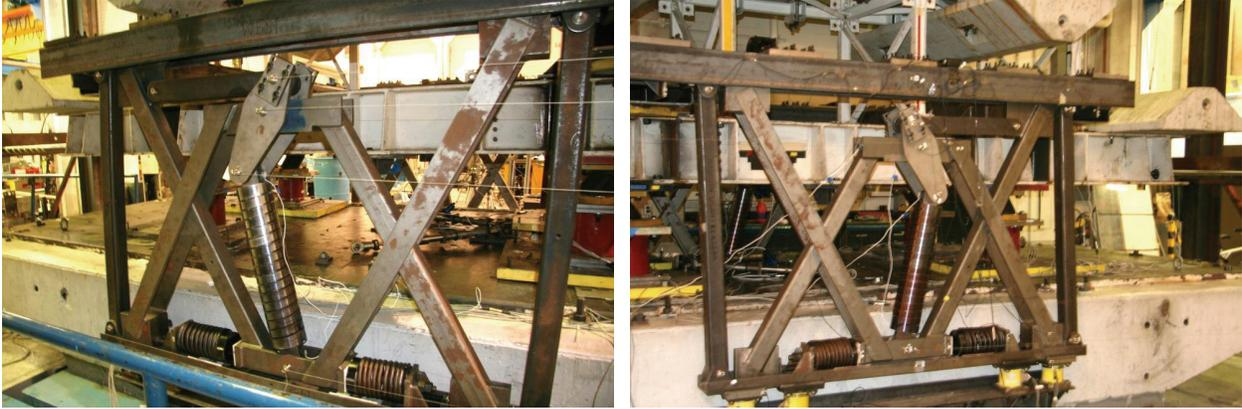
**Figure 6-11: Deformed NSD West (left) and NSD East (right) during displacement-controlled test at 6.4cm amplitude and 0.02Hz frequency**
