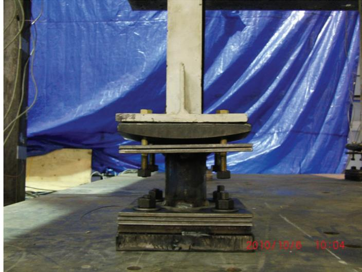
**Figure 4-3 Photograph of gravity frame connection.**
