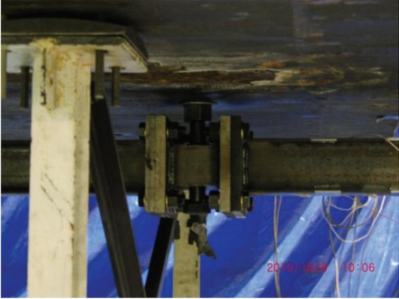
**Figure 4-5 Photograph of especial beam to gravity frame connection.**
