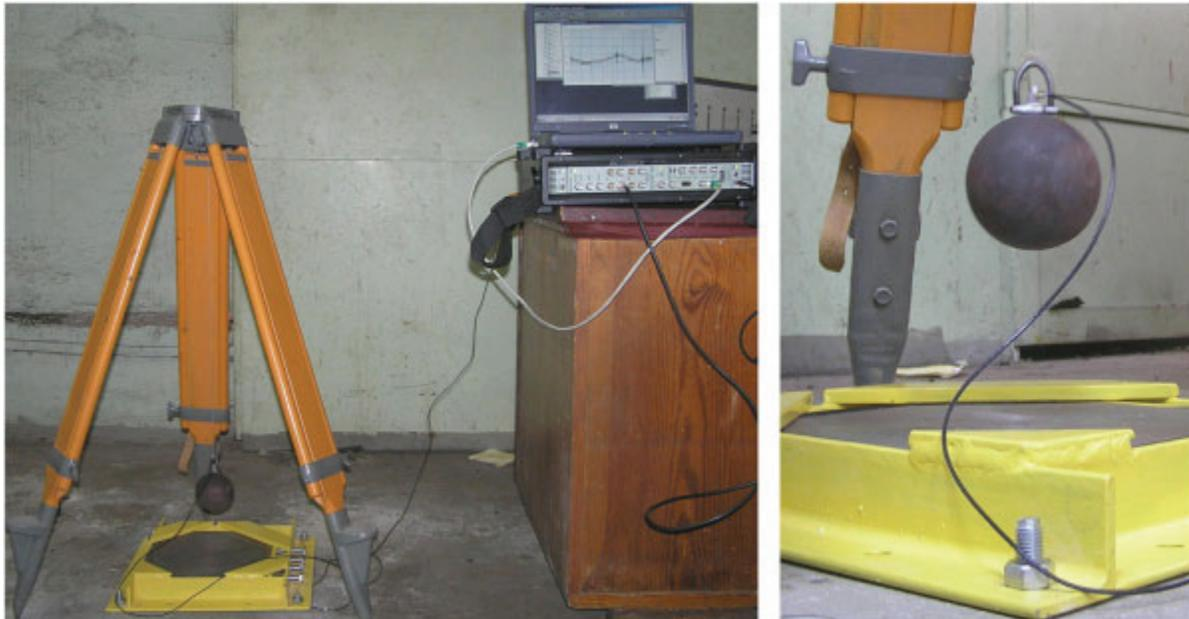
**Figure 2-14 Setup of the impact experiment by Jankowski (2010).**
