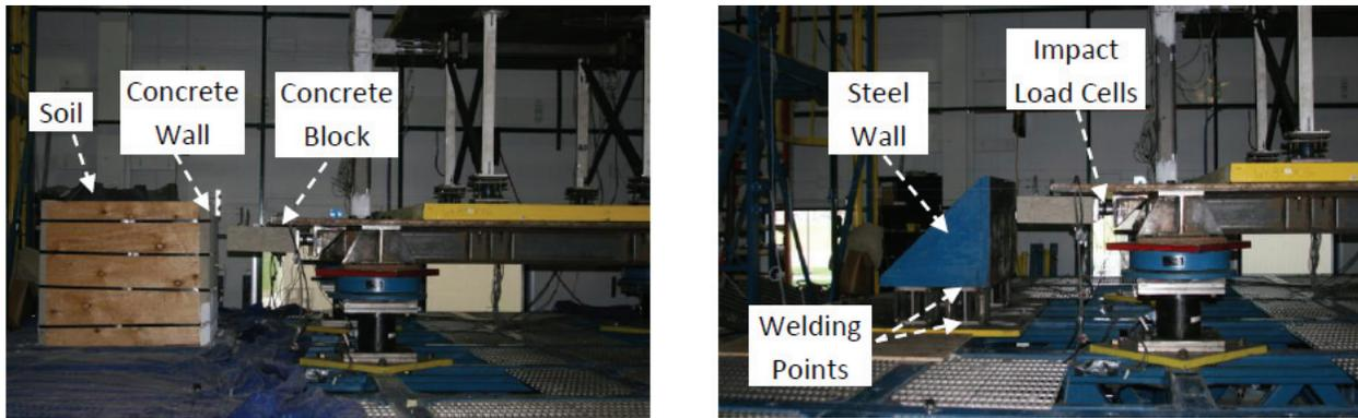
**Figure 4-8 Photograph of different types of moat wall used in impact purpose.**
