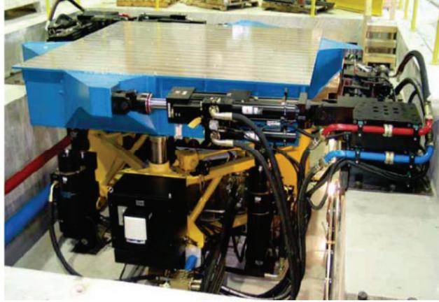
**Figure 5-32 NEES at buffalo shake table facility used to conduct the experimental program**
