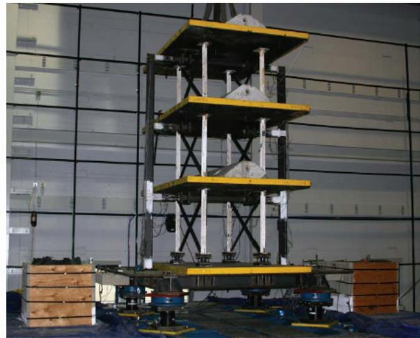
**Figure 4-4 Illustration and photograph of shake table test setup.**
