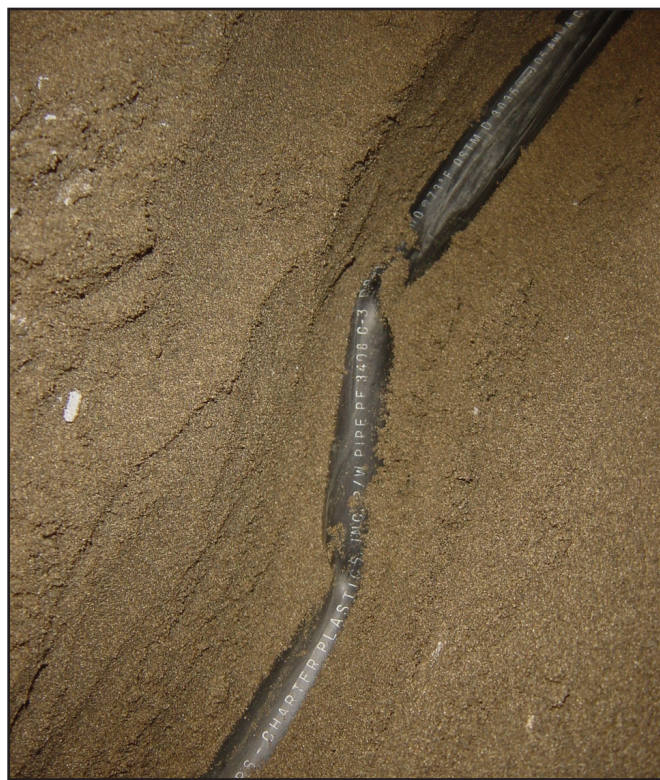
■ Figure 8.14 Close-up View of Two Buckles in HDPE Pipe Subject to Strike Slip-Nominal Compression Faulting (View After Overburden Soil Removed)
