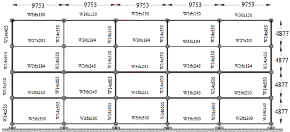
(a) Typical longitudinal frame
