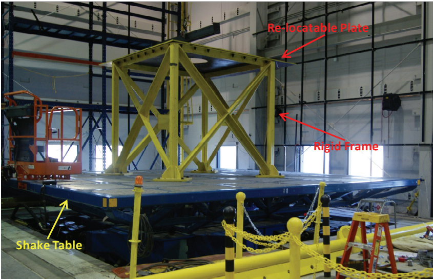
Figure 5-3 Support Structure on the Shake Table
