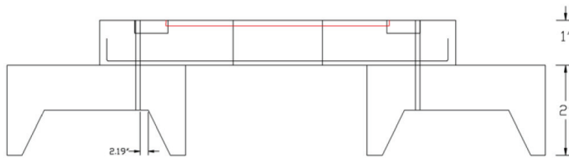
Figure 4-4 Front View of the Reinforced Concrete Slab (Muhammad, 2012)
