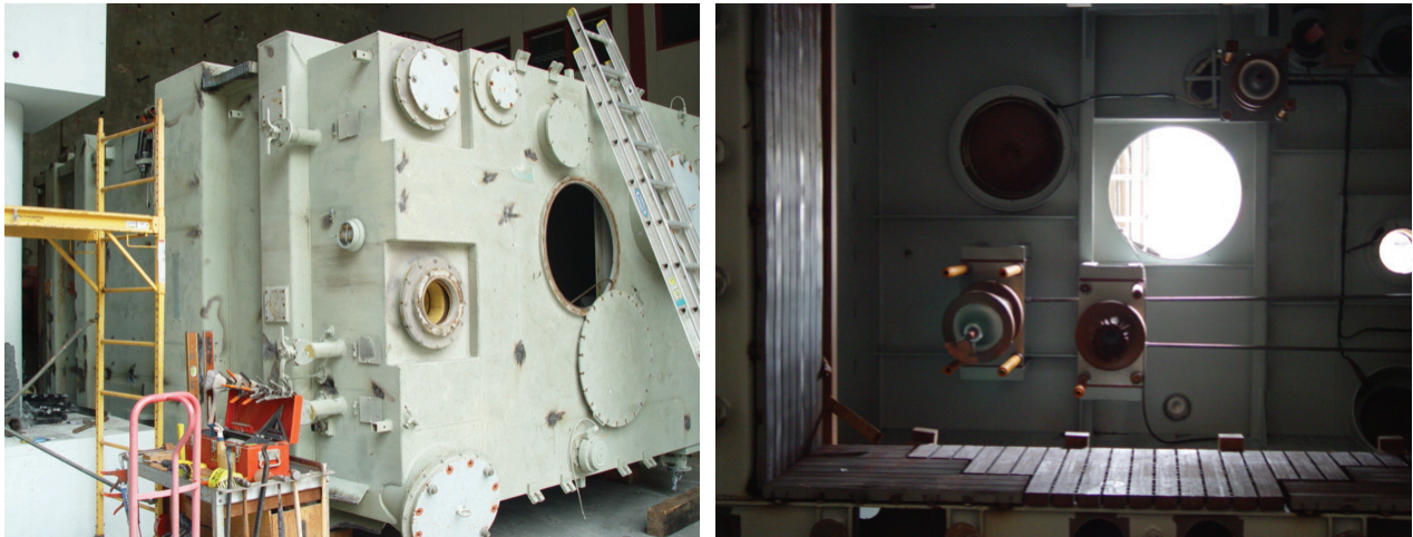
Figure 3-5 525kV Transformer Tank Incorporating Stiffening Elements Composed of Thin Plates and Channels (Matt & Filiatrault, 2004)
