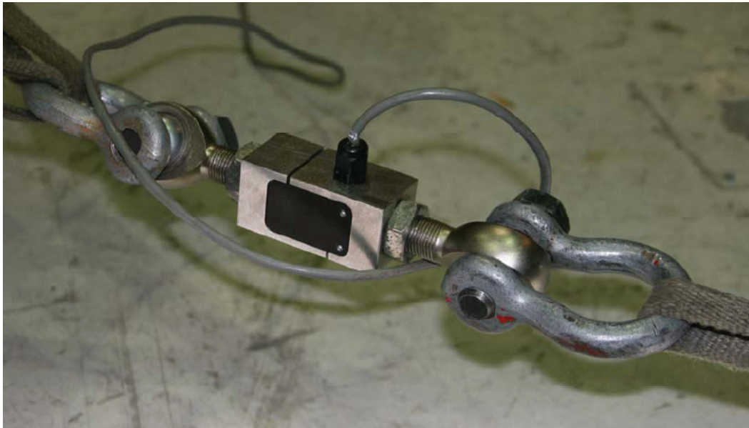
Figure 4-7 Load Cell used for the Pull-Back Tests
