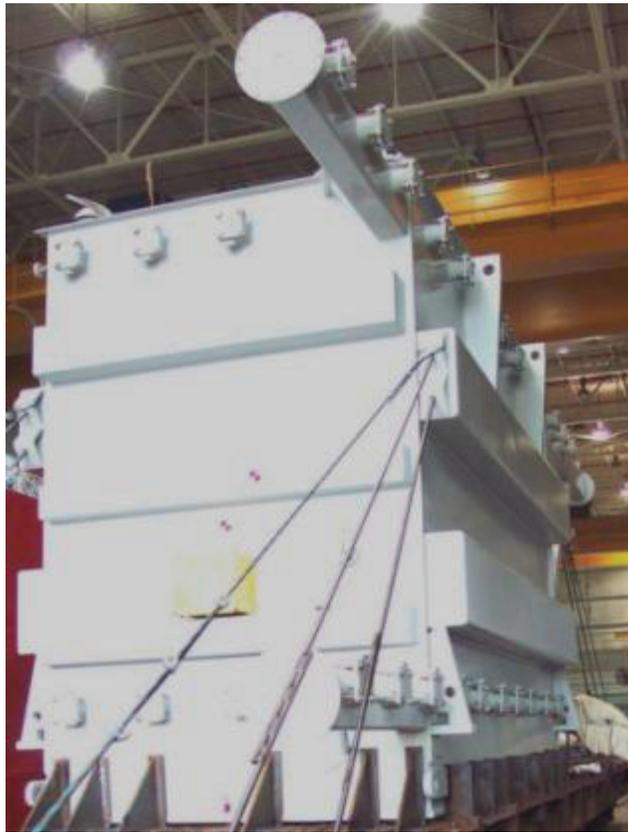
**Figure 2-7 Side of tank where the radiators are attached. (supporting joints shown)**
