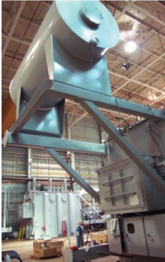
**Figure 2-3 Oil conservator and connection to the tank**
