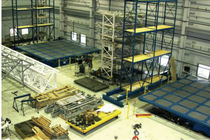
Figure 2-5: Dual shake tables (with extension platforms) at the SEESL at the University at Buffalo (see www.nees.buffalo.edu )
