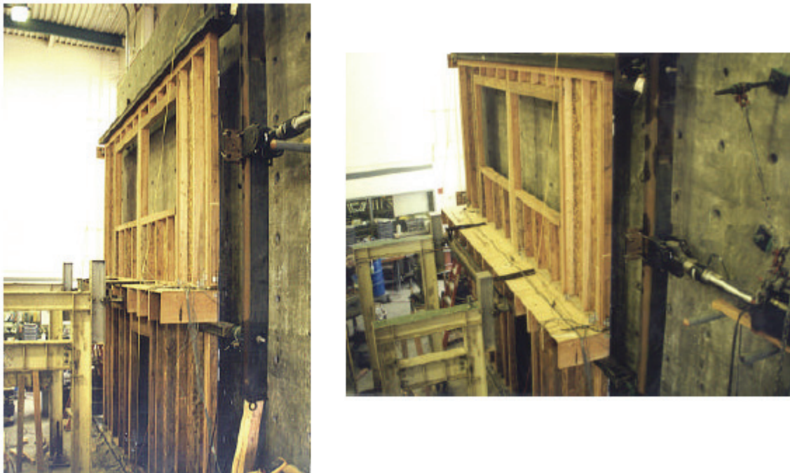
Figure 5.23 Photo of PD2S Wall during Testing (from Pardo et al. 2003)
