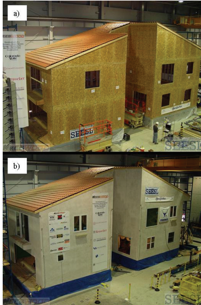
Figure 3.3 Test Building on Shake Tables: (a) without Wall Finishes – Test Phase 1 and (b) with Wall Finishes – Test Phase 5
