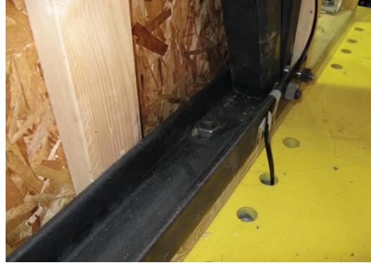
Bottom Channel Anchored to Shake Table with Two A325 Structural Bolts
