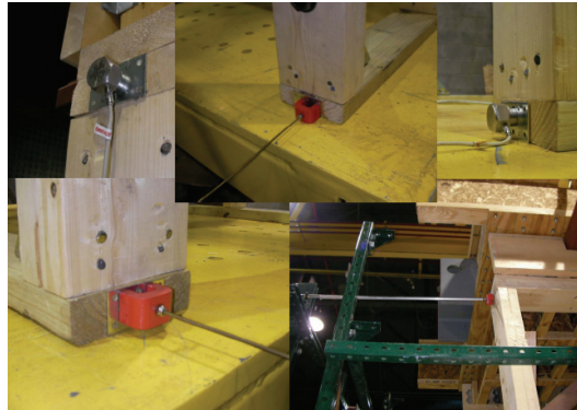
Sensors Installed at Various Locations
