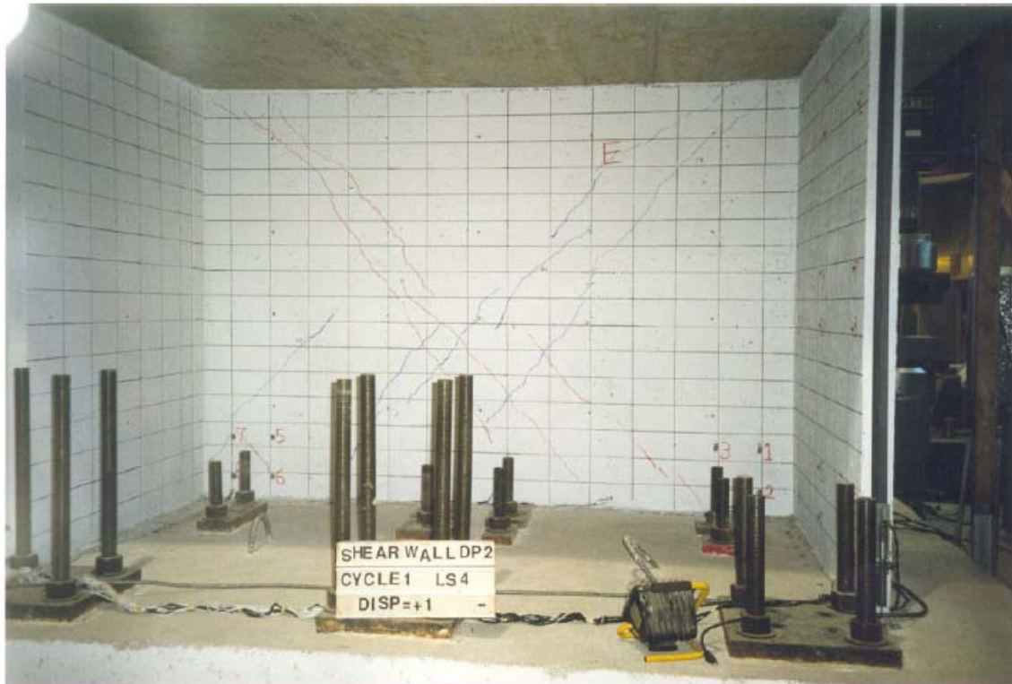
Figure C-305 Condition of wall DP2 at 0.05% drift [Palermo and Vecchio (2002)]
