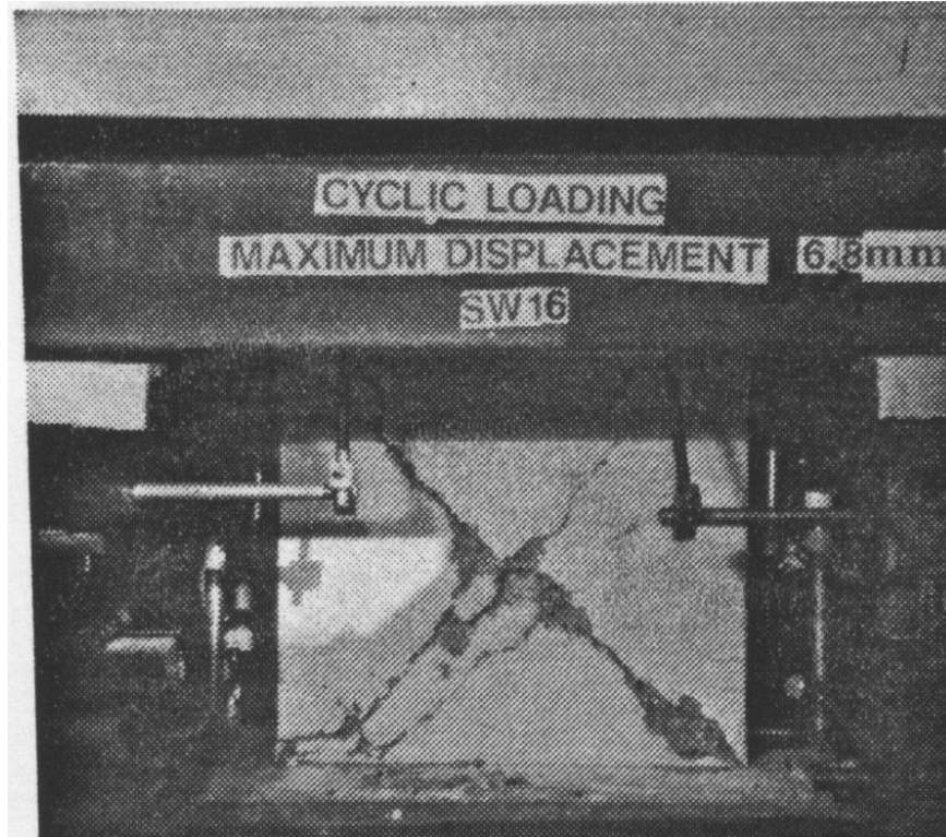
Figure C-141 Condition of wall SW16 at 1.37% drift [Lopes and Elnashai (1991)]
