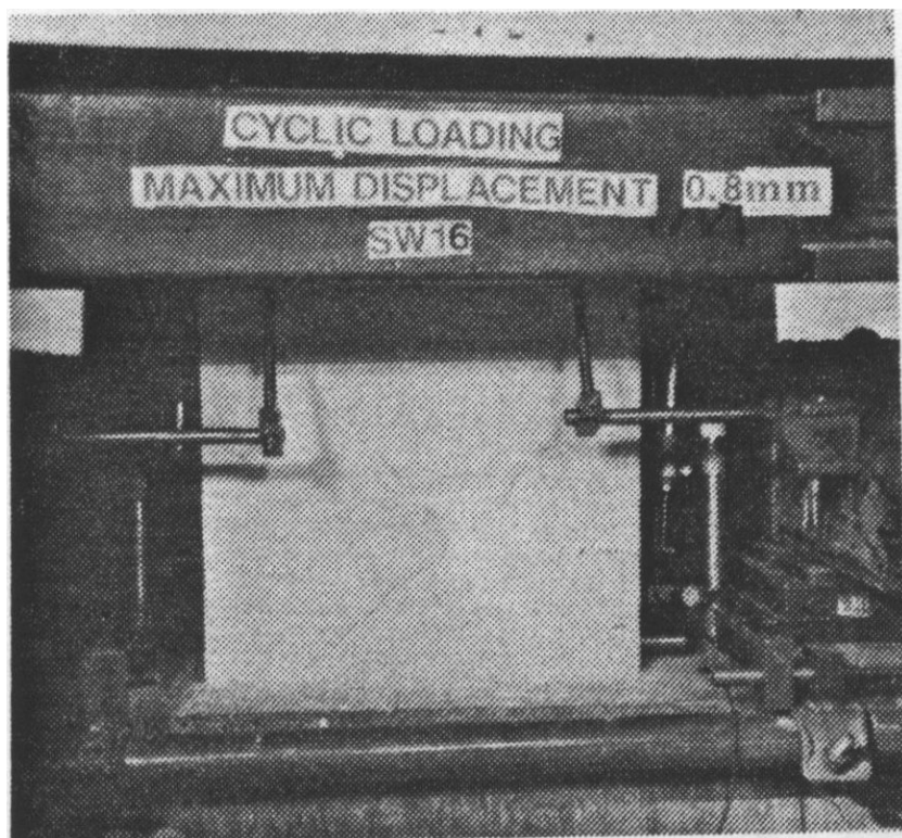
Figure C-135 Condition of wall SW16 at 0.16% drift [Lopes and Elnashai (1991)]
