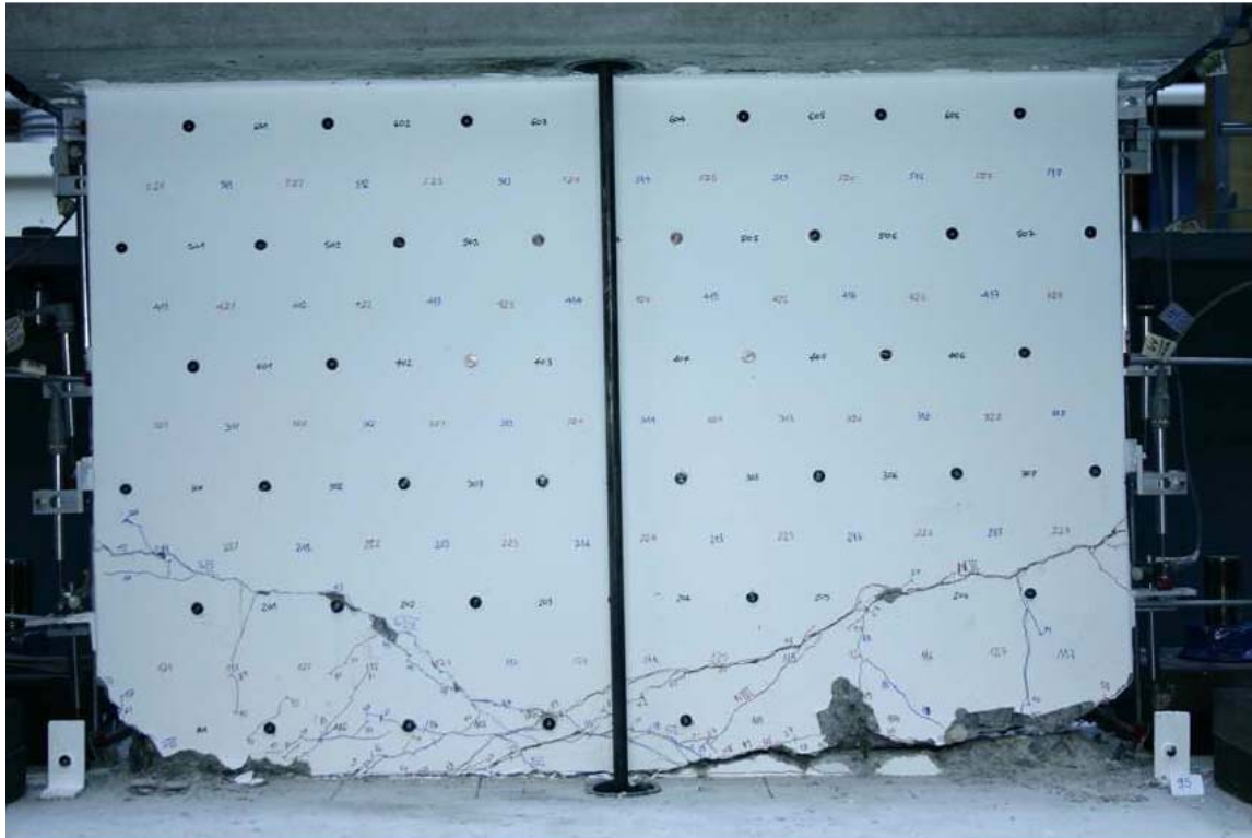
Figure C-94 Condition of wall M4 at 1.97% drift [Greifenhagen et al. (2005)]
