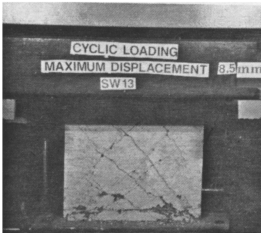
Figure C-118 Condition of wall SW13 at 1.72% drift [Lopes and Elnashai (1991)]
