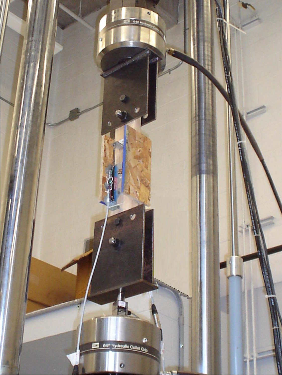
Figure 5.5: Parallel to grain connection test setup with 2x4 framing
