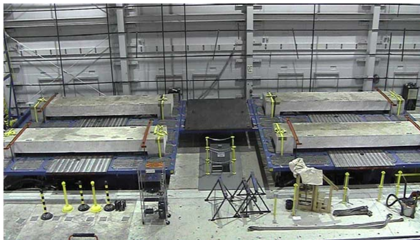
Figure 7.1: Ballast weights located on the shake tables and the connecting bridge
