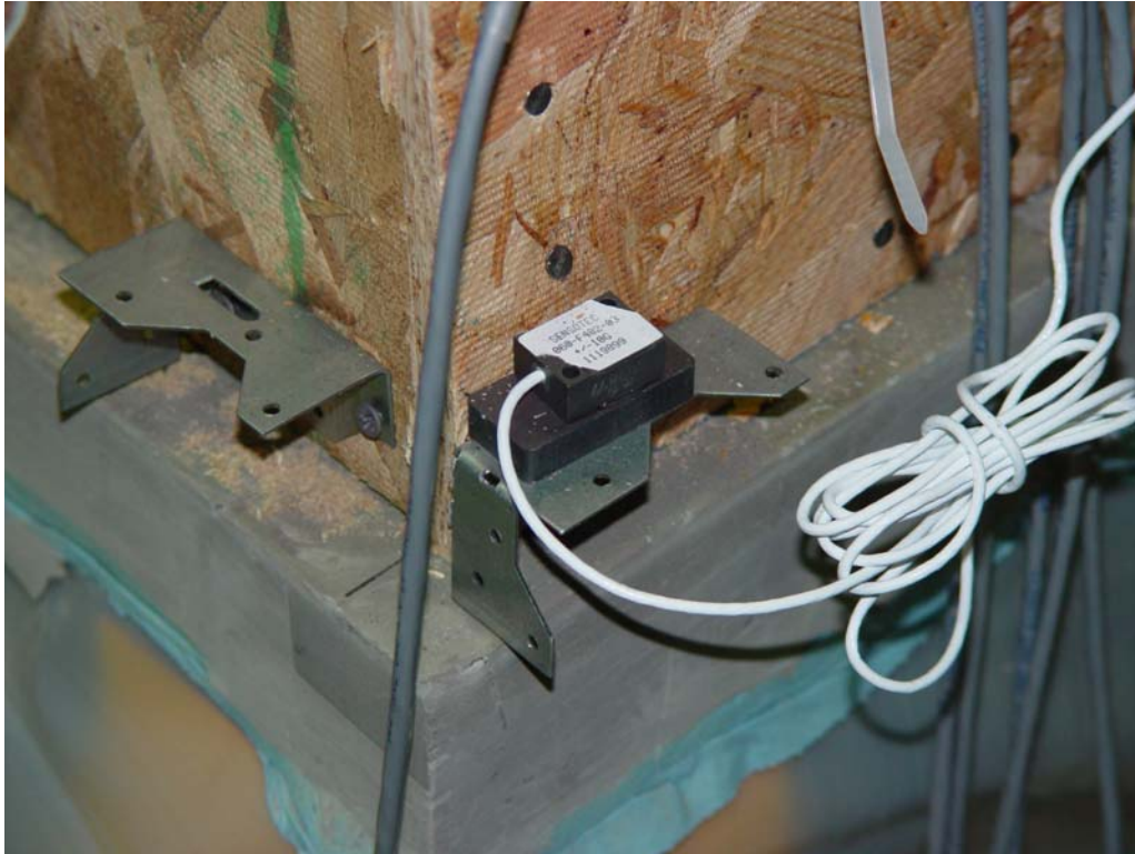
Figure 4.2: Accelerometer at the bottom corner of the structure measuring acceleration in the vertical direction
