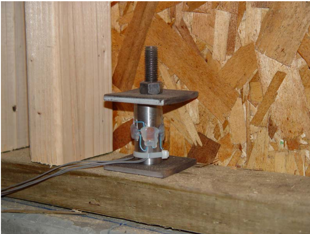
Figure 4.7: Load cell measuring tensile axial force in a shear transfer anchor bolt
