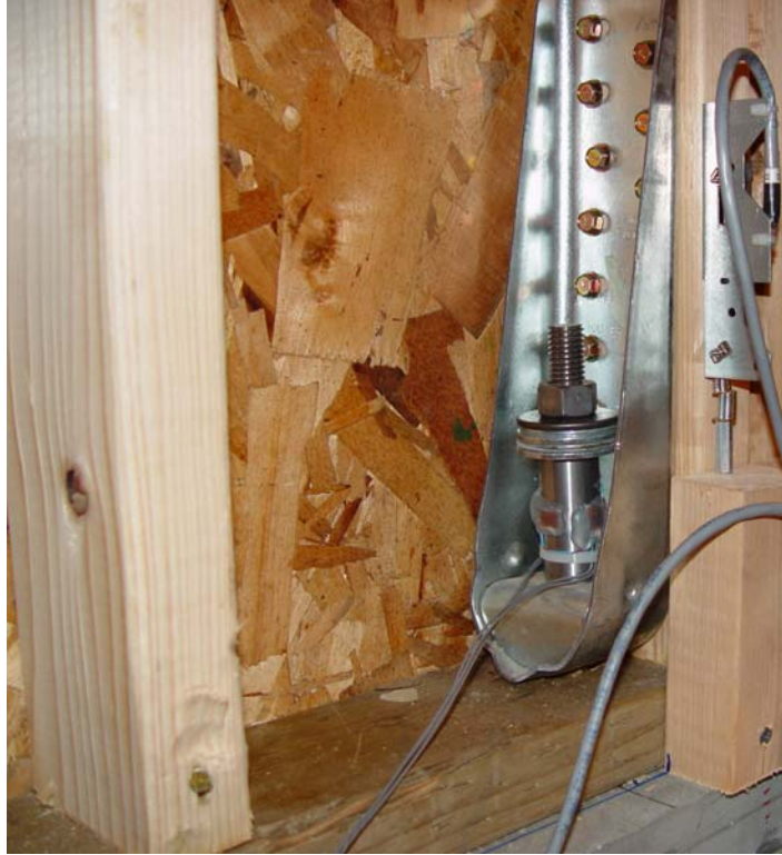
Figure 4.6: Anchor bolt load cell measuring tensile axial force in a PHD5 Holddown
