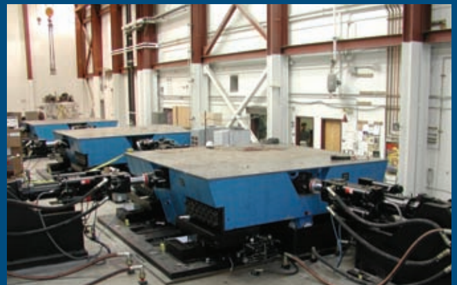
The James E. Rogers and Louis Weiner, Jr. Bridge Structures Laboratory at the University of Nevada, Reno features three identical shake tables.
