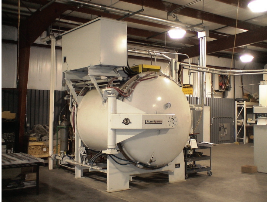
Figure 3-10 Vacuum Furnace for Annealing
