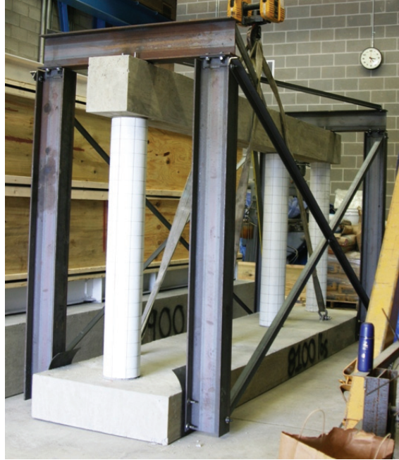
Figure 3-22 Shipping Frame for Model
