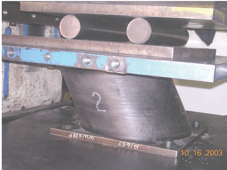
FIGURE 7-2 Lead-Rubber Bearing During High Speed Testing (Constantinou et al., 2007b)
