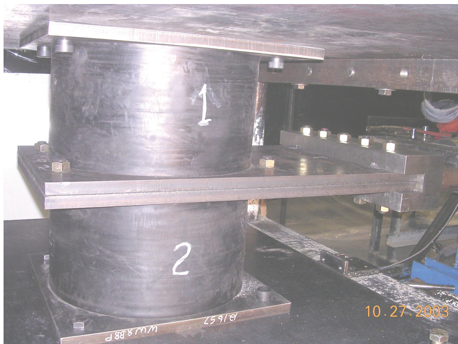
FIGURE 7-3 Lead-Rubber Bearings Tested in Pair in the 1.6km Cumulative Travel Test (Constantinou et al., 2007b)
