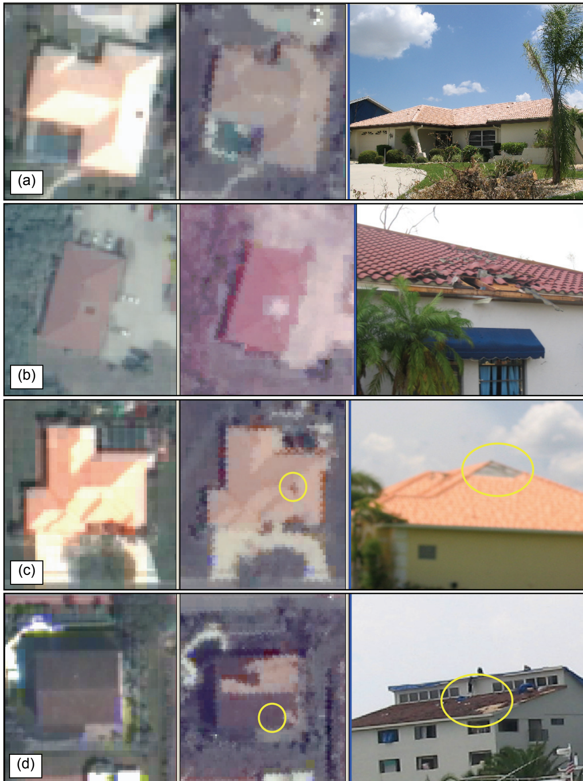
Figure 3-8 Examples of Windstorm Damage to Residential Buildings: Pre- and Post-Storm Quickbird Satellite Images and Ground-Truthing Photos. Credit: DigitalGlobe, Inc. < www.digitalglobe.com >.
