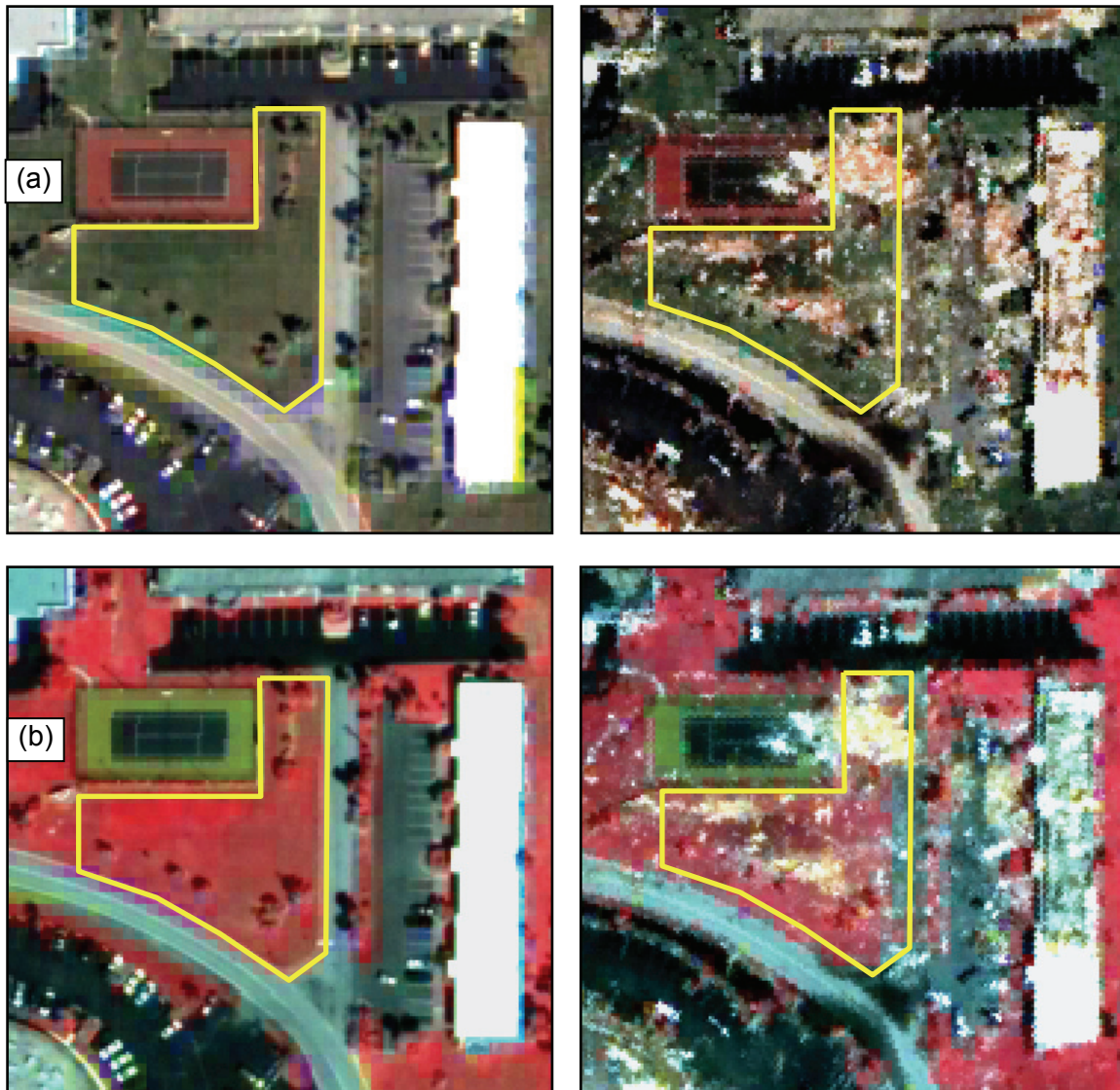
Figure 5-1 Example of Windborne Debris Spread. Quickbird Images from Before and After Hurricane Charley Show Windborne Debris from a Nearby Building Spread Across a Vegetated (Lawn) Area (Delineated in Yellow). Images are Shown in (a) Natural Color (B-G-R Bands) and (b) False-Color (G-R-NIR bands) to Highlight the Spectral Signature of Debris Atop the Vegetation Area. Credit: DigitalGlobe, Inc. < www.digitalglobe.com > and Womble (2005).
