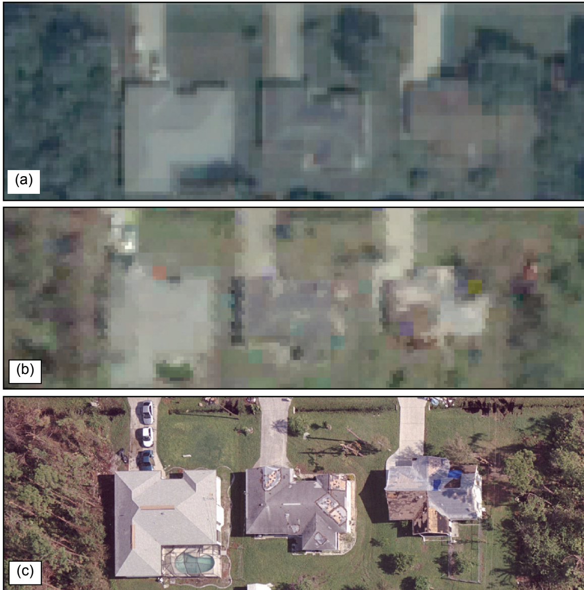
Figure 3-9 Comparison of Spatial Resolutions for Images of Residential Buildings (Hurricane Charley): (a) Pre-Storm 61-cm Quickbird Images; (b) Post-Storm 75-cm Quickbird Images; (c) Post-Storm 5-cm Digital Aerial Images. Credits: DigitalGlobe, Inc. < www.digitalglobe.com > and DMK Associates.
