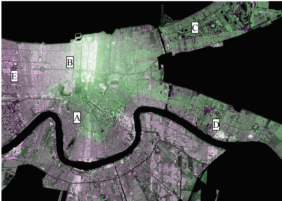
Figure 4-2 Fine Beam Mode False Color Composite Where Red = 13 th April Pre-Flood, Green = 9 th September – Flood, and Blue = 13 th April Pre-Flood
