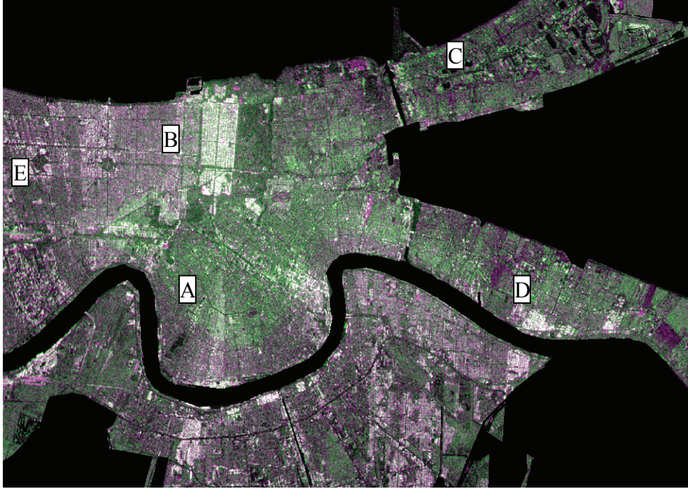
Figure 4-3 Standard Beam Mode False Color Composite Where Red = 30 th April Pre-Flood, Green = 2 nd September Flood, and Blue = 30 th April Pre-Flood
