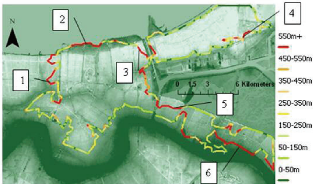
Figure 5-1 Boundary Intersection Analysis Between Fine Beam Derived Flood Boundary and SPOT Derived Validation Layer
