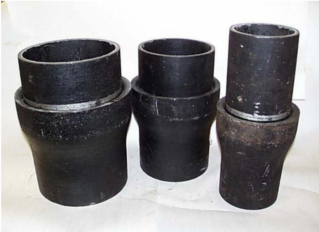
Figure 5.7 Ductile Iron Pipes with Bell-and-Spigot Push-On Joints (after American Lifelines Alliance, 2005)
