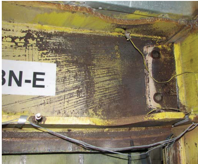
(g) Web of the intermediate HBE at the end of MCEER/NCREE testing
